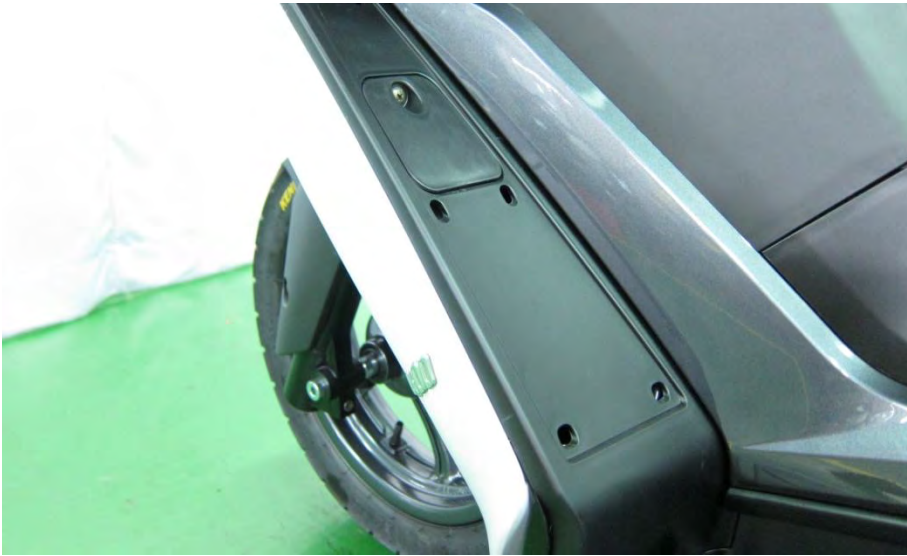
Install the engine coolant reserve tank cover. Insert the screw and tighten its securely with a #2 Phillips.
