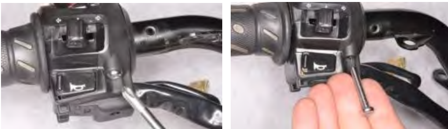
Remove the two left switch housing mounting screws with a #2 Phillips screwdriver.
