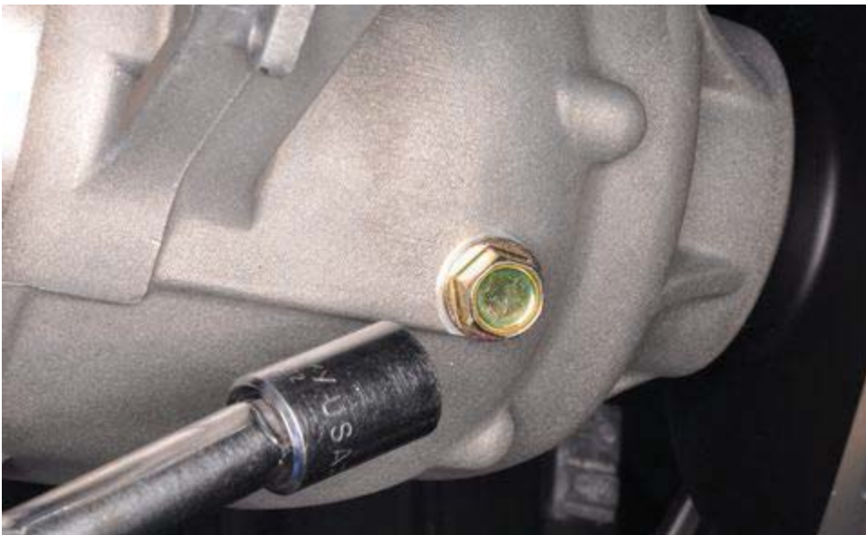
Install the oil filler plug and torque it to specification with a 12 mm socket.
