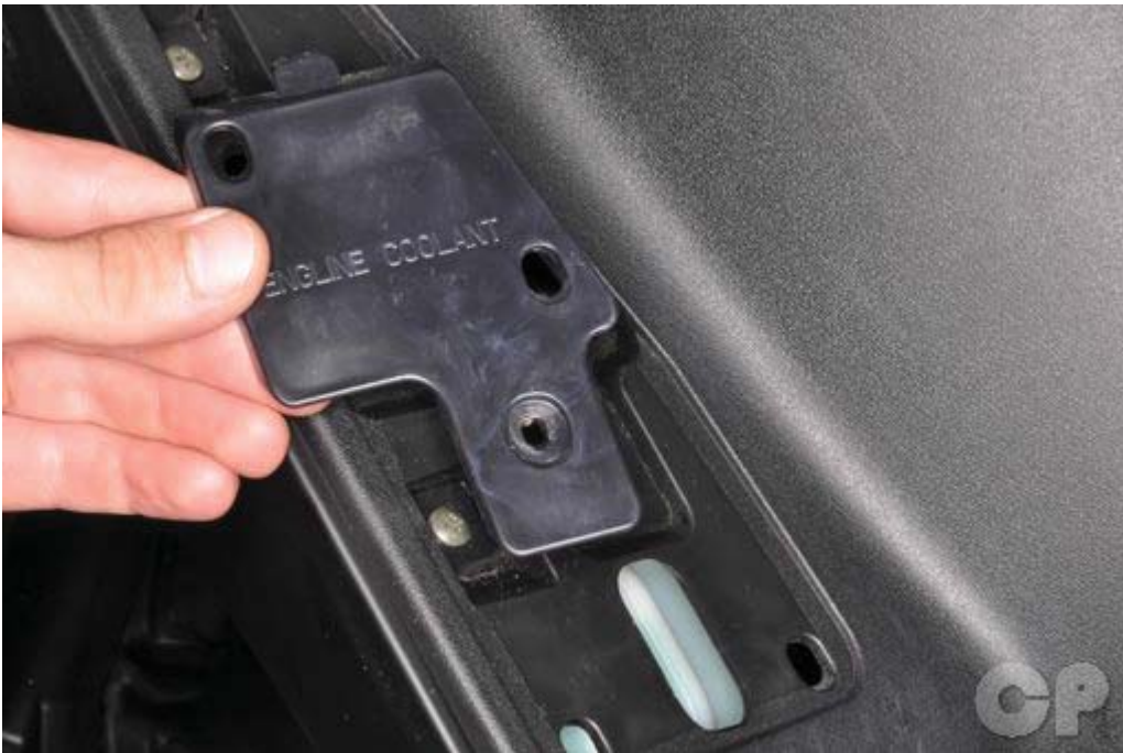
Remove the engine coolant reserve tank cover.
