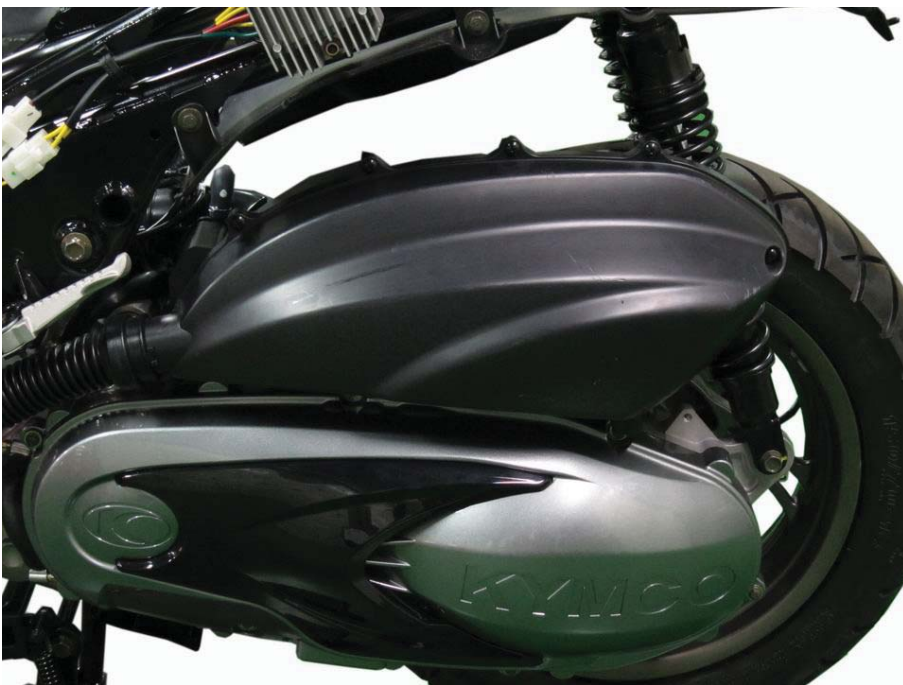
Install the 8 air filter cover screws and tighten them securely with a #2 Phillips screwdriver.
