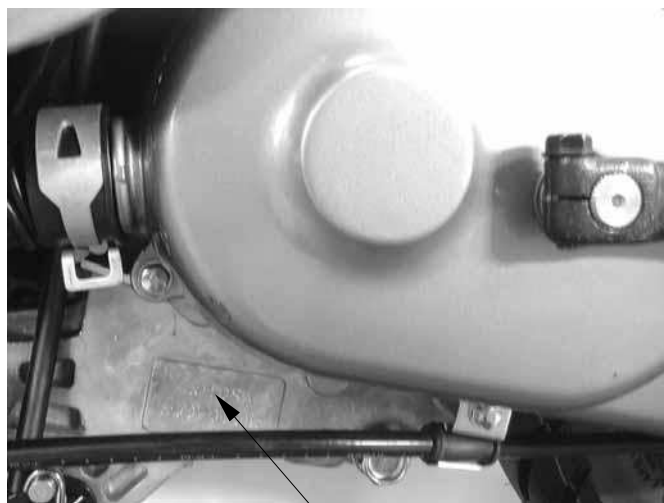
Location of Engine Serial Number
