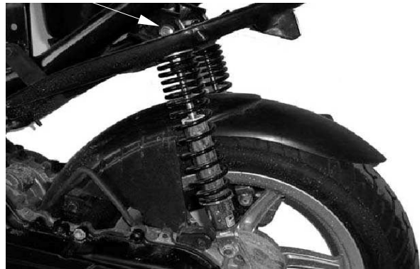
Rear Shock Absorber Upper Mount Bolt
