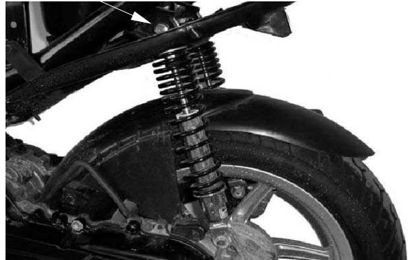
Rear Shock Absorber Upper Mount Bolt
