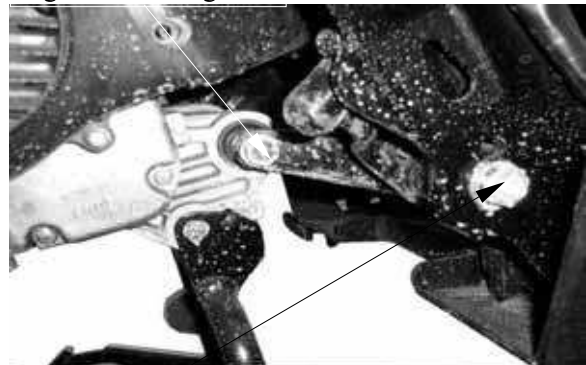
Engine Hanger Bracket Bolt
