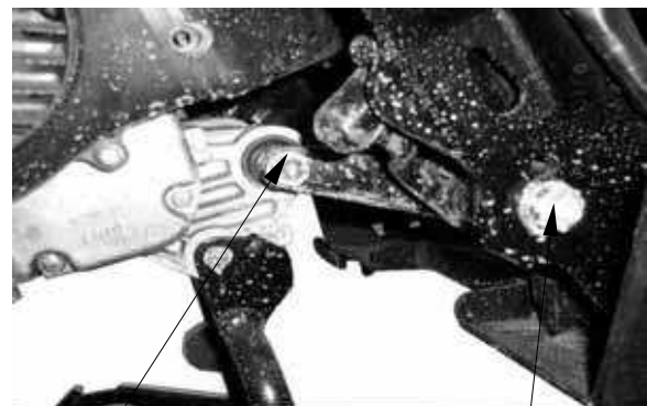
Engine Mounting Bolt
