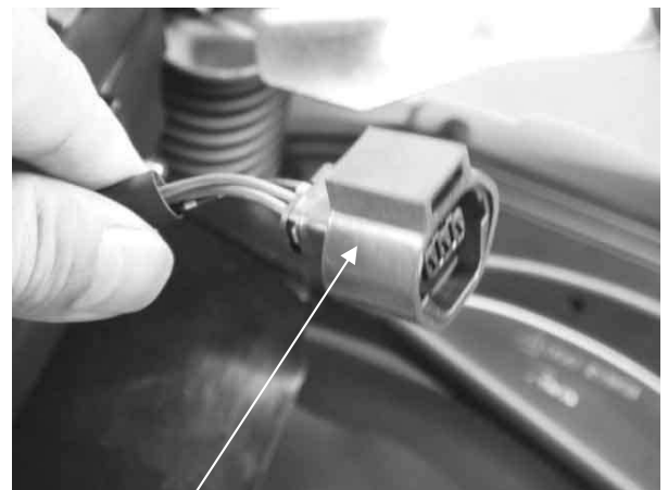
ABS diagnosis tool Connector (Near battery position)
