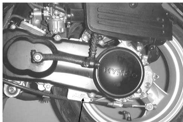
Location of Engine Serial Number
