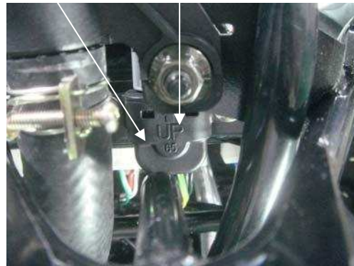
Tilt Switch "UP" Mark
