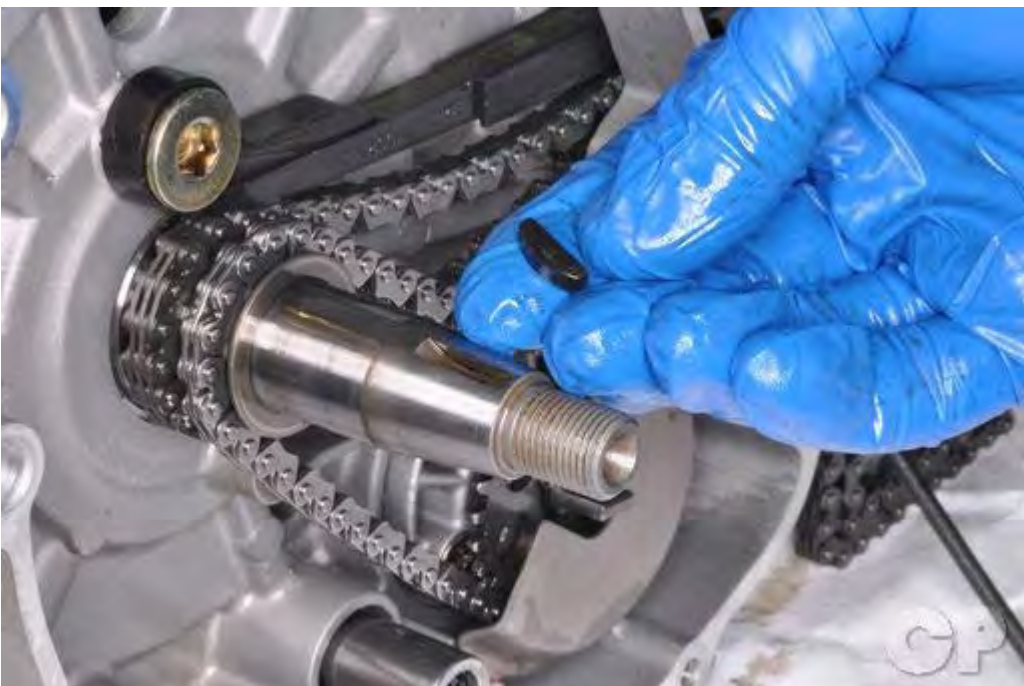
Remove the woodruff key from the crankshaft.
