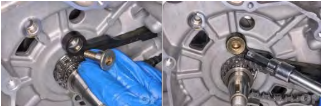
Insert the upper cam chain guide mounting bolt and tighten it to specification with an 8 mm Allen socket.
