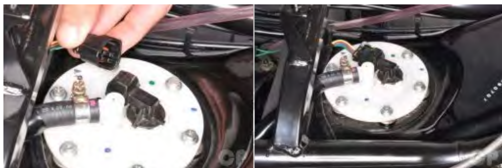
Plug in the fuel pump connector.
