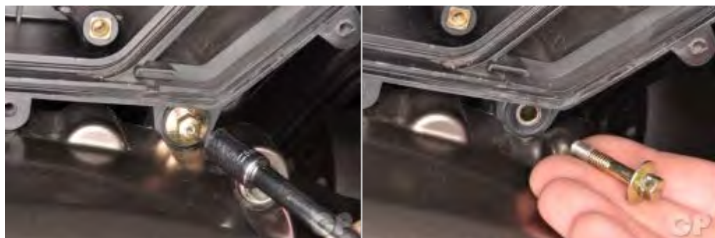
Remove the two front air box screws with an 8 mm socket.
