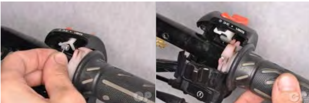
Lubricate the end of the throttle in grease. Fit the ends of the throttle cables into the throttle tube.
