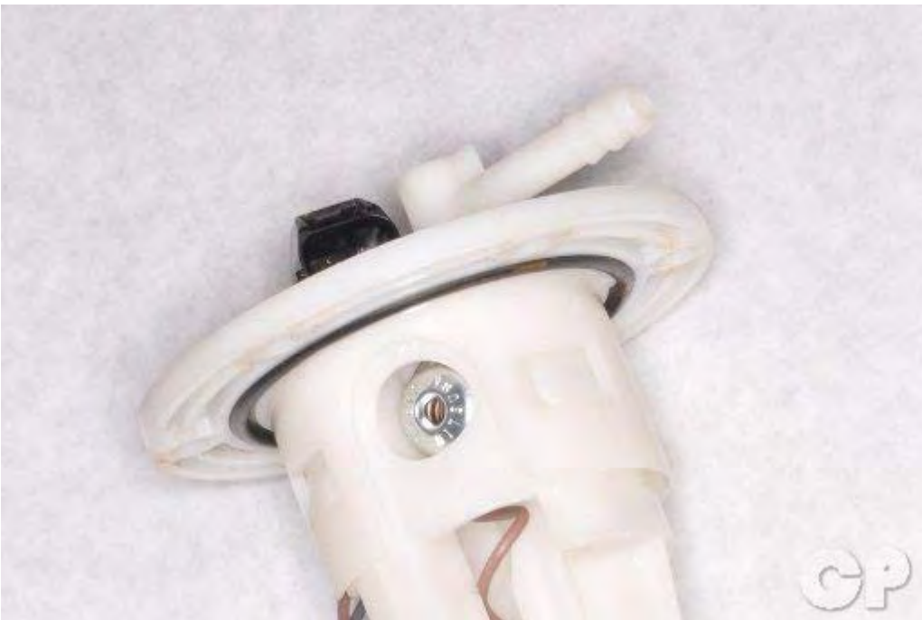
Discard the fuel pump O-ring, and replace it with a new item on assembly.
