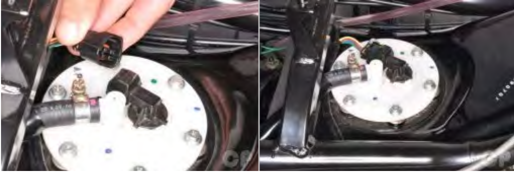
Plug in the fuel pump connecter.
