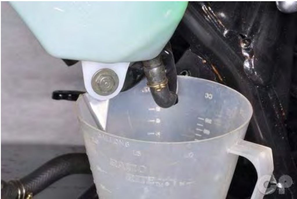
Position a suitable container below the reserve tank.
