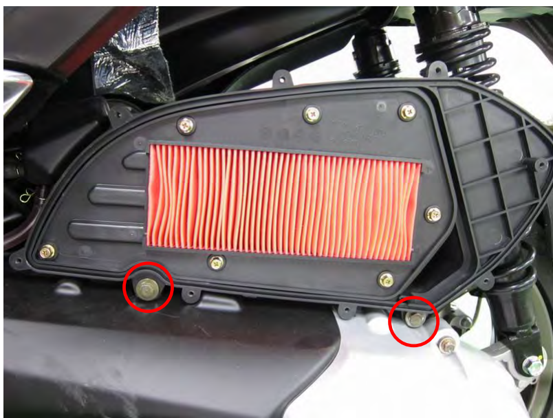
Disconnect the transmission vent hose.
