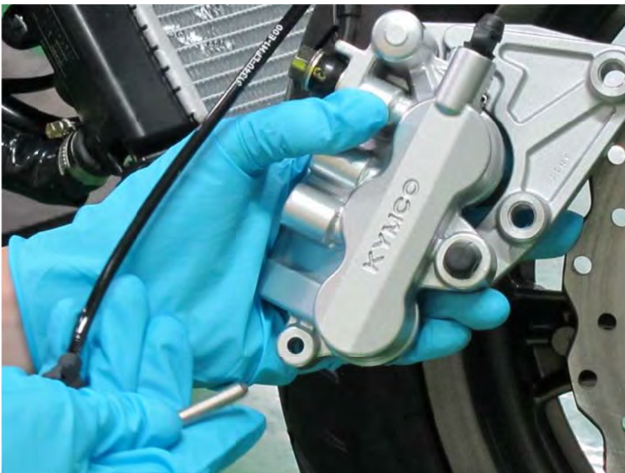
Remove the brake pad pin.
