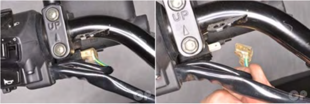
Unplug the brake light switch connector.
