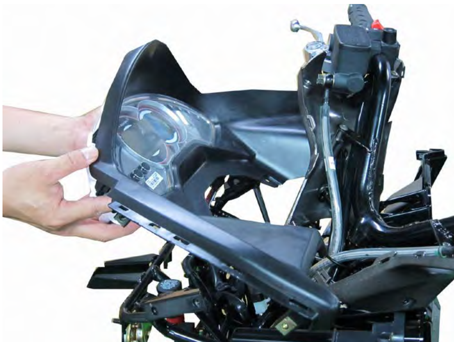
Install the speedometer assembly
