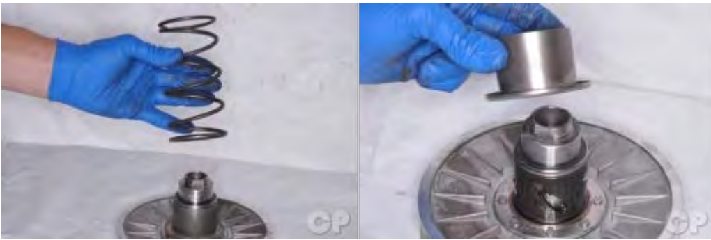
Remove the collars and spring.
