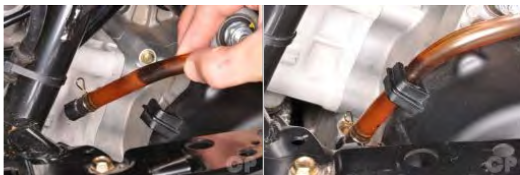
Connect the transmission vent hose.
