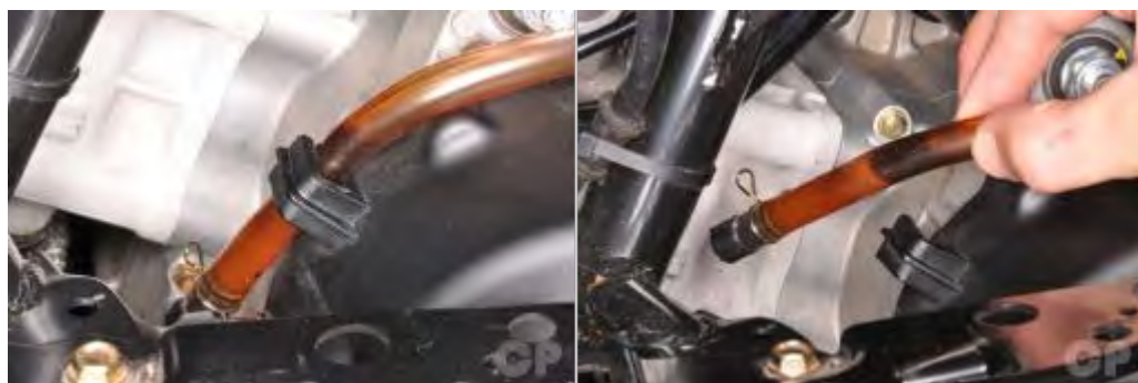
Disconnect the transmission vent hose.
