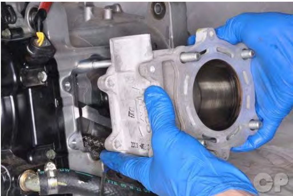
Install the new base gasket onto the crankcase.
