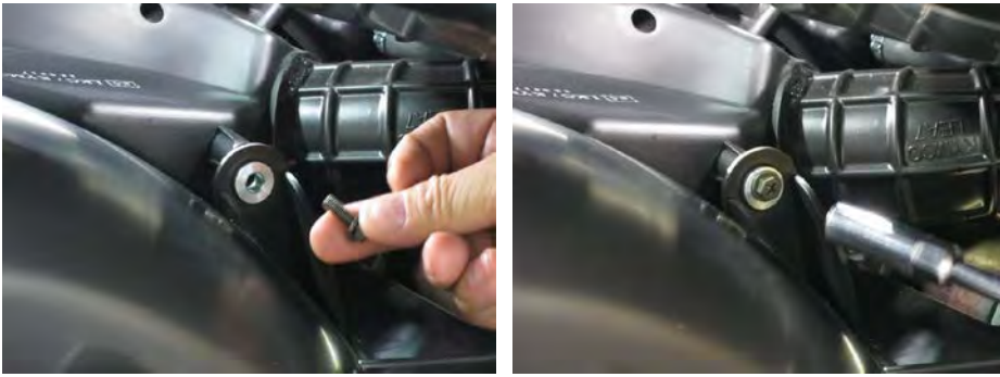
Install the fender mounting bolt with a 8 mm socket on the left side.
