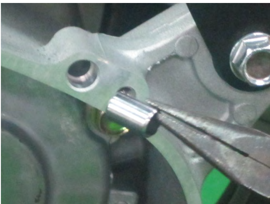
Remove the two dowel pins.
