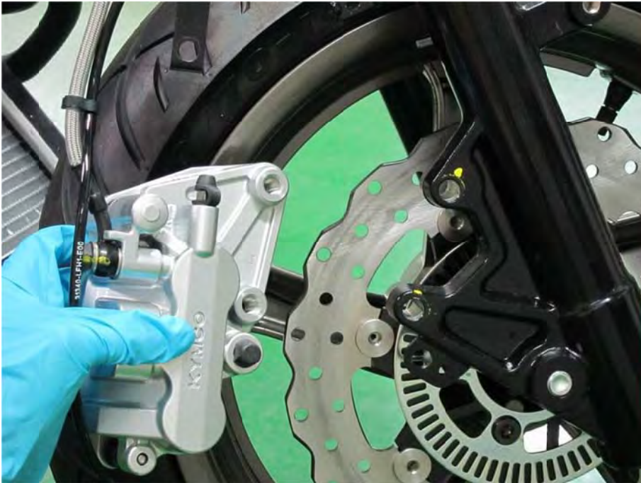
Remove the front caliper.
