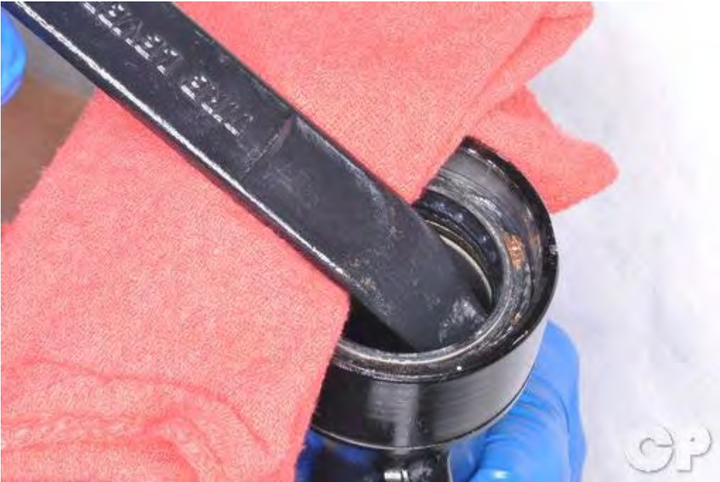
Place a rag across the top of the fork slider and pry our the oil seal as shown.
