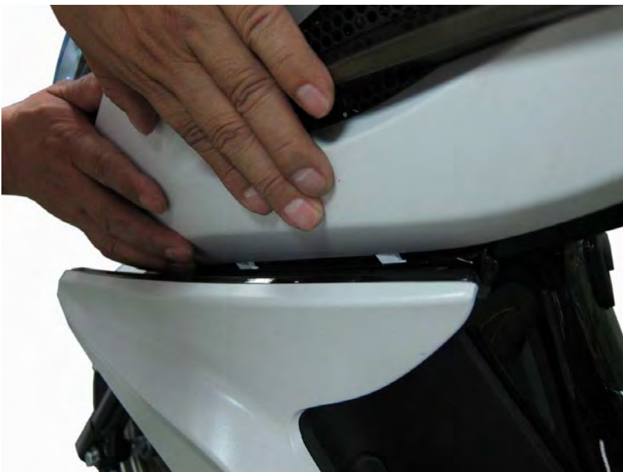
Carefully Align the side molding and side skirt with hand on each side.
