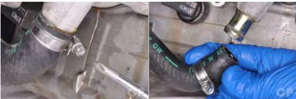
Loosen the cylinder coolant hose clamp with a #2 Phillips screwdriver. Free the coolant hose from the cylinder.
