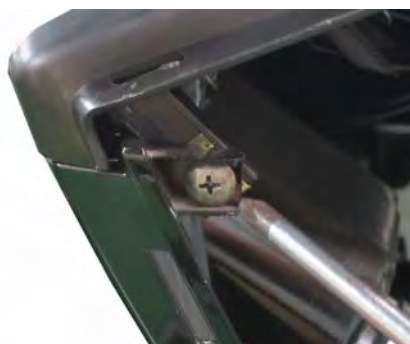
Install two screws mounting the speedometer cover on both sides with a #2 Phillips.
