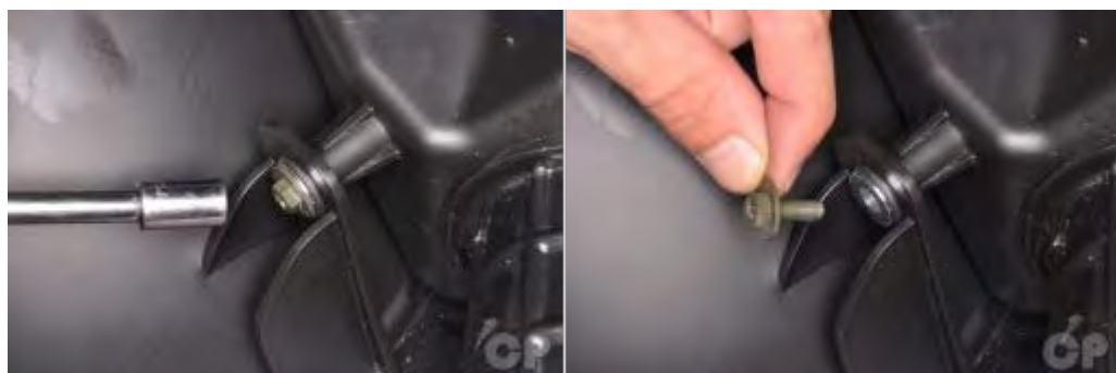
Remove the two rear air box screws with an 8 mm socket.
