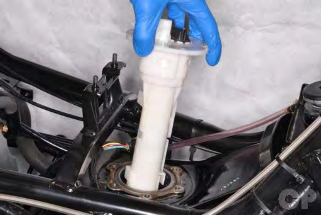
Lift the fuel pump out of the tank.
