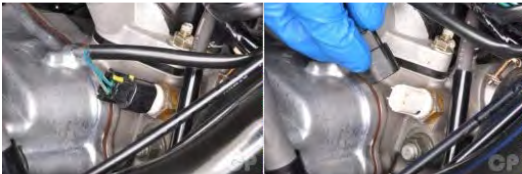
Plug in the water temperature sensor connector.
