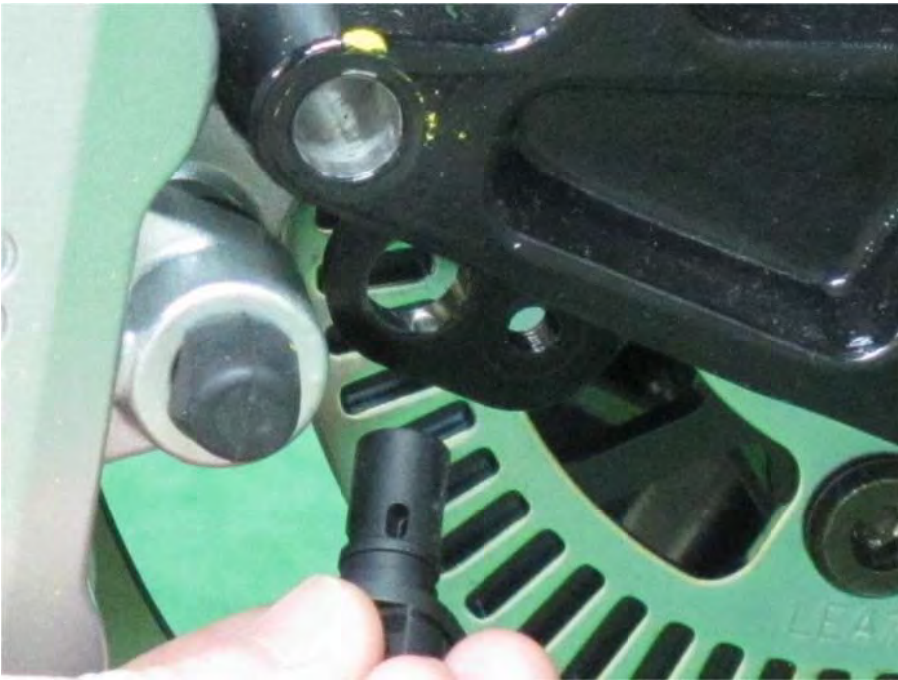
Remove the speedometer sensor.
