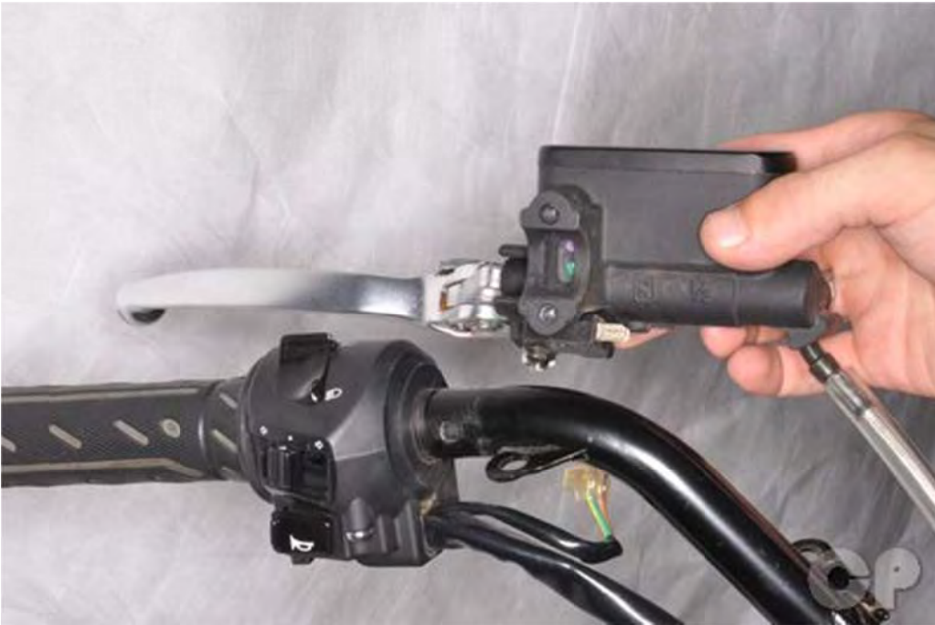
Remove the master cylinder.
