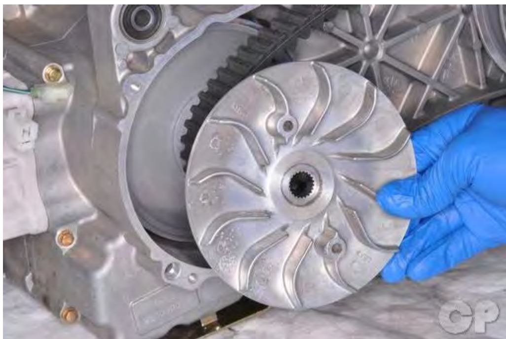
Remove the left face of the drive pulley.
