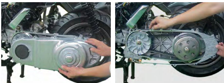
Remove the belt case cover and gasket.
