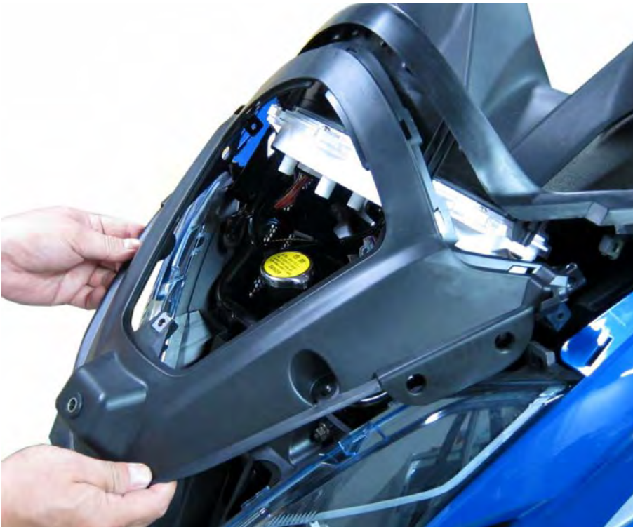
Install the front cover meter
