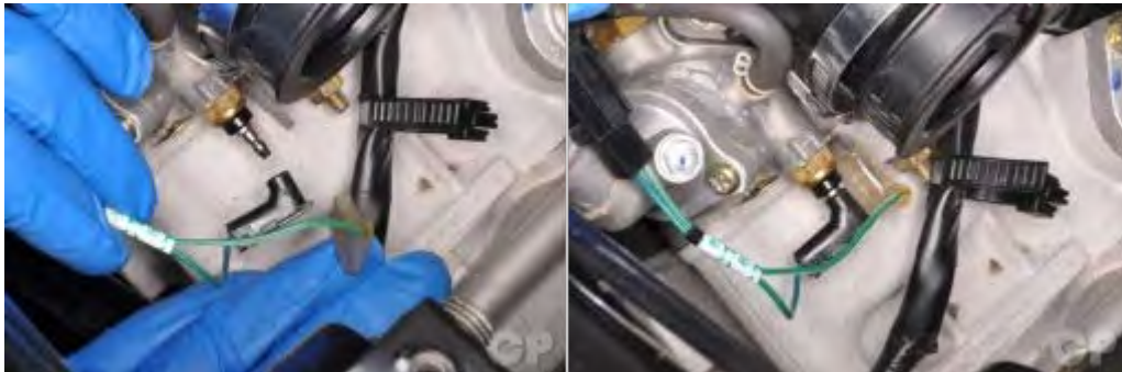
Plug in the thermo sensor unit and ground connectors.
