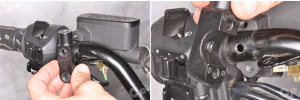
Remove the master cylinder clamp.
