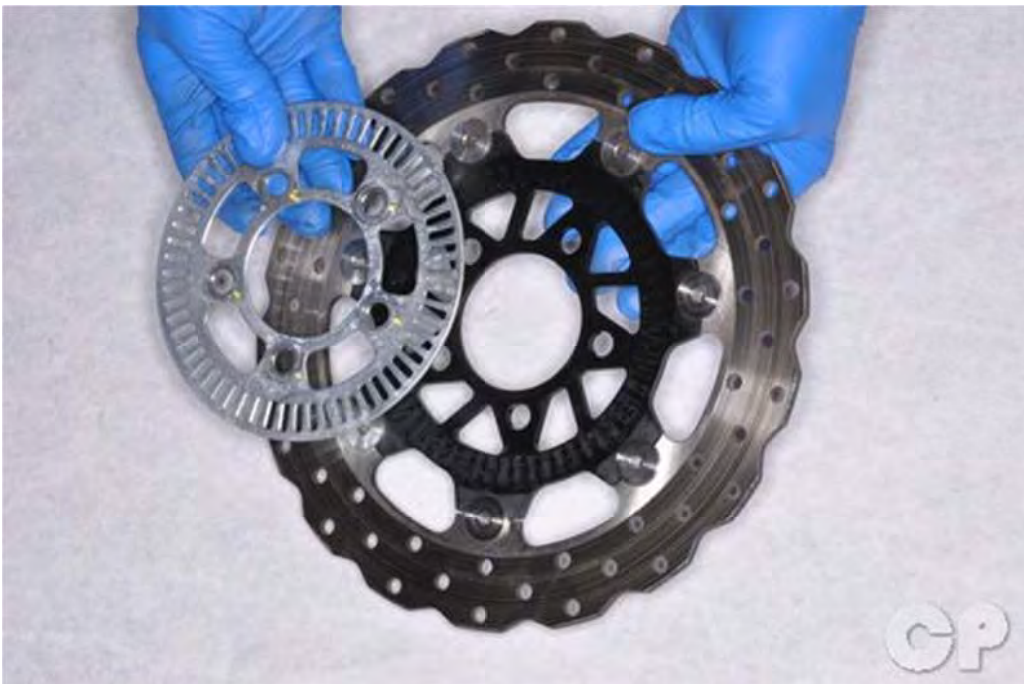
Separate the wheel speed sensor rotor from the brake disc.
