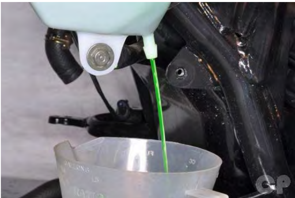
Pull back the clamp and free the overflow hose from the bottom of the reserve tank. Allow the coolant in the reserve tank to drain into the container.
