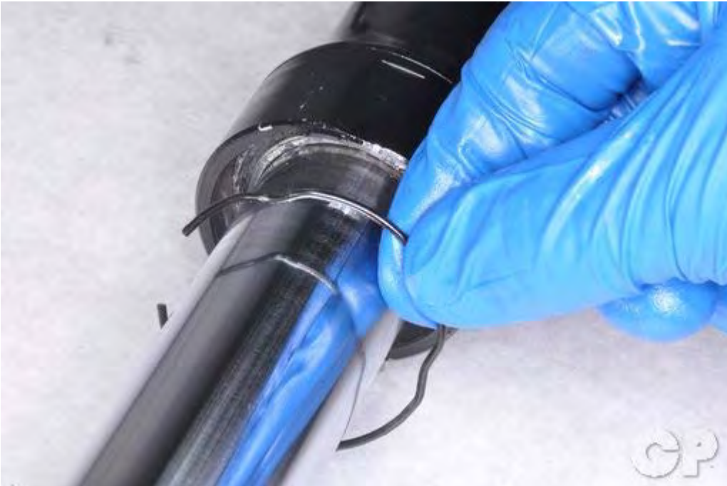
Insert the stopper ring into its groove.
