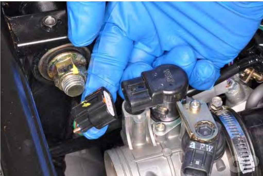
Plug in the ISC connector.
