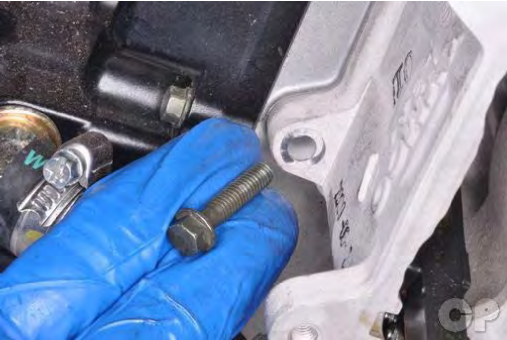
Remove the two right side cylinder bolts with an 8 mm socket.
