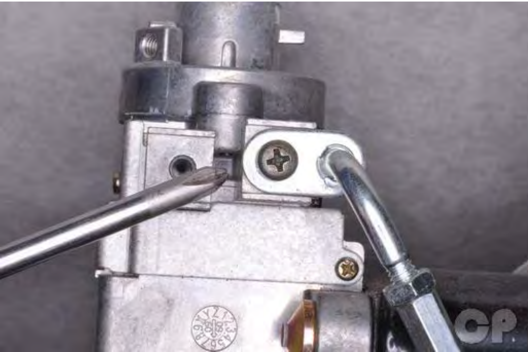
Loosen the seat latch cable screw with a #2 Phillips screwdriver.
