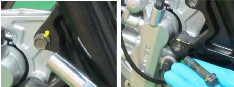
Remove the two caliper mounting bolts with a 12 mm socket.
