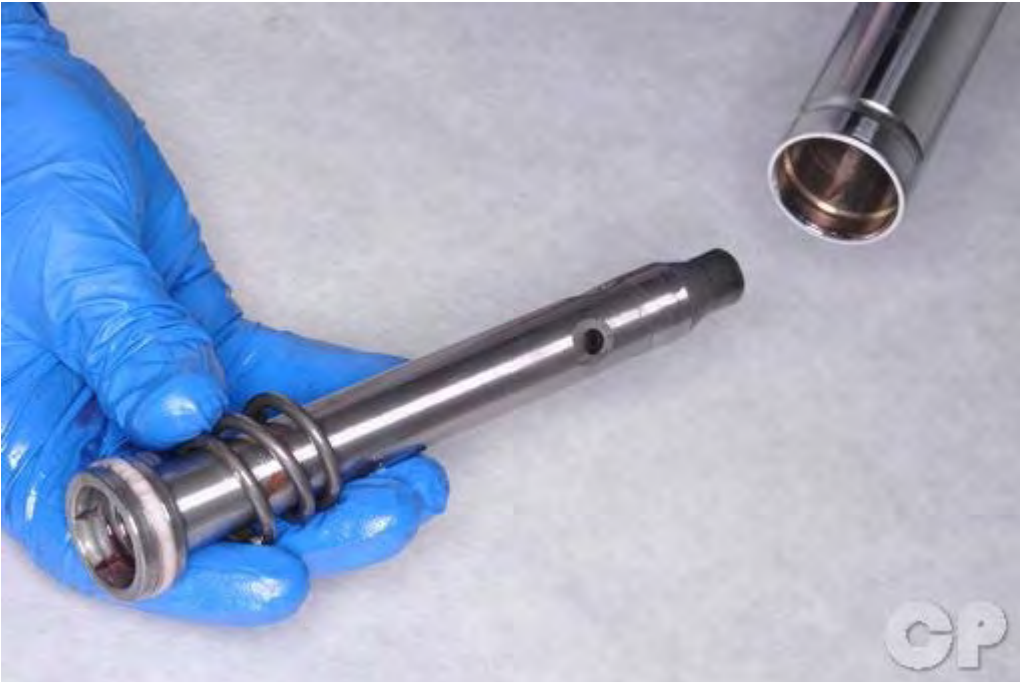
Remove the damper rod and rebound spring.
