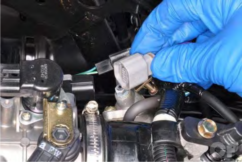
Plug in the TPS connector.
