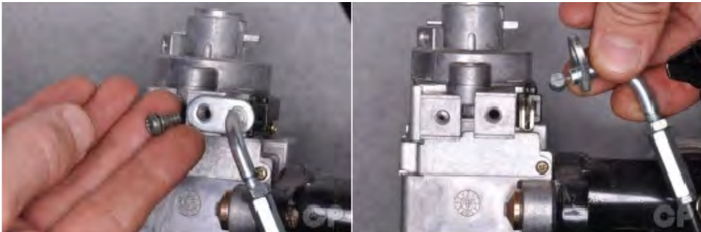
Remove the seat latch cable screw and free the seat latch cable from the ignition switch.
