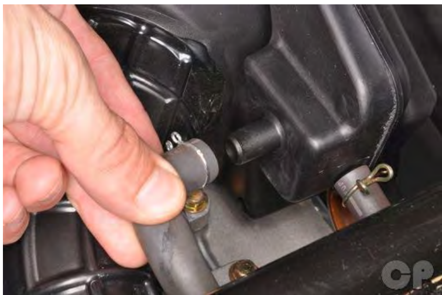
Connect the breather hose to the air box.
