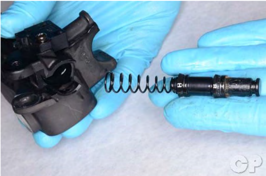
Remove the piston, spring and cups.
