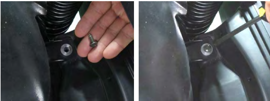
Install the connecting tube screw with a 2# Phillips.
