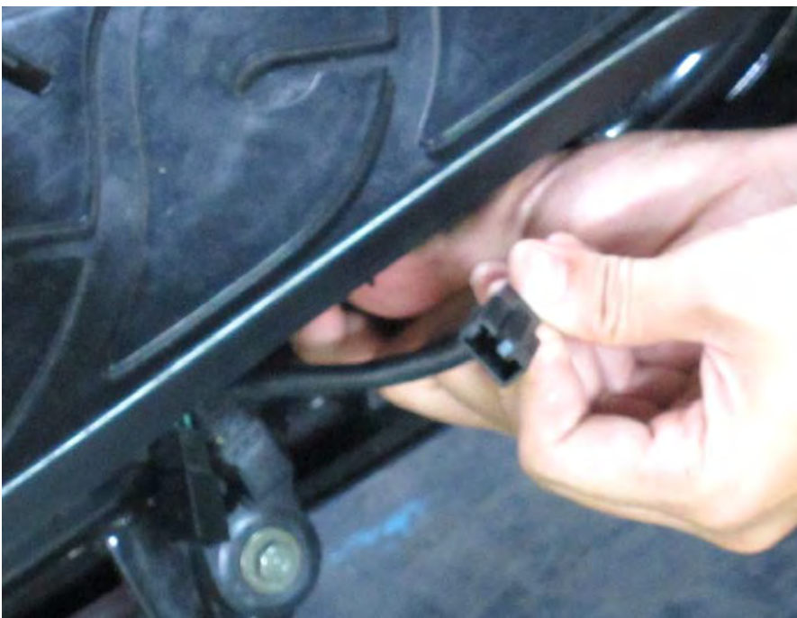
Plug in the side stand switch connector.
