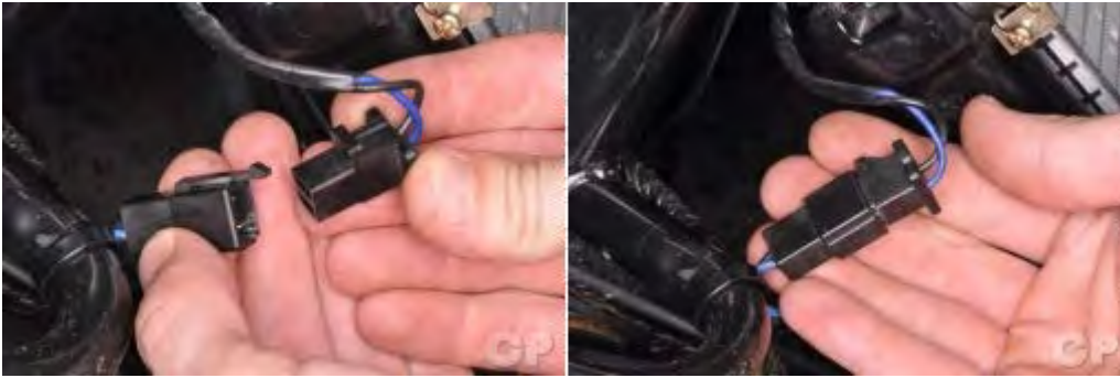
Plug in the cooling fan motor connector.
