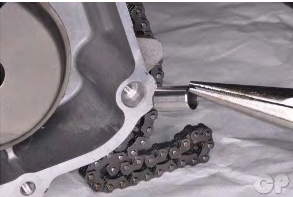
Remove the two dowel pins.
