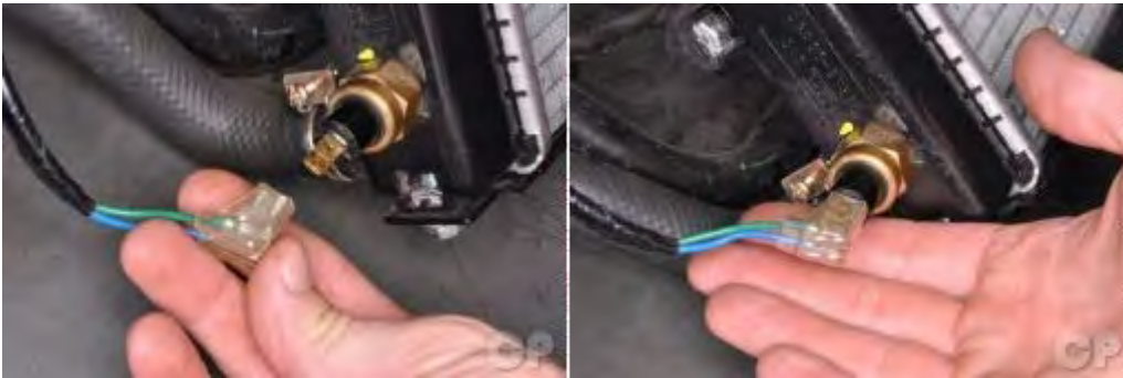
Plug in the thermostatic switch connectors.
