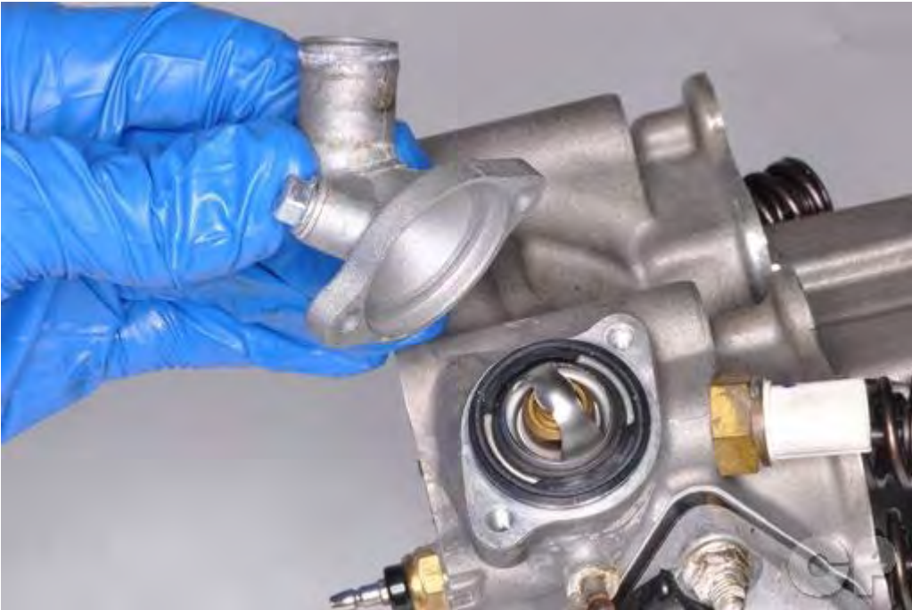
Lift off the thermostat cover.
