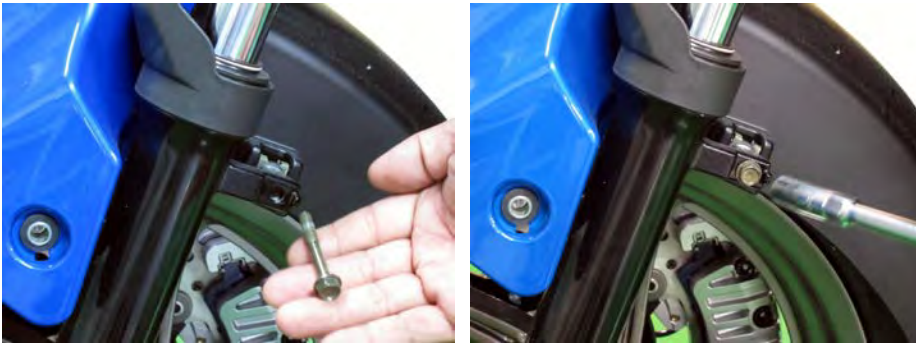
Install the left rear fender bolt with a 10 mm socket.
