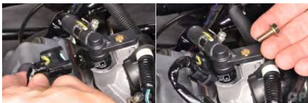
Plug in the fuel injector connector and thread in the mounting bolt.
