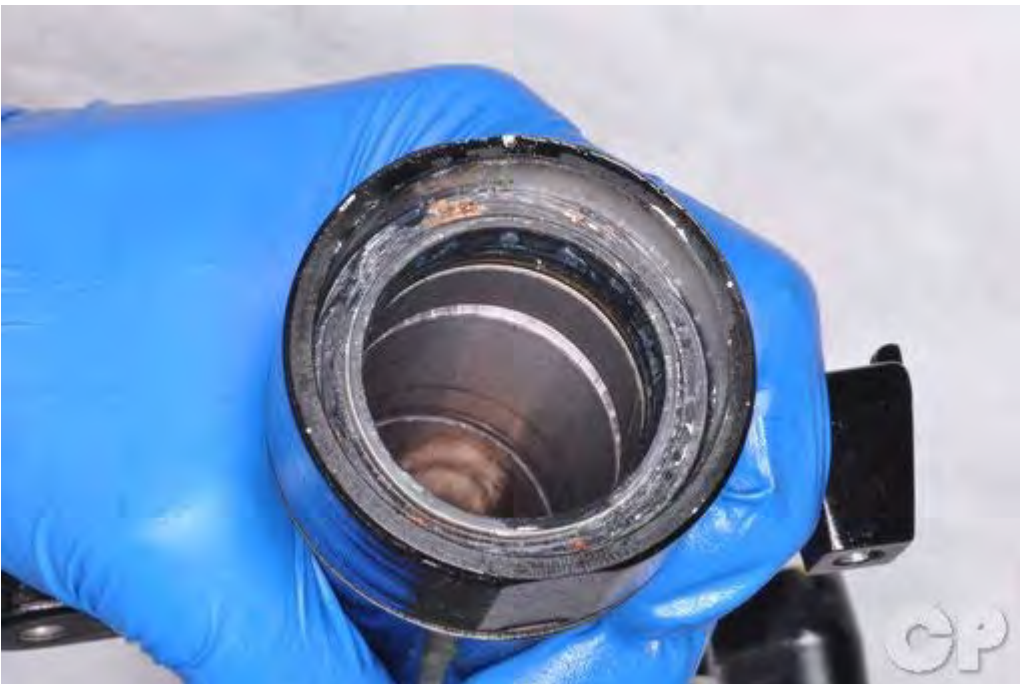
Inspect the oil seal and the bushing in the fork slider.
