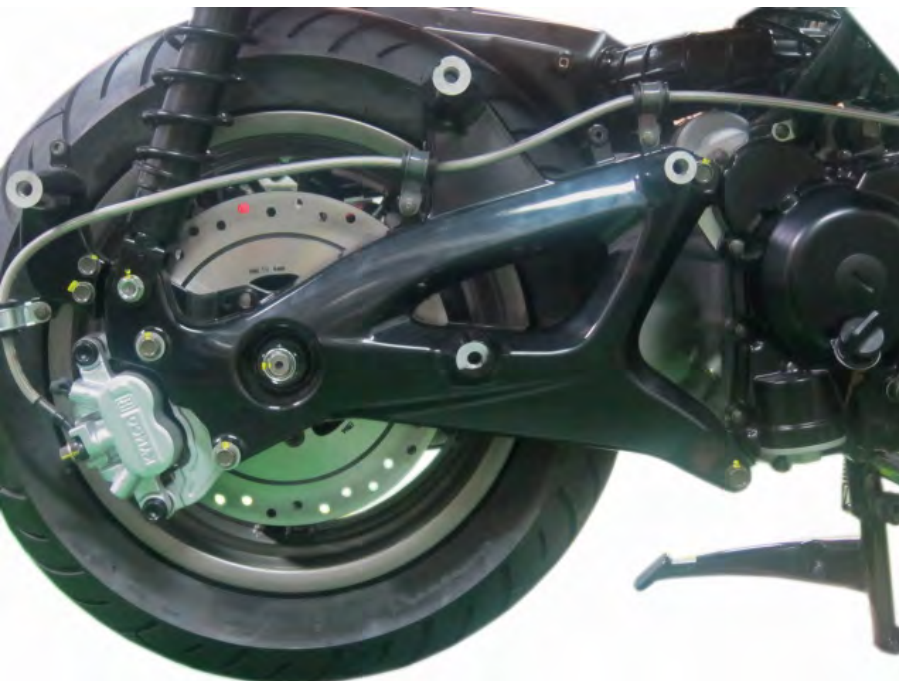
Fit the rear fork into place.
