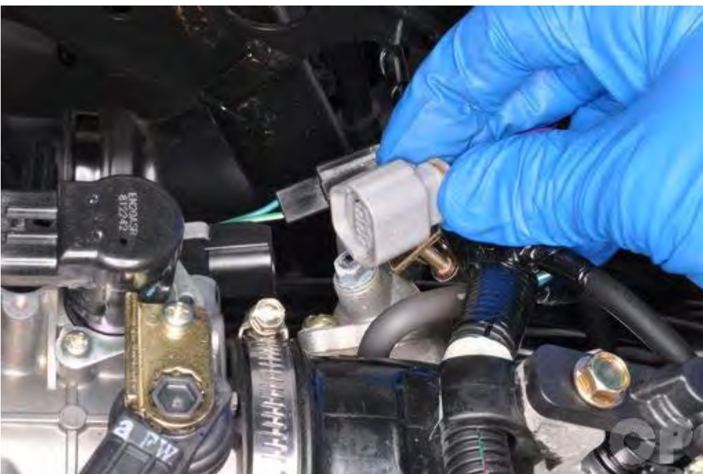
Unplug the throttle position sensor (TPS) connector.
