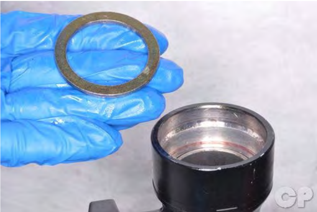
Place the spacer into the fork slider.
