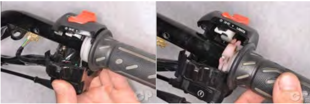
Separate the switch housing from the handlebar.
