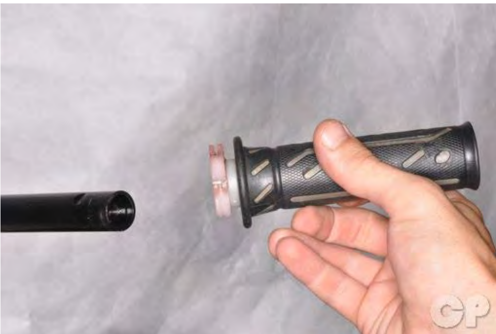
Slide the throttle grip onto the right side of the handlebar.
