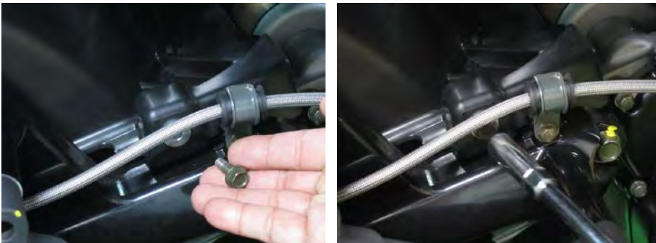
Install the connecting tube screw with a 2# Phillips.
