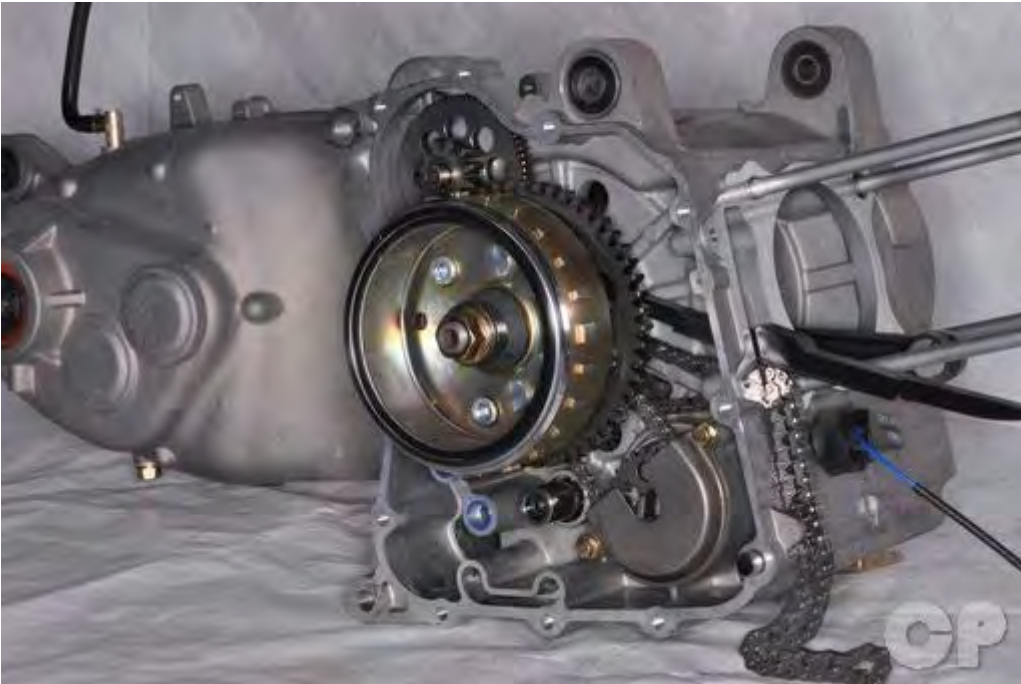
Remove the generator cover gasket.
