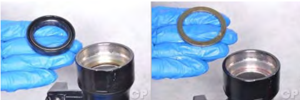
Remove the oil seal and spacer from the fork slider.
