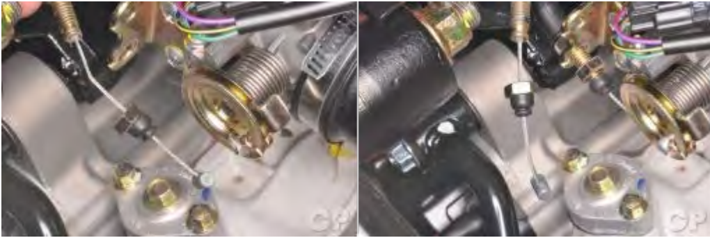
Connect the throttle cables to the throttle drum.
