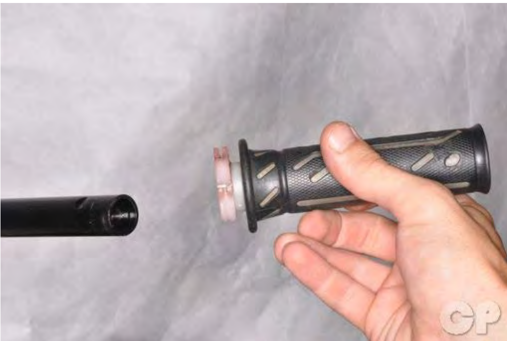
Slide off the throttle grip.
