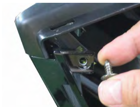
Install two screws mounting the speedometer cover on both sides with a #2 Phillips.
