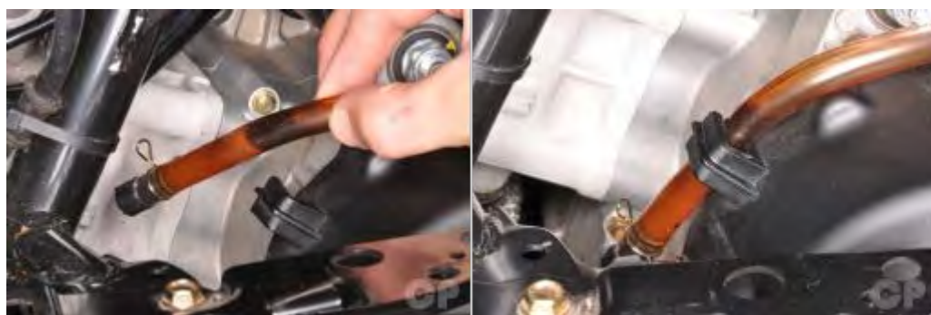
Fit the drain hose to the plastic belt case cover as shown.
