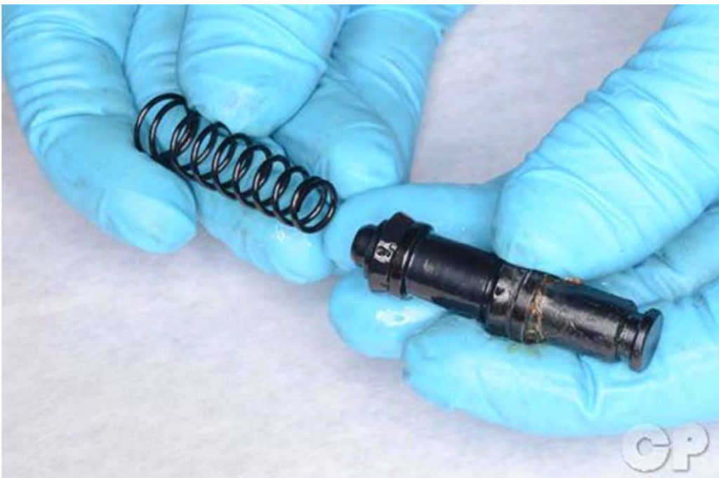
Remove the spring from the piston and
