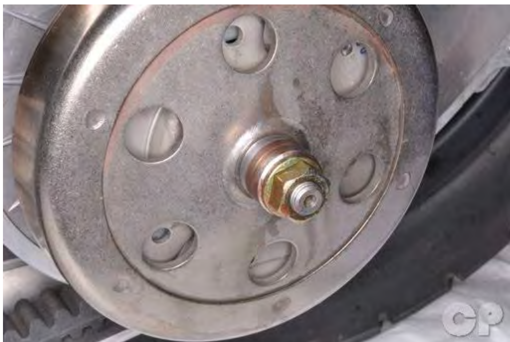
Loosen the driven pulley nut with a 19 mm socket.
