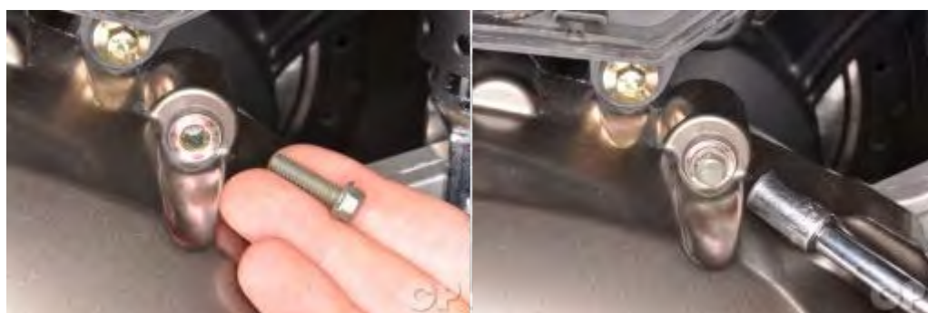
Insert the plastic cover bolts and tighten them securely with an 8 mm socket.
