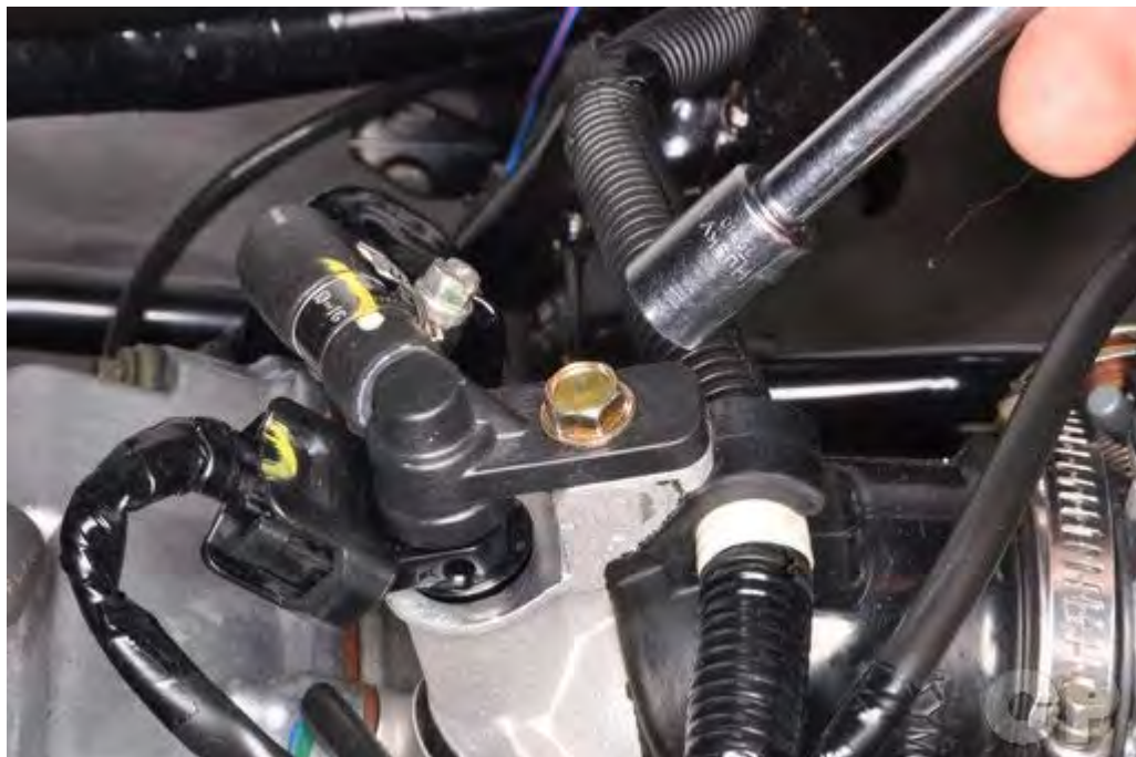
Tighten the fuel injector bolt securely with a 10 mm socket.
