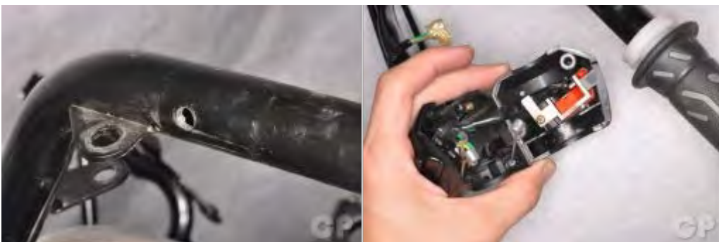
Install the right switch and throttle housing. The post on the housing should fit into the hole in the bar.
