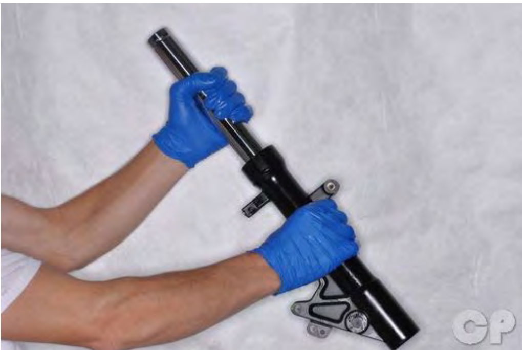
Insert the inner fork tube into the inner fork tube.
