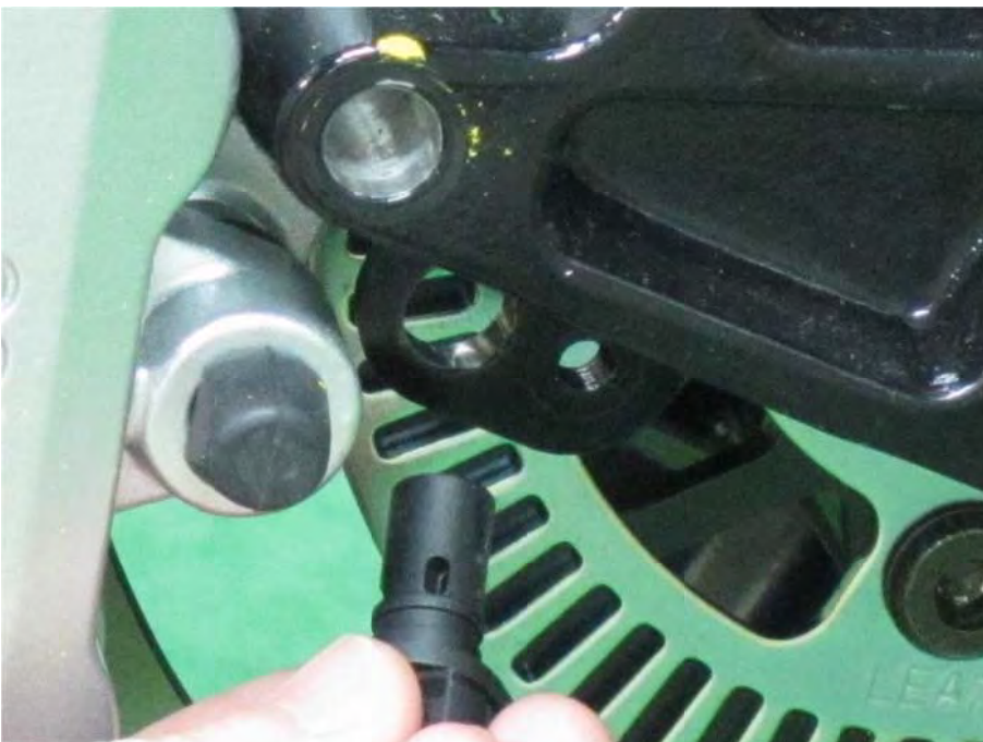
Remove the speedometer sensor.
