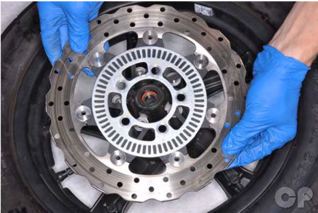
Remove the front brake disc and front wheel speed sensor rotor.
