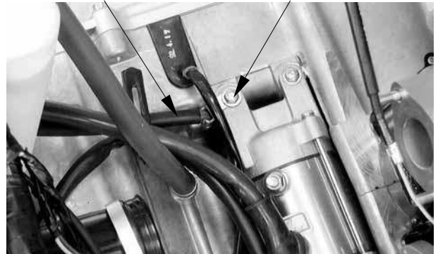
Ground Wire Bolt
