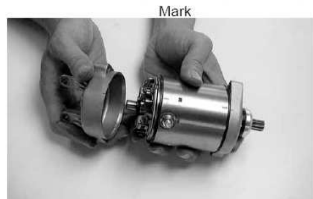
Mark O-ring Motor Case Starter Motor Cable
