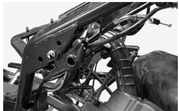
Engine Hanger Bracket Bolt Bushings
