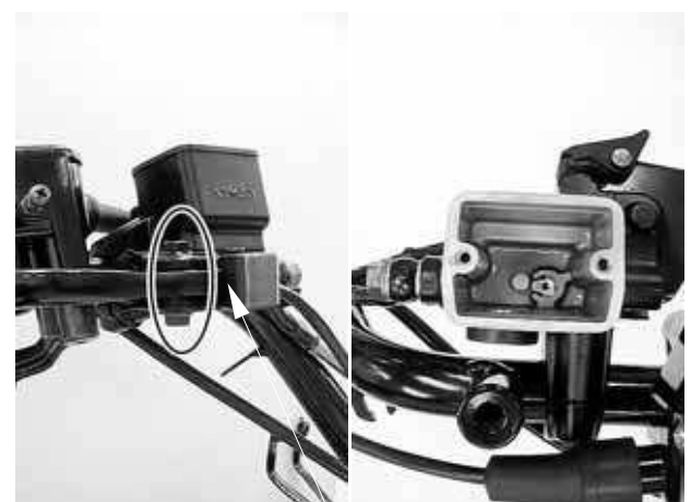
Apply grease to the dust boot
