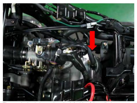
The spark plug is located on the left side of the cylinder.
