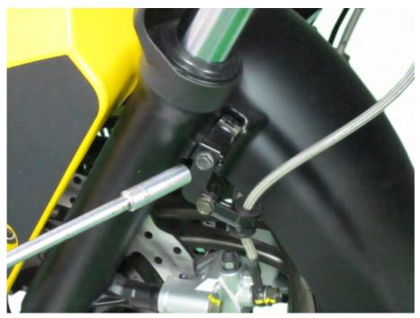
Remove the left forward front fender bolt with a 10 mm socket.
