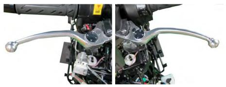
Pump the brake lever several times and hold the lever in. While holding the lever in, crack open the bleeder valve. The front brake lever will travel all the way to the grip and brake fluid and/or air will come out of the bleeder valve into the 6 mm hose. Tighten the bleeder valve before releasing the front brake lever. Pump the lever several times again and repeat the process.
