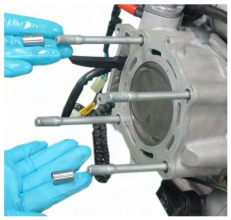
Remove the two cylinder dowel pins from the left studs. Place a clean shop towel under and around the base of the piston to prevent any parts or debris falling into the crankcase.
