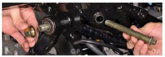
Remove the engine mounting nuts and bolts from both sides.
