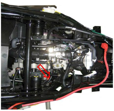
Route the starter motor lead to the starter motor and secure it in the stay on the right crankcase cover.
