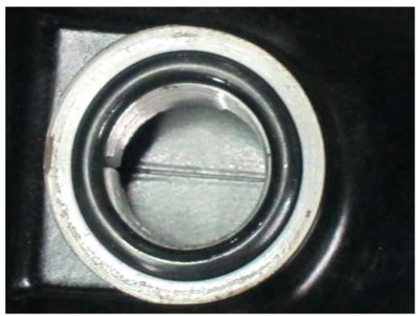
Turn crankshaft clockwise until the "T" mark aligns with the index notch in the timing inspection hole.
