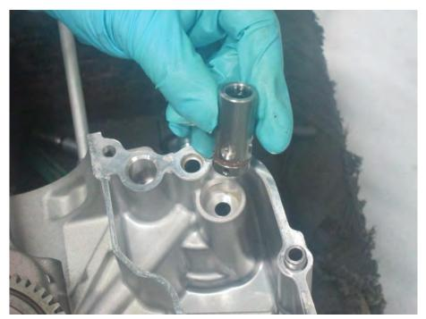
Make sure the oil release valve is in place and in good condition.
