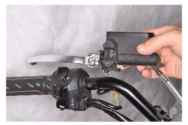
Position the master cylinder on the handlebar.
