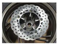
To remove the rear brake disc take out the five mounting bolts with a 6 mm Allen.
