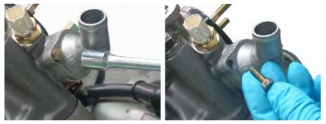
Remove the two thermostat mounting bolts with an 8mm socket.
