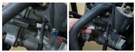
Remove the spark plug with a spark plug with a 5/8 in socket.
