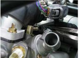
Squeeze the air bleed hose clamp with needle nose pliers and slide back the clamp. Free the air bleed hose from the thermostat.
