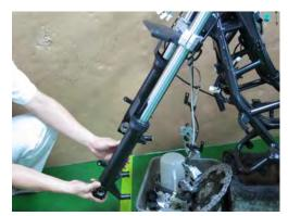
Slide the fork legs up into fork clamp using a twisting motion.
