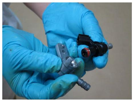
Fit the fuel injector pipe onto the top of the injector. The tab on the injector must fit into the pipe.
