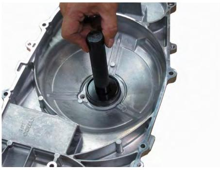
Drive in a new bearing with a suitable bearing driver that has the same outside diameter as the bearing.
