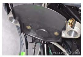
Remove the two inner front fender bolts with an 8 mm socket. Remove the inner front fender.
