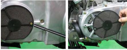
Remove 2 the air filter bolts with an 8 mm socket.
