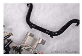
Remove the handlebar.
