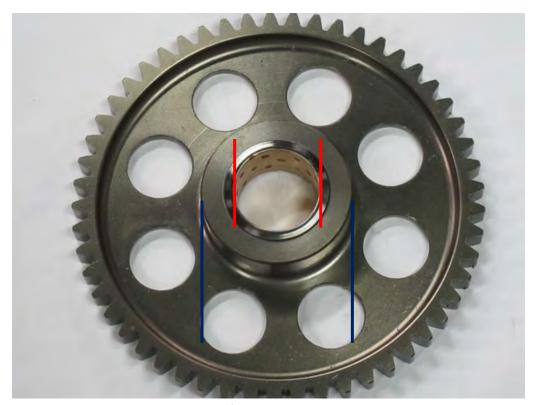
Inspect the starter driven gear for wear and damage. Measure the inside and outside diameter of the starter driven gear and replace it as needed.
