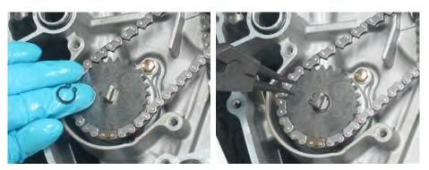
Install a new snap ring into its groove with snap ring pliers.
