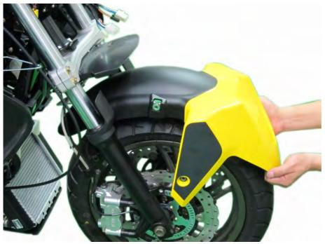
Remove the front fender from the forks.
