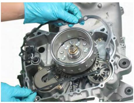
Remove the generator cover gasket.
