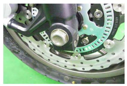
Loosen the front axle with an 24 mm socket.
