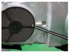
Install 2 the air filter bolts with an 8 mm socket.
