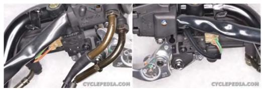
Plug in the brake light switch connectors.
