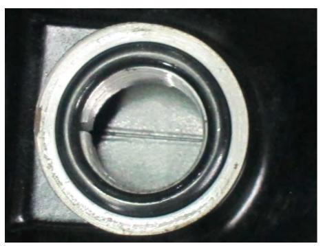
Position the piston at top dead center as above. The "T" mark should be aligned with the index notch in the timing inspection hole. Support the cam chain if the crank must be turned to position the piston correctly.
