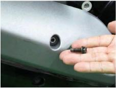
Remove the four muffler heat shield bolts with a 10 mm socket.
