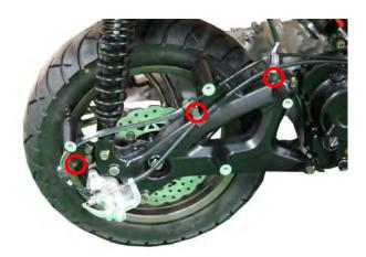
Remove the three rear wheel hose clamp bolts with an 8 mm socket.
