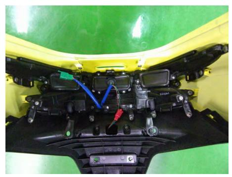
Remove the taillight mounting the tail light housing.
