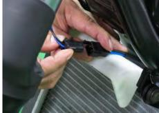
Unplug the cooling fan motor connector.
