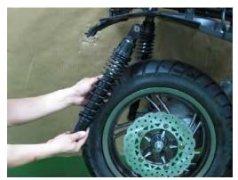
Install the upper shock absorbers. Insert the upper mounting bolt first. Tighten the bolts to specification with a 14 mm socket.
