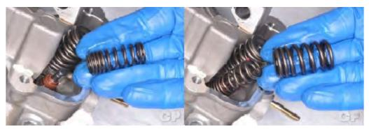
Install the valve springs. The tightly coiled end of the springs should sit against the spring seat.
