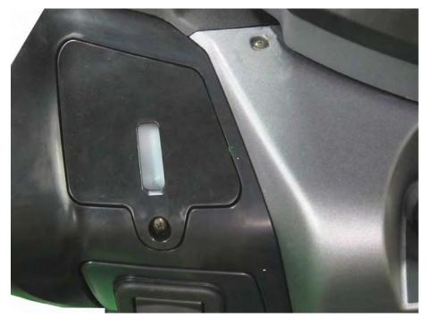
Install the engine coolant reserve tank cover. Insert the screw and tighten its securely with a #2 Phillips.
