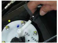
Loosen the fuel hose clamp with a special tool A120F00030. Slide back the clamp and free the injector fuel hose from the fuel pump pipe. Clean up any remaining fuel immediately.
