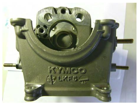
Inspect the camshaft bearing journals for scoring or scratches.
