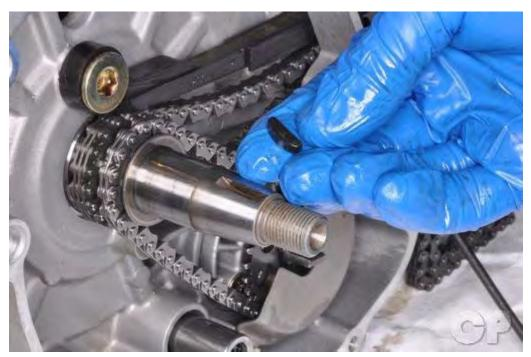
Install the woodruff key into its slot on the end of the crankshaft.
