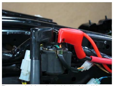
The starter relay is located on the right side of the vehicle.
