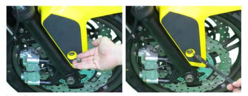
Install the forward front fender bolts with a 6 mm Allen on both side.
