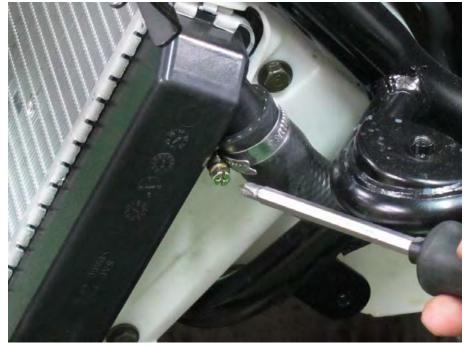
Connect the coolant hose clamps with a #2 Phillips screwdriver.
