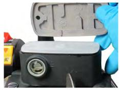
Place the rubber diaphragm, plastic piece and cover over the reservoir.
