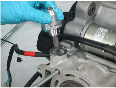
Lift the cam chain tensioner out of the cylinder. Remove the cam chain tensioner gasket.
