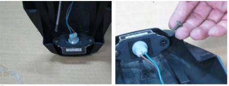
Remove the two license light assembly screws with a screwdriver.
