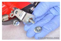
Remove the parking brake lock nut.
