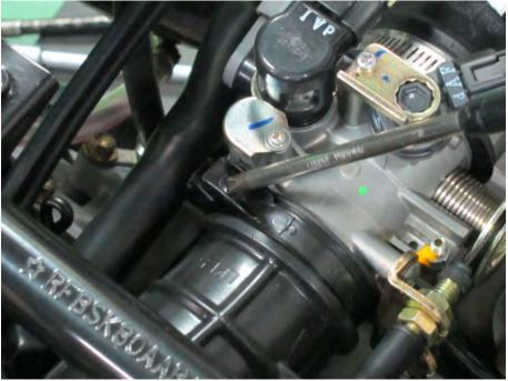
Tighten the air box connecting hose clamp screw at the throttle body with a #2 Phillips screwdriver.
