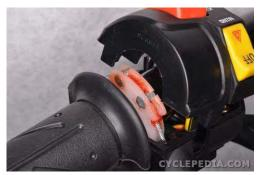
Disconnect the throttle cables from the throttle tube.
