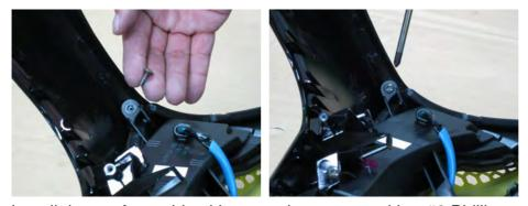
Install the ten front side skirt mounting screws with a #2 Phillips.
