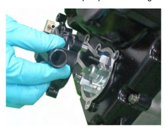
Install the two dowel pins into the generator cover and set a new water pump cover gasket in place.
