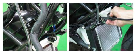
Route the filler neck coolant hose through the guide to the top left of the radiator.
