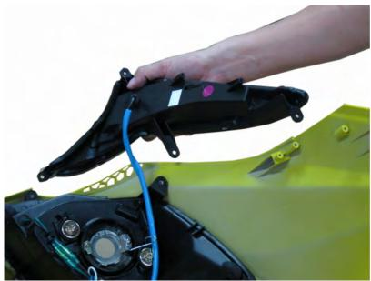
Install the turn signal light assembly.
