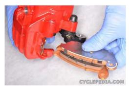
Fit the brake pads into place.
