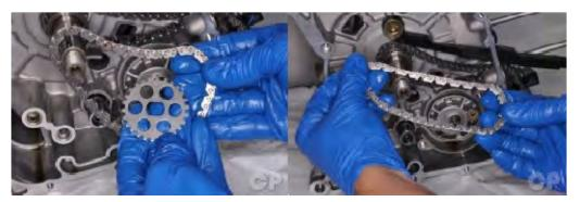
Inspect the oil pump drive chain and sprocket for signs of wear and damage. Replace the parts as needed.
