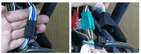
Unplug the black connector for the left handlebar switches.
