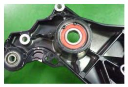
Remove the seal and snap ring.
