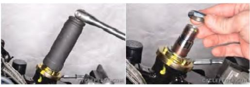
A special lock nut wrench is needed to loosen the steering stem lock nut. Remove the steering stem lock nut.
