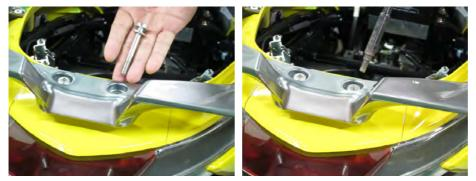
Install the two upper carrier bolts with a 6 mm Allen.
