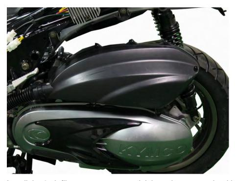
Install the 8 air filter cover screws and tighten them securely with a #2 Phillips screwdriver.
