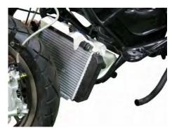
Slide the radiator to the left and free the grommet from the post above the right side of the radiator.
