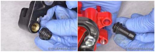
Remove the caliper bracket pin boots and inspect them for damage and deterioration. Replace the boots as needed.
