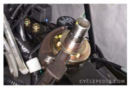
Loosen the steering stem adjusting nut with the special tool or a pin spanner.
