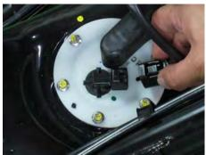
In order to drain the fuel from the fuel pipe and release the fuel pressure unplug the fuel pump connecter. Start the engine and let it run until it dies of fuel starvation. Turn the ignition switch off.
