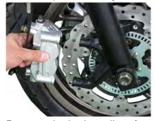
Remove the brake caliper from the fork leg.
