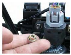
Remove the two tilt switch bolts with a 10 mm socket.
