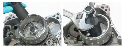
Apply a protect stay to the threads of the crankshaft before using it. Hold the tool with a large wrench and turn in the bolt until the pressure separates the flywheel from the crankshaft.
