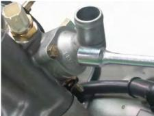
Insert the two thermostat bolts and tighten them securely with an 8mm socket.
