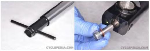
Use a suitable damper rod holder tool and loosen the fork bottom bolt with an 8 mm Allen socket. If a damper rod holder tool is unavailable temporarily reinstall the fork components. Discard the sealing washer.
