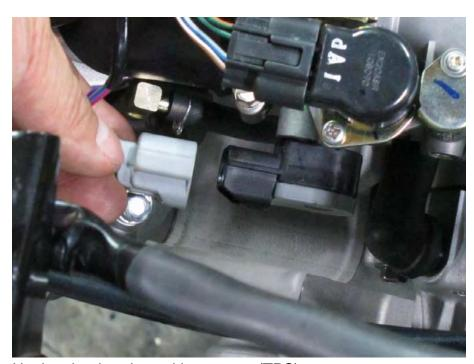
Unplug the throttle position sensor (TPS) connector.
