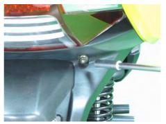
Install the two lower body cover nuts and tighten securely with a 10 mm socket.
