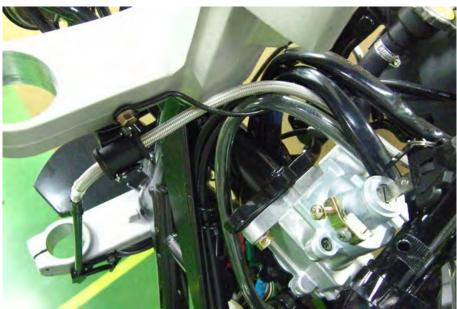
Remove the wire and cable guide bolts with an 8 mm socket. Remove the wire and cable guide from the back of the upper fork clamp.
