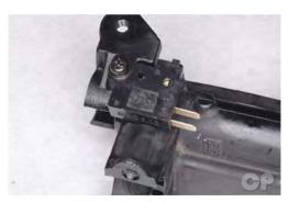
Install the brake light switch. Tighten the mounting screw securely with a #2 Phillips screwdriver.
