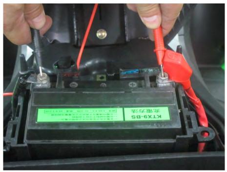
Check the battery voltage with a multi-meter. Place the positive probe onto the positive battery terminal and the negative probe to the negative battery terminal. If the battery reads under 12.3 V it is undercharged.
