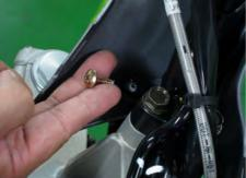
Remove the two lower handlebar cover screws with a #2 Phillips.
