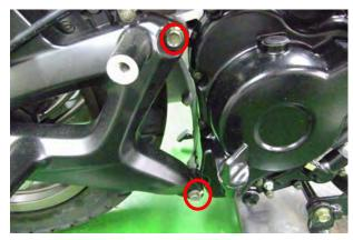
Remove the two rear fork bolts with a 12 mm socket.
