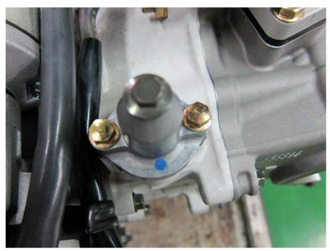
The cam chain tensioner is located on the back of the cylinder.
