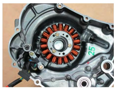
Fit the stator and the crankshaft position sensor into the generator cover together as shown. Insert the two crank position sensor mounting bolts and the three stator mounting bolts. Tighten the bolts securely with an 8 mm socket.
