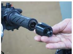
Remove the bar ends with a 6 mm Allen.
