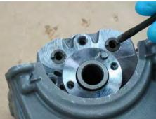
Wipe the rocker arm shafts clean. Insert the rocker arm shafts through the camshaft holders and rocker arms. Install the rocker arm shafts so that the end sits as shown.
