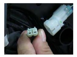
Disconnect the crank position sensor wire coupler. Measure the resistance between the Blue/White and green/white wire terminals.
