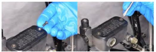
Thread in the reservoir cover screws and tighten them securely with a #2 Phillips screwdriver.
