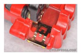
Remove the brake pad spring.
