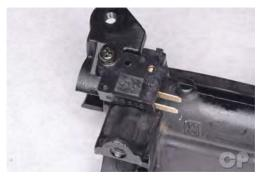
Remove the brake light switch mounting bolt with a #2 Phillips screwdriver. Remove the brake light switch.
