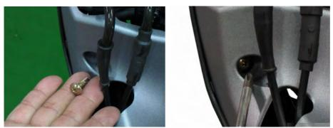
Install the two upper handlebar cover screws with a #2 Phillips.
