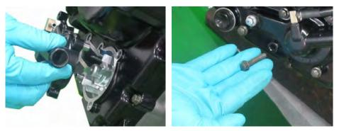
Install the water pump cover and insert the four bolts.
