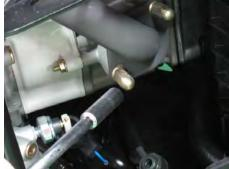
Install the two exhaust pipe joint nuts with a 12 mm deep well socket. Do not tighten.
