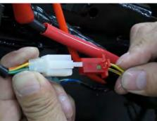
Disconnect the starter relay wire connector.
