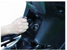
Install the fuel cap with the key.
