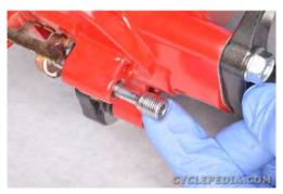
Apply a light coat of waterproof grease to the brake pad pin. Push the pads against the pad spring and insert the brake pad pin.
