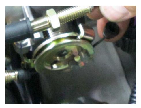
Connect the throttle cables to the throttle drum.
