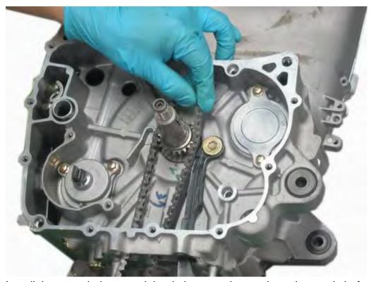
Install the cam chain around the timing sprocket teeth on the crankshaft.
