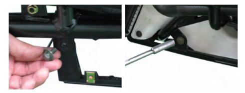
Install the two undercover bolts on both sides and then tighten securely with a 10 mm socket.
