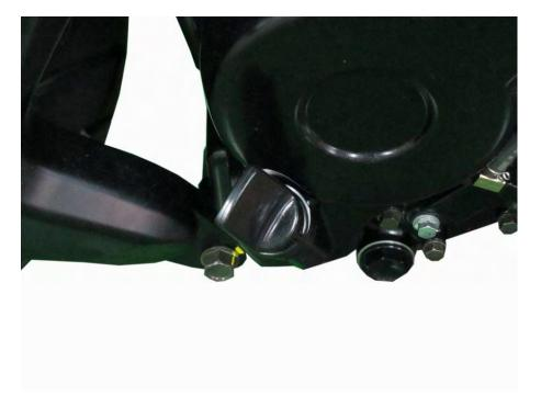
The oil filler cap/dipstick is located on the right side of the engine.
