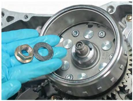
Remove the flywheel nut and washer.
