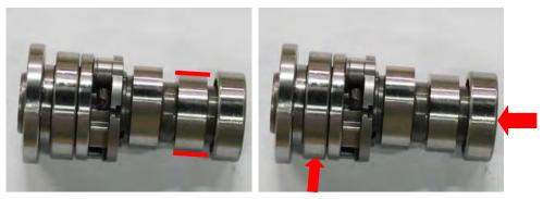
Inspect the camshaft cam heights for the intake and exhaust lobes.
