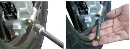
Remove the two caliper mounting bolts with a 12 mm socket. Discard the brake caliper mounting bolts.
