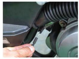
Unplug the oil pressure switch wire at the bullet connector. The oil pressure switch is located below the cylinder.
