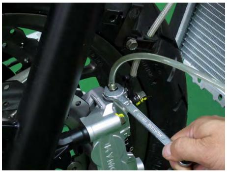
Pull off the rubber cap over the bleeder valve and crack open the bleeder valve on the brake caliper using an 8 mm wrench. This valve is usually very tight so use a box end wrench or a 6 point socket and ratchet to prevent rounding off the head. Snug the bleeder valve back down.
