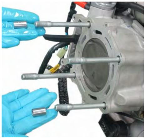
Make sure the cylinder head mating surface is clean. Install the two dowel pins as shown.
