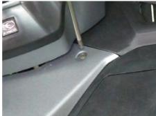
Install the two screws below the handlebar.
