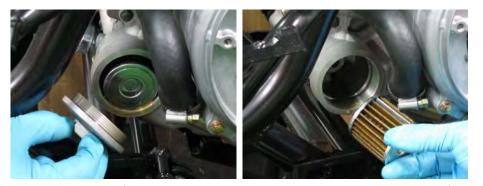
Remove the oil filter cap with spring and take out the used oil filter.
