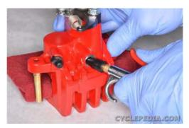
Place a 1/4" thick strip of wood or a shop rag between the caliper piston and the inside surface of the brake caliper. Blow compressed air into the banjo bolt opening to remove the caliper pistons. The pistons are a tight fit in the brake caliper and will pop out with a lot of force. Do not place your fingers over the caliper pistons while removing them as serious injury could result.
