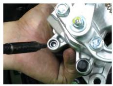
Loosen the brake pad pin with a 5 mm Allen. Remove the brake pad pin with a 5 mm Allen.
