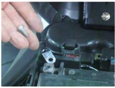
Remove the negative battery cable bolt with a 10 mm socket or #3 Phillips screwdriver. Free the negative cable from the battery.
