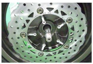
To remove the rear brake disc take out the five mounting bolts with a 6 mm Allen.
