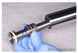
Place the rebound spring on the damper rod and insert the damper rod into the inner fork tube.
