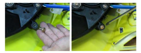
Install the headlight assembly mounting screws and tighten securely with a #2 Phillips.
