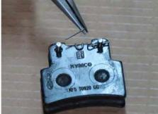
Remove the brake pad Clips with a splcier.
