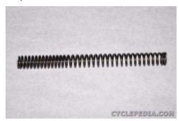
Inspect the fork springs for signs of fatigue. Replace the fork springs if they vary dramatically in length.
