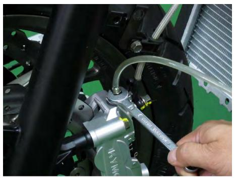
Place a length of 6 mm inside diameter clear hose on the bleeder valve and place the other end in a suitable container. A spare battery vent hose works well for this job.
