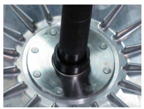
Drive in the new baring so the sealed side face out towards the clutch. Install the snap ring into the groove. Install the collar and drive in the new needle bearing so that its markings face out. Drive in the bearings with a suitable driver with the same outside diameter as the bearing.
