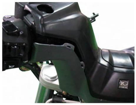
Carefully free the tabs and remove the upper handlebar cover.
