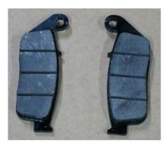
Replace the pads if the brake wear exceeds the wear indicator lines or if the wear is uneven. Always replace brake pads as a set.
