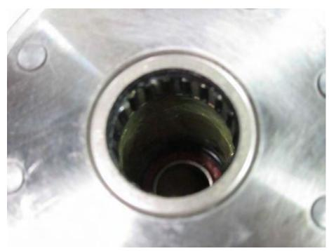
Inspect the bearings in the right face of the driven pulley.
