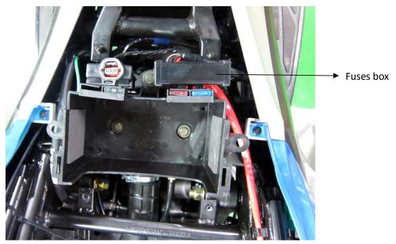
The fuse box is located in the front of the battery.
