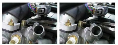
Squeeze the air bleed hose clamp with needle nose pliers and slide back the clamp. Free the air bleed hose from the thermostat.
