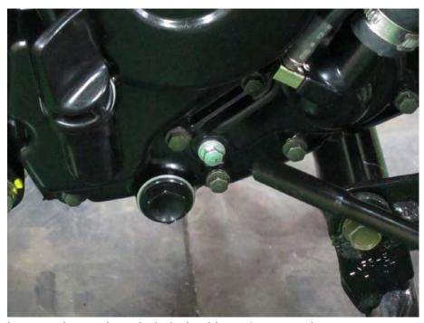
Loosen the coolant drain bolt with an 8 mm socket.
