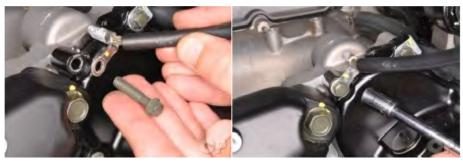
Install the main engine ground to the right side of the engine. Tighten the main engine ground bolt securely with an 8 mm socket.
