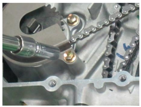
Loosen the two oil pump cover bolts with an 8 mm socket.
