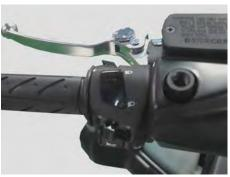
Use a digital multimeter to check for continuity to inspect the handlebar switches. Continuity should exist between the wires as indicated.
