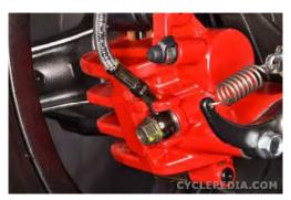
Install the banjo bolt with new sealing washers and tighten to specification with a 12 mm socket.
