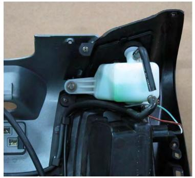
The coolant reserve tank is mounting to the inner cover with bolt/screw. There are two hoses that connect to the reserve tank. The top hose is a dump hose that hangs over the other side. The bottom hose is the overflow hose that runs to the filler neck.
