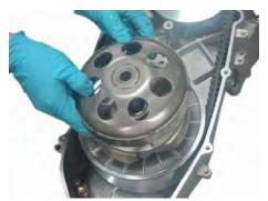
Remove the outer clutch.
