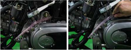
Disconnect the drain hose from the air cleaner.
