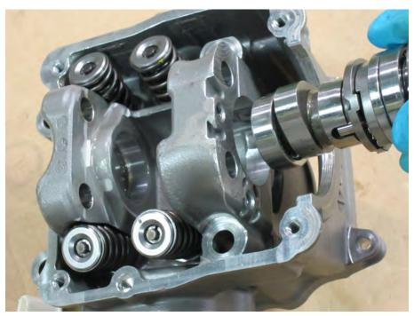
Remove the camshaft from the cylinder head.
