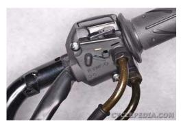
Insert the two housing screws and tighten them securely with a #2 Phillips screwdriver. Tighten the front before the rear.
