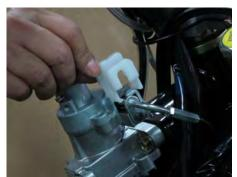
Install the seat latch cable cover.
