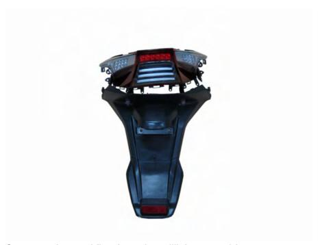
Separate the mud flap from the taillight assembly.
