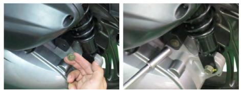
Install the left fender mounting bolts with a 10 mm socket on the back side.
