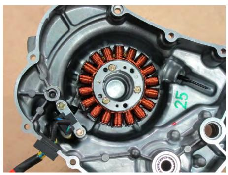
Remove the three stator mounting bolts and the two crank position sensor bolts with an 8 mm socket. Remove the stator and the crank position sensor together.
