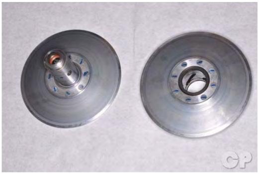
Inspect the faces of the driven pulley. Clean away any grease from the faces where the belt rides.
