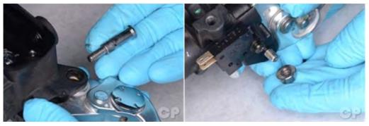
Apply a light coat of grease to brake lever pivot bolt. Insert the pivot bolt from above and thread on the nut.
