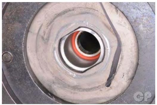
Inspect the left side bearing by turning it with a finger. If the bearing is rough turning or noisy it should be replaced.
