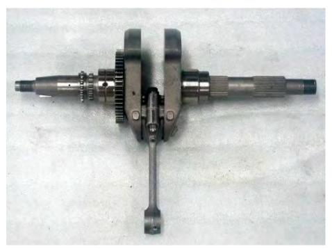
Grip the small end of the connecting rod and try and push the rod down towards the crank weights. If there is definite play between the connecting rod and crank the crankshaft should be replaced.
