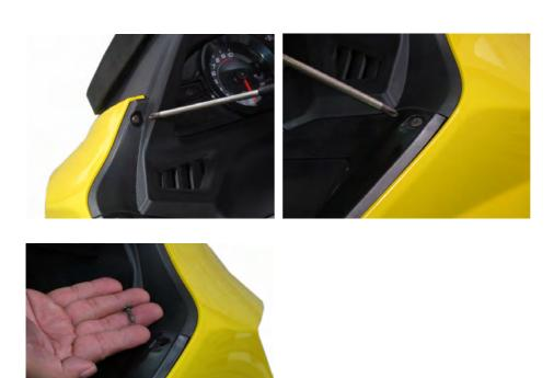
Remove the four front cover mounting screws with a #2 Phillips. There are two screws on each side.
