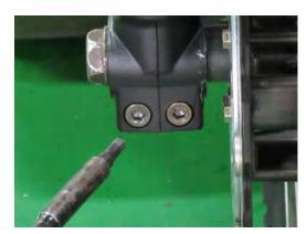
Tighten the front axle pinch bolt securely with a 6 mm Allen.
