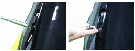
Remove the four windshield bolts with a 10mm socket. There are two bolts on each side.
