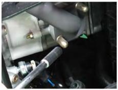
Tighten the two exhaust pipe joint nuts to specification with a 12 mm deep well socket.
