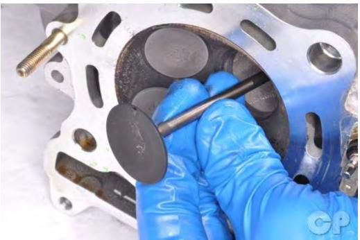
Push the valve stem down and remove the valve from the combustion chamber side of the cylinder head. Rotate the valve as it is removed.
