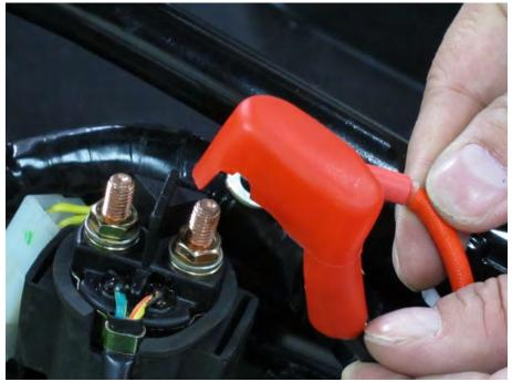
Remove the leads from the starter relay.
