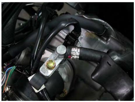
Inspect the fuel hose for signs of deterioration or damaged. Replace the fuel hose as needed.
