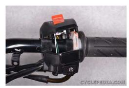
Install right switch housing. The post on the housing should fit into the hole in the bar.
