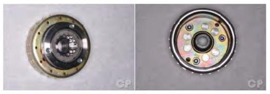
Fit the starter clutch to the back of the flywheel. Apply blue Loctite to the threads of the three starter clutch mounting bolts. Insert the three starter clutch mounting bolts.
