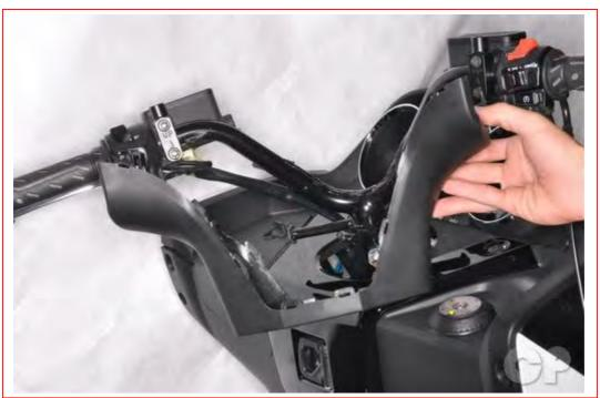
Place the lower cover onto the handlebar.
