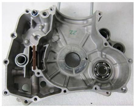
Apply sealant uniformly to the crankcase mating surface as indicated. Do not allow sealant to enter oil passages or get in bearings.
