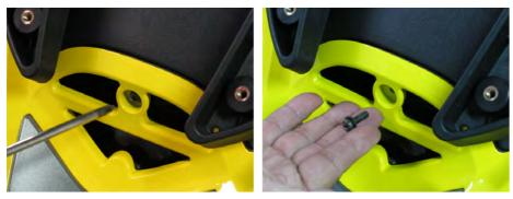
Remove the center front cover mounting screw with a #2 Phillips
