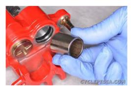
Install the normal rear caliper piston. Push the caliper piston completely into the caliper so that the open side faces out.
