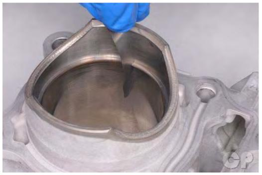
Measure the ring gap with a feeler gauge. Repeat this procedure with second ring and the oil side rails.
