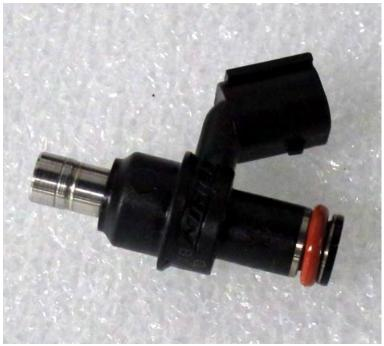
Inspect the seals on both sides of the fuel injector. Replace the injector if the seals are in poor condition. Check for signs of clogging. Set the multi meter to read ohms of resistance ( $\Omega$ ).
