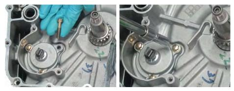
Insert the three oil pump mounting screws and tighten them securely with an 8mm socket.
