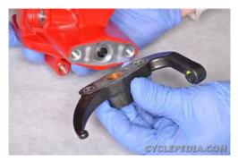
Remove the parking brake bracket and gasket.
