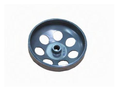
Inspect the inside of the clutch outer for excessive wear and damage. Measure the inside diameter of the clutch outer and replace the part as needed.
