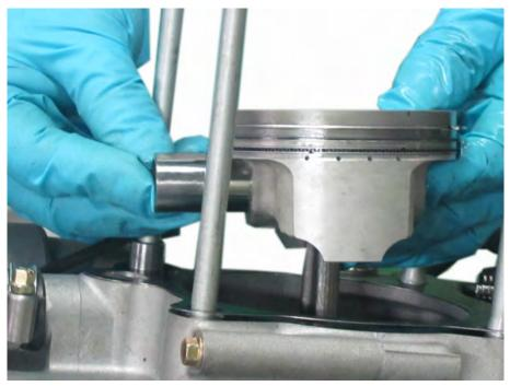
Remove the piston pin and the piston.
