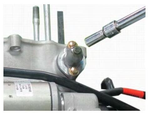
Install the cam-chain tensioner with a new gasket. Insert the mounting bolts and tighten them evenly to specification with an 8 mm socket. Remove the screwdriver and release the cam-chain tensioner rod.
