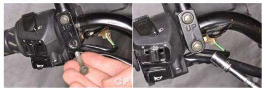
Install the two master cylinder mounting bolts and tighten them securely with an 8 mm socket.
