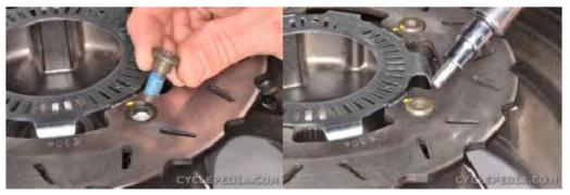
Apply a non-permanent thread locking agent to the threads of the rear disc bolts. Insert the bolts and tighten them to specification with a 6 mm Allen.
