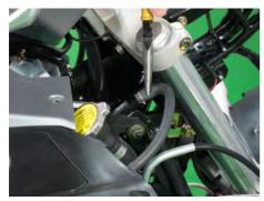
Remove the bottom hose is the overflow hose that runs to the filler neck.
