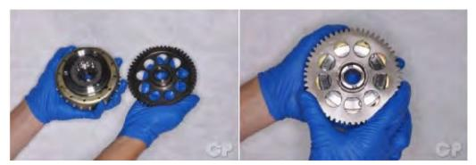
Fit the boss of the starter driven gear into the starter clutch. The starter clutch should only allow the driven gear to turn in one direction. If the starter clutch allows turning both ways or will not let the driven gear rotate smoothly in one direction the starter clutch must be replaced.
