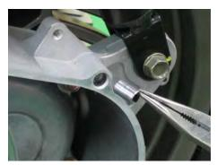
Install the two dowel pins into the belt case.
