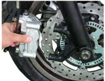
Remove the front brake caliper.
