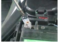
Connect the negative battery cable and install the bolt with a 10 mm socket or #3 Phillips screwdriver.
