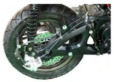
Remove the rear shock mounting bolts with a 14 mm socket.
