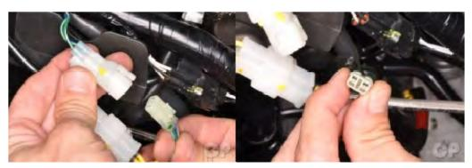
Disconnect the crank position sensor wire coupler.
