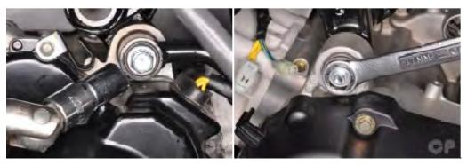
Tighten the engine mounting bracket damper bolt and nut with a 17 mm wrench for the nut and a 14 mm socket for the bolt.
