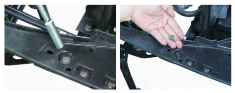
Remove the three mounting bolts on right side with a 10 mm socket.
