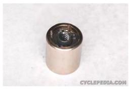
Clean the brake caliper pistons with steel wool. Inspect the brake caliper pistons for wear and damage.
