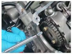
Apply a small amount of blue Loctite (non-permanent) to the threads of the camshaft sprocket bolts. Thread in the camshaft sprocket bolts and tighten to specification using a 5 mm Allen socket.
