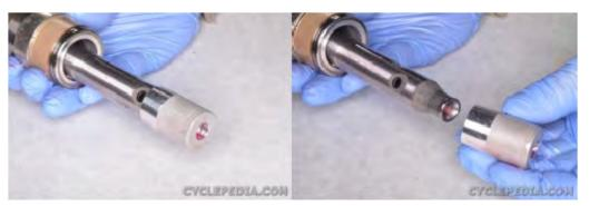
Remove the oil lock piece. The oil lock piece may come out with the damper rod in the inner fork tube or it may remain in the slider.
