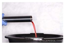
Dump the fork oil into a suitable container. Pump the fork through its stroke several times to free as much oil as possible. Hold the fork inverted for several minutes to let the oil drain completely.
