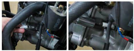
Thread the spark plug by hand before using a socket to tighten. Torque to specification with a 5/8" spark plug socket. Do not over tighten the spark plug. The cylinder head is made out of soft metal, and it can be easily damaged.
