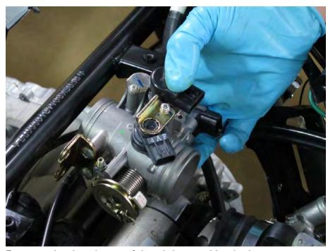
Remove the throttle out of the air box and intake boots.
