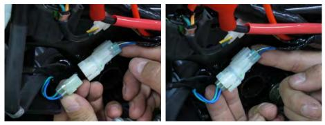
Disconnect the crank position sensor wire coupler.
