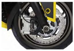
The brake calipers are each mounted to the front fork with two bolts.
