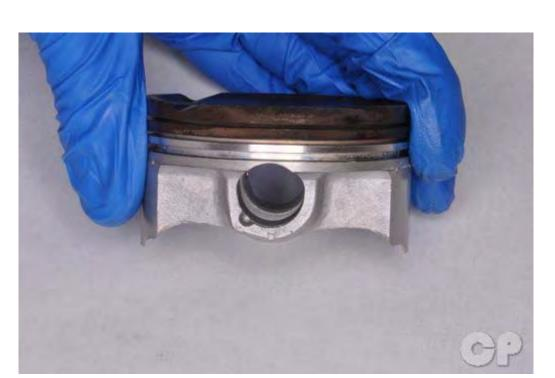
Also clean out the ring grooves. You can use an old ring to scrape out any carbon build up in the grooves.
