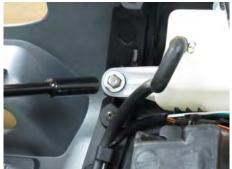
Install the left reserve tank mounting bolt with a 10 mm socket and bottom screw with a #2 Phillips screwdriver.
