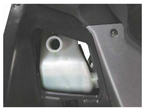
Open the coolant reserve tank lid. Siphon the coolant out of the reserve tank with an appropriate suction device. If a suction device is unavailable remove the reserve tank and poor it out. See the Radiator topic for more information.
