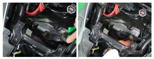
Squeeze the breather hose clamp with needle nose pliers and slide if back. Remove the breather hose from the cylinder head cover.
