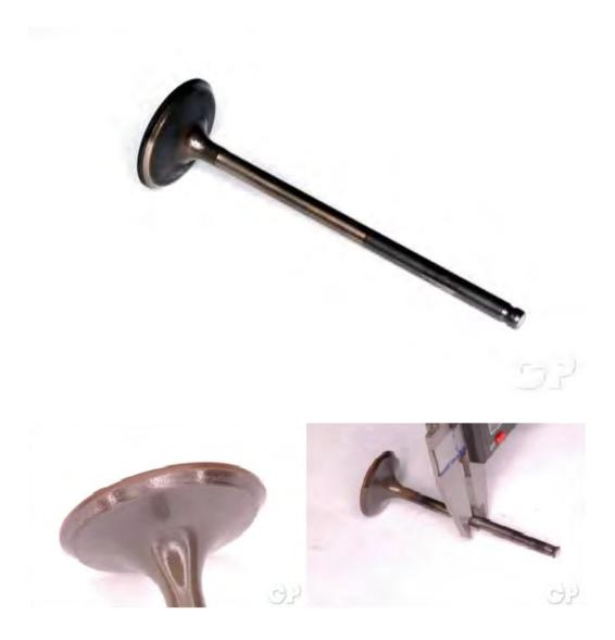
Inspect the valves for damage and burning. Measure the valve stem diameter in several places where the valve makes contact with the guide. If the measurement is below specification replace the valve.
