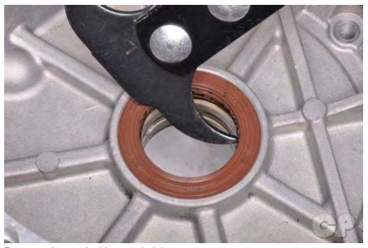
Remove the seal with a seal pick.
