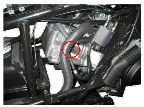
Leave the old spark plug installed. Connect known good spark plug to the coil and ground the plug to the cylinder head.
