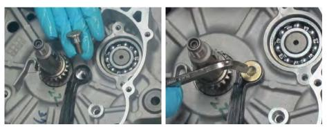
Fit the upper cam chain guide into place.
