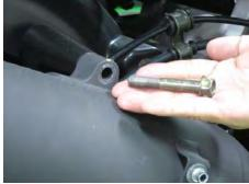
Remove the three muffler mounting bolts with a 14 mm socket.
