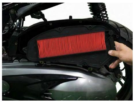
Fit the new air filter into place.
