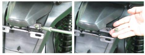
Remove the two license plate nuts with a 10 mm socket.
