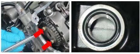
Rotate the crankshaft 360° clockwise and check the engine timing one more time.
