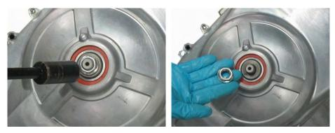
Remove the #M14 nut mounting the clutch outer.
