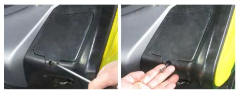
Remove the radiator coolant panel screws with a #2 Phillips screwdriver.
