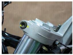
Loosen the top fork clamp bolts with a 6 mm Allen. If the fork is to be disassembled go ahead and loosen the fork caps with a 30 mm socket.
