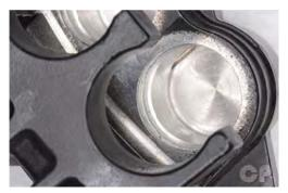
Inspect the piston bores for wear and damage.
