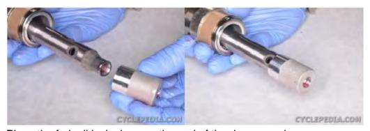
Place the fork oil lock piece on the end of the damper rod.
