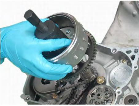
Line up the groove in the flywheel with the key and fit the flywheel onto the crankshaft. Guide the starter driven gear into the starter clutch on the back of the flywheel.
