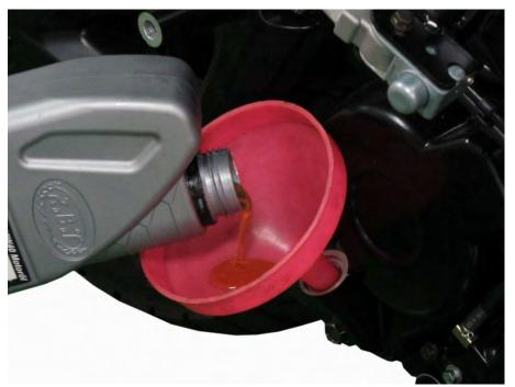
If the oil level is at or below the lower mark add more of the same type and brand of oil to the engine through the oil filler hole. If the oil level is to high remove the drain plug and the excess oil.
