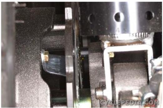
Inspect the wheel speed sensors, rotors, wires, and connectors if the speed doesn't show correctly.
