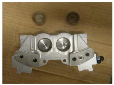
Inspect the pistons for wear and damage.
