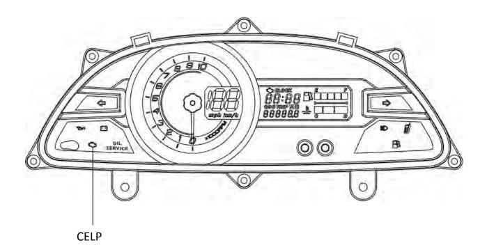
The check engine lamp (CELP) or Fi indicator is located next to the battery warning indicator.
