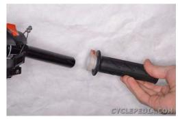
Slide the right switch housing and throttle grip onto the right side of the handlebar.
