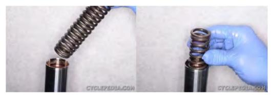
Fully extend the fork and insert the fork spring with its tightly coiled end facing down towards the axle.
