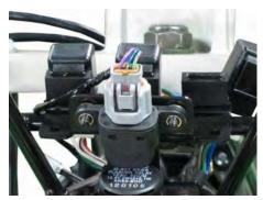
Place the tilt switch vertical as shown and the ignition switch "ON". Measure the voltage as below.
