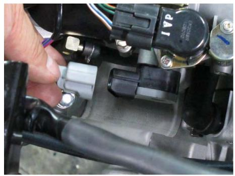
Measure if the ECU voltage outputs to TPS between the following terminals of the TPS connector.
