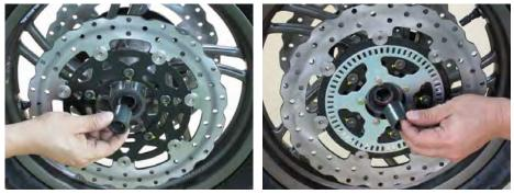
Remove the collars from each side of the wheel. Inspect the bearing seals and the O-rings seals on the collars. Replace the seals if they are in poor condition.
