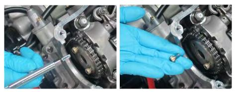
Use a 5 mm Allen wrench to remove the camshaft sprocket bolts.
