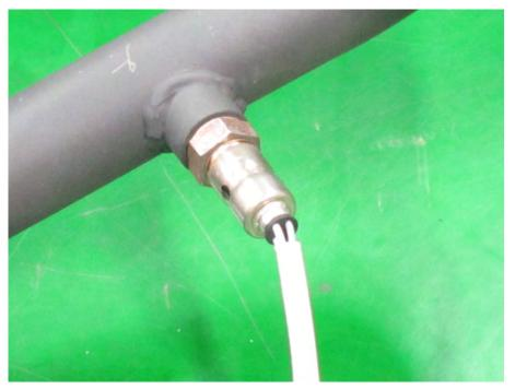
Apply anti-seize compound to the threads of the  $\rm O^2$  sensor. Install the  $\rm O^2$  sensor and tighten it to specification with a 17 mm wrench. Use care not to pinch the wires.
