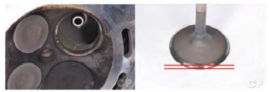
Inspect the valve seat and the valve seat width. The valve seat should be centered on the valve face. If the seat is pitted, worn out, or fits poorly on the valve face the valve seat must be resurfaced.
