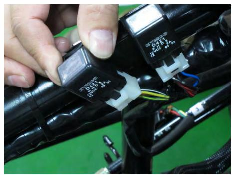
The start relay is located in front of battery. Remove and disconnect the start relay.
