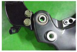
Inspect the shock absorber bushing and replace it as needed. Inspect the rear fork for damage and replace it as needed.
