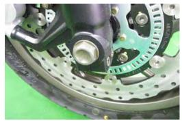
Tighten the front axle to specification with an 24 mm socket.
