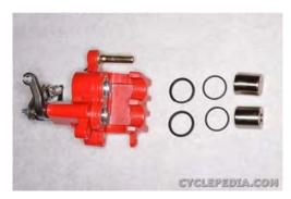
Lubricate the caliper pistons, the caliper piston bores and the seals with DOT 4 brake fluid from a tightly sealed container.
