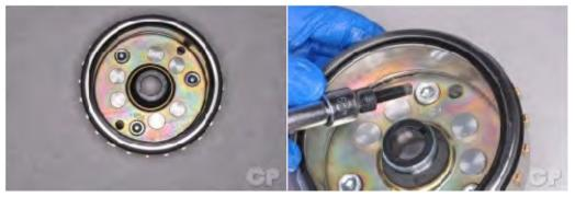
Remove the three starter clutch mounting bolts with a 6 mm Allen socket.
