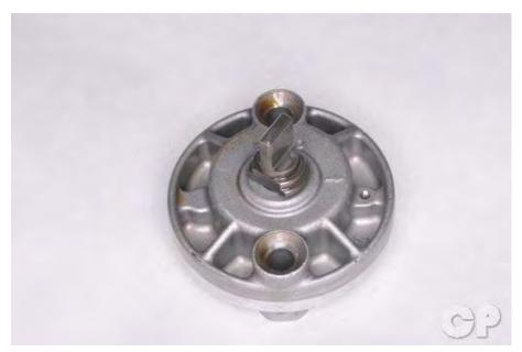
Turn the oil pump shaft by hand and make sure it turns smoothly. If the oil pump shaft will not rotate smoothly the oil pump should be replaced with a new unit.
