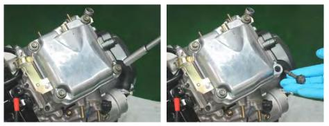
Loosen the four cylinder head cover bolts with a 10 mm socket. Remove the cylinder head cover bolts with washers and grommets. Note the gold colored and longer bolts are on the right side.
