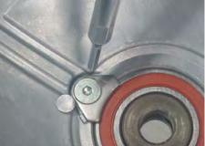
Install the bearing fixed plate with a 5 mm Allen
