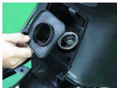
Remove the fuel cap with the key. Remove the gas cap overflow pad.
