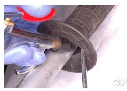
If you plan to replace the grips you can slice them lengthwise with a razor blade and peel them off. To remove the grips without cutting them use a screwdriver to open a gap between the grip and the handlebar. Spray in contact cleaner to break up the grip cement. Use compressed air to expand the grip so it can be easily slid off the end of the handlebar. Note the relationship between the angle of the grip and the throttle tube so that the new grip can be installed with the correct angle.
