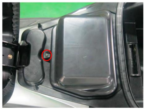
Install the battery cover. Install the four battery cover screws and tighten them securely.
