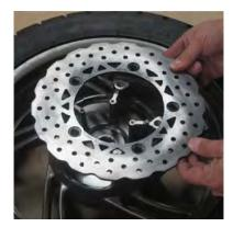
Fit the rear brake disc into place on the wheel as shown.
