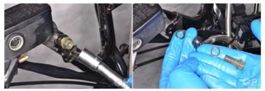
Remove the brake hose banjo bolt from the master cylinder using a 12 mm socket. Discard the sealing washers.
