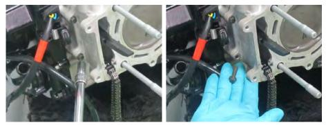
Remove the two cylinder bolts on the right side of the engine.
