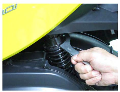
Use a pin spanner to adjust the rear shock spring preload. The shock absorbers are adjustable for pre-load. There are 5 settings. Position 1 is the softest and 5 is the stiffest.
