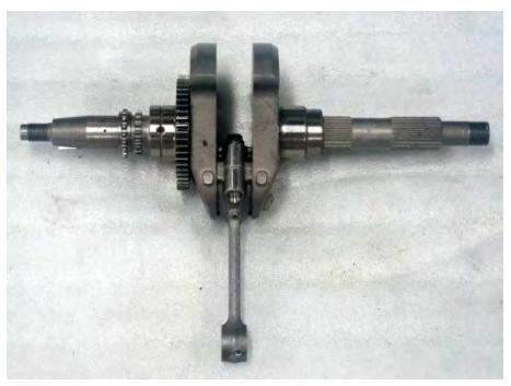
Check the side clearance of the big end of the connecting rod with a feeler gauge.
