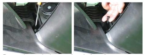
Remove the two plastic screws from the front of center cover.
