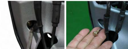
Remove the two upper handlebar cover screws with a #2 Phillips.
