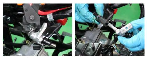
Loosen the fuel hose clamp with a special tool A120F00030. Slide back the clamp and free the injector fuel pipe from the fuel hose.
