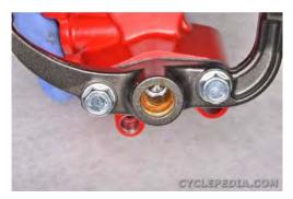
Remove the two parking brake bracket bolts.
