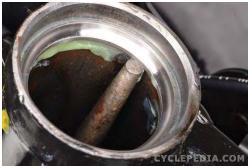
Have the drift set against the lip of the race, and work around the race evenly to drive it out. Repeat the process with the remaining bearing race.
