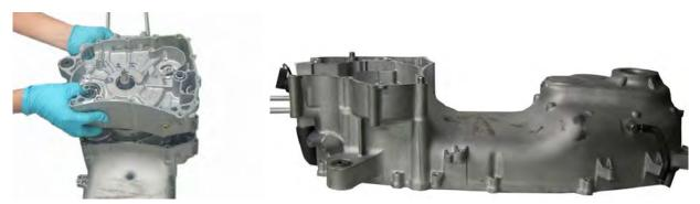
Set the right case half down on top of the left. Install the engine mount spacer.
