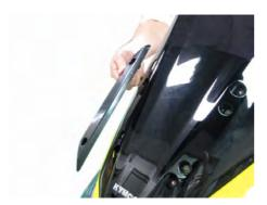
Remove four windshield cover bolts on both sides with a 10mm socket.
