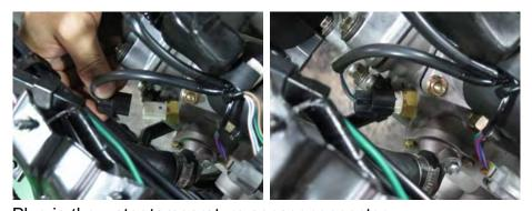
Plug in the water temperature sensor connector.
