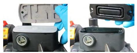
Remove the master cylinder cover, plastic piece and rubber diaphragm. Clean and inspect the rubber diaphragm for tears or other damage. Replace as necessary.
