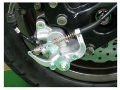
Place a suitable container under the banjo bolt to catch any remaining brake fluid. Remove the banjo bolt that holds the brake hose to the caliper using a 12 mm socket. Discard the two sealing washers.
