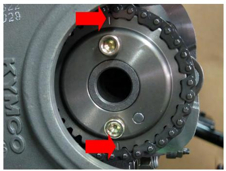
For correct engine timing the marks on the camshaft sprocket must be even with the cylinder head mating surface at the same time the "T" mark is lined up with the with the index notch in the timing inspection hole. Also the camshaft sprocket mounting boss should be visible above the cylinder head surface.
