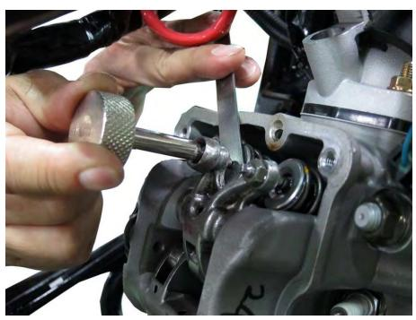
Place a 9 mm box end wrench over the locknut, and loosen the locknut. If the valve clearance is tight back out the valve tappet adjusting screws with the tappet adjustment tool. If the clearance is to loose turn in the adjusting screw until there is a light drag on the feeler gauge. Hold the adjusting screw locknut in place with the wrench to make sure it doesn't interfere with the adjustment.
