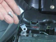
Remove the negative battery cable bolt with a 10 mm socket or #3 Phillips screwdriver. Free the negative cable from the battery.
