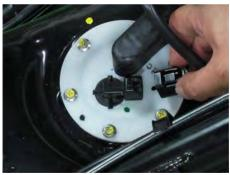
In order to drain the fuel from the fuel pipe and release the fuel pressure unplug the fuel pump connecter. Start the engine and let it run until it dies of fuel starvation. Turn the ignition switch off.
