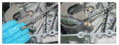
Install the oil pump cover and its two mounting bolts.
