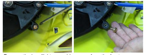
Remove the headlight assembly screws from the front cover.
