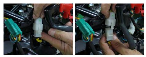
Disconnect the generator 3-pin connector.
