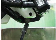
Install the two radiator bottom mounting bolts with a 10 mm socket.
