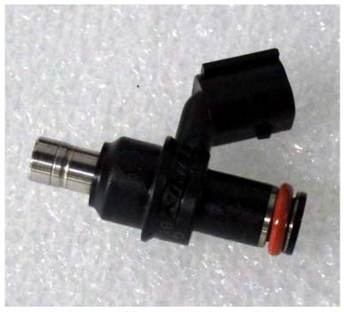
Apply a light coat of fresh engine oil to the fuel injector O-ring seals.
