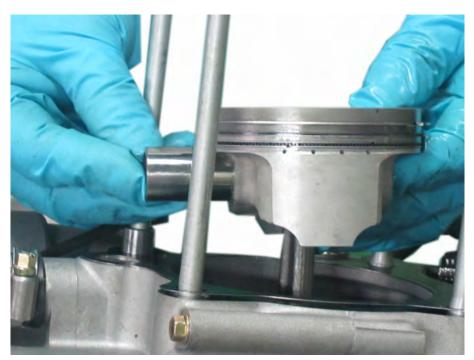
Place the piston over the connecting rod. Insert the piston pin into the piston and rod.
