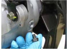
Remove the transmission oil level check bolt with a 12 mm socket. The oil level is correct when oil flows from the bolt hole. Install the oil level check bolt and tighten it to specification with a 12 mm socket.
