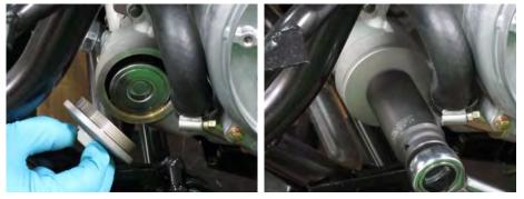
Install the oil filter cap with spring. Makes sure the spring fits against the filter correctly. Tighten the oil filter cap securely with a 24 mm socket.
