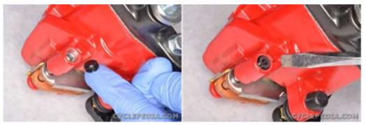
Install the brake pad pin plug and tighten it to specification with a flat blade screwdriver.
