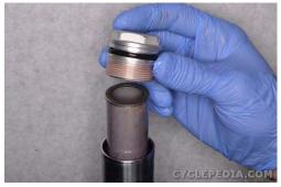
Lubricate the top cap O-ring with fresh fork oil and install the cap into the top of the inner fork tube as shown. Wait to tighten the cap with a 30 mm socket until the fork is installed.
