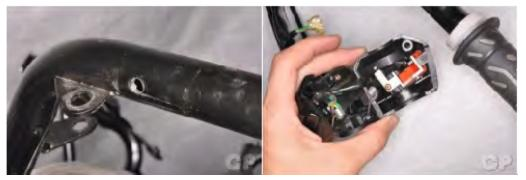
Install the right switch and throttle housing. The post on the housing should fit into the hole in the bar.
