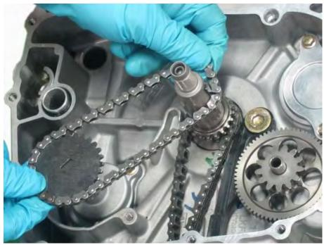
The oil pump is driven by a chain off of the crankshaft.
