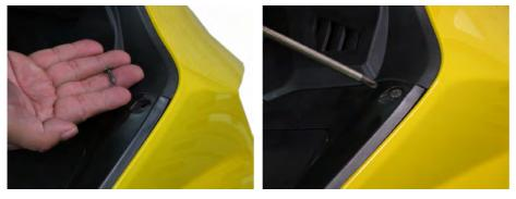
Install the four front cover mounting screws and tighten securely with a #2 Phillips. There are two screws on each side.
