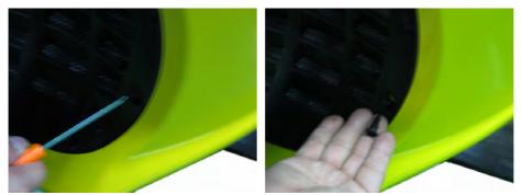
Remove the six lower fairing push pins.
