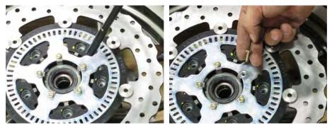
To remove the front brake disc take out the five mounting bolts with a 8 mm Allen.
