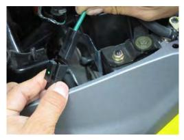
Disconnect the main engine ground wire. Free the engine ground from the left side of the engine.
