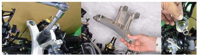
Remove the bridge stem nut and washer.
