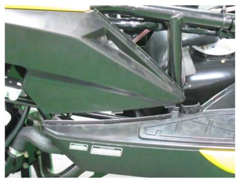
Carefully push the hooks into the corresponding tabs on both sides of the body cover.
