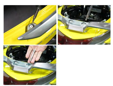
Remove the four carrier bolts with a 6 mm Allen.
