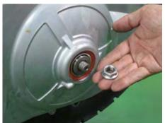
Remove the driven pulley nut with a 24mm socket.
