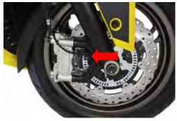
Remove the front wheel speed sensor mounting bolt with an 8 mm socket. Free the front wheel speed sensor from the right fork.
