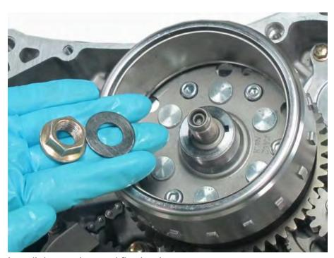
Install the washer and flywheel nut.
