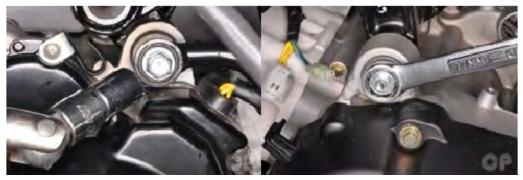
Loosen the engine mounting bracket damper bolt and nut with a 17 mm wrench for the nut and a 14 mm socket for the bolt.
