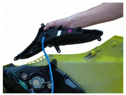
Remove the turn signal light assembly.
