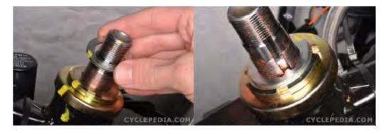
Slide the lock washer onto the steering stem as shown.
