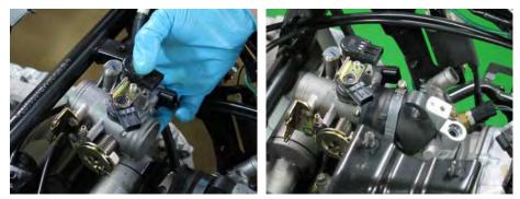
Fit the throttle body into the air box and intake boots.
