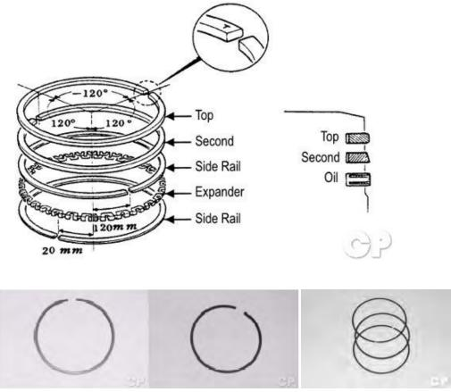
The two upper rings are each a single piece of metal. The oil ring consists of an expander ring and two side rails.
