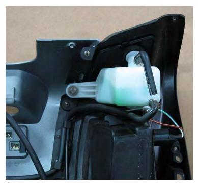
Connect the dump hose to the bottom of the reserve tank and the overflow hose to the upper. Secure the hoses with the clamps.
