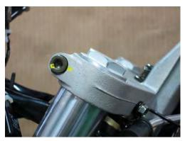
Fit the fork into place so that the mark on the top of the fork tube lines up with the upper fork clamp as shown.
