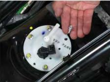
Remove the 6 fuel pump bolts with a 7 mm socket or #2 Phillips screwdriver.
