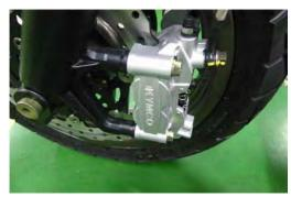
Install the banjo bolt with new sealing washers and tighten to specification with a 12 mm socket.
