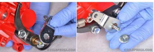
Install the parking brake arm and return spring as shown. Thread on the lock nut.
