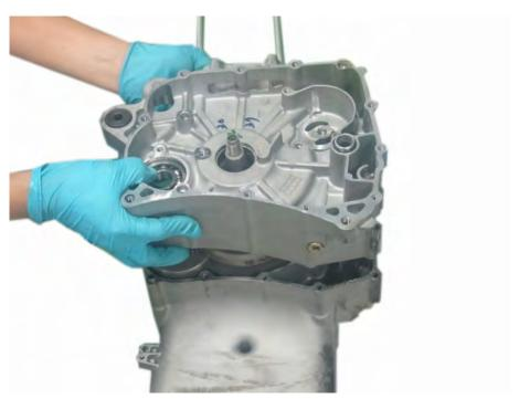
Separate the halves of the crankcase. If needed gently tap the reinforced areas of the right crankcase half with a rubber mallet. Lift the right crankcase off of the left.
