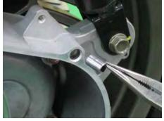
Remove the two dowel pins.
