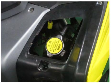
Fill the cooling system with a mix of distilled water and Coolant Concentrate. Continue filling until the coolant until it reaches the bottom of the filler neck as shown.
