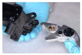
Remove the brake lever.
