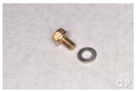
Inspect the drain plug and washer.
