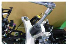
Torque the bridge stem nut to specification with the special deep well socket.
