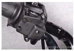
Insert the two housing screws and tighten them securely with a #2 Phillips screwdriver. Tighten the front screw before the rear.
