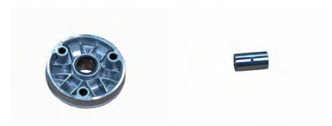
Inspect the movable drive face and bushing for wear and damage. Replace the parts as needed.
