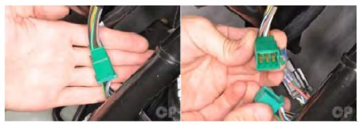
Unplug the green connector for the right handlebar switches.
