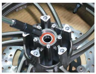
Remove one of the bearings with a bearing puller. Special Tools- Bearing Remover: A120E00093
