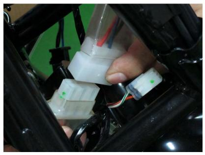
Unplug the white six-pin ignition switch connector.
