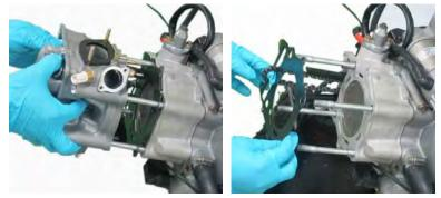
Remove the cylinder head assy and gasket.
