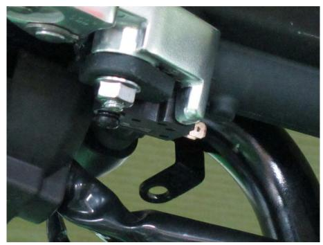
Check for continuity between the brake light switch connectors. There should be continuity when the lever is pulled and none when released.
