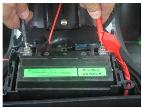
Start the engine and warm it up to the operating temperature; stop the engine. Connect the multimeter between the positive (+) and negative (-) terminals of the battery. To prevent short, make absolutely certain which are the positive (+) and negative (-) terminals or cable.
