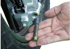
Remove the two caliper mounting bolts with a 12 mm socket. Discard the brake caliper mounting bolts.
