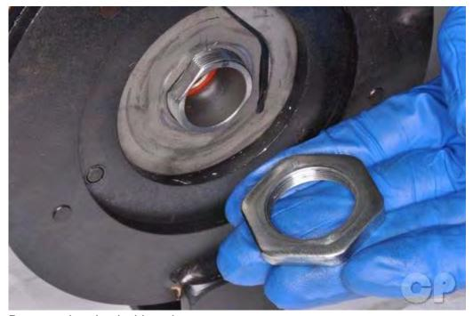
Remove the clutch drive plate nut.
