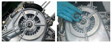
Remove the #M18 nut mounting the drive face.
