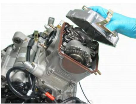
Install the cylinder head cover over the gasket. Make sure the ridge on the gasket fits into the groove on the cylinder head cover correctly. Align the bolt holes and dowel pin.
