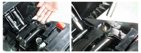
Install the two luggage box hinge nuts and tighten securely with a 10 mm socket.
