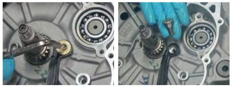
Remove the upper cam chain guide bolt with an 8 mm Allen.
