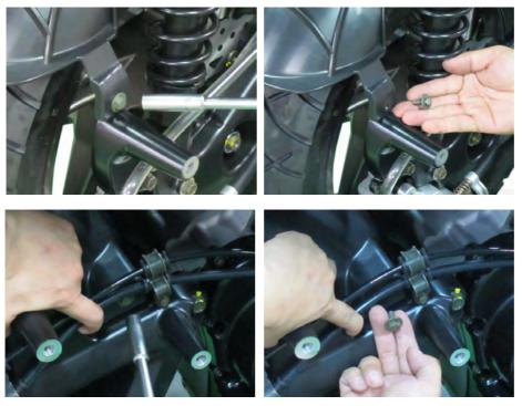
Remove the two right fender mounting bolts with a 10 mm socket.
