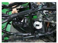
Fit the fuel tank into place.
