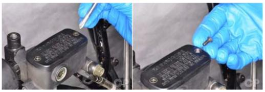
Remove the two master cylinder cover screws with a #2 Phillips head screwdriver.
