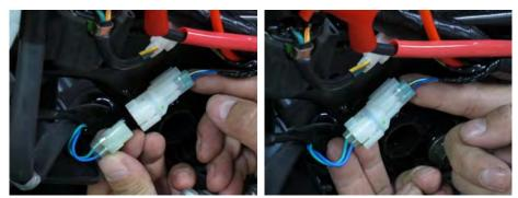
Plug in the crank position sensor wire coupler on the right side of the frame.
