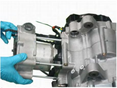
Slide the cylinder off of the studs and piston. Guide the cam chain through its opening and do not allow if to fall into the crankcase. Remove the cylinder.
