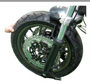
Make sure the tire direction of rotation marker is correct. Slide the front wheel into the fork.
