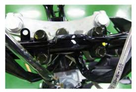
Loosen the four handlebar bolts with a 12 mm socket.
