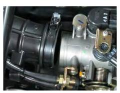
Loosen the air box hose clamp screw at the throttle body with a #2 Phillips.
