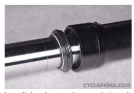
Install the dust seal securely into the outer fork tube.
