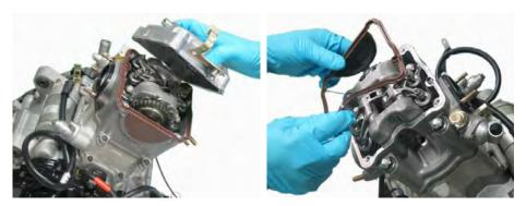
Remove the cylinder head cover and gasket.
