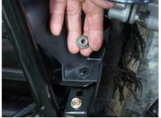
Remove the left fuel tank mounting nuts.
