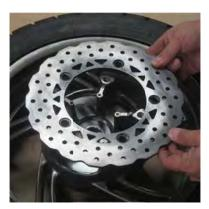
Lift off the rear brake disc.
