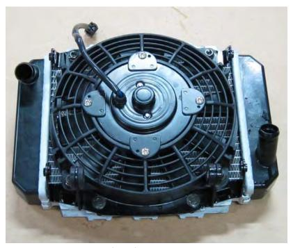
Inspect the radiator fins for damage and clogging. To remove the fan be taken out the four mounting bolts with a 10 mm socket.
