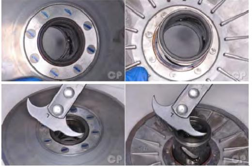
Remove the seals from the left face of the driven pulley.
