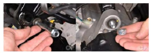
Insert the engine mounting bracket and damper bolt from the right side. Thread on the nut.
