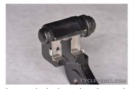
Inspect the brake pad retainer and replace it as needed.
