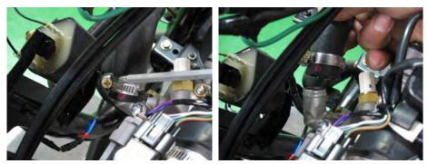
Loosen the thermostat hose clamp with a #2 Phillips screwdriver. Slide up the clamp and free the coolant hose from the thermostat.
