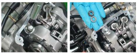
Remove the two nuts and washers on the top with a 14mm socket.
