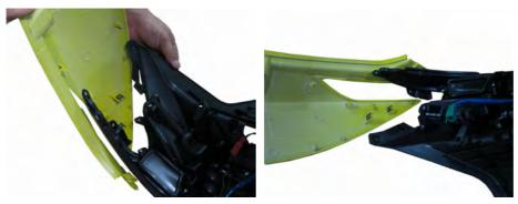
Unhook the taillight section and separate from the body cover.
