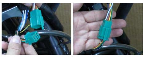
Plug in the green connectors for the right handlebar switches.
