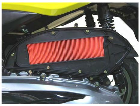
Remove the 7 air filter bolts with an 8 mm socket or a #2 Phillips screwdriver.
