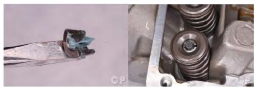
Apply grease to the inside of the split keepers. Apply a dab of grease to the end of a flat blade screwdriver. Set the keeper in the grease on the screwdriver and insert it onto the valve stem. Repeat this with the other keeper.
