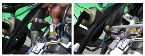
Connect the coolant hose to the thermostat. Move the clamp into place and tighten it securely with a #2 Phillips screwdriver.
