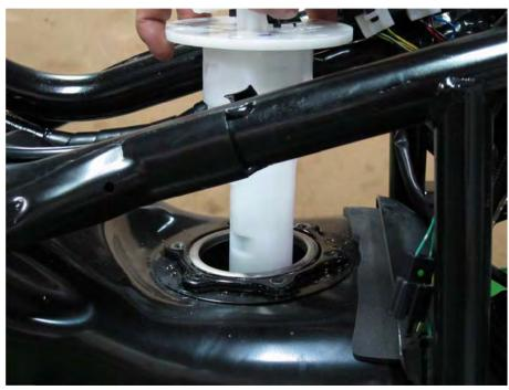
Lift the fuel pump out of the tank.
