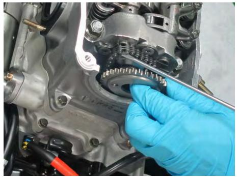
Remove the camshaft sprocket as shown. Support the chain so it does not fall into the cylinder head.
