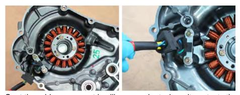
Coat the rubber grommet in silicone sealant where it contacts the generator cover. Fit the rubber wire grommet into its cutout in the crankcase cover.
