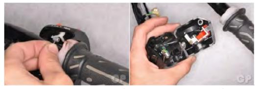
Disconnect the throttle cables and free the right switch housing from the handlebar.
