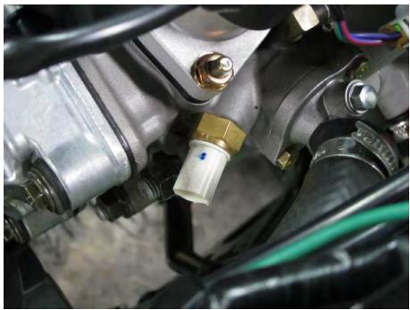
Install the WTS with a new O-ring. Tighten the WTS to specification with a 17 mm wrench.
