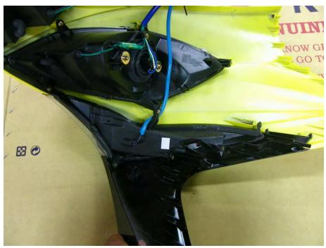
Remove the front turn signals LED mounting the front turn signals housing.
