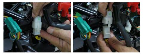
Plug in the regulator/rectifier 3-pin connector.
