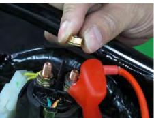
Remove the nuts that hold the starter motor lead and battery lead wires to the starter relay with a 10 mm socket.
