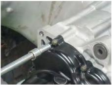
Insert the 12 generator cover bolts. Note the upper bolt holds a wire stay. Tighten the bolts securely in a with an 8 mm socket.
