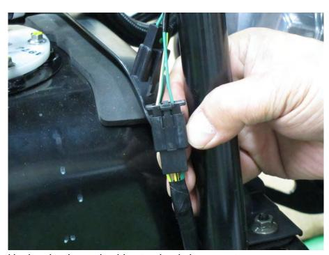
Unplug the three-pin side stand switch connector.
