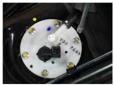
Insert the 6 fuel pump mounting bolts. Tighten the bolts to specification with a 7 mm socket or #2 Phillips screwdriver.
