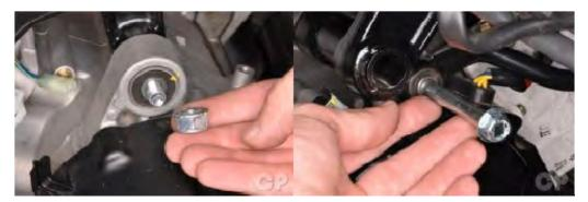
Remove the engine mounting bracket damper bolt and nut.
