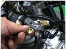
Remove the fuel injector mounting bolt with a 10 mm socket.
