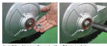
Install the driven pulley nut with a 24mm socket.
