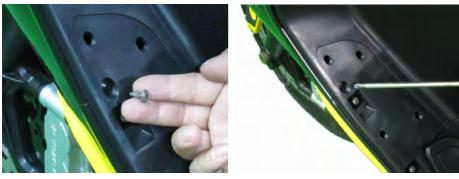
Install the left leg shield mounting screws with a #2 Phillips.
