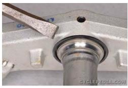
Use a chisel to remove the bottom bearing inner race and dust seal. Do not damage the steering stem.
