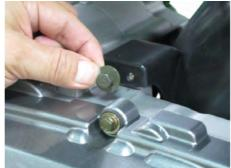
Remove the left fender mounting bolts with a 10 mm socket on the front side. Remove the airbox.
