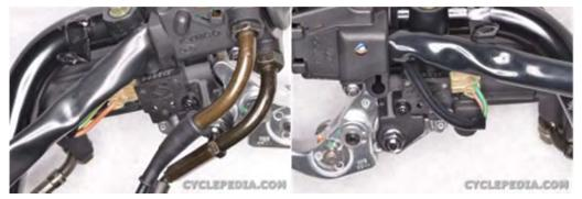
Unplug the brake light switch connectors.
