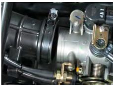
Loosen the air box connecting hose clamp screw at the throttle body with a #2 Phillips.
