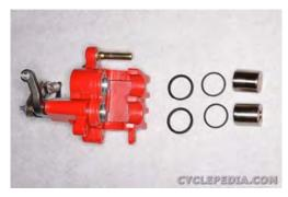
Clean all of the brake caliper components using aerosol brake cleaner and a lint free cloth. Discard the old seals.
