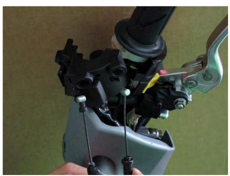
Route the throttle body end of the cables through the opening in the lower handlebar cover.
