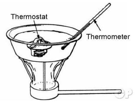
Suspend the thermostat and a thermometer in a pot of water with string. Make sure the thermostat and the thermometer are not touching the pot. Bring the temperature up to the specification slowly and check the operation of the thermostat.
