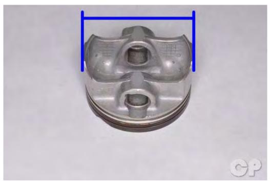
Measure the outside diameter of the piston at 9 mm up from the bottom of the skirt at a 90° angle to the piston pin. Measure the piston with vernier calipers or a micrometer. Check the piston for wear, damage, and extreme discoloration.
