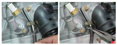
Install air bleed hose and secure it with the clamp.
