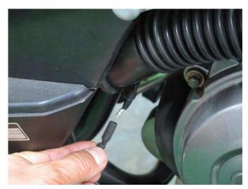
Plug in the oil pressure switch bullet connector.
