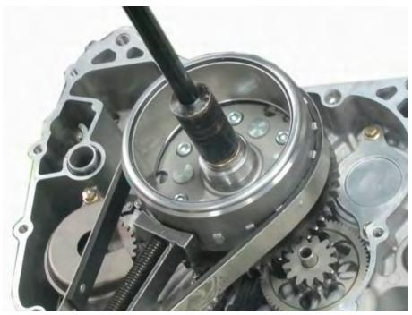
Hold the flywheel with the universal holder and torque the flywheel nut to specification with a 19 mm socket.
