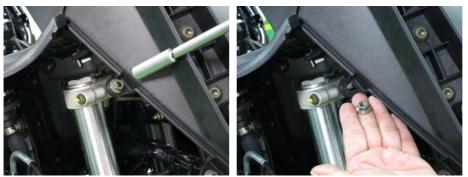
Remove the two nuts mounting on the front cover meter on both side.
