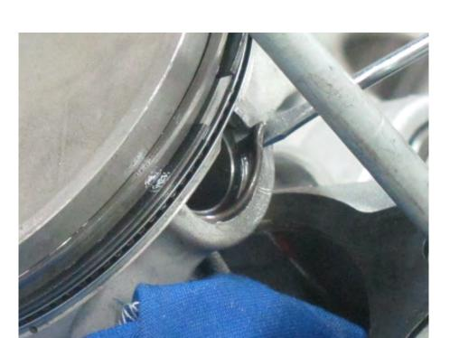
Install new piston pin clips securely into their grooves. Turn the gap in the clips away from the access gap.
