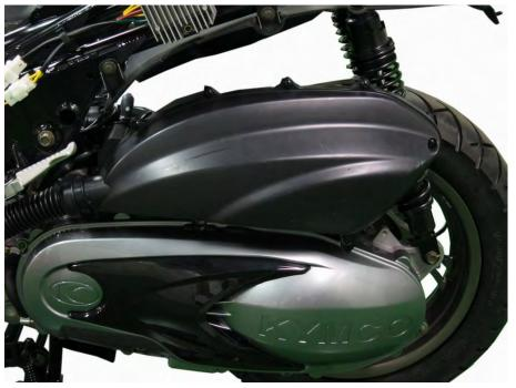
Remove the 8 air filter cover screws with a #2 Phillips screwdriver.
