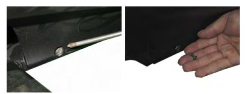
Remove the two under cover screws on both sides with a 10 mm socket.
