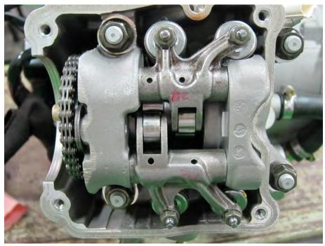
The piston should now be at TDC on the compression stroke. You can make sure that it is on the compression stroke by checking that there is some slack in the rocker arms. If the rocker arms are rigid, rotate the crankshaft 360° clockwise until the "T" mark is once again aligned with the notch on the case cover.
