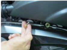
Remove the left fender mounting bolts with a 8 mm socket on the front side.
