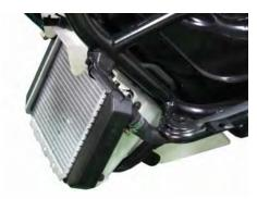
There are two coolant hoses that connect to the radiator. The top left hose runs to the filler neck and cap. The top right hose runs to the thermostat on the cylinder head. The bottom left hose runs to the water pump.
