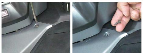
Remove the two screws below the handlebar.
