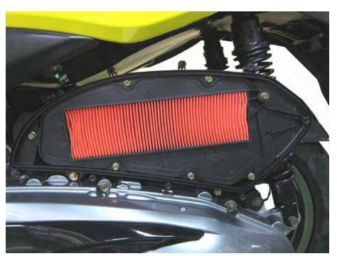
Insert the 7 air filter bolts. Tighten the air filter bolts securely with an 8 mm socket or a #2 Phillips screwdriver.
