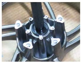
Drive in the other bearing. The bearing should fit against the distance collar. Do not continue to force the bearing in or the distance collar will begin to push the right bearing back out.
