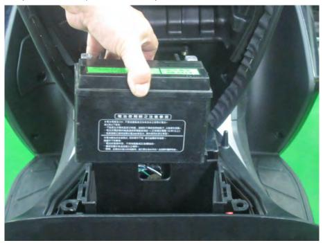
Fit the battery into the battery tray.
