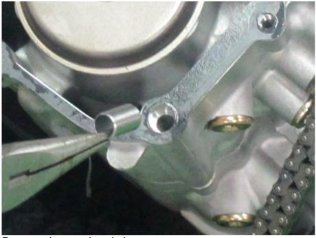
Remove the two dowel pins.
