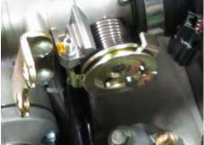
Free the throttle cables from the throttle drum.
