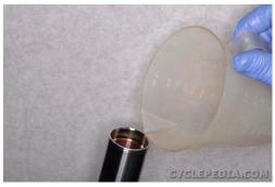
Compress the fork tube all the way. Fill the fork tube with the specified quantity of fork oil 397 cc. Use fork oil type SAE 10 weight.
