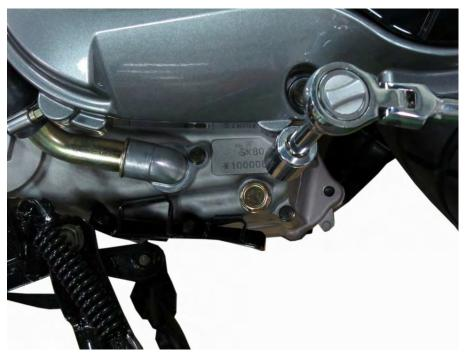
When the oil has drained completely Install the drain bolt with a new sealing washer. Tighten the drain bolt to specification with a 17 mm socket.
