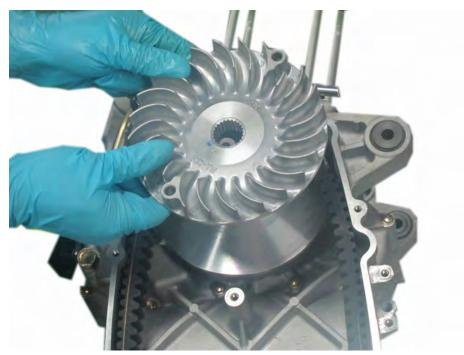
Remove the left face of the drive pulley.
