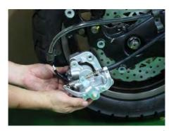
Remove the rear brake caliper from the rear fork.
