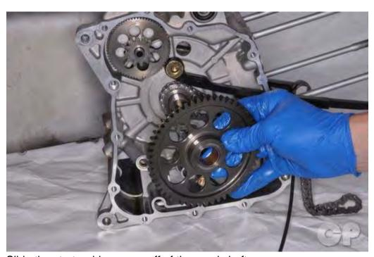
Slide the starter driven gear off of the crankshaft.
