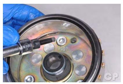
Tighten the starter clutch mounting bolts to specification with a 6 mm Allen socket.
