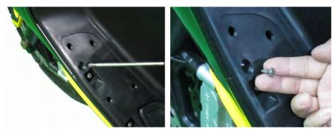
Remove the left leg shield mounting screws with a #2 Phillips.
