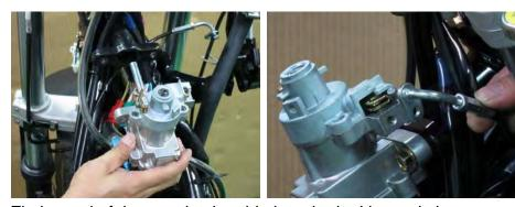
Fit the end of the seat latch cable into the ignition switch.
