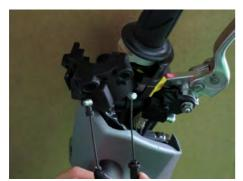
Route the throttle cables into the handlebar cover.
