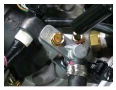
Tighten the fuel injector bolt securely with a 10 mm socket. Connect the Fuel Pump Relay or Fuel Pump Connector.
