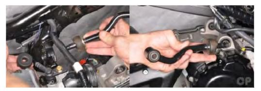
Remove the engine mounting bracket damper assembly.
