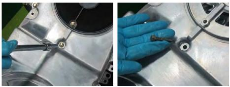
Remove the nine bolts mounting the left crankcase cover.
