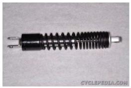
Fit the shock absorber into place. Make sure the preload arrow indicator faces out from the lower mount.
