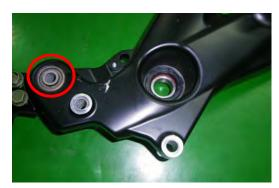
Inspect the shock absorber bushing and replace it as needed.
