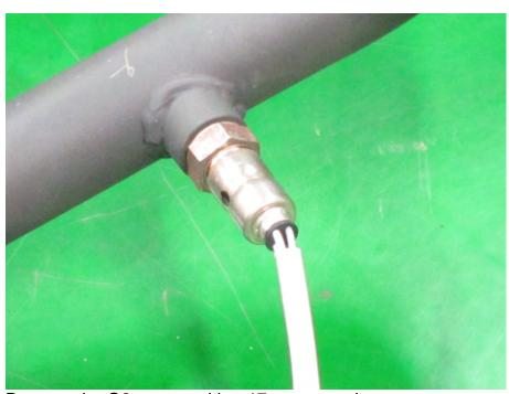
Remove the O2 sensor with a 17 mm wrench.
