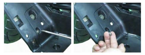
Remove the mounting screw with a #2 Phillips on left side.
