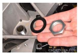
Install the bridge stem washer and nut onto the steering stem.
