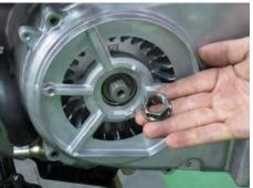
Remove the drive pulley nut with a 24mm socket.
