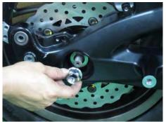
Remove the rear axle nut with a 27 mm socket.
