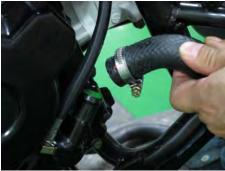
Loosen the water pump hose clamp with a #2 Phillips screwdriver. Slide up the clamp and free the coolant hose from the water pump. Allow any remaining coolant to drain into a suitable container.
