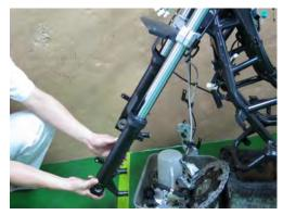
Clean the outside of the forks before disassembly and inspect them for any cracks, dents or other damage.
