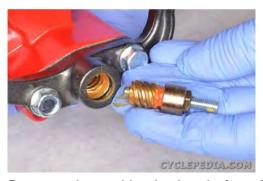
Remove the parking brake shaft and adjuster bolt.
