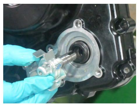
Install the impeller to the water pump shaft.
