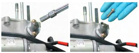
Loosen the cam chain tensioner mounting bolts evenly with an 8 mm socket.
