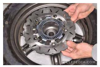
Lift off the rear brake disc.
