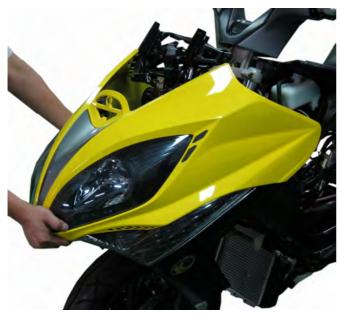
Gently pull the cover forward and free the tabs. Remove the front cover.
