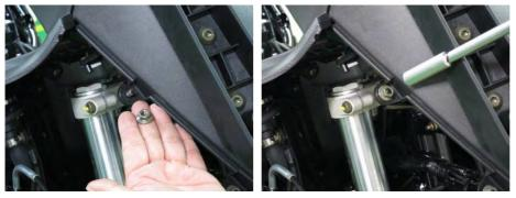
Install the two nuts mounting on the front cover meter on both side.
