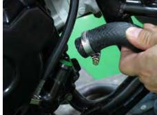
Loosen the water pump hose clamp with a #2 Phillips screwdriver. Slide up the clamp and free the coolant hose from the water pump. Allow any remaining coolant to drain into a suitable container.
