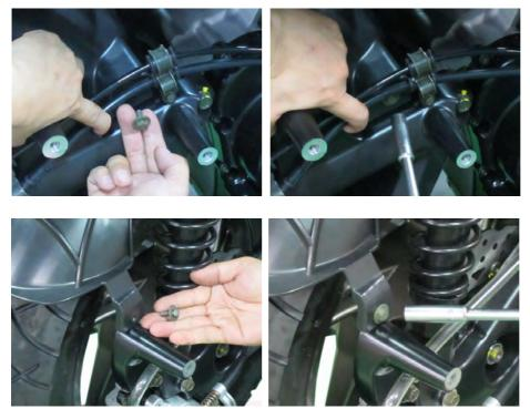
Install the two right fender mounting bolts with a 10 mm socket.
