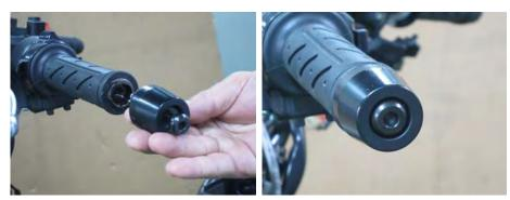
Install the bar ends with a 6 mm Allen.
