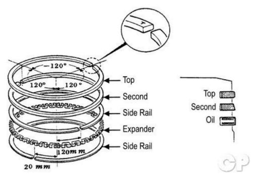
Install the top and second rings with their markings facing up. Install the rings to the piston as shown above so that no ring end gaps line up with the piston pin or perpendicular to the piston pin. The rings should turn easily on the piston without sticking or roughness.
