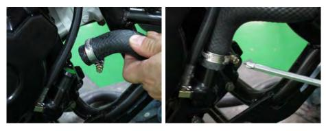
Connect the coolant hose to the water pump. Move the clamp into place and tighten it securely with a #2 Phillips screwdriver.
