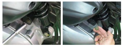
Remove the left fender mounting bolts with a 10 mm socket on the back side.
