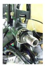
Install the inner race around the steering stem and into the upper bearing.
