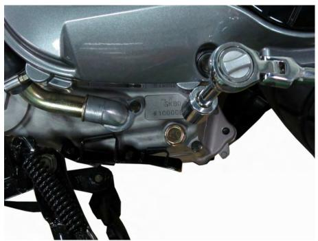
Loosen the engine oil drain bolt with a 17 mm socket. Remove the bolt and allow the oil to drain into the pan.
