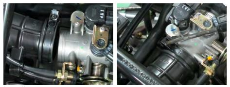
Install the screw mounting the connecting tube airbox.
