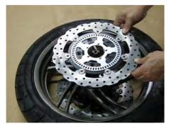
Fit the brake disc into place as shown.
