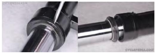
Use a flat blade screwdriver to pop the dust seal out of the fork slider. Take care to avoid scratching the fork tube.
