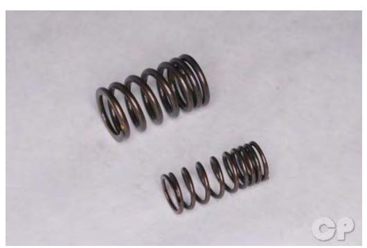
Inspect the valve springs for fatigue and damage. Replace the valve springs as needed or if the valve is also to be replaced.
