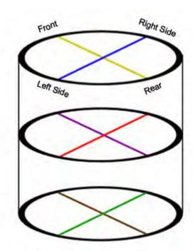
Inspect the cylinder front to back and side to side at three different height levels with a dial bore gauge.
