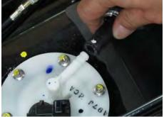
Remove the fuel hose with a plier. Slide back the clamp and free the injector fuel hose from the fuel pump pipe. Clean up any remaining fuel immediately.
