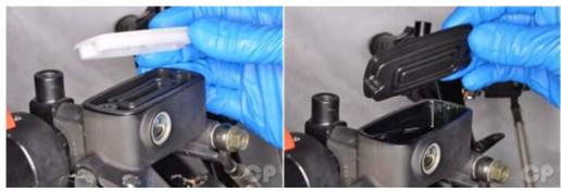
Remove the master cylinder cover, plastic piece and rubber accordion diaphragm. Pour out any remaining brake fluid.
