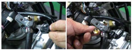
Plug in the fuel injector connector and thread in the mounting bolt.
