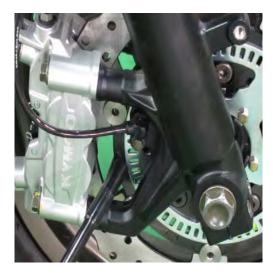
Check the speed sensor to rotor clearance with a feeler gauge and make sure that it is 0.3 - 1.2 mm (0.0012 - 0.048 in).
