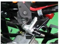
Fit the fuel hose onto the fuel injector pipe. Secure the hose to the fuel injector with the clamp. Tighten the clamp securely with a special tool A120F00030.
