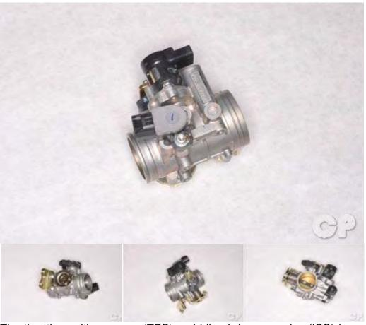
The throttle position sensor (TPS) and idle air bypass valve (ISC) have to be reset when the throttle body MAP, TPS, ISC or ECU have been reinstalled.
