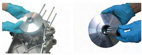
Remove the right (movable) face of the drive pulley from the crankshaft. Slide the bushing out of the movable drive face.
