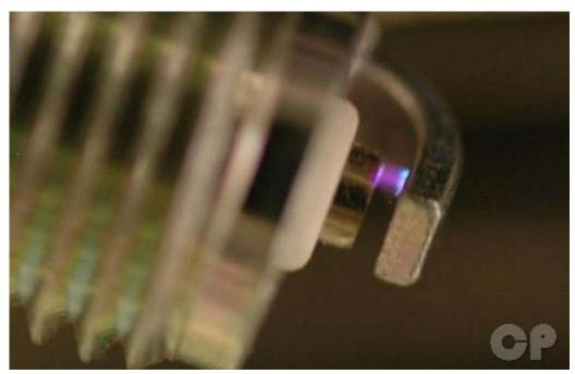
Turn the ignition switch to ON, lift the side stand, hold in one of the brake levers, and push the engine start button. The plug should spark.
