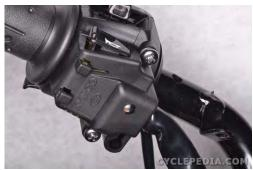
Remove the two left switch housing mounting screws with a #2 Phillips screwdriver.
