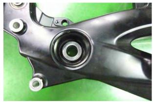
Remove the collar into the rear fork.
