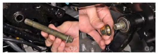
Install the two engine mounting bracket to frame mounting bolts and nuts. Insert the bolts from the outside of the frame.
