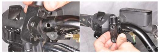
Install the master cylinder clamp. Be sure to insert the pin on the clamp into the hole on the handlebar.
