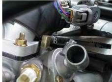
Install air bleed hose and secure it with the clamp.
