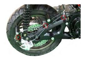
Remove the rear wheel hose clamp bolts with an 8 mm socket. Place the scooter on its center stand so that the rear wheel is off the ground.
