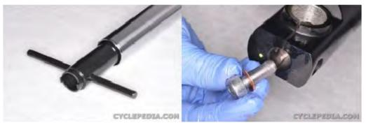
Place the axle holder of the outer fork tube in a soft jawed vise. Use a suitable damper rod holder tool to keep the damper rod from turning. Insert the fork bottom bolt with a new sealing washer. Tighten the fork bottom bolt securely with an 8 mm Allen socket. If a damper rod holder tool is unavailable temporarily install the fork components.
