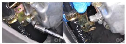
Loosen the fuel hose stay bolt with an 8 mm socket. Free the fuel hose stay from the cylinder head cover.
