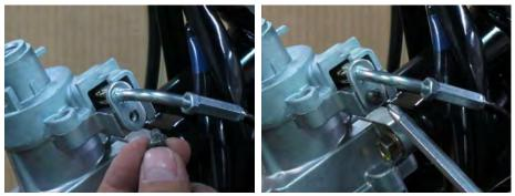
Install the seat latch cable screw and tighten it securely with a #2 Phillips screwdriver.
