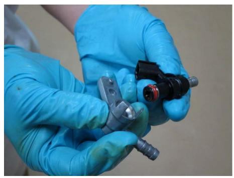
Lift the fuel pipe off the top of the injector.
