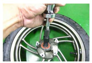
Repeat the procedure and remove the other bearing and seal. The seal should be replaced with a new item.
