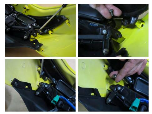
Remove the ten taillight assembly screws with a #2 Phillips.
