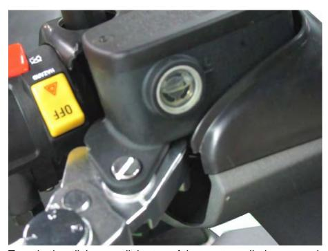
Turn the handlebars until the top of the master cylinder reservoir is level with the ground. Do this for both master cylinder reservoirs and check the level of brake fluid.
