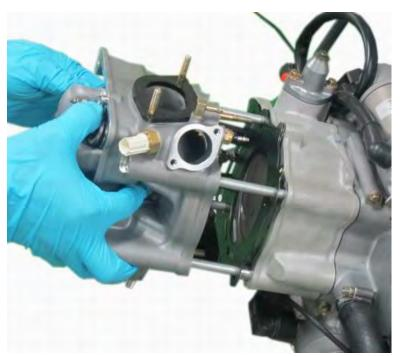
Coat the inside of the cylinder, piston rings, and piston in fresh engine oil. Lower the cylinder over the studs and guide the piston into the cylinder while you are compressing the rings with your fingers. Be careful to not damage the rings during this step. Bring the cam chain and guide through the opening.
