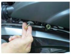
Remove 2 the air cleaner bolts with an 8 mm socket.
