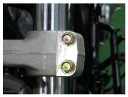
Tighten the lower fork clamp bolts evenly to specification with a 12 mm socket.
