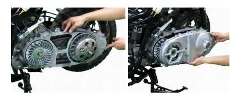
Install a new gasket with the belt case cover.
