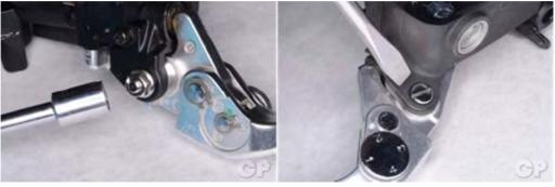
Loosen the brake lever pivot nut with a 10 mm socket and the pivot bolt with a flat blade screwdriver.
