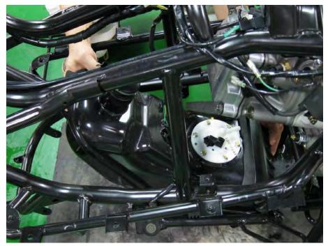
Remove the fuel tank from the bottom of the frame.
