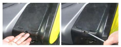
Install the radiator coolant panel screws and tighten securely with a #2 Phillips screwdriver.
