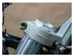
Tighten the fork caps securely with a 30 mm socket. Tighten the upper fork clamp bolts to specification with a 6 mm Allen socket.
