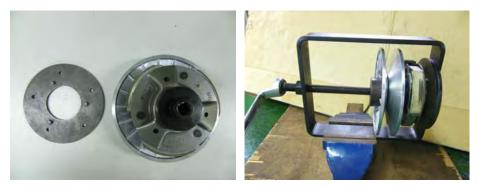
Use the clutch spring compressor tool to compress the spring in the driven pulley assembly.
