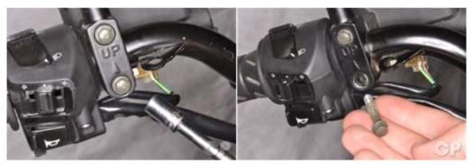
Remove the two master cylinder mounting bolts with an 8 mm socket.
