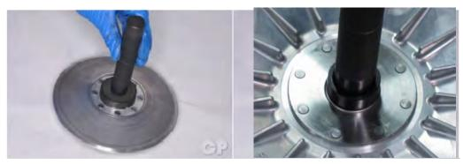
Drive in the new seals with a suitable driver with the same outside diameter as the seal.
