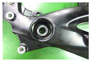
Apply grease to the lips of the dust seal and install the collar into the rear fork.
