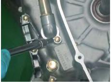
Fit the coolant hose to the right crankcase cover pipe. Secure the hose with the clamp and tighten the coolant hose clamp securely with a #2 Phillips screwdriver.
