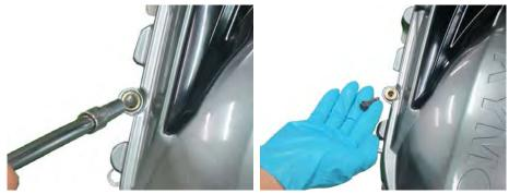
Remove the crankcase cover protector on the left side of the engine with a 8mm socket.
