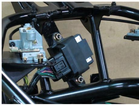
Note: The ignition control module or ECU maybe damaged if dropped or the connector is disconnected when the key is "ON". The excessive voltage may damage the ignition control module or ECU. Always turn off the ignition switch before servicing.
