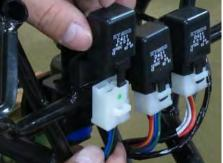
Remove and disconnect the Fan relay.
