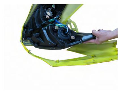
Install the light assembly on the front cover.
