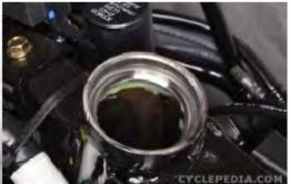
Drive the new bearing races into the steering head with a suitable driver with the same outside diameter as the bearing race.
