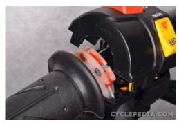
Lubricate the ends of the throttle cables with grease and fit them into the throttle tube.
