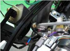
Connect the coolant hose to the thermostat. Move the clamp into place and tighten it securely with a #2 Phillips screwdriver.
