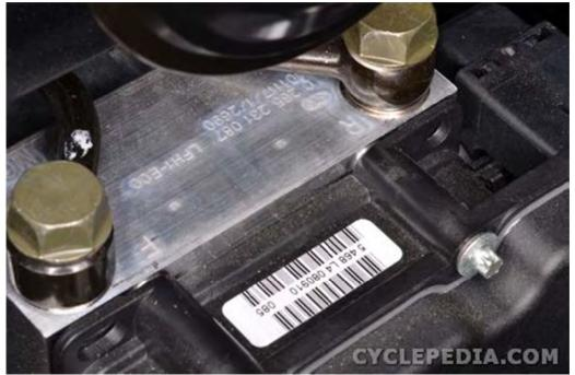
Note the markings on the ABS unit for the brake Front (F) and Rear (R) brake hose positions.
