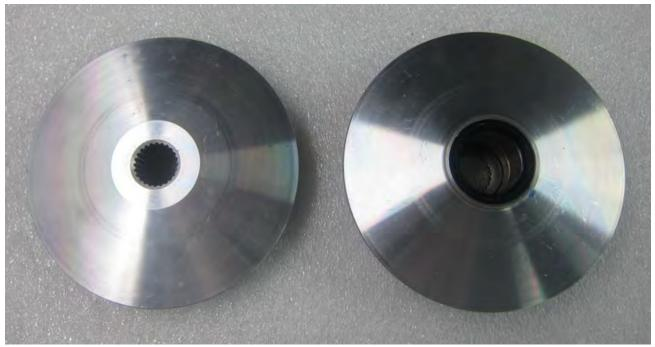
Inspect the faces of the drive pulley. Clean away any grease from the faces. Inspect the oil seal of the drive pulley for broken or excessive wear.
