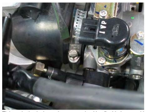
Tighten the intake hose clamp securely with a flat blade screwdriver.
