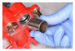
Remove the normal rear caliper piston.
