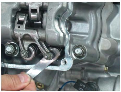
Measure the valve clearance with a thickness feeler gauge. Insert the feeler gauge between the tappet adjusting screw and the valve stem. The clearance is correct when there is a light drag on the feeler gauge. The clearance is the same for the exhaust and intake valves. If the clearance is out of spec, move on to the adjustment section.
