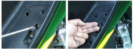
Remove the right leg shield mounting screws with a #2 Phillips.
