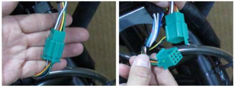
Unplug the green connectors for the right handlebar switches.
