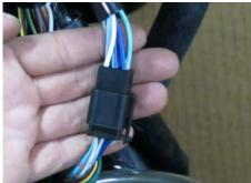
Plug in the black connector for the left handlebar switches.
