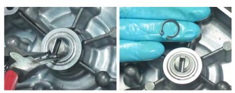
Remove the clip with the pliers and then remove the water pump shaft.
