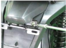
Install the two license plate nuts with a 10 mm socket.
