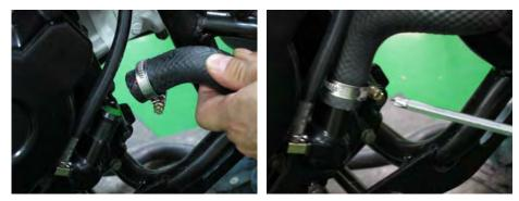
Connect the coolant hose to the water pump. Move the clamp into place and tighten it securely with a #2 Phillips screwdriver.
