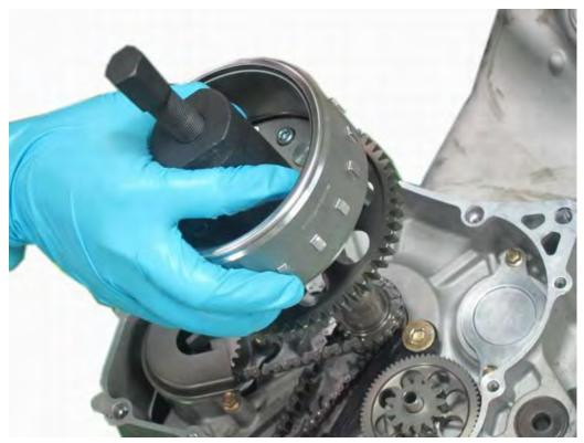
Remove the flywheel from the crankshaft.
