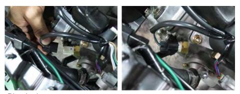
Plug in the water temperature sensor connector.
