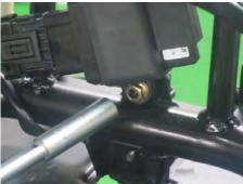
Install the two mounting nuts and tighten securely with a socket.
