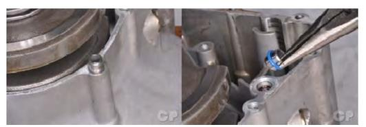
Remove the two dowel pins from the crankcase. Inspect the O-ring and replace it as needed.
