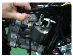
Remove the two ignition coil leads.
