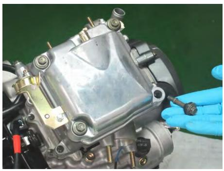
Coat the cylinder head cover bolt seals in fresh engine oil. Insert the cylinder head cover bolts with grommet seals and washers. Note the gold colored and longer bolts go on the right side.
