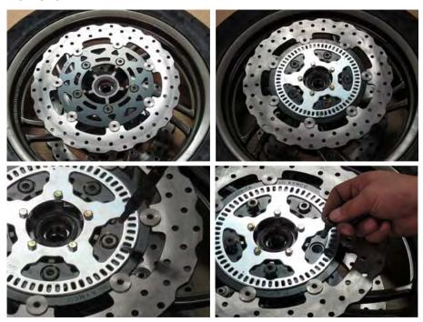
Remove the five mounting bolts with a 6 mm Allen.
