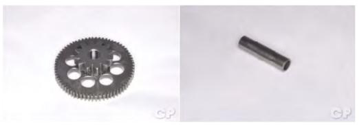
Inspect the starter idle gear and shaft for wear and damage. Replace the idle gear and shaft as needed.
