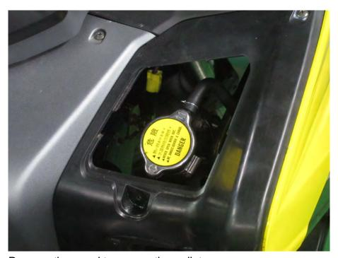
Remove the panel to access the radiator cap.
