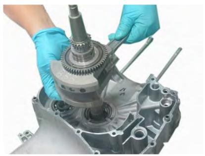
Fit the crankshaft into the left crankcase bearing. Take care to avoid damaging the new oil seal.
