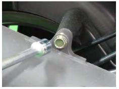
Install the three muffler mounting bolts and tighten to specification with a socket.
