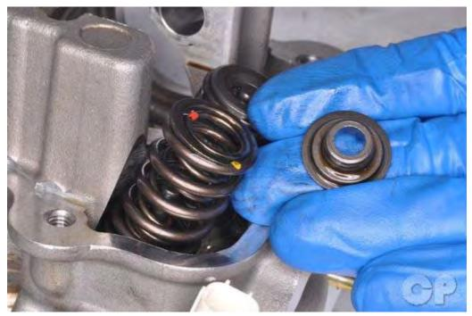
Remove the spring retainer.
