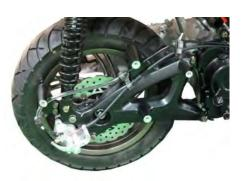
Install the lower shock absorber mounting bolts and torque them to specification with a 14 mm socket.
