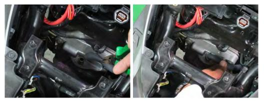
Install the breather hose to the cylinder head cover. Secure the hose with the clamp.
