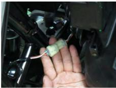
Install the connector output voltage device.
