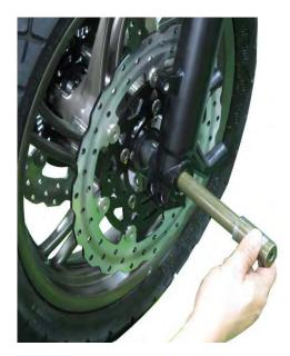
Support the front wheel and slide the front axle out from the left side.
