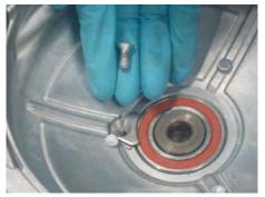
Remove the bearing fixed plate with a 5 mm Allen.
