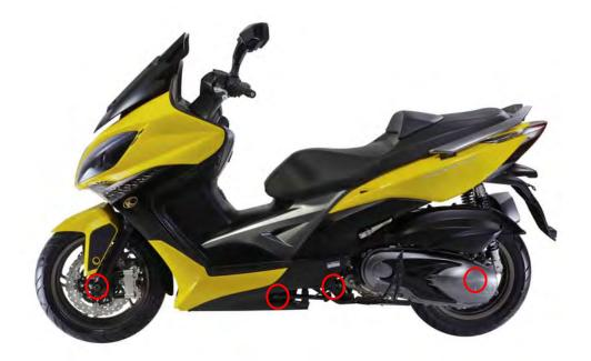
The frame lubrication points are listed below. Use general purpose grease. Apply clean engine oil or grease to cables and movable parts not specified. This will avoid abnormal noise and increase the durability of the motorcycle.
