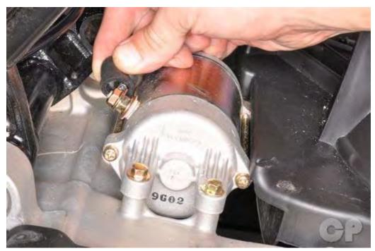
Fit the rubber starter motor lead cover into place.
