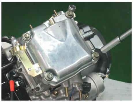
Tighten the cylinder head cover bolts securely in two steps and in a crisscross pattern with an 10 mm socket.
