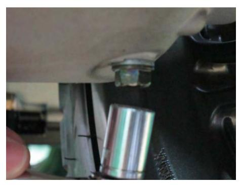
Install the oil drain plug and washer with a 12 mm socket. Tighten to specification.
