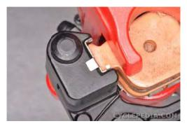
Fit the ends of the pads into the pad retainer as shown.
