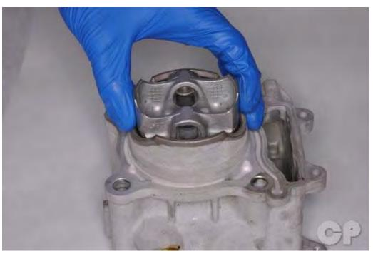
Insert the top ring into the cylinder. Push the top ring in the cylinder about an inch. Use the piston to push in the ring to keep it square with the cylinder.
