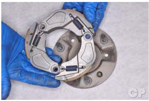
Slide the clutch shoes off of the pivots on the drive plate.
