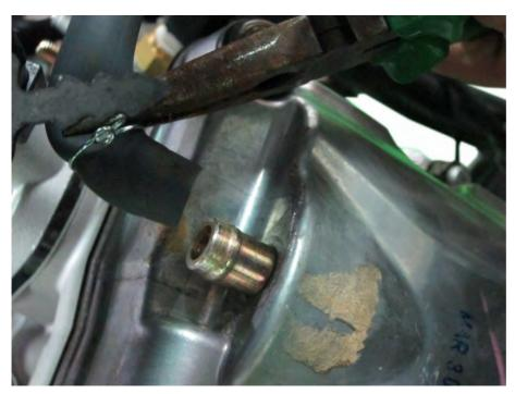
Disconnect the blow-by tube mounting the cylinder head with a splicer.
