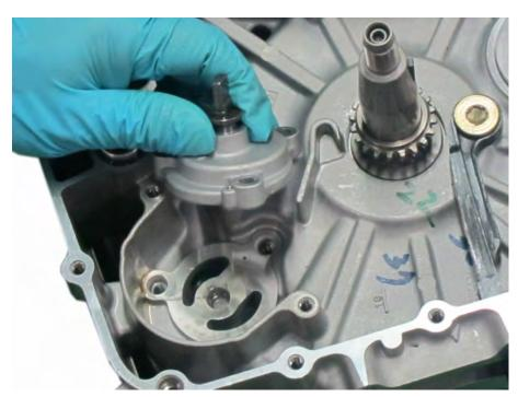
Fit the oil pump into place so that the arrow is pointing up.
