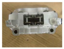
Install the brake pad as shown.
