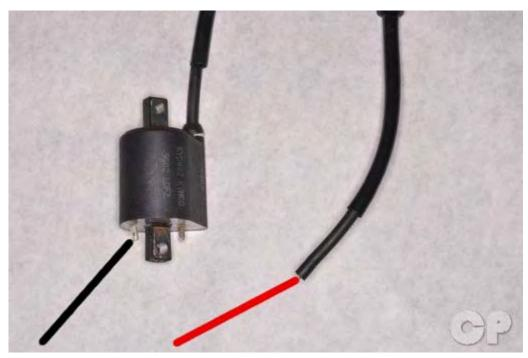
Check the secondary resistance between the ignition coil terminal and the spark plug wire without the cap. Touch the negative meter lead to the terminal and the positive meter lead to the spark plug wire as shown.
