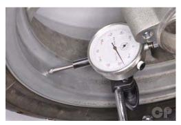
Check for radial hop. The service limit is 2.0 mm (0.08 in) or less.
