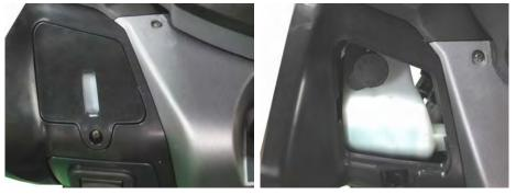
The coolant reserve tank is behind the inner cover. Remove the engine coolant lid screw with a #2 Phillips. Remove the engine coolant lid.
