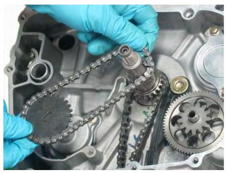
Remove the oil pump drive chain and driven sprocket.
