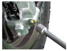
Install the two new caliper bracket mounting bolts. Tighten the mounting bolts to specification.
