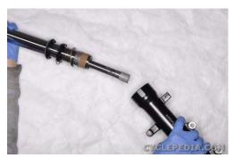
Insert the inner fork tube into the outer fork tube.
