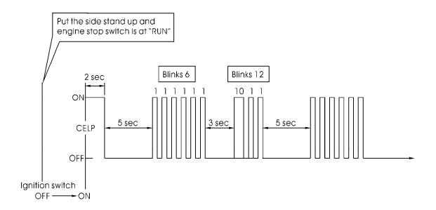
The "CELP" denotes the failure codes. When the indicator lights for one second is equal to ten.
