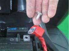
Remove the positive battery cable bolt with a 10 mm socket or #3 Phillips screwdriver. Free the positive cable from the battery.
