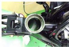
Inspect the bearings and races for wear and damage. Replace them as needed.
