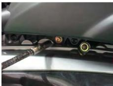
Install the two air box bolts and tighten securely with an 8 mm socket.
