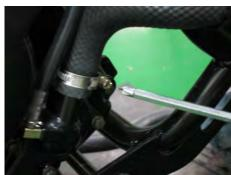
Connect the coolant hose to the water pump. Move the clamp into place and tighten it securely with a #2 Phillips screwdriver.
