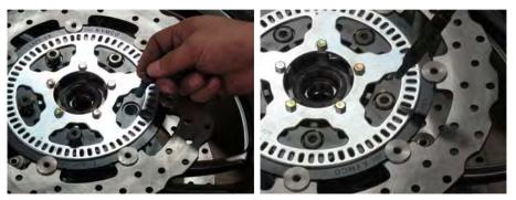
Coat the threads of the disc bolts in a non-permanent thread locking agent. Thread in the bolts and torque them to specification with an Allen socket.
