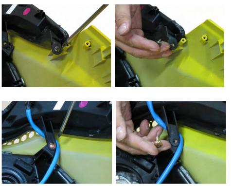
Remove the turn signal light assembly screws from the front cover.
