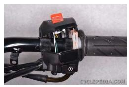
Separate the switch housing. The right switch housing has wires on both sides so it cannot be completely opened.
