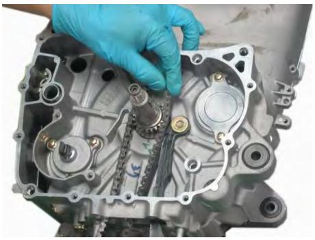
Remove the cam chain from the crankshaft and crankcase. Inspect the cam chain for wear and damage. Replace the cam chain as needed.
