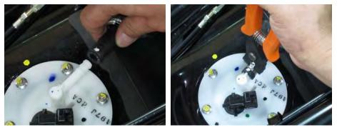
Connect the fuel hose to the outlet pipe on the fuel pump. Tighten the clamp securely with a special tool A120F00030
