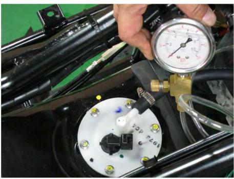
Disconnect the fuel hose from the fuel injector. Connect the fuel pressure gauge. Remove the fuel hose clamp. Turn the key to the ON position. Check the fuel pressure.
