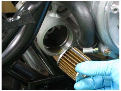
Pour a small amount of fresh engine oil into the oil filter. Insert the oil filter into place with the rubber seal side facing up.
