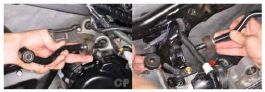
Fit the engine mounting bracket and damper assembly into place.
