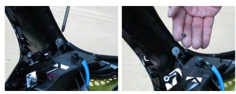
Remove the ten front side skirt mounting screws with a #2 Phillips.
