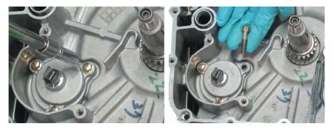
Remove the three oil pump screws with an 8mm socket.
