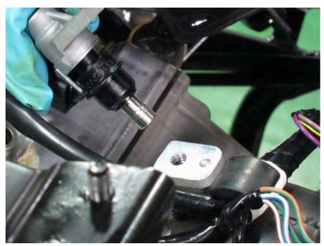
Fit the injector into the intake pipe as shown.
