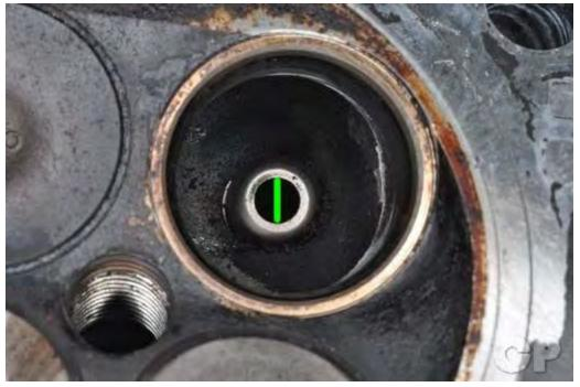
Measure the inside diameter of the valve guides. Replace the guides if the measurement is out of specification. Calculate the valve stem-to-guide clearance. Replace the guide and valve if the clearance is out of specification
