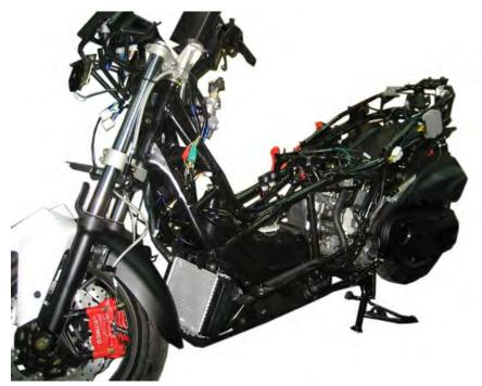
Route the cables down the inside of the left side of the frame.
