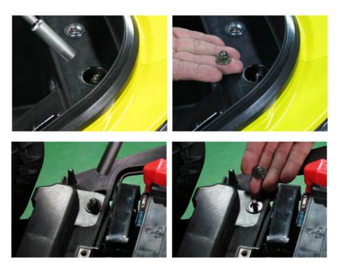
Remove the four luggage nuts with a 10 mm socket.
