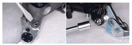
Tighten the brake lever bolt with a flat blade screwdriver and then tighten the nut with a 10 mm socket.
