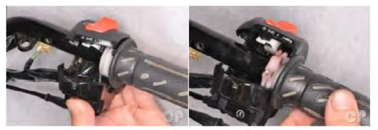
Separate the switch housing from the handlebar.
