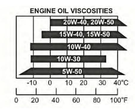
If these viscosities are not available, select an alternative engine oil according to the chart shown above.
