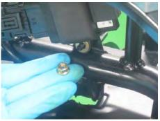
Remove the two mounting nuts with a socket.
