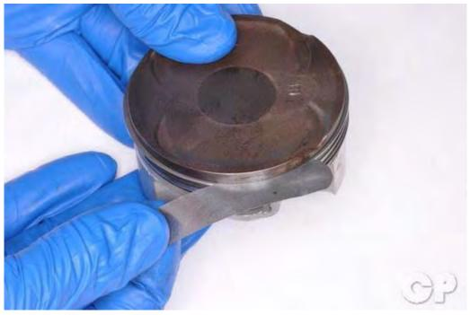
Measure the ring groove width and the ring-to-groove clearance with feeler gauges.
