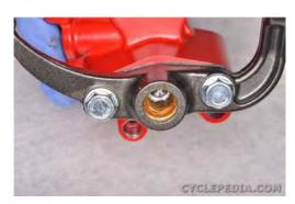
Install the two parking brake bracket bolts and tighten them to specification with a 12 mm socket.
