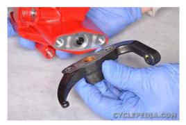
Fit the parking brake bracket into place with a new gasket.
