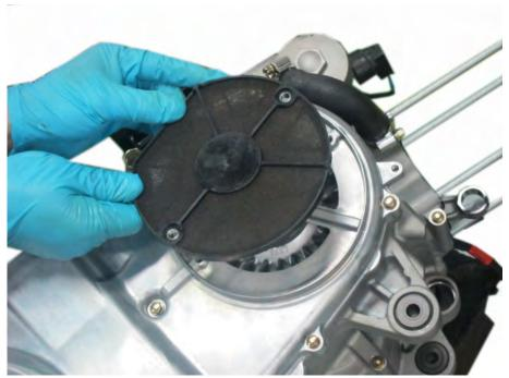
Remove the element duct.
