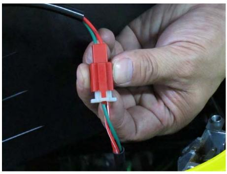
Unplug the two-pin luggage box light LED switch connector with red/white and green wires.
