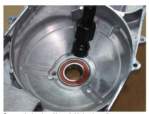
Remove the bearing with a suitable bearing puller.
