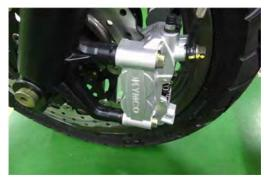
Push the caliper body inward to push in the pistons. This will allow room to change the brake pads.
