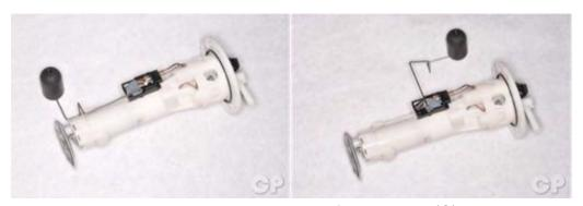
Using a digital multi meter set to ohms of resistance  $(\Omega)$ , measure the resistance between the fuel pump/level gauge connector terminals (green and yellow/white) with the float raised to the positions indicted below.
