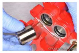
Remove the parking brake piston.
