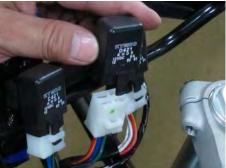
Remove and disconnect the high beam relay. The Low beam relay is on the left.
