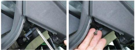
Remove the two screws mounting on the front cover meter on both side.
