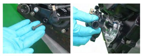
Remove the bolts and the water pump cover.
