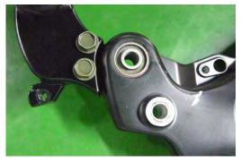
Inspect the shock absorber bushings for wear and damage. Replace the shock absorbers or bushings as needed.
