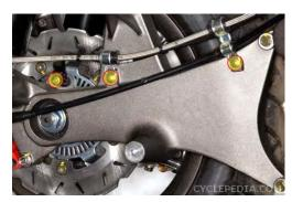
Install the rear wheel speed sensor and hose clamp bolts with an 8 mm socket.
