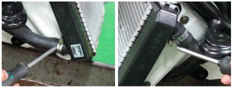
Connect the water pump and thermostat hoses in the same manner. Tighten the coolant hose clamp screws securely with a #2 Phillips screwdriver.
