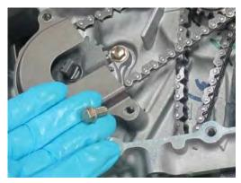
Remove the two oil pump cover bolts and the oil pump cover.
