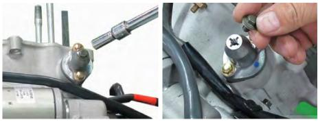
Remove the cam chain tensioner cap bolt with a 8 mm socket.
