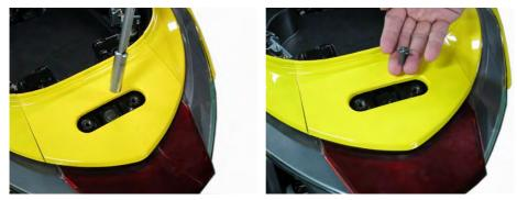
Remove the upper body cover bolt with a 10 mm socket.
