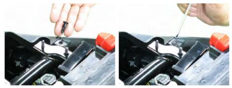
Install the two seat plastic screws from the front of body cover.
