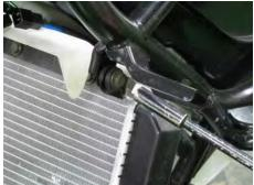
Install the two upper radiator mounting bolts and tighten them securely with a 10 mm socket.
