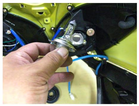
Fit the bulb into the lamp and then remove the headlight bulbs to free it from the lamp.
