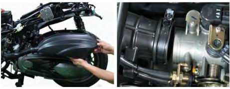
Fit the air box into the frame and guide the boot over the mouth of the throttle body.
