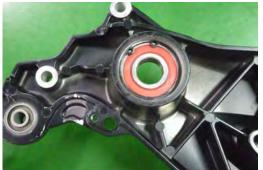
Inspect the wheel bearing by turning it with a finger. Replace the bearing and seal as needed. Remove the seal and snap ring. Drive the bearing. out from the inside out. Drive in the new bearing with a suitable driver that is the same outside diameter as the bearing. Install the snap ring into the groove. Apply grease to the lips of the new seal and drive it into place in the same manner as the bearing.
