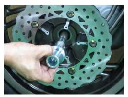
Apply grease to the lips of the dust seal and install the collar into the rear fork.
