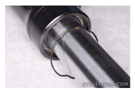
Install the stopper ring into the groove above the oil seal.
