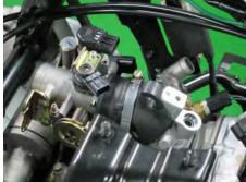
Loosen the intake hose clamp screw at the throttle body with a flat blade screwdriver.
