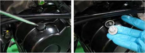
Remove the timing inspection cap from the right side of the engine with a large flat blade screwdriver. Inspect the O-ring on the cap and replace it as needed.
