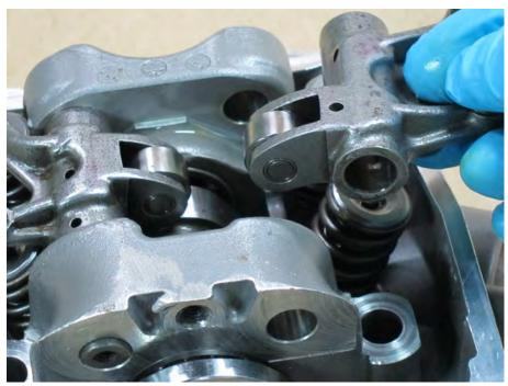
Lubricate the inside diameter of the rocker arms and the roller with fresh engine oil. Position the rocker arms to accept the rocker arm shafts.
