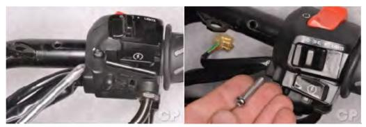
Remove the two right switch housing mounting screws with a #2 Phillips screwdriver. Disconnect the switch.
