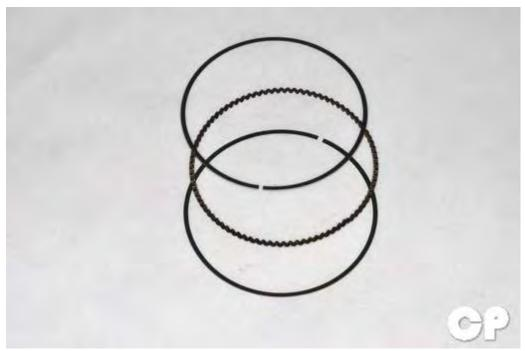
Install the oil expander ring so that the ends are not overlapping. Install the steel rails above and below the oil ring.
