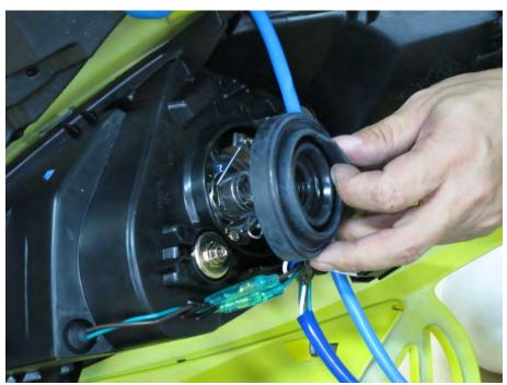
Fit the rubber cover into place. Make sure the rubber covers are secured in place.
