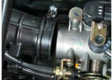
Remove the screw mounting the connecting tube airbox.
