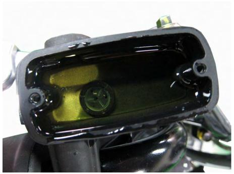
Make sure the reservoir has the proper amount of fluid.
