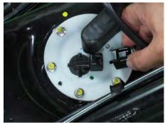
In order to release fuel pressure from the fuel pipe when removing the fuel injector, unplug the fuel pump connecter. Start the engine and let it run until it dies of fuel starvation. Turn the ignition switch off.
