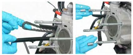
Slide out the lower cam chain guide. Inspect the guide for excessive wear and damage. Replace the guide as needed. Remove two towel pins
