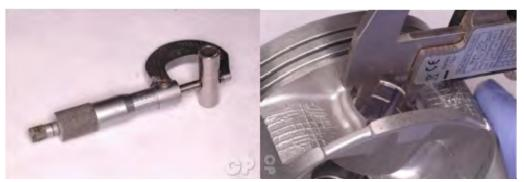
Measure the piston pin diameter with a micrometer. Measure the piston pin bore diameter with vernier calipers or a small bore gauge. Measuring at three different points for each. Replace the parts if any of the specifications are not met.
