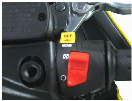
Set the engine stop switch to the "RUN" position.
