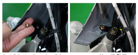
Install the two lower handlebar cover screws with a #2 Phillips.
