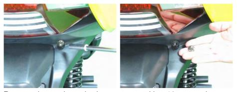
Remove the two lower body cover nuts with a 10 mm socket.
