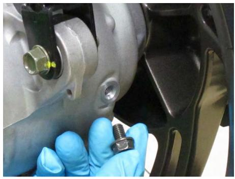
Thread in the final drive oil level check bolt.
