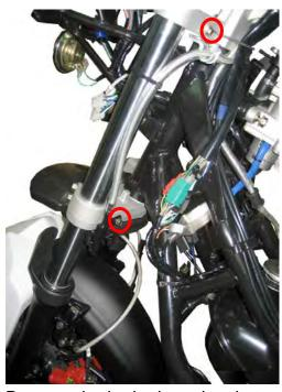
Remove the brake hose bracket on the left side of the lower fork clamp with an 8 mm socket.
