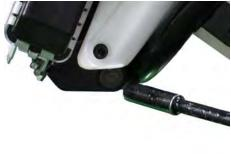
Remove the two radiator bottom mounting bolts with a 10 mm socket.
