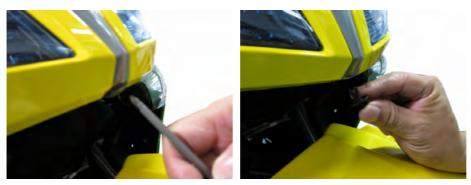
Remove the push pin. Depress the head of the fastener center piece. Pull out the fastener.
