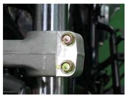
Tighten the lower fork clamp bolts evenly to specification with a 12 mm socket.
