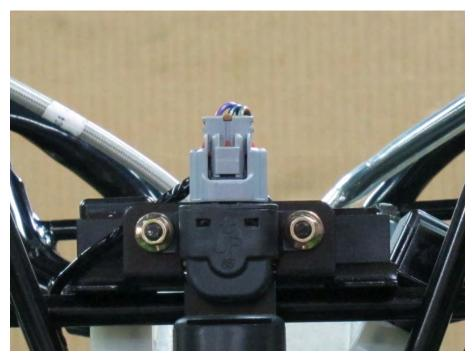
The tilt switch is under the front cover.
