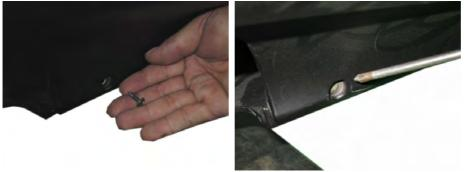
Install the two under cover screws on both sides with a 10 mm socket.
