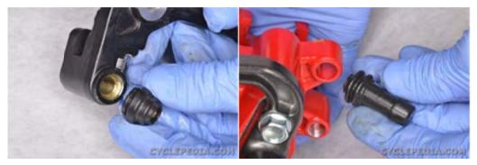
Install the caliper bracket pin boots.
