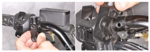
Remove the master cylinder clamp.
