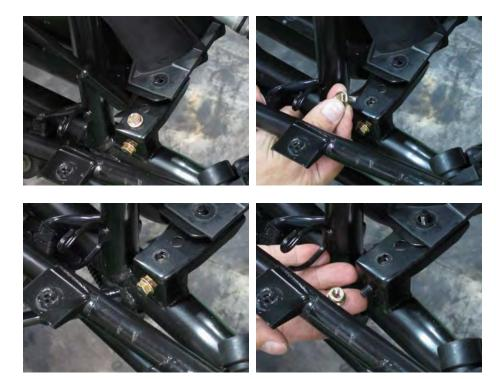
Remove the left fuel tank mounting bolts and brackets.
