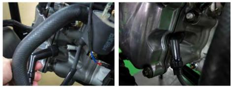
Install the spark plug wire over the plug.
