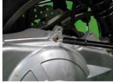
Install the belt case cover bolts and tighten them securely with an 8 mm socket.
