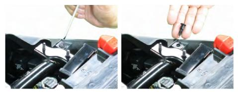
Remove the two seat plastic screws from the front of body cover. Remove the seat with the piston pivot.
