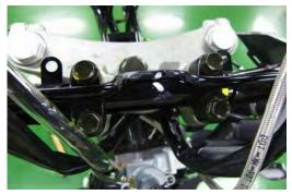
Tighten the handlebar bolts to specification with a 12 mm socket. Tighten the front bolts before the rear bolts.
