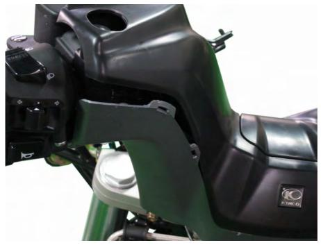
Install the tabs and the upper handlebar cover.
