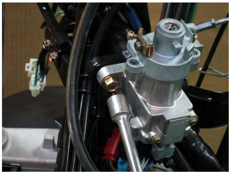
Remove the two Ignition Switch bolts with a 14 mm socket.
