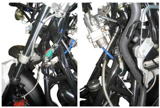
Install the brake hose guide to the left side of the lower fork clamp and tighten its bolt securely with an 8 mm socket.
