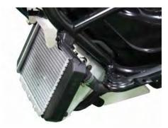
Fit the radiator into place so that the post on the frame fits into the rubber grommet on the right side of the radiator.
