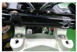
Install the handlebar onto the holders. Fit the posts into the holes as shown.
