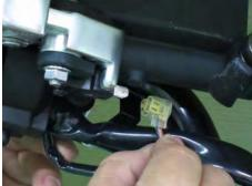
Unplug the brake light switch connectors.
