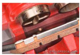
Make sure the post on the inner pad fits into the groove in the parking brake piston.
