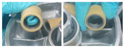
Remove the rollers and check them for excessive or uneven wear. Measure the weight of the rollers. Replace the weight rollers as needed.
