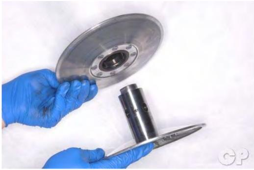
Separate the left and right faces of the driven pulley.
