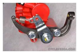
Loosen the parking brake lock nut with a 10 mm wrench.
