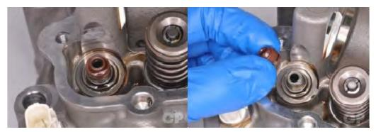
Remove the valve seal from the valve guide. The valve seals should be replaced if they are removed or you are going to install new valves.
