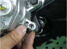
Remove the brake pad pin plug with a flat blade screwdriver.
