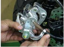
Free the parking brake cable from the rear brake caliper.
