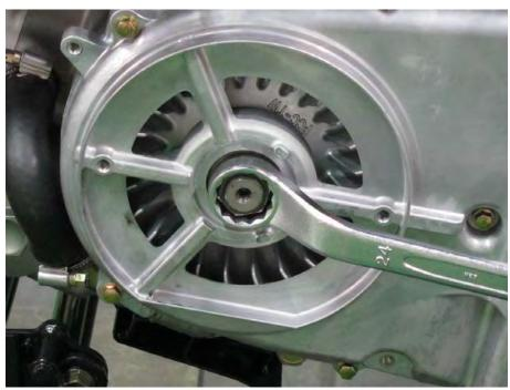
The crankshaft must be rotate until the piston is at top dead center (TDC) on the compression stroke.
