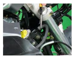
Install the bottom hose is the overflow hose that runs to the filler neck.
