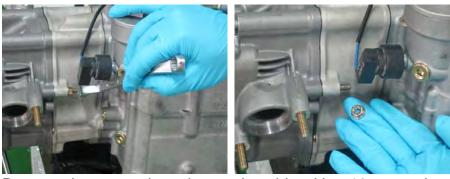
Remove the nut on the exhaust pipe side with a 10mm socket.
