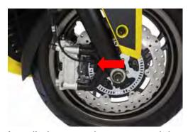
Install the speed sensor and its mounting bolt to the right fork leg. Tighten it securely with an 8 mm socket.
