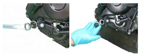
Remove the oil strainer screen bolt with a 17 mm socket. Inspect the strainer screen bolt O-ring and replace it as needed.
