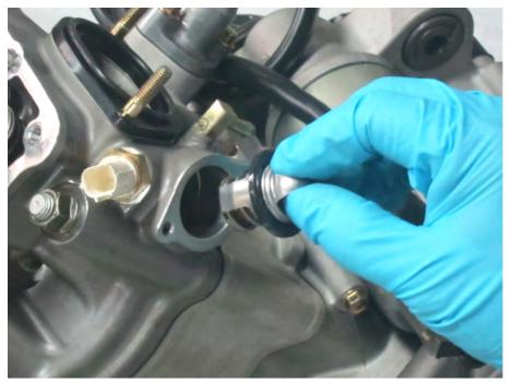
Make sure the thermostat seal is in good condition. Replace the thermostat if needed. Apply a light coat of waterproof grease to the thermostat seal. Insert the thermostat into its cavity in the cylinder head.
