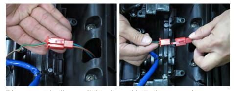
Disconnect the license light wires with the harness wires.
