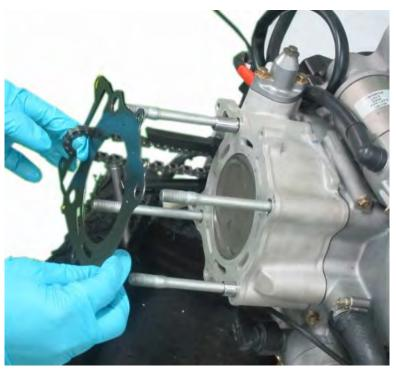
Install the new base gasket onto the crankcase.
