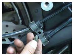
Remove the two rear brake hose holder mounting bolts with a 8 mm socket.
