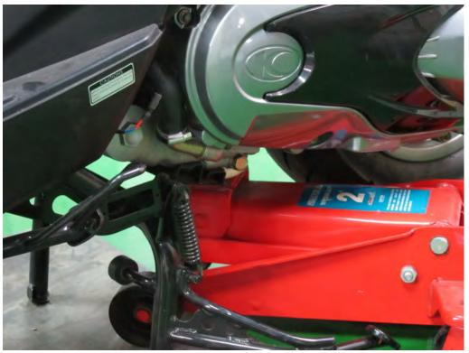
Set the chassis on its center stand. Use a jack to support the engine. Guide the engine into the back of the frame.
