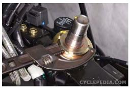
Tighten the steering stem adjusting nut to the initial specification with a pin spanner or the special wrench.
