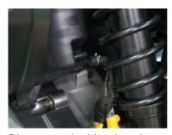
Disconnect the blow-by tube mounting the transmission box assy.
