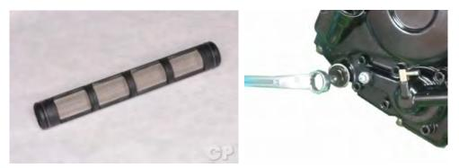
Return the O-rings to the oil strainer screen and install it into the left side of the engine. Tighten the oil strainer screen cap to specification with a 17 mm socket.
