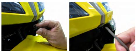
Align the two posts with the grommets. Carefully push on the small black cover. Install the small black cover push pin.
