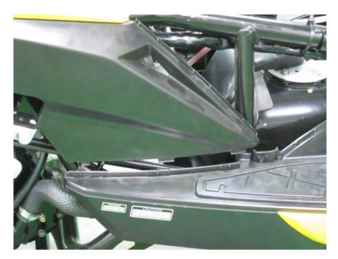
Carefully unhook the tabs on both sides of the body cover.
