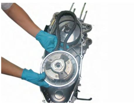
Slide the driven pulley off of the shaft.
