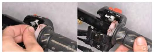
Lubricate the end of the throttle in grease. Fit the ends of the throttle cables into the throttle tube.
