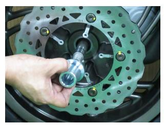
Install the rear axle collar as shown.
