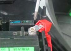
Connect the positive battery cable and install the bolt with a 10 mm socket or #3 Phillips screwdriver.
