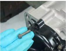
Remove the 12 generator cover bolts with an 8 mm socket. Note the upper bolt holds a wire stay.
