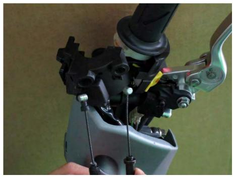
Guide the throttle cables out towards the handlebar side.
