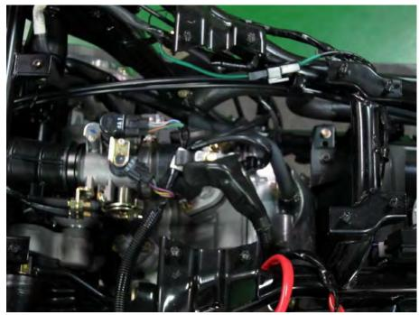
Route the cables to the throttle body as shown.
