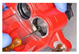
Remove the seals with a mechanics pick. Discard the old seals.
