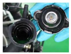
Remove the panel to access the radiator cap.
