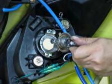
Slide back the rubber headlight covers and then remove the headlight bulbs to free it from the lamp.
