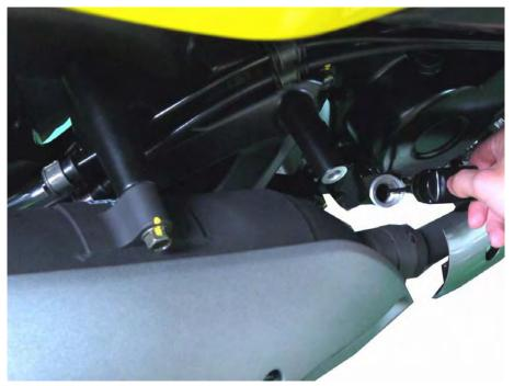
Remove the oil filler cap to allow for faster oil draining. Inspect the oil filler cap O-ring and replace it as needed.
