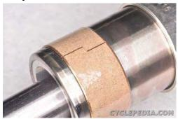
Inspect the fork bushings. Replace the guide bushing if needed. The inner fork tube bushing must be replaced with the inner fork tube if it is in poor condition.
