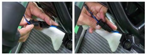
Plug in the cooling fan motor connector.
