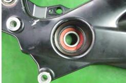
Inspect the wheel bearing by turning it with a finger. Replace the bearing and seal as needed.
