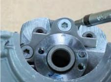
Apply a small amount of blue Loctite (non-permanent) to the threads of the set plate bolt. Thread in the bolt and tighten it to specification with a
