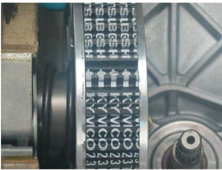
Inspect the drive belt for cracks or excessive wear.
