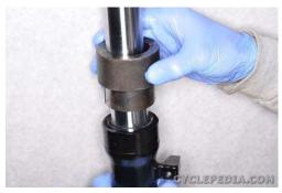
Drive the guide bushing into position in the outer fork tube using the fork seal driver. If a fork seal driver is not available, you can use a piece of PVC pipe that has been split down the middle. Make sure the bushing is fully seated in the outer fork tube. Drive in the oil seal in the same manner.
