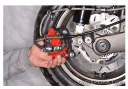
Fit the rear brake caliper into place. Insert two new mounting bolts.
