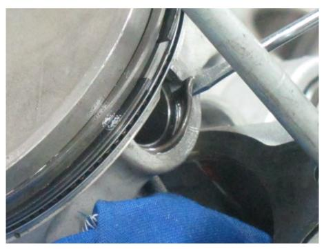
Remove the piston pin clips with a pick or needle nose pliers. Discard the piston pin clips.
