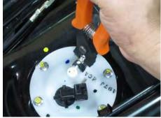
To clip the fuel hose with a special tool A120F00031 and loosen the clamp with a special tool A120F00030
