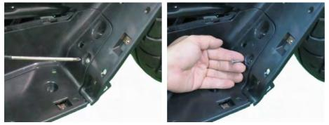
Remove the mounting screw with a #2 Phillips on right side.
