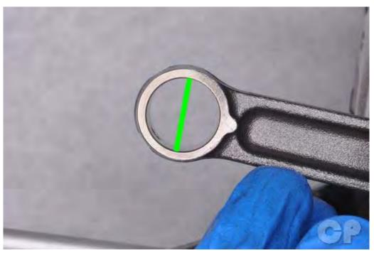
Measure the inside diameter of the small end of the connecting rod with vernier calipers.
