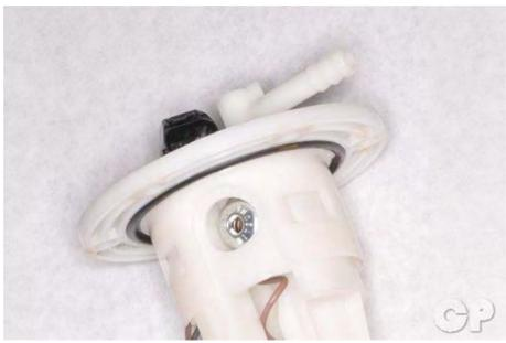
Replace the O-ring with new item and apply a small amount of fresh engine oil to the new O-ring.
