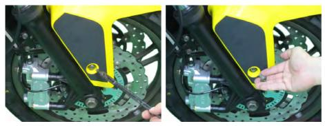
Remove the forward front fender bolts with a 6 mm Allen on both side.
