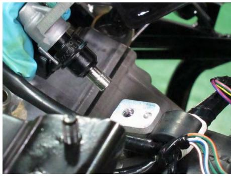
Lift the fuel injector out of the intake pipe.
