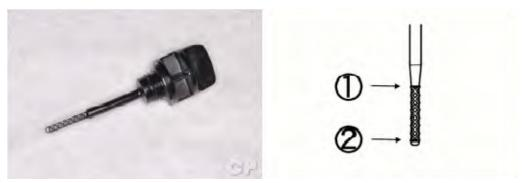
The level must be maintained between the upper (1) and lower level (2) marks on the oil filler cap/dipstick.
