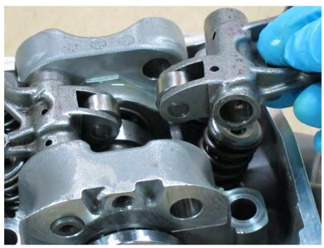
Lift out the rocker arms as the shafts are removed.
