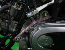
Fit the drain hose to the plastic belt case cover as shown.
