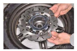
Fit the rear brake disc into place on the wheel as shown.
