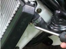
Remove the water pump and thermostat hoses in the same manner.
