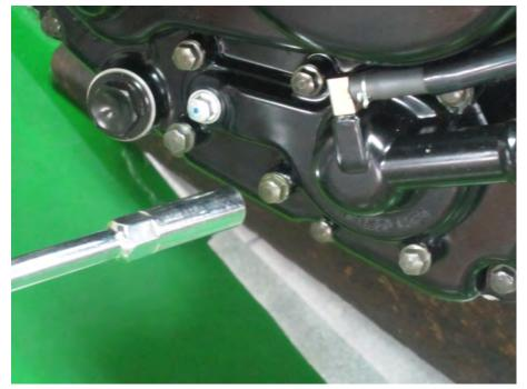
Tighten the water pump cover bolts to specification with an 8 mm socket.
