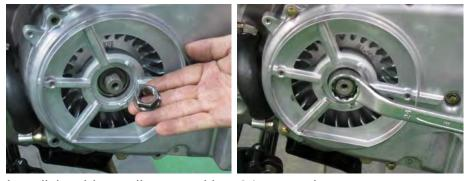
Install the drive pulley nut with a 24mm socket.
