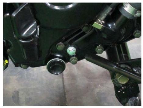
Tighten the drain bolt securely with an 8 mm socket.
