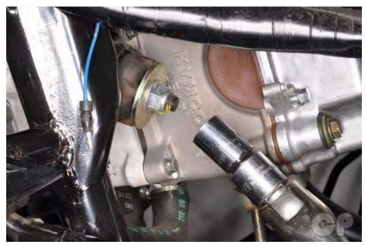
Tighten the damper nut securely with a 14 mm socket.
