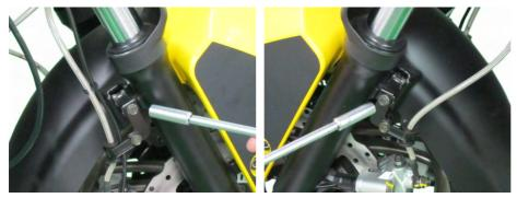
Install the forward front fender bolts with a 10 mm socket on both side.
