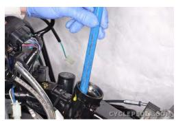
Use the special tools or a drift and hammer to drive out the bearing races in the steering head.
