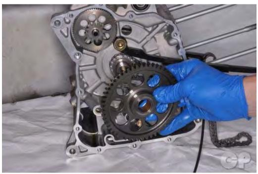
Lubricate the inside of the starter driven gear with fresh engine oil. Slide the starter driven gear onto the flywheel as shown.
