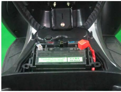
The battery is located under the seat.
