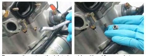
Remove the nut on the inlet pipe side with a 10mm socket.
