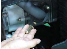
Remove the two exhaust pipe joint nuts with a 12 mm deep well socket.
