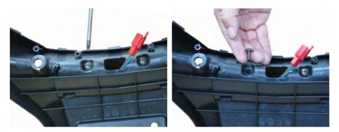
Remove the two license light cover screws with a screwdriver.
