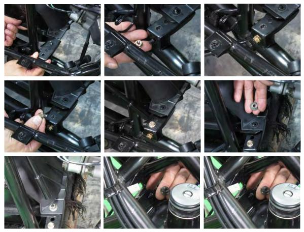
Install the brackets and nuts/bolts. Tighten the nuts/bolts securely.
