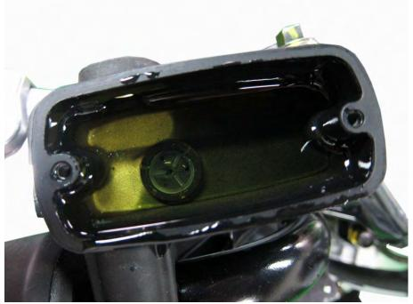
Fill the brake fluid with the proper type from a fresh, newly opened container.
