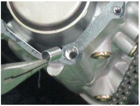
Make sure the generator cover mating surface is clean. Install the two dowel pins and a new generator cover gasket.
