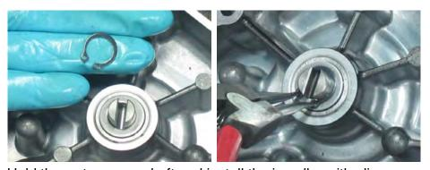
Hold the water pump shaft and install the impeller with pliers.
