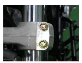
Loosen the lower fork clamp pinch bolts with a 12 mm socket. The top bolts must be removed.
