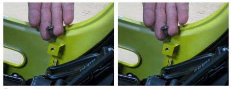
Remove the two rear center cover screws.
