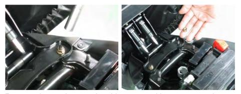
Remove the two luggage box hinge nuts with a 10 mm socket.
