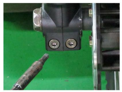
Loosen the front axle pinch bolt with a 6 mm Allen.
