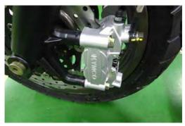
Place a suitable container under the banjo bolt to catch any remaining brake fluid. Remove the banjo bolt that holds the brake hose to the caliper using a 12 mm socket. Discard the two sealing washers.
