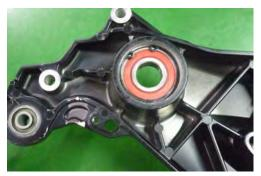
Install the snap ring into the groove.
