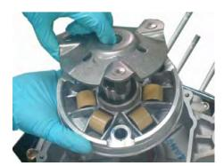
Lift the ramp plate out of the back of the left drive pulley face.
