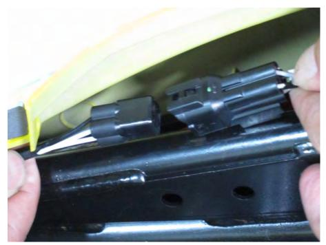
Measure the resistance between the white wire terminals of the  $O^2$  sensor connector. Replace the  $O^2$  sensor if the reading is out of specification.
