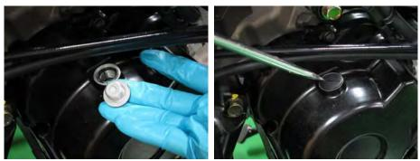
Make sure the O-ring on the timing plugs are in good condition. Replace it as needed. Install the timing inspection cap to the right side of the engine. Tighten the cap securely but not overly with a large flat blade screwdriver.
