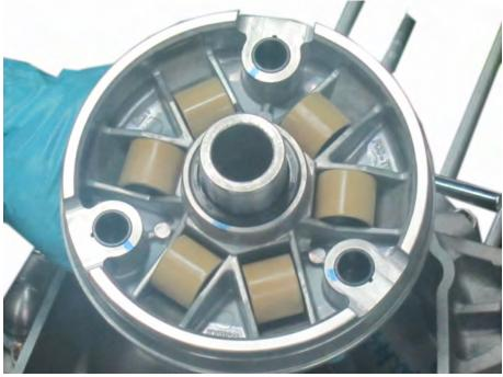
There are 6 weight rollers in the back of the right face of the drive pulley.
