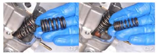
Remove the valve springs.
