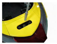
Install the upper body cover bolts and tighten securely with a 10 mm socket.
