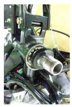
Remove the inner race for the upper bearing.
