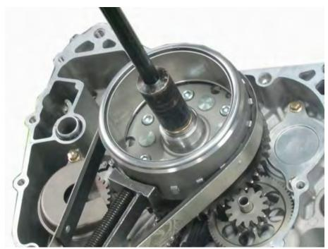
Hold the flywheel with the universal holder and loosen the nut with a 19 mm socket.
