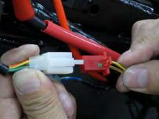
Disconnect the starter relay wire connector.
