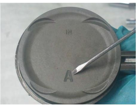
The "IN" mark should face the intake side (rear) of the engine.
