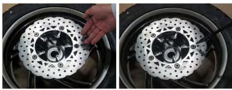
Apply a non-permanent thread locking agent to the threads of the rear disc bolts. Insert the bolts and tighten them to specification with a 6 mm Allen.
