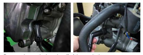
Remove the spark plug wire off of the spark plug.
