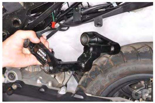
Remove the engine mounting bracket.
