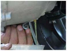
Place a suitable container under the drain plug to capture the final drive oil. Loosen the oil drain plug with a 12 mm socket. Remove the drain plug and slowly rotate the rear wheel to drain the transmission oil.
