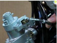
Remove the seat latch cable screw and free the seat latch cable from the ignition switch.
