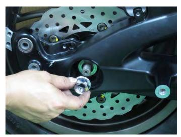
Install the rear axle nut and tighten it to specification with a 24 mm socket.
