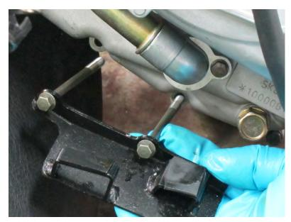
Remove the plate with the bottom two crankcase bolts.
