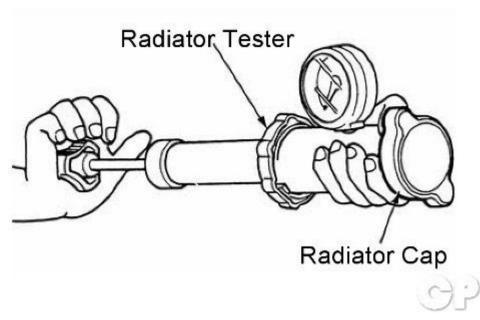
Wet the seal on the radiator cap and install it to the pressure tester. Replace the cap if it does not relieve the pressure as specified.
