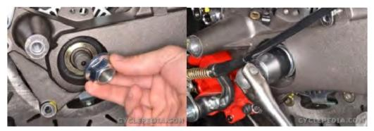
Install the rear axle nut and tighten it to specification with a 24 mm socket.
