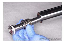
Remove the damper rod and rebound spring.
