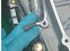
Loosen the right crankcase coolant hose clamp with a 8mm socket. Slide up the clamp and free the coolant hose from the right crankcase cover. Allow any remaining coolant to drain into a suitable container.
