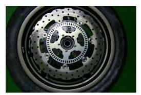
To remove the speed sensor rotor take out the five bolts.
