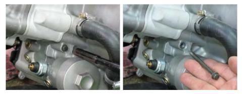
Loosen the 12 crankcase bolts in a crisscross pattern with an 8 mm socket. Remove the crankcase bolts from the left side of the engine.
