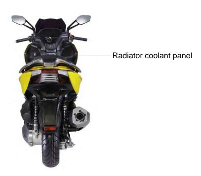
Remove the radiator coolant panel screws with a #2 Phillips screwdriver.
