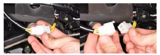
Disconnect the generator 3-pin connector.
