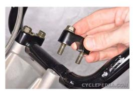
Remove the handlebar holders and bolts.
