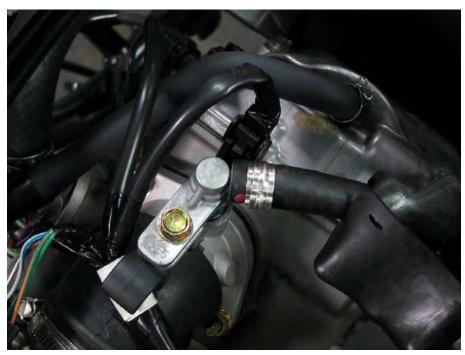
Free the wiring harness from its guide above the intake pipe.
