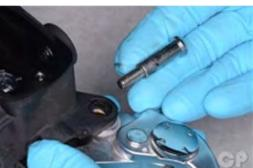
Remove the pivot nut and bolt.
