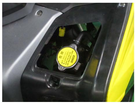
Install the radiator cap access panel.
