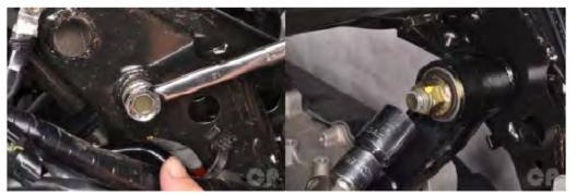
Hold the engine mounting bolts with a 14 mm wrench and loosen the nuts with a 19 mm socket.
