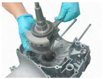
Lift the crankshaft out of the left crankcase half.
