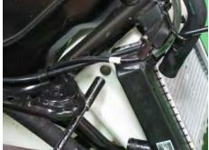
Remove the two radiator upper mounting bolts with a 10 mm socket.
