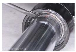
Use a small flat blade screwdriver to pry out the fork oil seal stopper ring. Take care to avoid scratching the fork tube.
