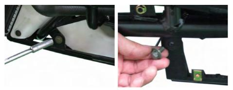
Remove the two under cover bolts on both sides with a 10 mm socket.
