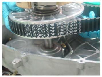
Remove the belt from the driven pulley.
