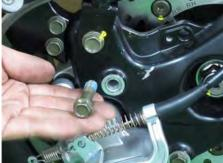
Remove the two rear caliper mounting bolts with a 12 mm socket.
