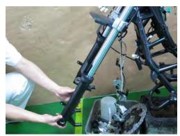
Slide the forks legs down and out of the fork clamp using a twisting motion.
