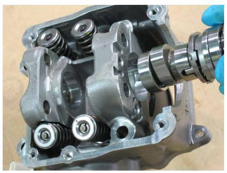
Insert the camshaft into the camshaft holders with the lobes facing down.
