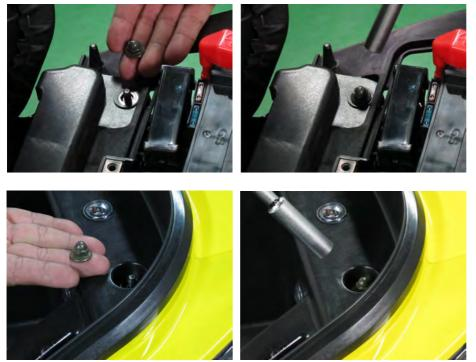
Install the four luggage nuts and tighten securely with a 10 mm socket.
