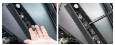
Install the four cover windshield bolts with a 6mm Allen. There are two bolts on each side
