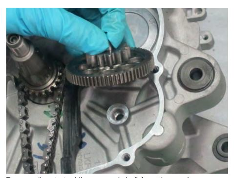
Remove the starter idle gear and shaft from the crankcase.
