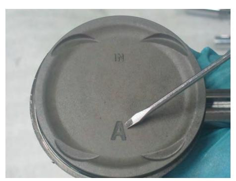
Clean the piston ring grooves and apply fresh engine oil to the piston rings. Spread the rings the minimum amount possible to install them. Do not try and force them on the piston.
