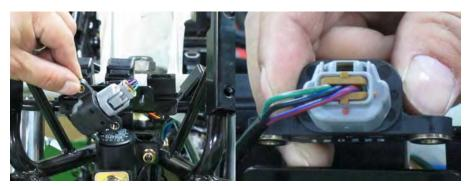
Incline the tilt switch 65±10 degrees to the left or right at the ignition switch "ON". Measure the voltage as below.
