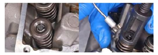
Remove the split keepers. There are two per valve.
