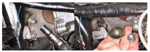
Loosen the engine mounting bracket damper nut with a 14 mm socket. Remove the nut and washer.
