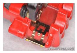
Install the brake pad spring into the caliper.
