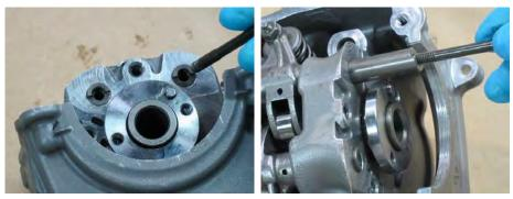
Thread a bolt into the rocker arm shafts and pull the shafts out.
