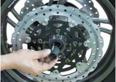
Apply grease to the lips of the dust seals and collar O-rings. Insert the collars into the hub as shown.
