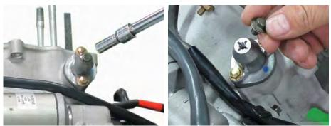
Make sure the cam chain tensioner cap bolt washer is in good condition. Install the washer and cam chain tensioner cap bolt. Tighten the bolt to securely with a 10 mm socket. Check the valve clearance.
