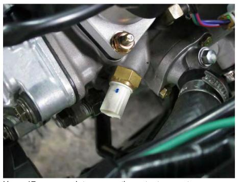
Use a 17 mm wrench to remove the water temperature sensor.
