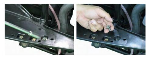
Remove the three mounting bolts on left side with a 10 mm socket.
