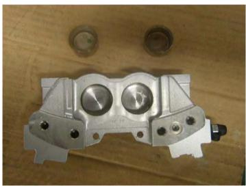
Lubricate the caliper pistons, the caliper piston bores with DOT 4 brake fluid from a tightly sealed container.
