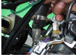
Loosen the thermostat hose clamp with a #2 Phillips screwdriver. Slide up the clamp and free the coolant hose from the thermostat. Allow any remaining coolant to drain into a suitable container.
