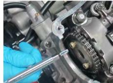
Install the camshaft sprocket onto the camshaft so the camshaft sprocket boss fits into the appropriate hole on the camshaft sprocket.
