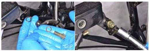
Install the brake hose to the master cylinder with the banjo bolt. Use new sealing washers. Tighten the banjo bolt to specification with a 12 mm socket.
