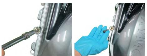
Remove the six bolts mounting the left crankcase cover protector.
