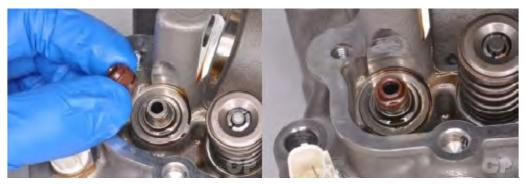
Coat the new valve seal in fresh engine oil and install it onto the valve guide.
