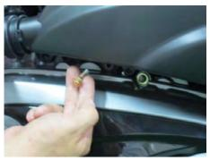
Remove the two air box bolts with an 8 mm socket.
