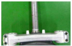
Drive the new lower bearing inner race with dust seal onto the steering stem with a pipe with the same outside diameter as the bearing race. Use a press if available.
