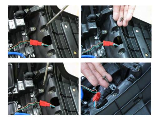
Remove the four mud flap screws with a #2 Phillips.
