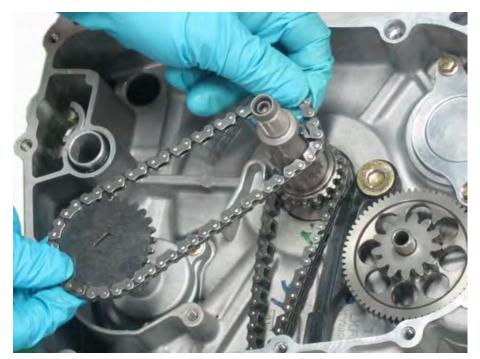
Fit the oil pump driven sprocket into the drive chain. Install the gear onto the oil pump shaft and fit the chain onto its teeth on the crankshaft.
