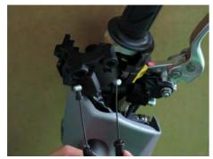
Route the throttle cables out of the handlebar cover.
