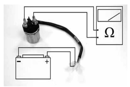
Connect the electric meter to the starter relay terminals that connect to the battery positive cable and the starter motor cable. Connect a fully charged battery across the starter relay yellow/red and green/yellow wire terminals. Check for continuity between the starter relay large terminals. The relay is normal if there is continuity and hear sounds.
