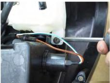
Remove the left reserve tank mounting bolt with a 10 mm socket and bottom screw with a #2 Phillips screwdriver.
