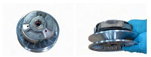
Inspect the clutch shoe lining thickness. Replace the shoes if the wear is below the service limit.
