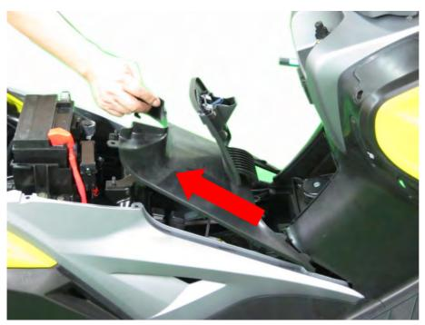
Pull the center cover back and up to free the claws and then move the cover backward to free it from the scooter.
