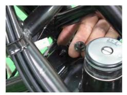
Remove the front fuel tank mounting nuts.
