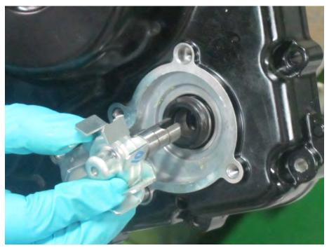
Remove the impeller.
