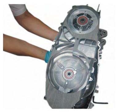
Inspect the belt case bearing by turning it with a finger. Replace the bearing if it is rough or noisy.
