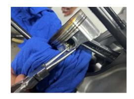
Remove piston pin by suitable tools. Remove piston
