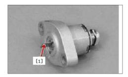
To fasten the installation bolt[1] of tensioner.
