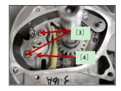
Note: Before disassembly, the oil needs to be drained
