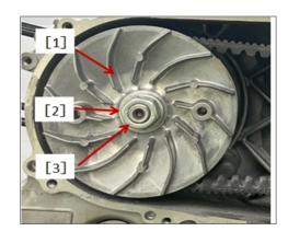
• Install turning stop fixture, then fasten nut for transmission belt. Fastening torquefor driving wheel:  $(63\sim77)~\text{N} \cdot \text{m}_{\circ}$
