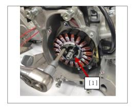
Straighten up wires of trigger, install wire pressing plate, then fasten bolt to given torque. Install trigger fastening bolt, then fasten to given torque. Torque: 9Nm (9kgfm, 6.66bfft)
