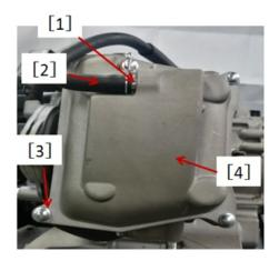
Installation of Cylinder head cover
