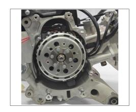
Fix rotor [1] of magneto by its fixer, Disassemble fastening nut by torque wrench [2].
