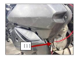
Remove the fuel tank and hold. Check crankcase exhaust pipe [1] for cracks, aging, damage and loosening. Replace the exhaust pipe if necessary. Install fuel tank.
