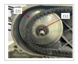
• Disassembly: Sloping plate [1] and its side piece [2].
