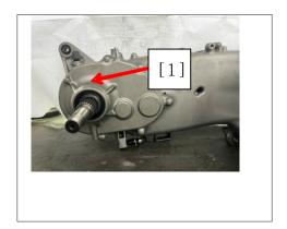
Remove countershaft kit [1] and output shaft kit [2].
