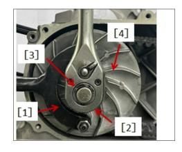
• Disassembly: Sleeve [1] for sliding & driving plate Sliding & driving plate [2]
