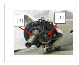
Remove gasket [1] of gear box and positioning pin. [2].
