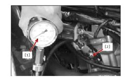
• Start engine, fully open throttle until data on cylinder pressure gauge stopped rising, now the data is the highest pressure in cylinder. Range for cylinder pressure:  $(800 \sim 1200) \, \text{kPa} (900 \sim 1100 \, \text{rpm})$ .
