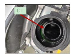
Remove air from the cooling system as follows:
