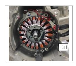
Installation for hall sensor, preinstallaxial bolt of socket hexagon, pre-fasten to given torque. Torque: 9Nm (9kgfm, 6.7lbfft)
