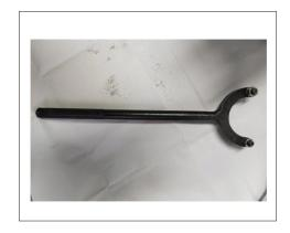
Fixture for removing rotor of magneto
