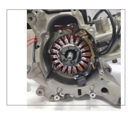
Lock up crankshaft by rotor fixture. Install stator, then nstall flat washer to crankshaft, and fasten nut to given torque.
