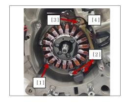
Remove fastening screw [1] of stator by socket hex. wrench. Remove stator kit of magneto.
