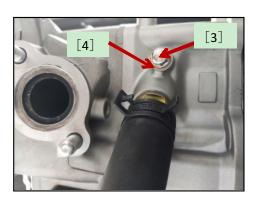
3. After replacing the new flat washer, preinstall the drain bolt  $(2 \sim 3)$  teeth on the cylinder block and tighten the bolt. Torque:
