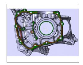
Install positioning pin, install right crankcase onto left one, installation case combination bolts and fastening to given torque.
