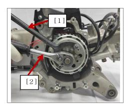
Eject out fixture [1] by magneto, then remove the rotor.
