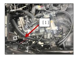
Spark Plug Remove the fuel tank.
