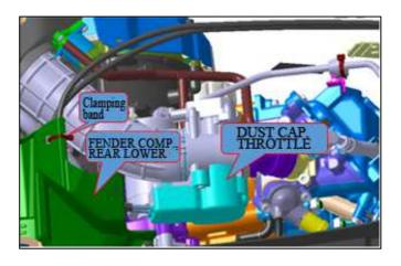
② Remove the greaser base 7 on handle bar, then remove the upper end of 2 throttle cables, cut off the clamping bad on rear fender, then remove the throttle cable 8 and replace for a new one with same specification.
