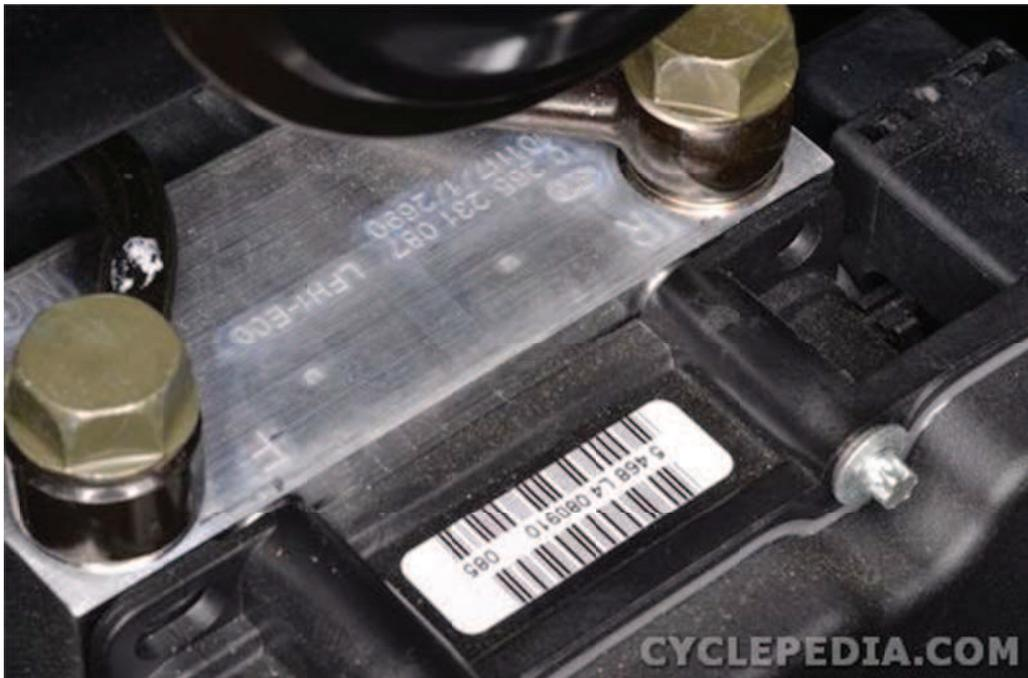
Note the markings on the ABS unit for the brake Front (F) and Rear (R) brake hose positions.
