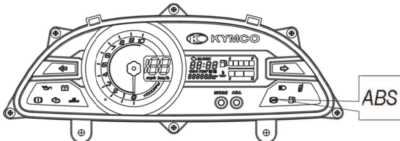
The ABS indicator light is on the right side of the meter. This light will come on when the ignition switch is turned on and goes off shortly after the vehicle starts moving it stays off as long as the system is ok.
