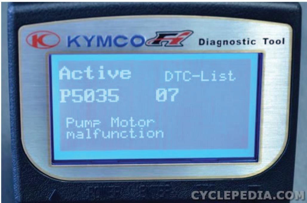
Check and clear the ABS DTCs in the same manner as the fuel injection DTCs.
