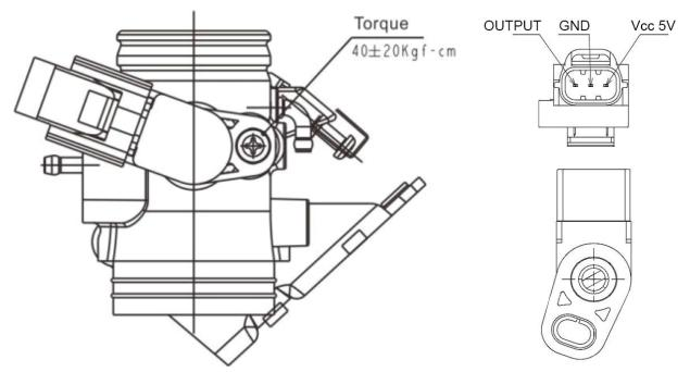
When installation, apply oil onto a new O-ring. Install the TPS onto the throttle body, being careful not to damage the O-ring. Install and tighten the screw securely.
