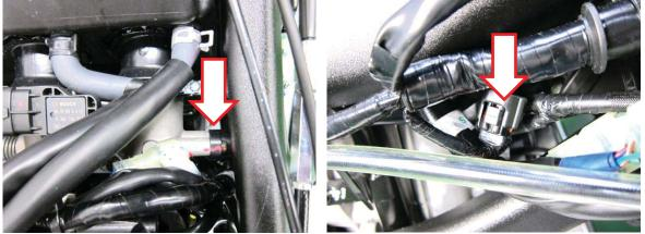
Measure if the ECU voltage outputs to TPS between the following terminals of the TPS connector.
