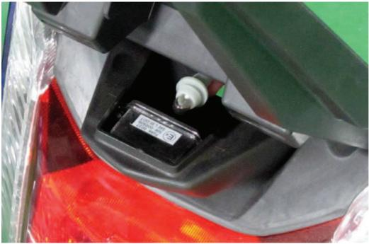
Pull the rubber tag light socket out of its housing. Pull the bulb straight out and insert a new one.
