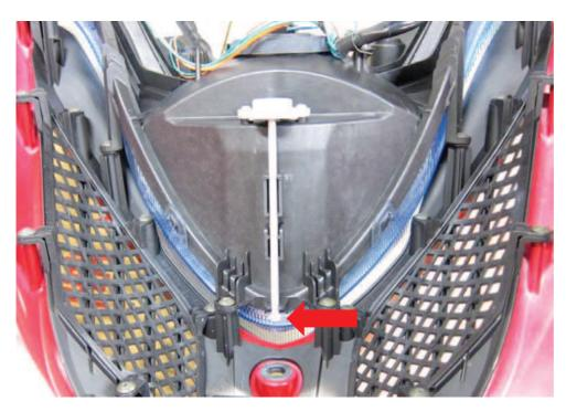
Turn the screws to adjust the head light aim as needed.
