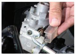
Remove the seat latch cable cover.
