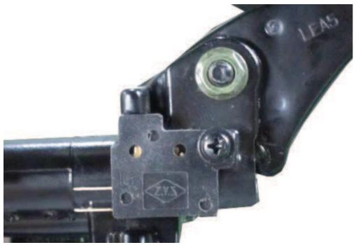
Check for continuity between the brake light switch connectors. There should be continuity when the lever is pulled and none when released.
