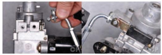
Fit the end of the seat latch cable into the ignition switch.
