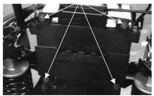
Install the battery cover. Install the four battery cover screws and tighten them securely.
