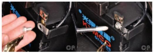
Connect the negative battery cable and install the bolt with a 10 mm socket or #3 Phillips screwdriver.
