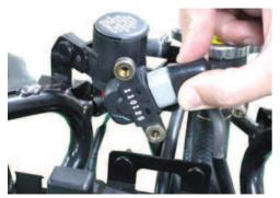
Incline the tilt switch 65±10 degrees to the left or right at the ignition switch "ON". Measure the voltage as below.
