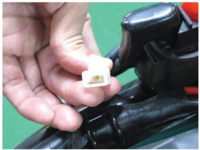
Check for continuity between the yellow/red wire and green/yellow wire. There should be continuity when the starter button is depressed. If there is no continuity, check the starter button for continuity and inspect the wire.
