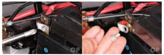
Remove the positive battery cable bolt with a 10 mm socket or #3 Phillips screwdriver. Free the positive cable from the battery.
