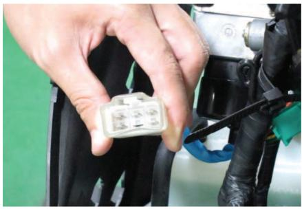
Use a digital multimeter to check for continuity to inspect the ignition switches. Continuity should exist between the wires as indicated.
