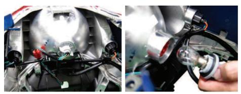
Remove the taillight socket with bulb from the tail light housing by turning it counterclockwise.
