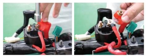
Remove the nuts that hold the starter motor lead and battery lead wires to the starter relay with a 10 mm socket.
