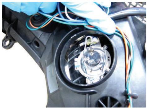
Fit the bulb into the lamp.
