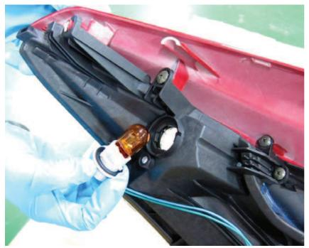
Turn the turn signal bulb socket counterclockwise and free it from the lamp.
