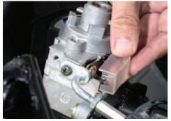
Install the seat latch cable cover.
