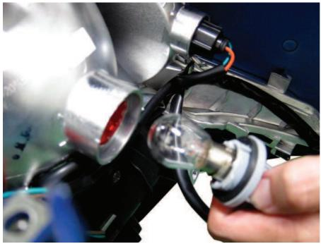
Install the taillight socket into the lamp and turn it clockwise to lock it into place.
