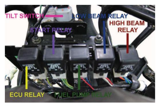
Remove and disconnect the high beam relay. The high beam relay is on the right.
