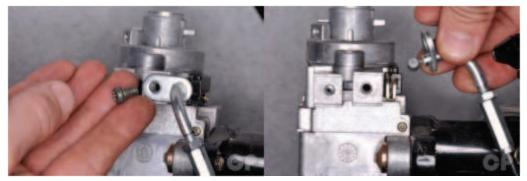
Remove the seat latch cable screw and free the seat latch cable from the ignition switch.
