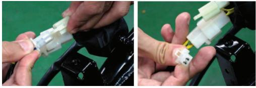
Disconnect the crank position sensor wire coupler. Measure the resistance between the Blue/White and green/white wire terminals.
