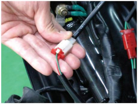
Unplug the two-pin luggage box light switch connector with green and green/red wires.
