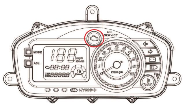
The check engine lamp (CELP) or Fi indicator is located in the center of meter.
