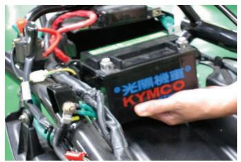
Fit the battery into the battery tray.
