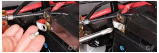
Connect the positive battery cable and install the bolt with a 10 mm socket or #3 Phillips screwdriver.
