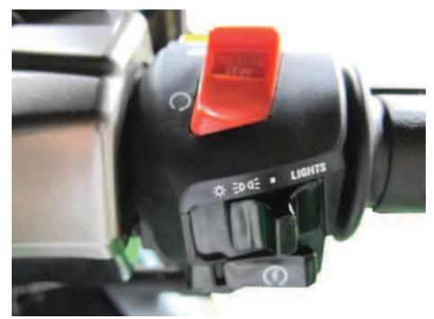
Use a digital multimeter to check for continuity to inspect the handlebar switches. Continuity should exist between the wires as indicated.
