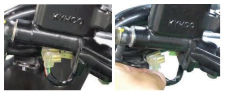
Unplug the brake light switch connectors.
