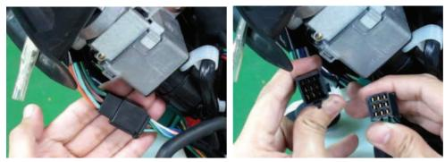
Unplug the black connector for the left handlebar switches.
