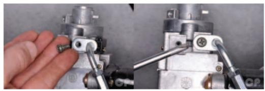
Install the seat latch cable screw and tighten it securely with a #2 Phillips screwdriver.
