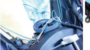
Slide back the rubber headlight covers. Remove the clip with a screwer.
