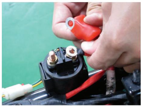
Remove the leads from the starter relay.
