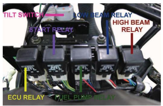
The ECU relay is located in the front under the dash panel, to the left of the start relay. Remove and disconnect the ECU relay. Disconnect the dash if needed. See the <u>Dash</u> topic for more information.
