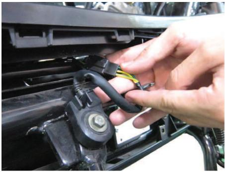
Unplug the three-pin side stand switch connector.
