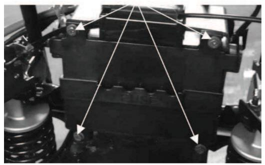
Remove the four battery cover screws. Remove the battery cover.
