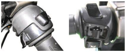
Use a digital multimeter to check for continuity to inspect the handlebar switches. Continuity should exist between the wires as indicated.
