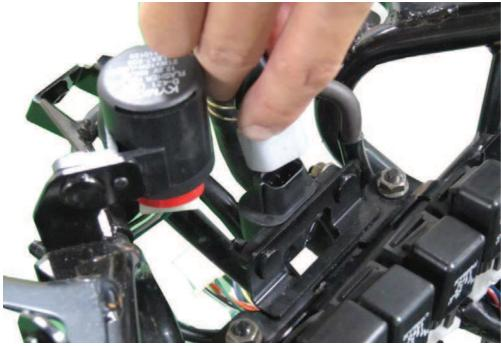
Disconnect the connector to remove the tilt switch.
