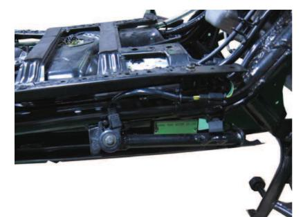
With the side stand retracted there should be continuity between the yellow/green wire and the green wire terminals.
