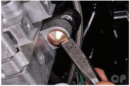
To remove the anti-tamper bolts use a punch and a hammer to strike the bolts so that they rotate loose. Turn the bolts clockwise to loosen them.
