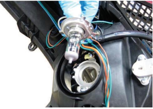
Remove the headlight bulbs from the lamp. Unplug the bulb from its connector. Do not touch the bulb with your bare hands if you plan to reuse it.
