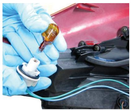
Push in on the bulb and rotate it clockwise to remove if from the socket. Insert the new bulb. Push down on the bulb and rotate it counterclockwise to lock it into place.
