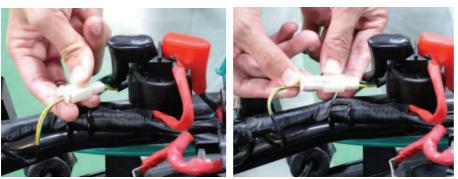
Disconnect the starter relay wire connector.
