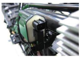
Remove the ignition coil leads.
