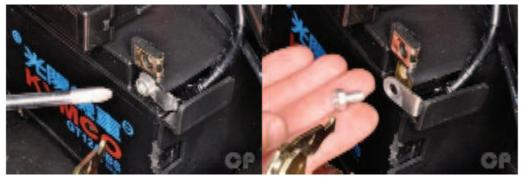
Remove the negative battery cable bolt with a 10 mm socket or #3 Phillips screwdriver. Free the negative cable from the battery.
