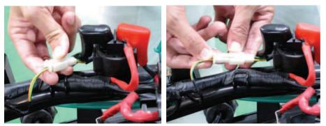
Disconnect the starter relay wire connector.
