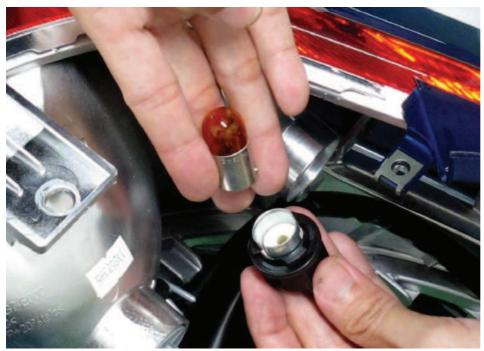
Push in the bulb and turn it counterclockwise. Remove the bulb. Insert the new bulb and turn it clockwise to lock it in place.
