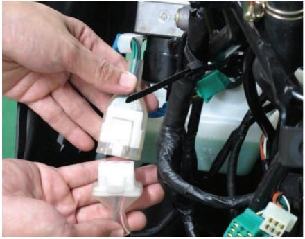
Unplug the white six-pin ignition switch connector.
