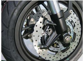
Remove the bolt of front axle.
