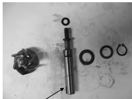
Water pump shaft
