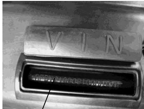
Location of Frame Serial Number (inside luggage box)
