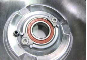
Remove the bearing snap ring with snap ring pliers. Remove the bearing with a suitable bearing puller.
