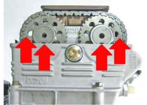
For correct engine timing the marks on the camshaft sprocket must be even with the cylinder head mating surface at the same time the "T" mark is lined up with the with the index notch in the timing inspection hole.
