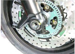
Apply a light coat of grease to the front axle when installation.
