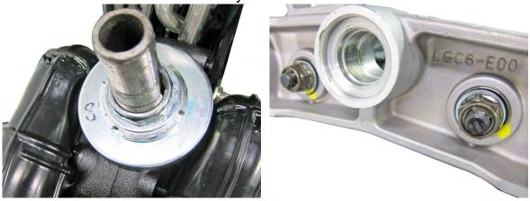
Remove the nuts and washer to separate the handle bar assembly. Installation torque: 3~4 kgf-m (30~40 N-m)
