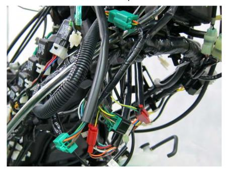
Unplug the black connector for the left handlebar switches.
