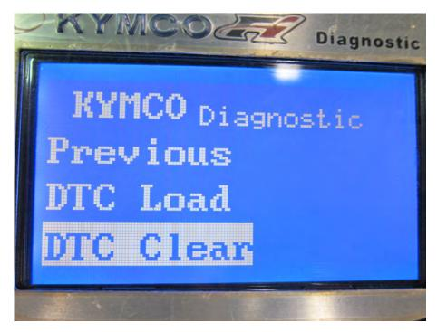
Move the selector down to the Clear DTC option and press enter.
