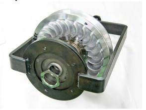
Loosen and remove the spring compressor tool. Remove the collar of spring.
