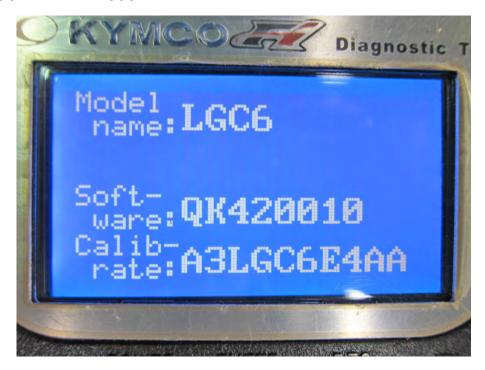
Pressing the enter button on the ECU version will show model name, ECU number, identifications number and software version.
