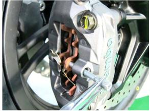
Remove the spring of the brake pad.
