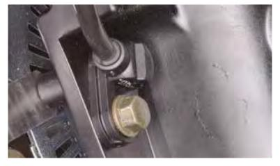
Check the speed sensor to rotor clearance with a feeler gauge and make sure that it is 0.3 - 1.2 mm (0.0012 - 0.048 in).
