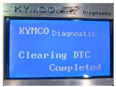
The diagnostic tool will show when the DTC in memory are cleared. Also, the DTC indicator light between the center and right buttons will be off.
