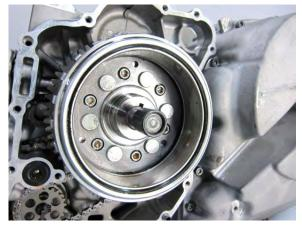
Use the special tool and remove the flywheel.
