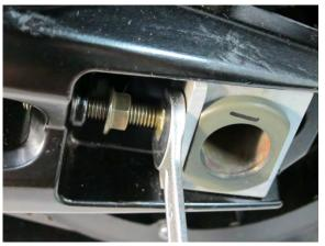
Remove two bolts and remove the chain up cover A. Remove two bolts and remove the chain low cover A.
