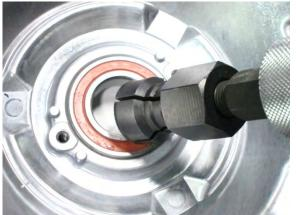
Drive in a new bearing with a suitable bearing driver that has the same outside diameter as the bearing.
