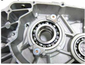
Remove the two bearing fixed plate.
