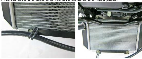
Remove the radiator from the frame.
