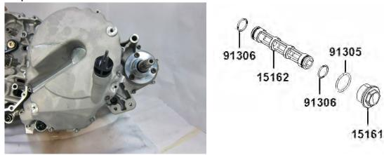
Remove the bolts and remove the mission cover. Installation torque: 1~1.4 kgf-m (9.8~13.7 N-m)
