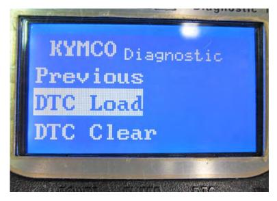
Press the down button to select the load DTC option. Press the enter button on the Load DTC item to display the DTC options.
