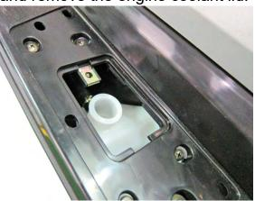
Open the coolant reserve tank lid. Siphon the coolant out of the reserve tank with an appropriate suction device. If a suction device is unavailable remove the reserve tank and poor it out.
