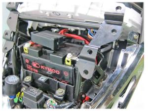
Remove the screws and remove the front cover set.
