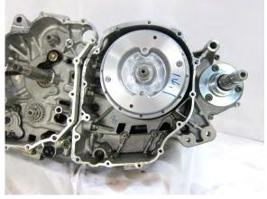
Remove the nut and remove the wet clutch. Installation torque: 5.9~7.3 kgf-m (58.5~71.5 N-m)
