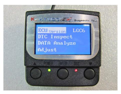
The four functions will display when the tool is powered on. The model name will show LGC6 for the AK 550.
