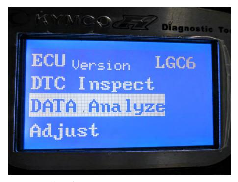
Press the down button (right) to move the item selector down to the DATA Analyze item. Press enter to bring up the DATA Analyze page 01 shown below. Press the down button to continue through the seven DATA Analyze pages.
