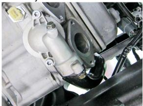
Loosen the coolant hose clamps with a #2 Phillips screwdriver.
