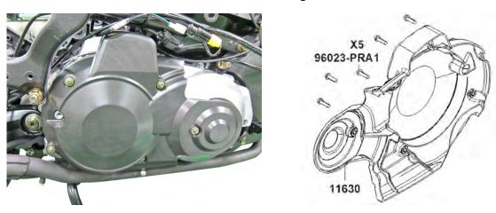
Remove two bolts and remove the CVT cover element.
