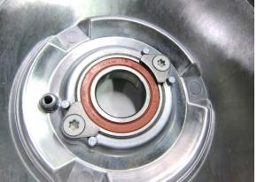
Remove the bearing snap ring with snap ring pliers.
