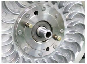
Remove the belt from the driven pulley.
