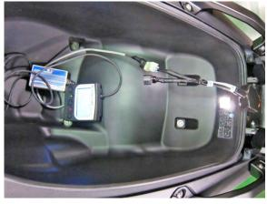
OBD diagnostics connecter (part number:36205-LGC6-E00) and can linker .
