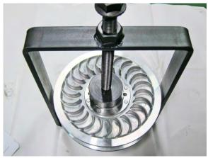
Tighten the bolt of the fitting tool to compress the spring.
