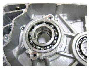
Remove the bearing by bearing puller tool.
