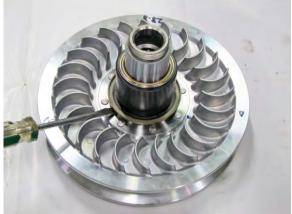
Remove the six guide rollers with guide roller pins.
