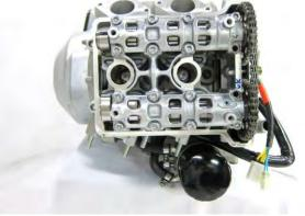
Loosen and remove the camshaft holder bolts in a crisscross pattern in several steps, then remove the camshaft holder. And remove camshafts.
