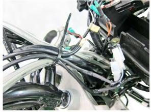
Disconnect the connecters and couplers of the switches.
