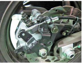
Remove the screws of handle bar switch, parking brake wire and remove the parking brake set.
