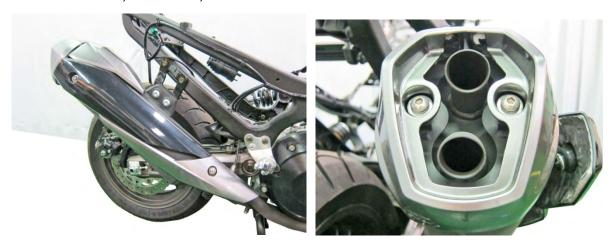
Remove bolts, washers, rubbers and remove the heat shields.
