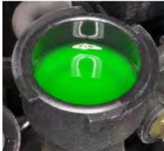
When the air bubbles stop coming up turn off the engine and recheck the coolant level, add coolant if necessary. Check the reserve tank and add coolant if needed. Wet the seal of the radiator cap and install.
