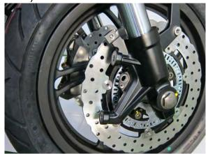
Remove the bolt of front axle.
