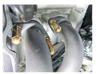
Remove the exhaust pipe.
