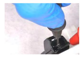
Using a digital multi meter set to ohms of resistance ( $\Omega$ ), measure the resistance between the fuel pump/level gauge connector terminals (green and yellow/white) with the float raised to the positions indicted below.
