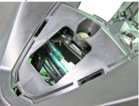
Remove the bolts, screws and remove the handle bar heater connecters. Remove throttle and brake wire and remove the low handle cover.
