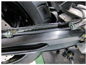
Remove the bolt of rear fixed plate.
