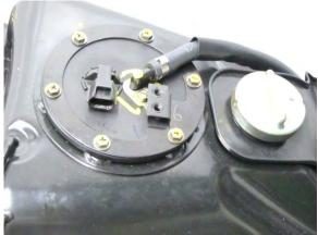
Clamp the fuel hose for safety. And loosen the fuel hose clamp.
