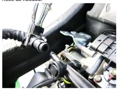
Remove the two fuel injector mounting bolt with a socket.
