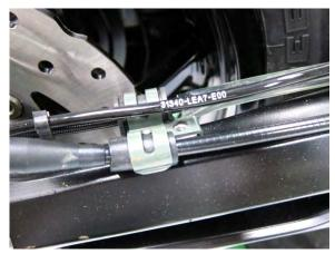
Remove the bolt of front fixed plate.
