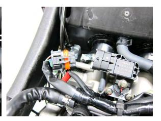
Measure if the ECU voltage outputs to the MAP between the following terminals of the MAP connector.
