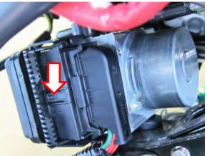
Press the craw to release the coupler of ABS module.
