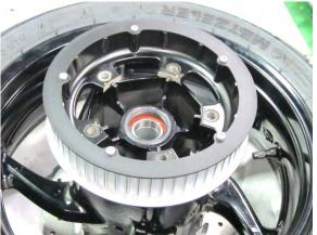
Remove the driven belt sprocket.
