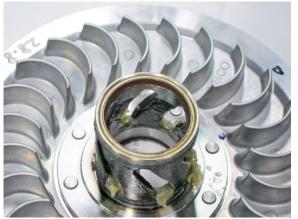
Replace the O-rings of the driven pulley.
