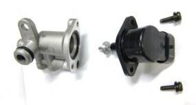
When installation, apply oil onto a new O-ring. And being careful not to damage the O-ring.
