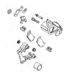
Loosen and remove the two bolts of rear caliper. The bolts are with blue Loctite (non-permanent) to the threads. Using this type of bolts when installation. Installation torque: 3~4 kgf-m (30~40 N-m)
