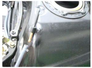
Remove the fuel tank mounting nuts.
