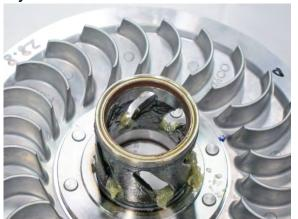
Replace the O-rings of the driven pulley.
