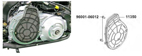
Remove the bolts, nut and remove the CVT cover.
