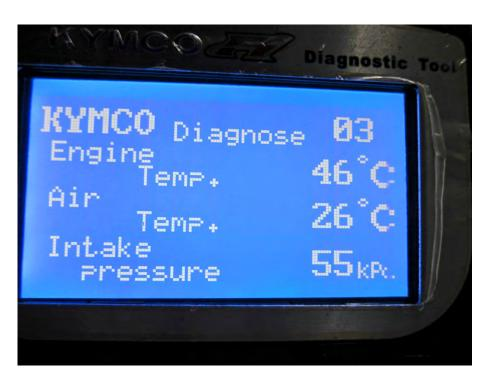
The 03 page shows engine temperature, air temperature, and intake pressure.
