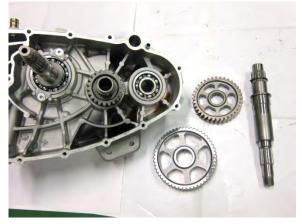
Remove the counter B gear and remove the counter gear.
