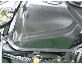
Remove the fuel tank mounting nuts and remove the fuel tank from the frame.
