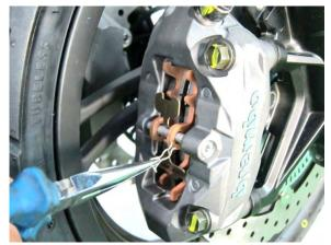
Remove the screw, loosen the brake pad.
