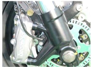
Remove the bolt of state of front fender.
