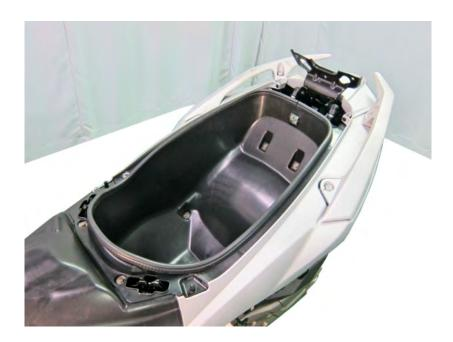
Remove 6 bolts, lift up the luggage box. See the external topic for the details. Remove the luggage box switches connectors. Remove the luggage box and switches.
