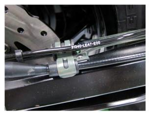
Remove the bolt of front fixed plate.
