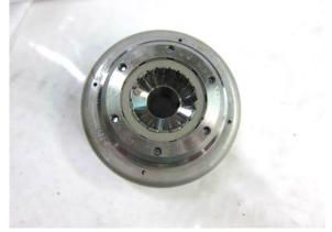
Remove the starting clutch gear.
