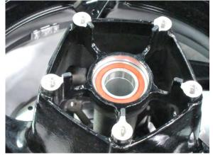
Replace the bearings if the races do not turn smoothly, quietly, or if they fit loosely in the hub.
