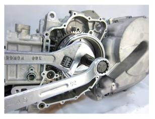
Inspect the one way bearing, replace if necessary.
