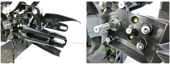
Remove the two bolts and nuts of left rear fork. And Slide out and remove the left rear fork.
