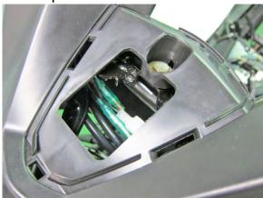
Remove the bolts, screws.
