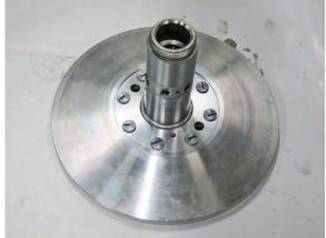
Replace the seals from the driven pulley.
