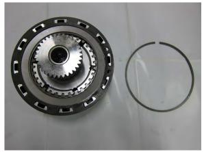
Remove the retainer and spring.
