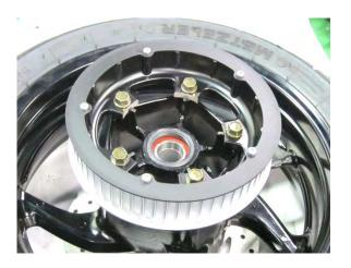
Remove the five bolts of the driven belt sprocket. Installation torque: 3~4 kgf-m (30~40 N-m)
