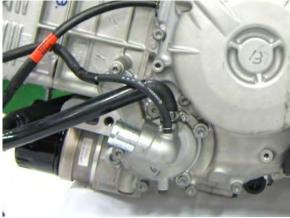
Remove the other coolant hose and tube. And remove the bolts of coolant pump cover.
