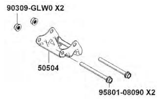
Remove the bolt, nut and upper plate.
