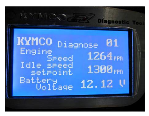
The 01 page shows engine speed, idle speed set point, and battery voltage.
