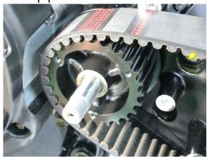
The bolts are all with blue Loctite (non-permanent) to the threads. Using this type of bolts when installation.
