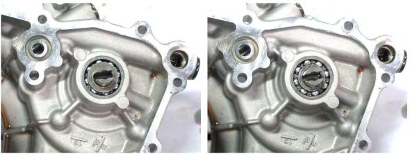
Remove the water pump shaft and impeller
