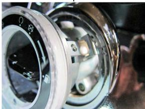
Remove bolts, screws, couplers and remove the leg shield assembly.
