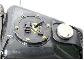
Note: When slide back the fuel hose carefully not to damage the fuel pump pipe, and replace the clamp with a new one when installation.
