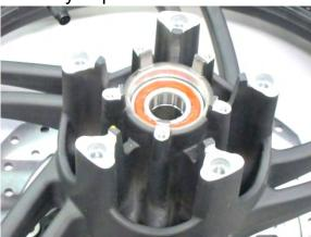
Remove the dust seal from the right side of the front wheel using a seal pick or large flat blade screwdriver. Discard the dust seal, it should be replaced by a new item.
