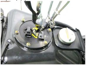
Clean up any remaining fuel immediately. Disconnect the fuel hose from the fuel injector. Connect the fuel pressure gauge. Remove the fuel hose clamp. Turn the key to the ON position. Check the fuel pressure.
