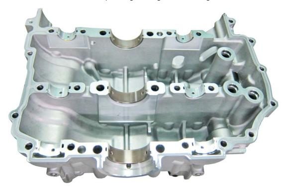
And set the upper crank case half down on top of the lower case.
