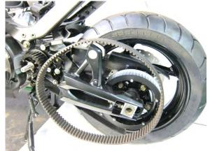
Remove the drive sprocket.
