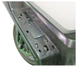
Remove the engine coolant lid screw, and remove the engine coolant lid.
