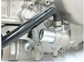
Remove the water pump cover bolts. Remove the water pump cover.
