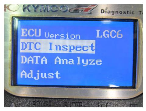
Press the down button (right) to move the item selector down to the DTC Inspect item.
