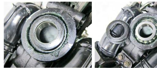
Remove the collar and remove the upper ball bearing.
