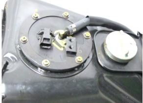
Touch the multi meter leads to the harness side of the fuel pump connector, with the positive lead touching the red/black wire terminal and the negative lead touching the green wire terminal.
