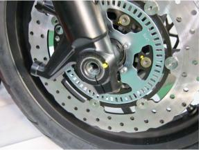
Loosen the front axle pinch bolt with a 6 mm Allen. Installation torque: 2~2.6 kgf-m (20~26 N-m)
