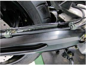
Remove the bolt of rear fixed plate.
