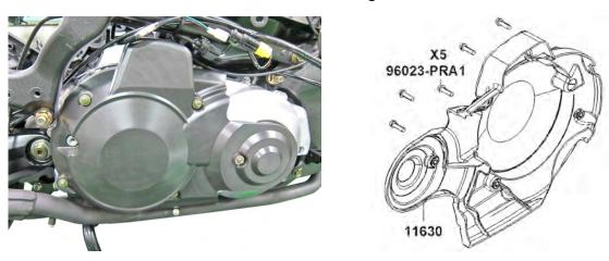
Remove two bolts and remove the CVT cover element. Clean the cover element if necessary.
