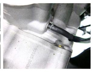
Loosen the two bolts of thermostat cover.
