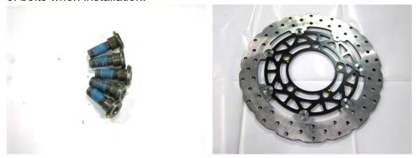
When installation, follow the order below, first time tighten the bolts with torque: 1.5 kgf-m (15 N-m)
