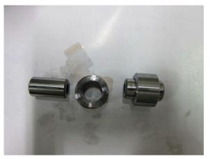
Remove the left side three nuts and right side two nuts. Remove the mission case set.
