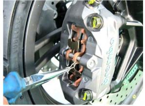
Remove the screw, loosen the brake pad.
