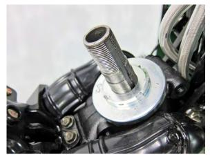
A special race nut wrench is needed to loosen the steering stem lock nut. Special Tool - race Nut Wrench: F00023.
