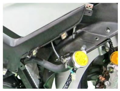
Remove the radiator cap in two stages. Allow any built up pressure to vent and then open the cap all the way and remove it.
