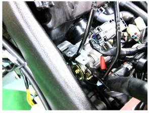
Free the throttle cables from the throttle drum.
