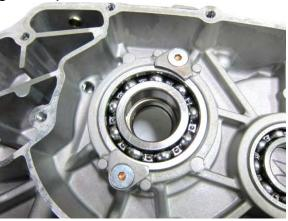
Remove the two bearing fixed plate.
