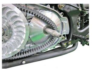
**Drive Pulley Disassembly**
