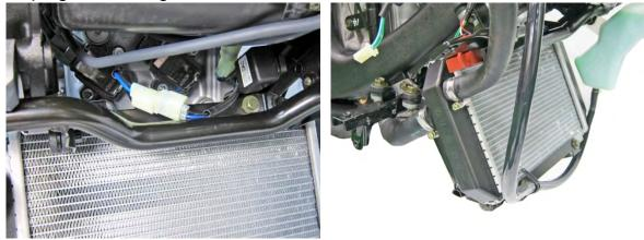
There are three coolant hoses that connect to the radiator. The top left hose runs to the filler neck and cap. The top back of left hose runs to the thermostat on the cylinder head. The bottom right hose runs to the water pump.
