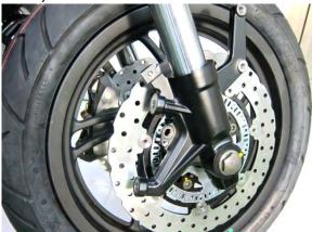
Remove the two caliper mounting bolts with a 12 mm socket. And remove the front caliper.
