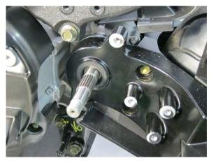
Slide out and remove the rear wheel axle.
