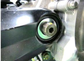
Loosen the rear swing axle bolt.
