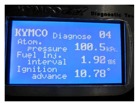
The 04 page shows atmospheric pressure, fuel injection interval, and ignition advance.
