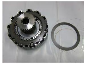
Remove the retainer and brake shoes set.
