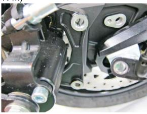
Remove the hex bolt, and separate the caliper.
