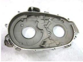
Remove the gaskets of CVT case.
