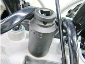
Remove the washer of bottom bridge.
