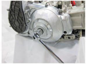
Rotate the crankshaft to TDC mark.
