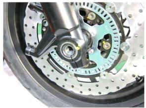
When installation: Apply grease to the lips of the dust seals and collar O-rings. Insert the collars into the hub.
