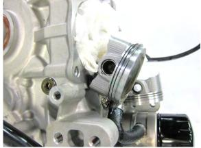
Remove the piston pin and the piston.
