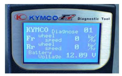
When using the DATA Analyze feature of the diagnostic tool with the ABS system the front and rear wheel speed sensors should show speed when the wheels are rotated.
