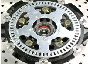
Remove the bolts of brake disk.
