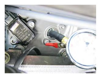
Thread a compression tester into the spark plug hole hand tight. Hold the throttle all the way open. Crank the engine with the starter motor until the needle on the gauge stops rising. Do not crank the engine more than a few seconds.
