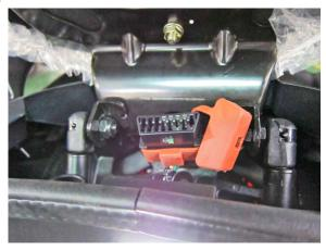
Use the Sub cord, OBD diagnostics connecter (part number:36205-LGC6-E00) and can linker to connect between vehicle and diagnostic tool.
