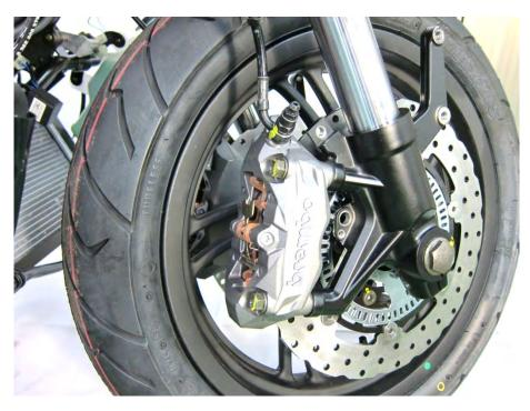
Remove the snap clip of the pin.
