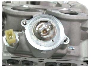
Lift out and remove the thermostat.
