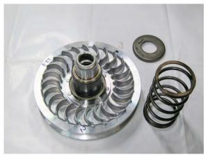
Measure the free length of the clutch spring. Replace the spring if needed.
