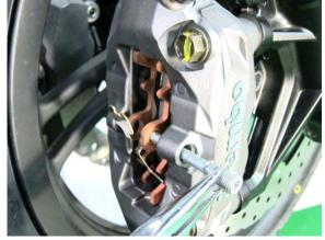
Remove the spring of the brake pad.
