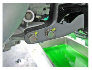
Carefully move the front frame forward and separate it from the engine. Installation torque: 1~1.4 kgf-m (9.8~13.7 N-m)
