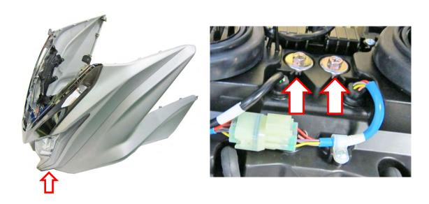
Turn the screws to adjust the right and left head lights aim as needed.
