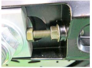
Loosen and remove the rear wheel axle nut, move wheel forward to loosen the belt. Installation torque: 12~14 kgf-m (120~140 N-m)
