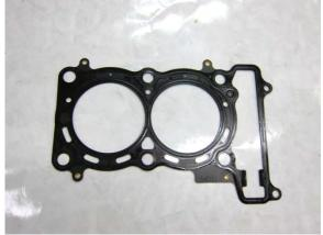
Remove the cylinder, gasket and dowel pins. Replace a new gasket when installation.
