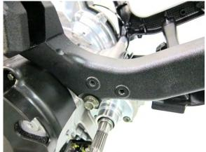
Remove the bolts and nuts and remove the rear frame body. Installation torque: 8.6~9.1 kgf-m (86~91 N-m)
