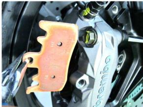
Remove the two bolts of caliper and remove the caliper.
