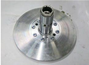
Replace the seals from the driven pulley.
