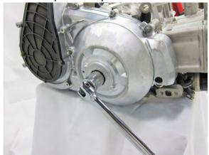
Rotate the crankshaft to TDC mark.
