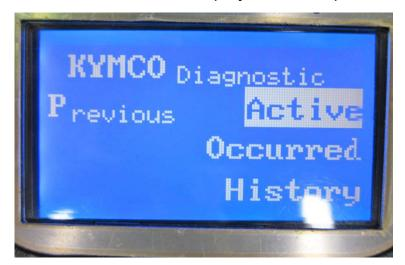
Move the selector to the Current option and press enter to display current DTC.
