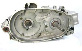
Remove the five bolts of the CVT case. Installation torque: 1.8~2.2 kgf-m (17.7~21.6 N-m)
