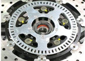
Remove the bolts of brake disk.
