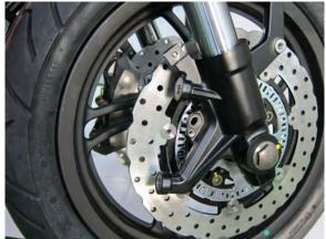
Remove the bolt of front axle.
