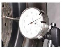
Check if the brake rotor runout is within the service limit.
