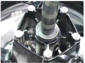
Heat the bearing area of the wheel with a heat gun, take the bearing out of the freezer and install it. You can use a bearing installer tool or a socket with the same outside diameter as the bearing. Make sure the bearing is fully seated and the marked side is facing out.
