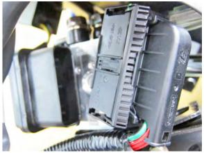
Disconnect the ABS hydraulic unit connector.
