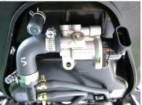
Remove the ISC screw with a #2 Phillips.
