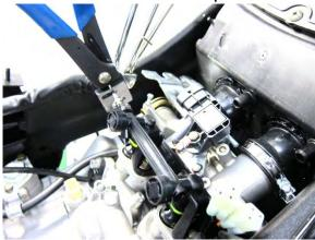
To separate the fuel hose from the fuel pump pipe.
