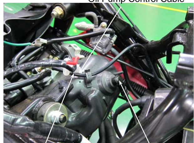
Oil Pump Control Cable
