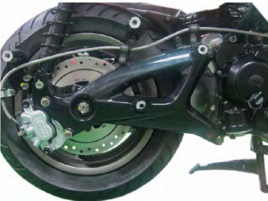
Fit the rear fork into place.
