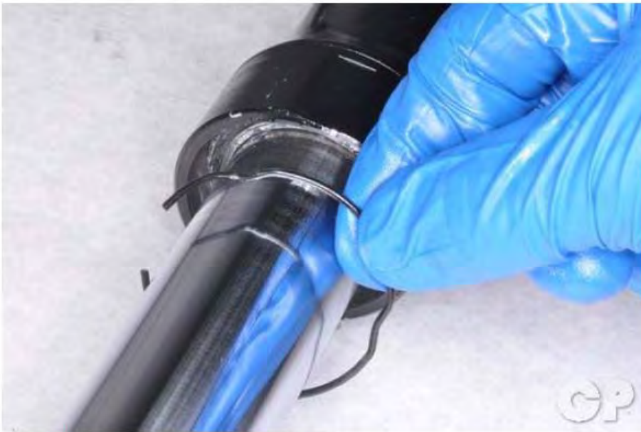
Insert the stopper ring into its groove.
