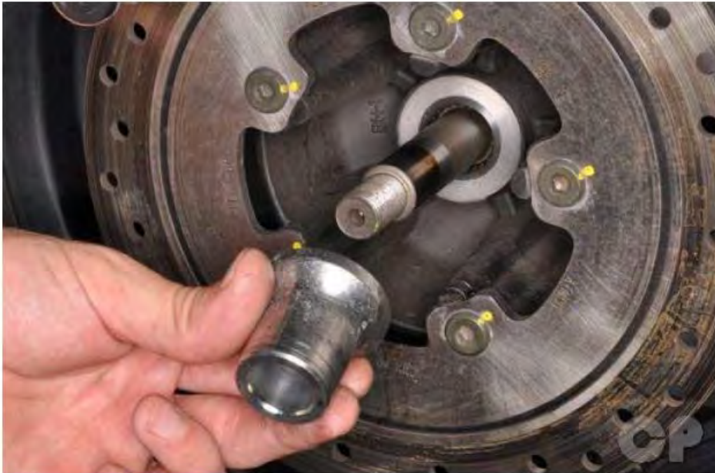
Slide on the rear axle collar.
