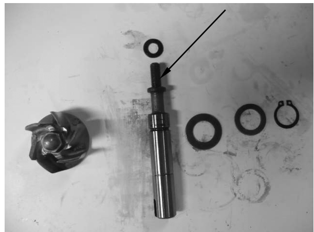
Water Pump Shaft
