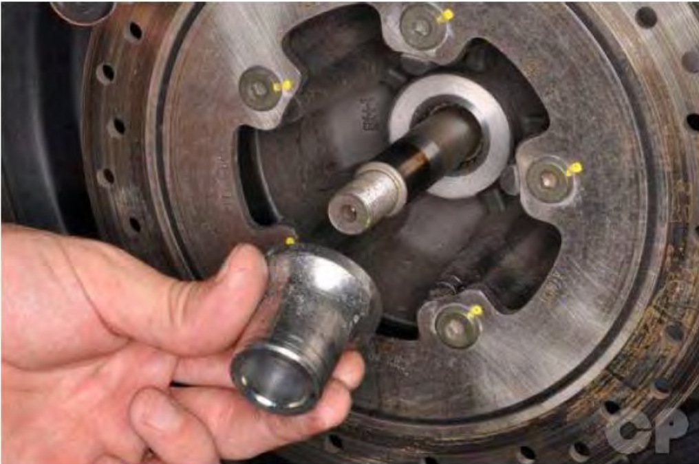
Slide on the rear axle collar.
