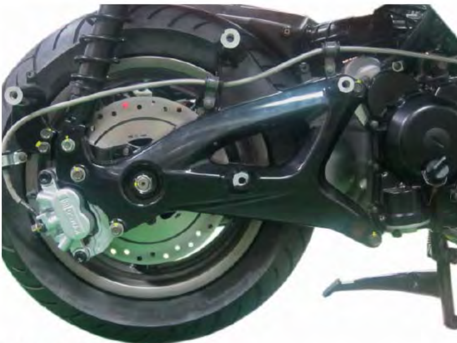
Fit the rear fork into place.
