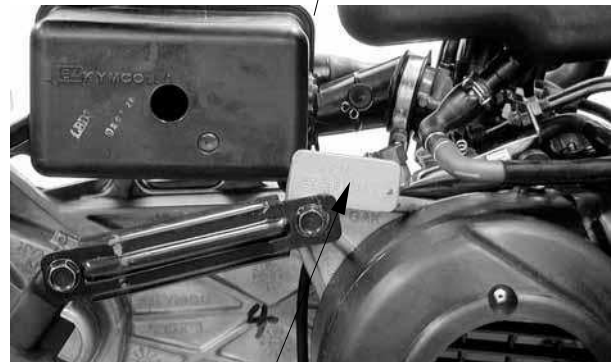
Location of Engine Serial Number
