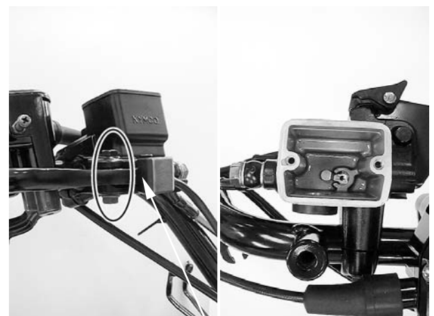
Apply grease to the dust boot
