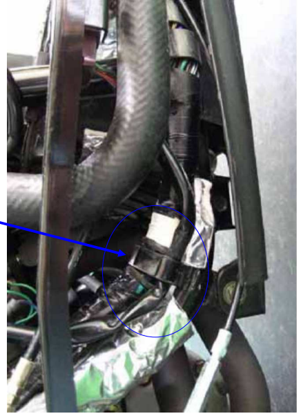
Fix the hazard controller wire by soft hook.
