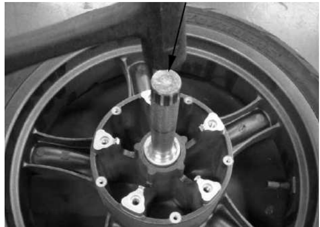
Bearing install driver
