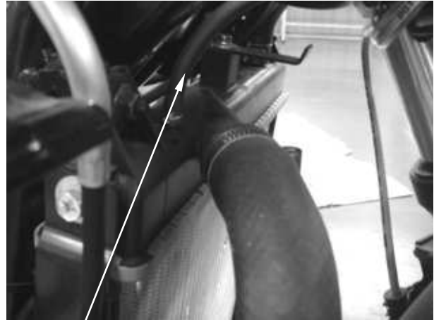
Air Bleed Hose
