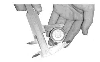
Check each caliper cylinder for scratches or wear and measure the cylinder bore.
