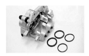
Check the piston for scratches or wear.
