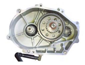
Install the final gear onto the final shaft as shown.
