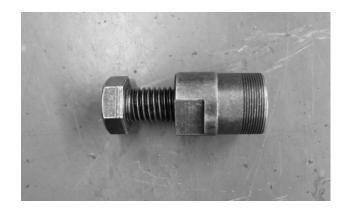
Apply grease to the threads of the flywheel puller tool before using it. Thread the puller onto the flywheel. Hold the tool with a large wrench an turn in the bolt until the pressure separate the flywheel from the crankshaft.
