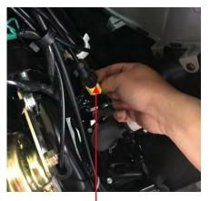
Front Wheel speed Sensor's connector
