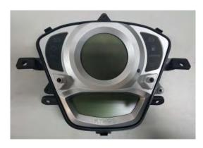
Install 4 fixing screws in diagonal sequence
