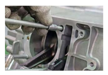
Install a new base gasket onto the crankcase.
