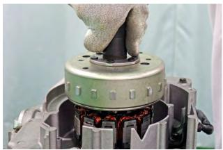
Remove the flywheel from the crankshaft.
