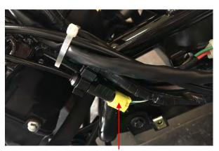
Rear Wheel speed Sensor's connector
