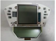
Remove 4 fixing screws of Noodoe in sequence as shown .
