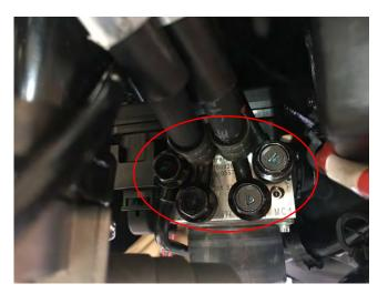
₩ When replacing a new Hydraulic Unit, don't need to drain the brake fluid.
