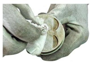
Also clean out the ring grooves. You can use an old ring to scrape.
