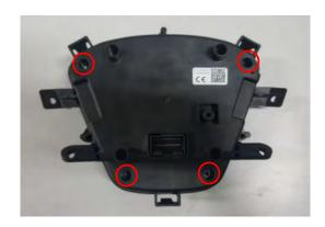
Push the Noodoe upwards to separate the lower cover and Noodoe.
