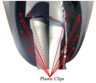
Remove 2 plastic fasteners beneath the wind cowl.
