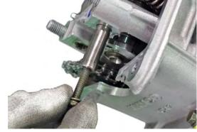
Lift the rocker arms as the shafts are removed.
