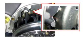
Apply a small amount of Loctite to threads of the camshaft sprocker bolts. Thread in the bolts and tighten to specification.
