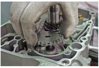
Remove the oil pump shaft.
