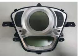
Remove the 4 screws attaching the lower meter cover.
