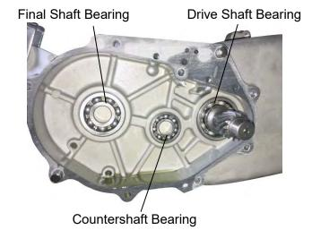
Check the transmission case cover bearings for excessive play and inspect the final shaft bearing oil seal for wear or damage.
