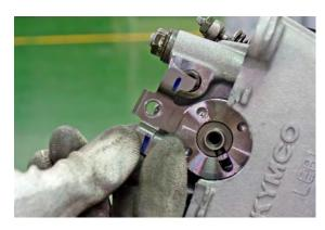
Remove the 4 camshaft holder nuts with a 14mm socket.
