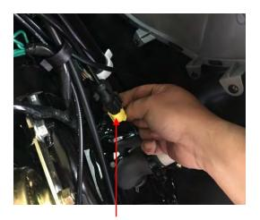
Front Wheel speed Sensor's connector
