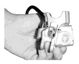
Measure the brake master cylinder piston O.D.
