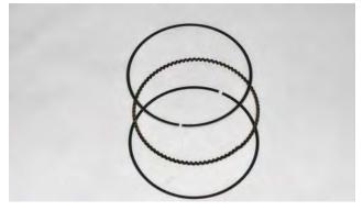
The "IN" mark should face the intake side of the engine.
