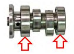
Inspect the rocker arm shaft outer diameter for the intake and exhaust valves.
