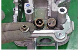
Remove the valve springs.
