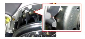
Lubricate the camshaft lobes and bearings with fresh engine oil.
