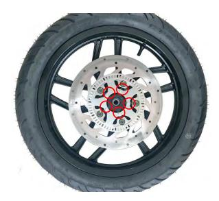
Remove the 5 bolts to remove the break disk.
