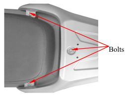
Remove the 2 clips and remove the rear central body cover
