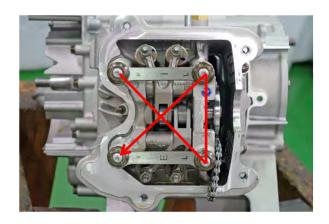
Install the set plate so it fit into the groove on the camshaft and between the projections on the rocker arm shafts.
