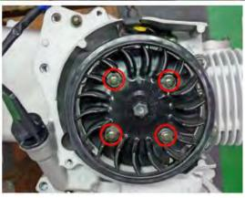
Remove the 17mm nut and washer.
