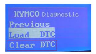
2. Clearing DTC completed until the DTC red lamp is off.
