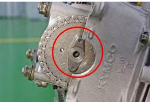
Remove the camshaft sprocket as shown, Support the chain so it does not fall into the cylinder head.
