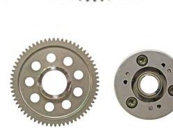
Fit the boss of the starter driven gear into the starter clutch. The Starter clutch should only allow the driven gear to turn in on direction. It the starter clutch allows turning both ways or will not let the driven gear rotate smoothly in one direction, the starter clutch must be replaced.
