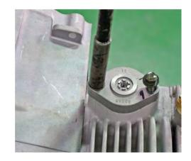
Rotate the crankshaft 360° clockwise and check the engine timing one more time.
