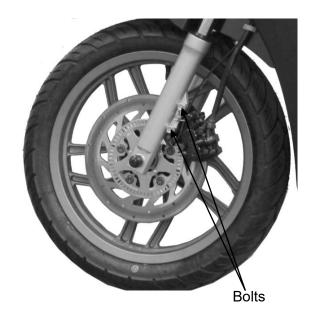
Remove the 5 bolts to remove speed rotator plate.
