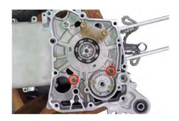
Lift the crankshaft out of the left crankcase half. Remove the cam chain from the crankshaft and crankcase. Inspect the cam chain for wear and damage. Replace the cam chain if needed.
