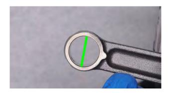
Measure the ring groove width and the ring-to-groove clearance with feeler gauge.
