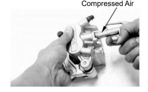
Push the piston oil seal outward to remove it. Clean the oil seal groove with brake fluid.
