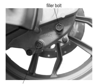
fluid drain bolt
