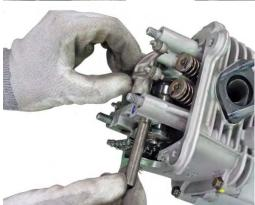
Remove the camshaft from the cylinder head.
