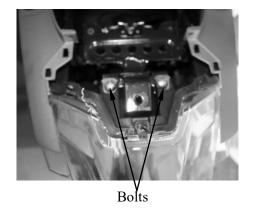
Remove 2 bolts attaching the rear fender.
