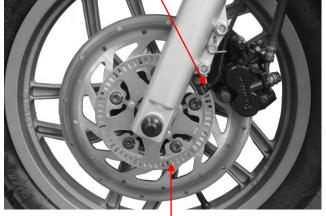
Front Wheel Speed Sensor Rotor
