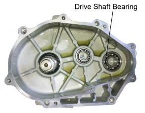
Check the transmission cover bearings for excessive play. Inspect the drive shaft, drive shaft bearing and oil seal for wear or damage.
