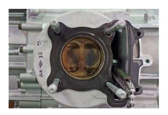
Remove the cylinder head gasket.
