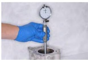
Inspect the cylinder front to back and side to side at three different height levels with a dial bore gauge. Replace the cylinder and piston as a set if the cylinder is out of specification.
