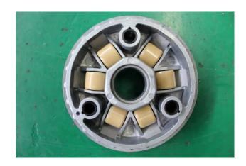
Check the drive pulley collar for wear or damage. Measure the O.D. of the drive pulley collar sliding surface.
