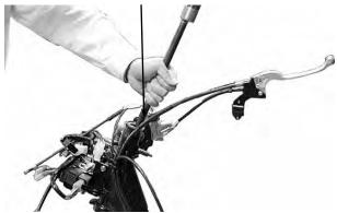
Drive new top and bottom ball races into the steering head using the outer driver.
