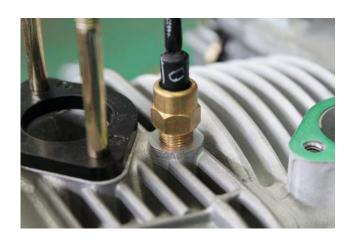
remove the engine temperature sensor if needed.
