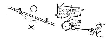
■ Protect wires and harnesses with electrical tape or tube if they contact a sharp edge or corner.
