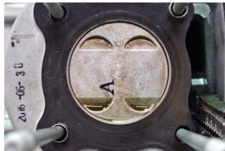
Place the piston over the connecting rod. Insert the piston pin into the piston and rod.
