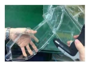
Assemble the upper cover of meter, tighten 3 screws
