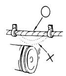
■ When fixing the wire harnesses, do not make it contact the parts, which will generate high heat.
