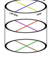
Measure the outer diameter of the piston at 8mm up from the bottom of the skirt at a
