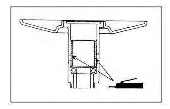
Press a new needle bearing into the driven face.
