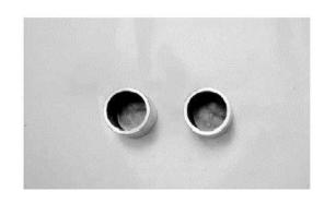
Check the caliper cylinder for scratches or wear and measure the cylinder bore.
