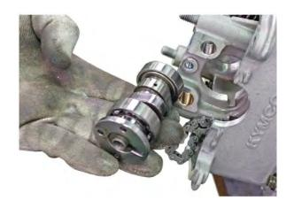
Lubricate the inside diameters of the rocker arms and the roller with fresh engine oil. Wipe the rocker arm shafts clean. Insert the rocker arm shafts into the camshaft holders and rocker arms.
