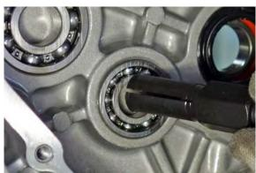
Use a bearing puller to remove the crankcase or transmission cover.
