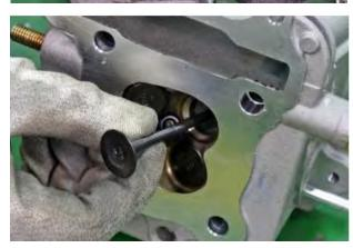
Remove the valve seal from the valve guide. The valve seal should be replaced if they are removed or you need to install new valves.
