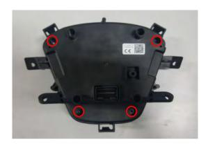
Install the Mode button lever and ADJ button lever
