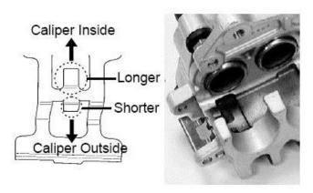
Install two brake pads and brake pad dowe pin.l
