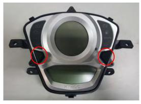
clean the meter and cover with Electrostatic dust gun
