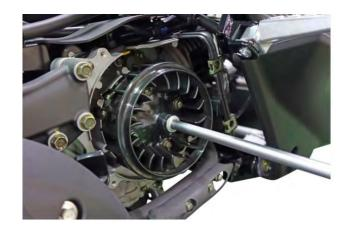
Position the pistion at top dead center as right The "T"mark should align with the index notch in the timing inspection hole. Support the chain if the crank must be turned to the correct position.
