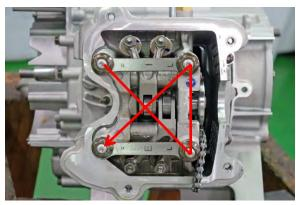
Remove the 2 camshaft holders.
