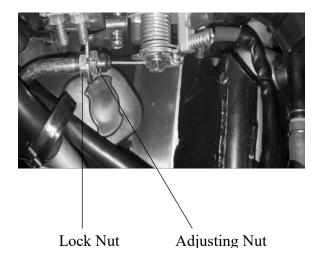
Minor adjustment is made with the adjusting nut at the throttle grip side.
