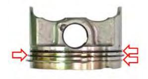
Install the top and second rings with their makings facing up.Install the rings to the piston as shown above so that no ring end gaps line up with the piston pin or perpendicular to the piston pin.The rings should turn easily on the piston without sticking or roughness.
