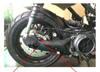
Rear Wheel Speed Sensor Rotor Rear Wheel Speed Sensor
