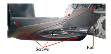
Remove the 4 bolts from the floor board. Remove the floor board.
