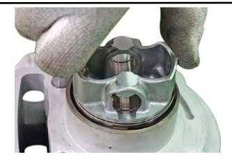
Measure the ring gap with a feeler gauge. Repeat this procedure with second ring and the oil side Rails.
