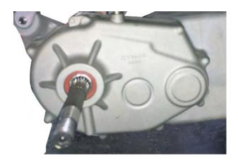
Install the transmission case cover. Tighten the 9 bolts.
