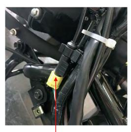
Rear Wheel speed Sensor's connector
