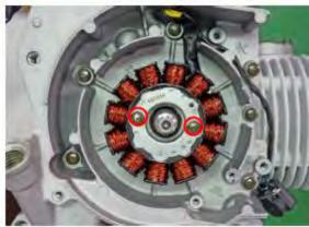
Remove the 3 stator mounting bolts and the 2 crank position sensor bolts with an 8mm socket Remove the stator and the crank position sensor together.
