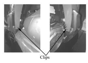
Remove 2 big clips from inside attaching the frame body cover.
