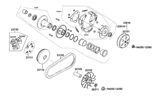
Install the weight rollers into the movable drive face.
