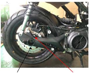
Rear Wheel speed Sensor Rotor Rear Wheel speed Sensor
