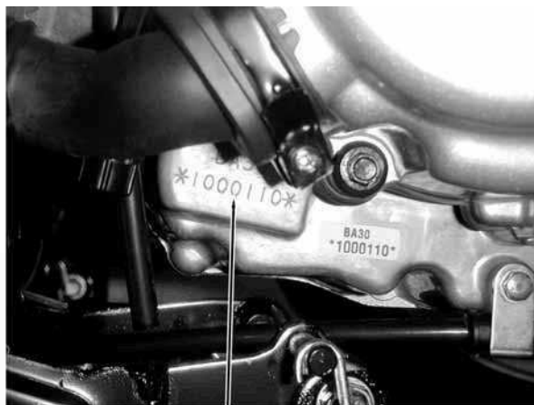
Location of Engine Serial Number
