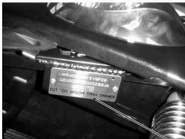
Vehicle Identification Serial Number
