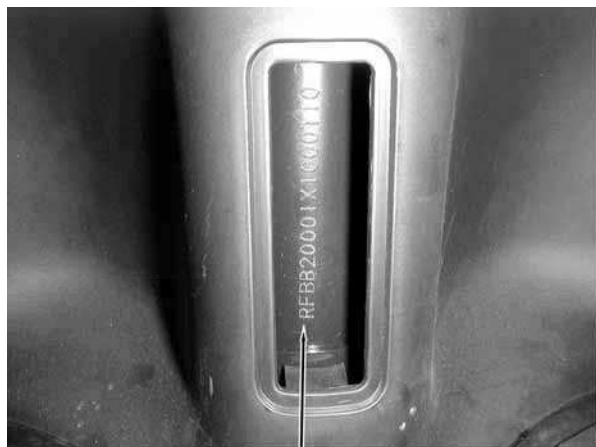
Location of Frame Serial Number
