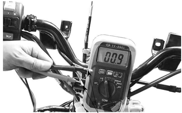
Stop Switch Wire
