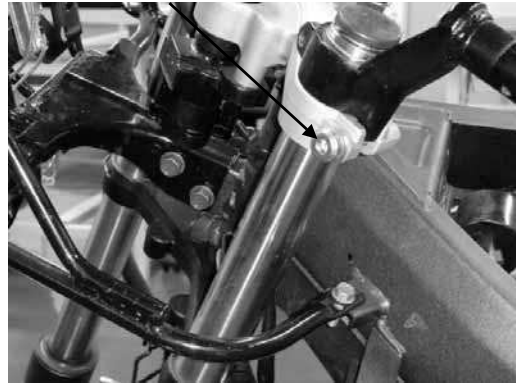
Upper Fork Bridge Bolts
