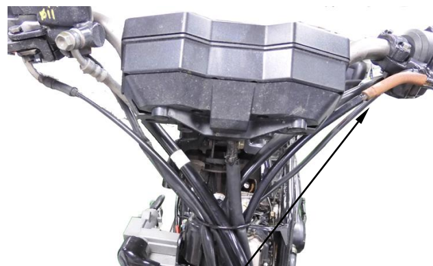
Stop Switch Wire
