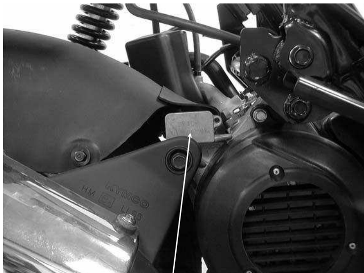
Location of Engine Serial Number
