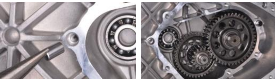
Install the dowel pins. Install a new gasket onto the transmission case.
