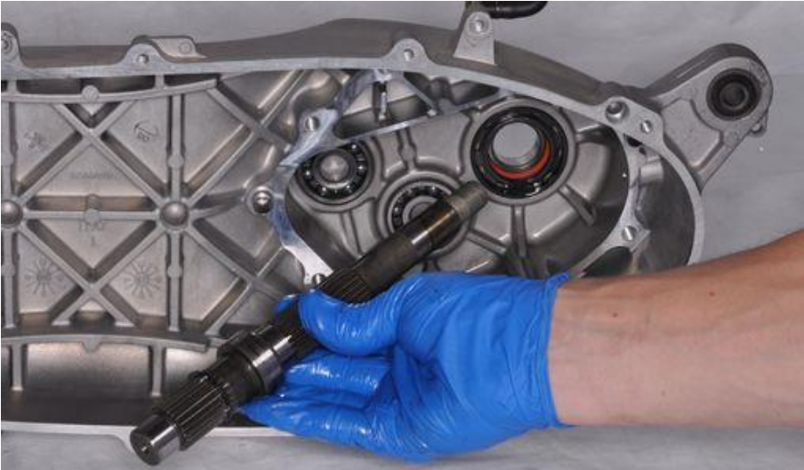
Insert the final shaft through the oil seal and bearing.
