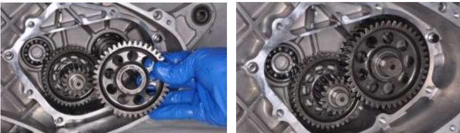
Install the final gear onto the final shaft as shown.
