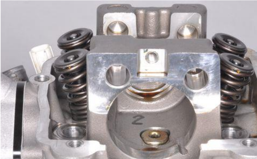
Inspect the camshaft bearing journals for scoring or scratches.
