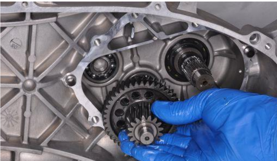
Install the countershaft into its bearing as shown.
