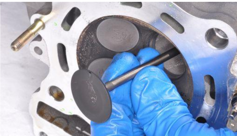
Push the valve stem down and remove the valve from the combustion chamber side of the cylinder head. Rotate the valve as it is removed.
