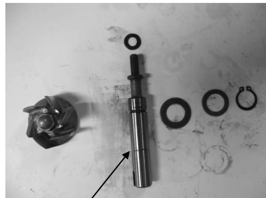
Water pump shaft
