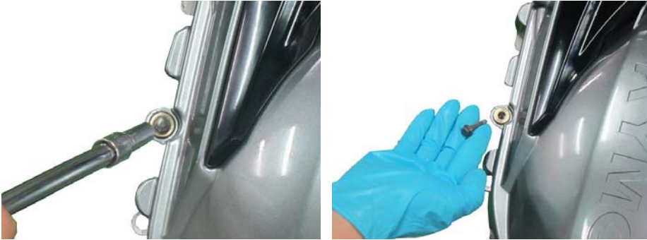
Remove the six bolts mounting the left crankcase cover protector.
