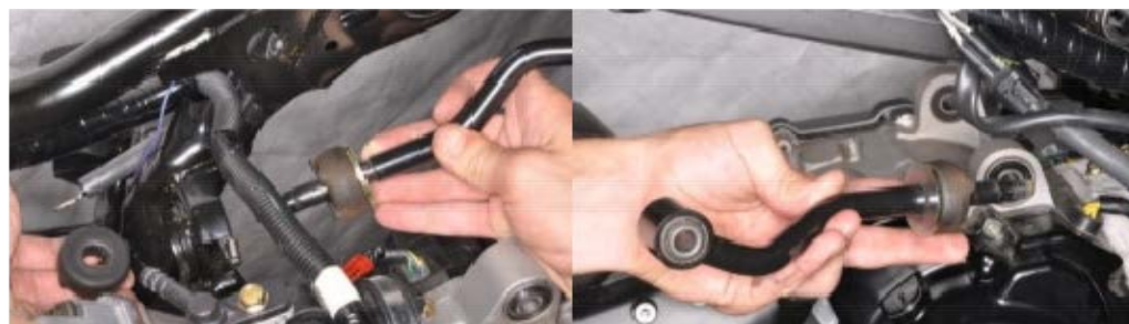
Remove the engine mounting bracket damper assembly.
