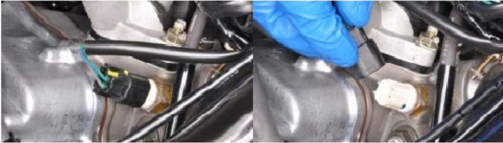
Unplug the water temperature sensor.
