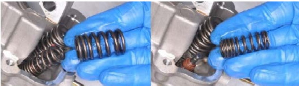
Remove the valve springs.
