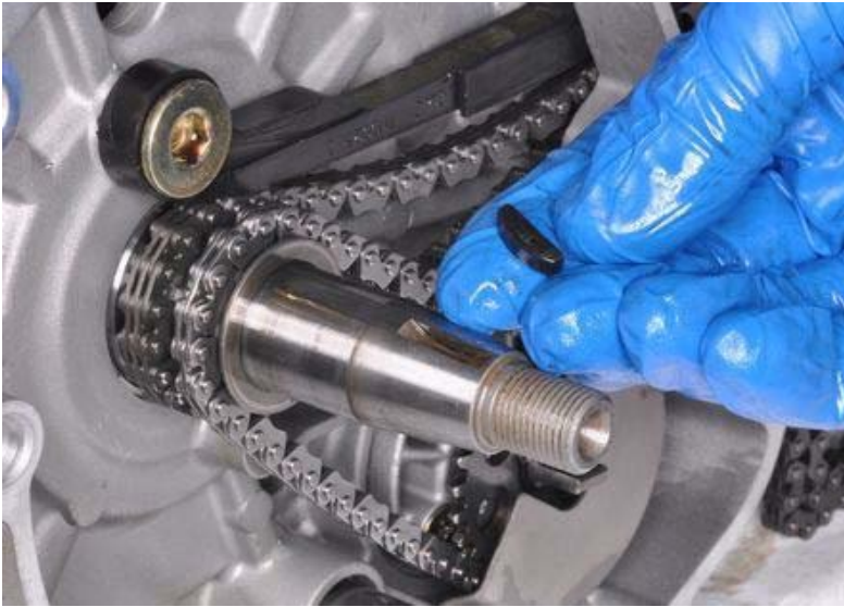
Remove the woodruff key from the crankshaft.
