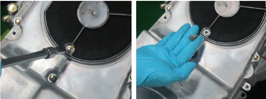
Remove the two bolts mounting the element duct left crankcase cover.
