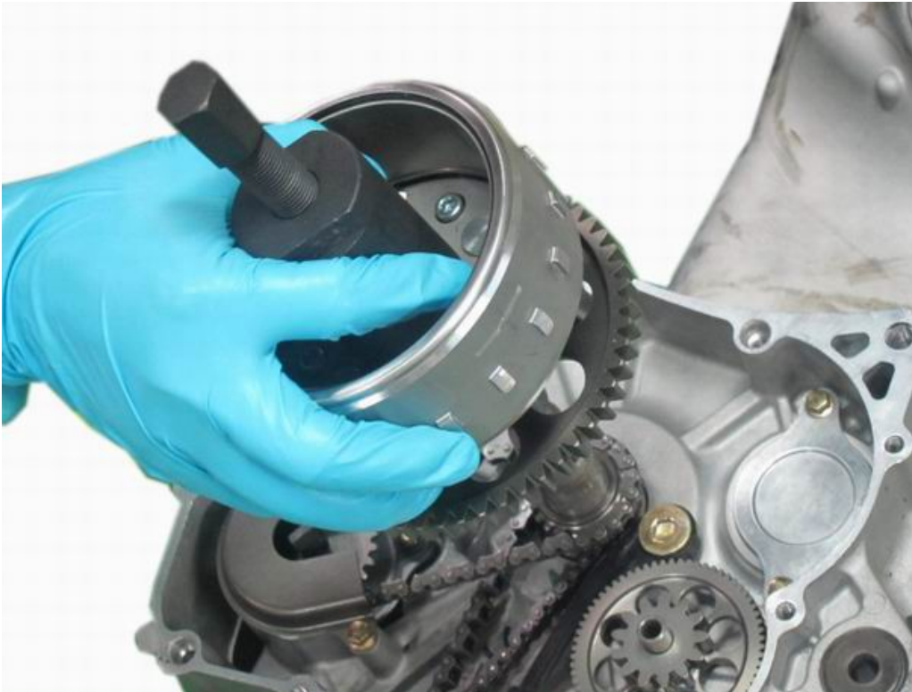
Remove the flywheel from the crankshaft.
