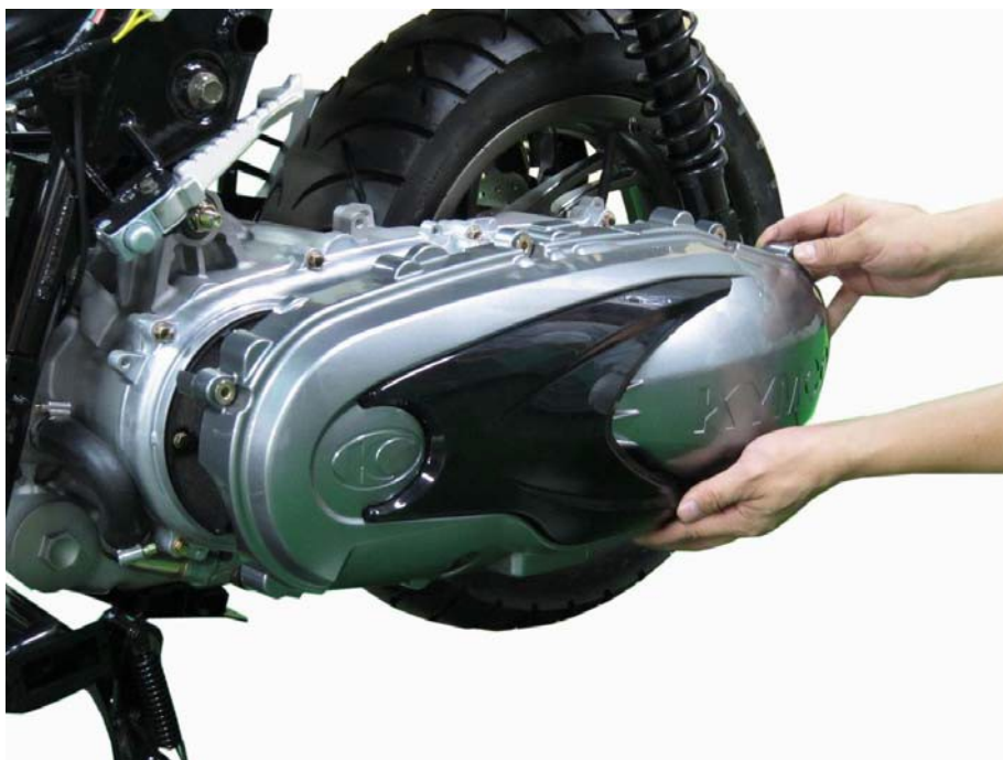
Install the belt case plastic cover.
