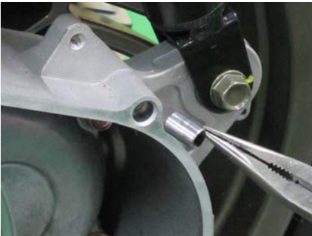
Remove the two dowel pins.
