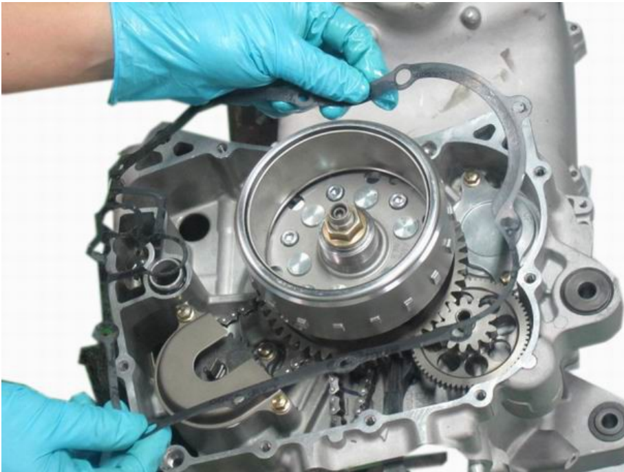
Remove the generator cover gasket.
