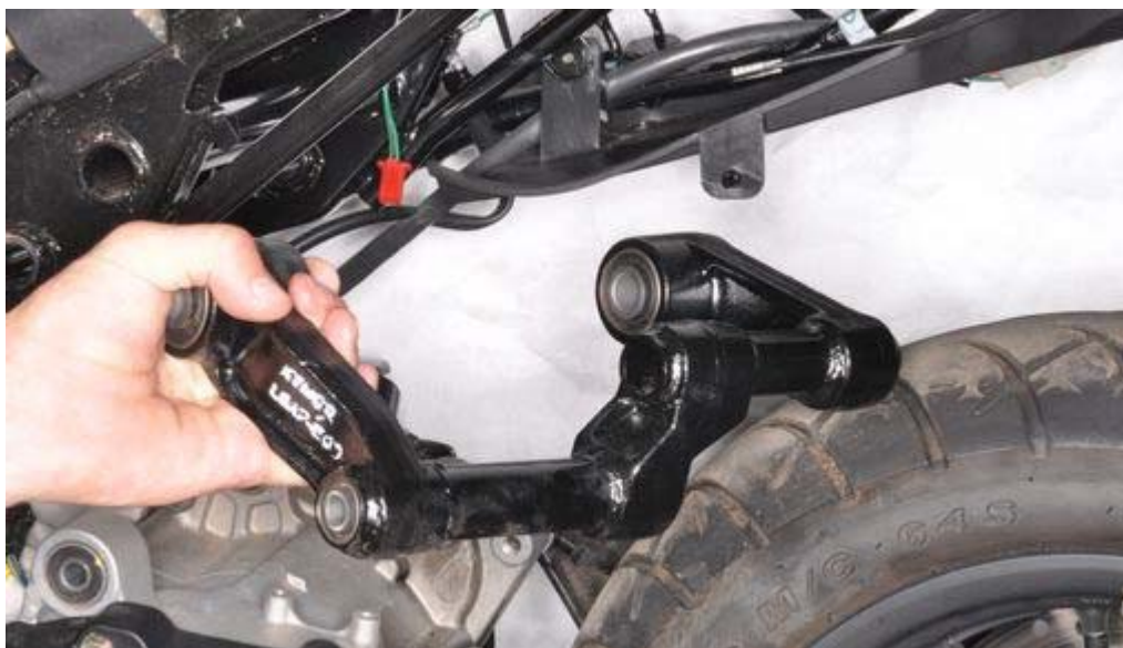
Remove the engine mounting bracket.
