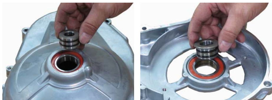
Remove two bearing collar.
