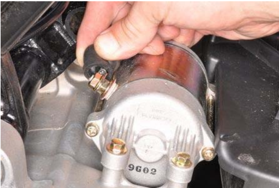
Pull back the rubber starter motor lead cover.
