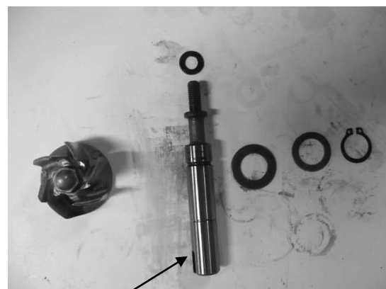
Water pump shaft
