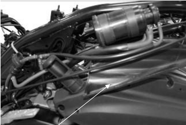
Charcoal Canister/ Purge Control Valve
