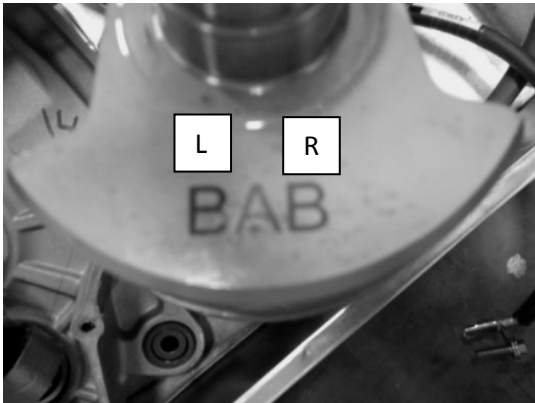
Crankshaft Select mark A or B. Picture L with L case select Picture R with R case select
