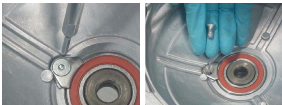
Remove the bearing fixed plate with a 5 mm Allen.
