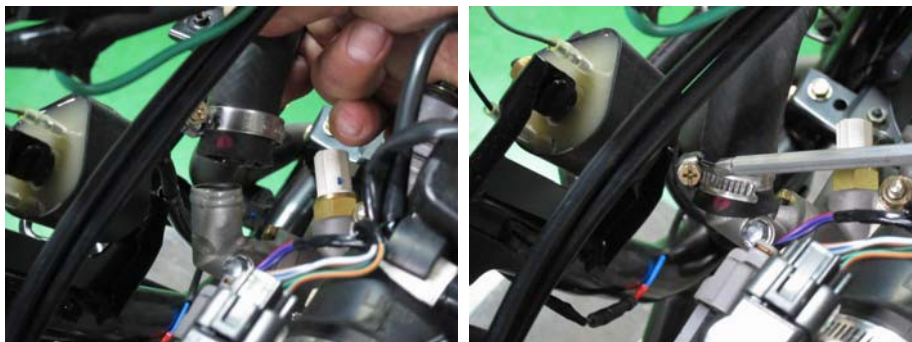
Connect the coolant hose to the thermostat. Move the clamp into place and tighten it securely with a #2 Phillips screwdriver.
