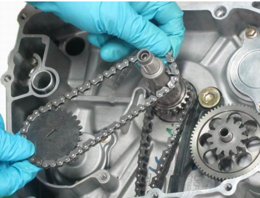
Remove the oil pump drive chain and driven sprocket.
