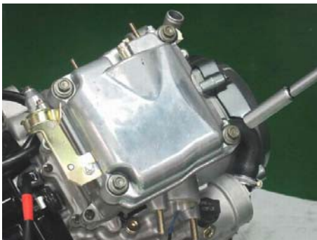
Loosen the four cylinder head cover bolts with a 10 mm socket. Remove the cylinder head cover bolts with washers and grommets. Note the gold colored and longer bolts are on the right side.
