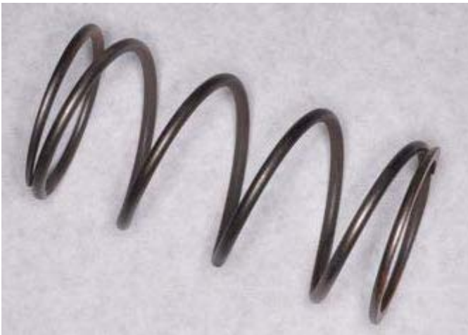
Measure the free length of the clutch spring. Replace the spring if the measurement fails to meet the service limit.
