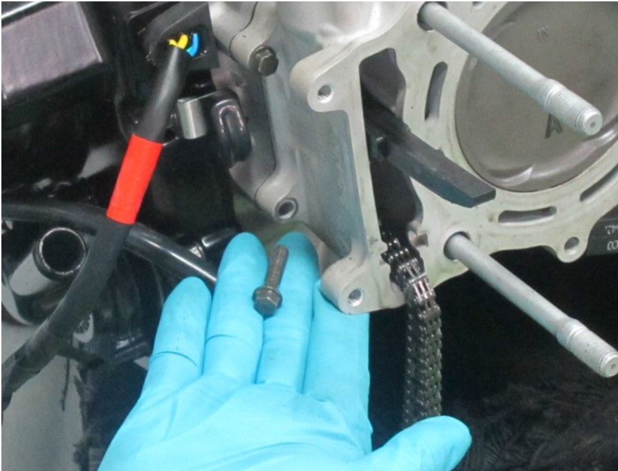
Thread in the two cylinder bolts on the right side of the engine.
