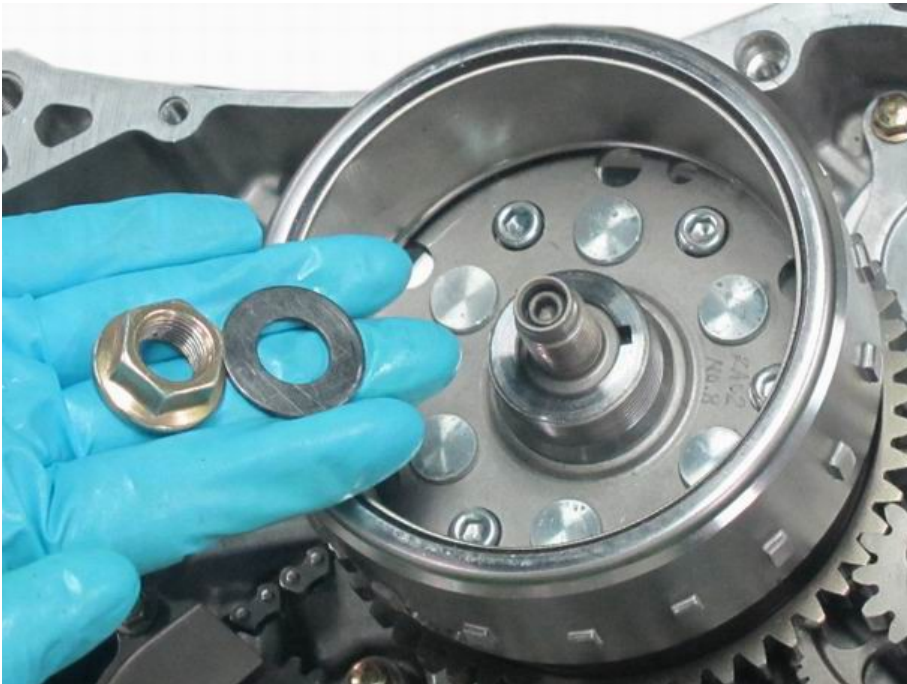
Remove the flywheel nut and washer.
