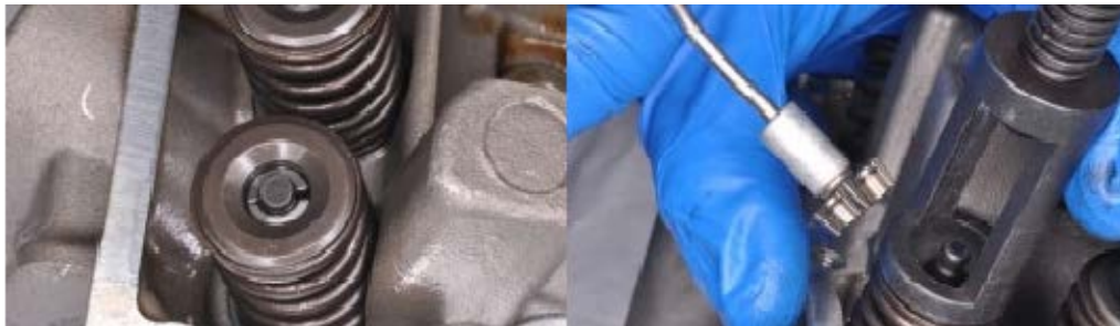
Remove the split keepers. There are two per valve.
