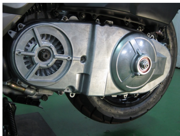
Remove the belt case cover and gasket.
