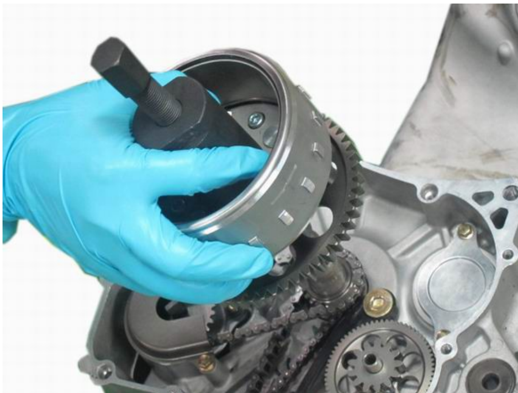
Remove the flywheel from the crankshaft.
