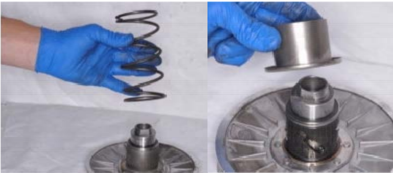
Remove the collars and spring.
