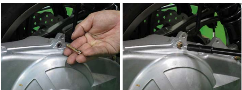
Install the belt case cover bolts and tighten them securely with an 8 mm socket.
