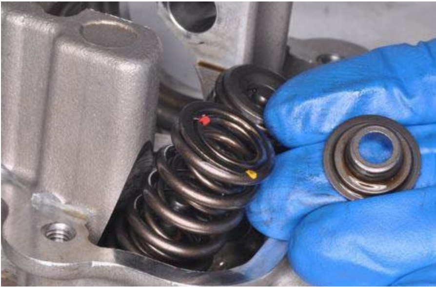
Place the spring retainer on top of the spring.
