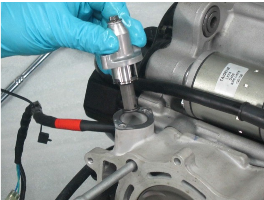
Lift the cam chain tensioner out of the cylinder. Remove the cam chain tensioner gasket.
