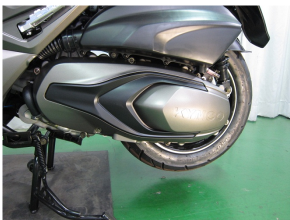
Remove the belt case protector.
