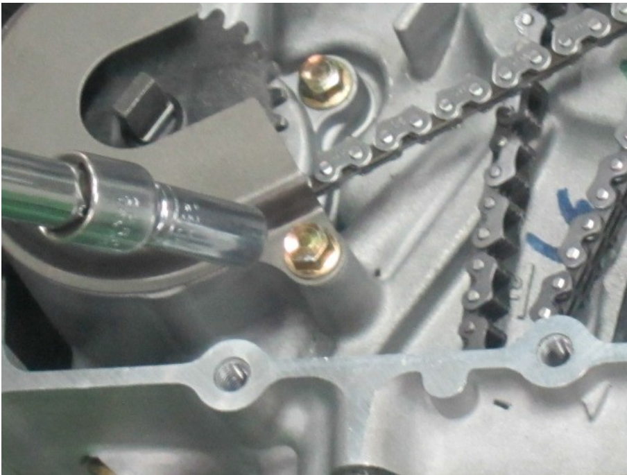
Tighten the two oil pump cover bolts securely with an 8 mm socket.
