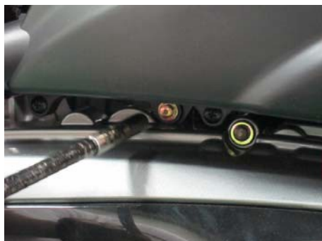
Remove 2 the air cleaner bolts with an 8 mm socket.
