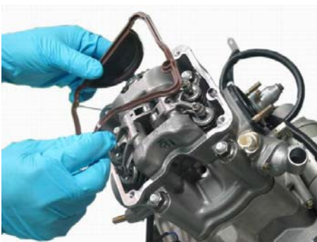
Remove the cylinder head cover and gasket. Discard the gasket and replace it with a new item on installation.
