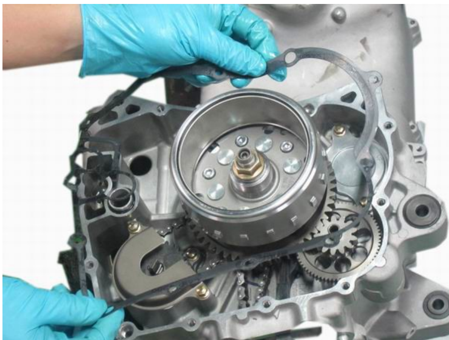
Remove the generator cover gasket.
