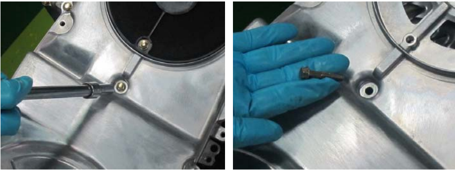
Remove the nine bolts mounting the left crankcase cover.
