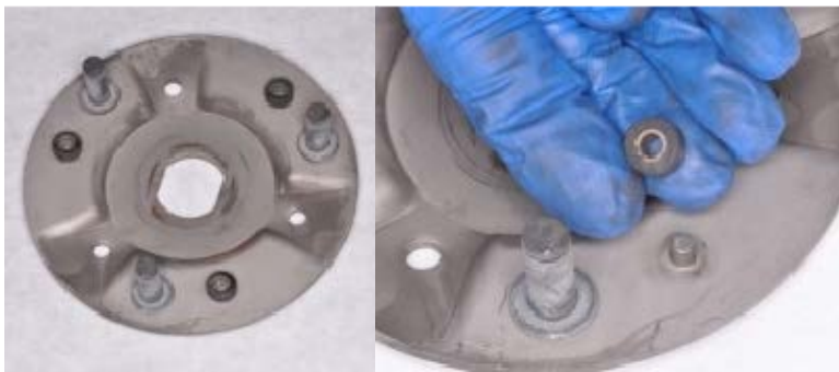
Inspect the clutch shoe bumpers and replace them as needed.
