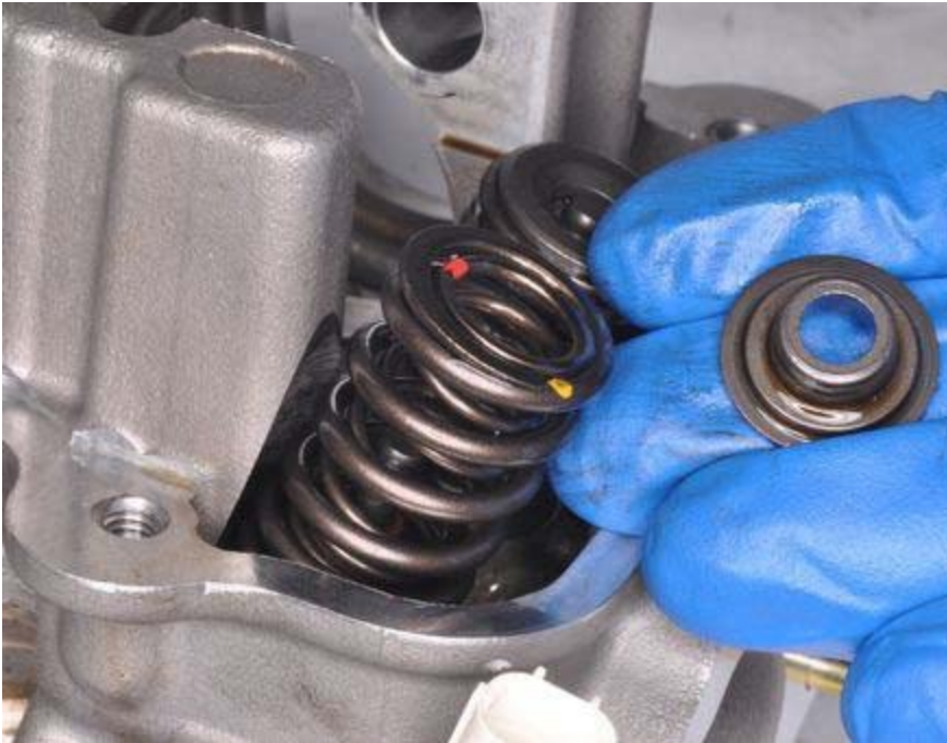
Remove the spring retainer.
