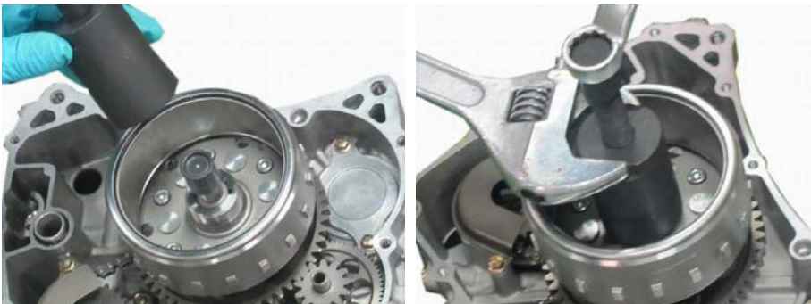
Apply a protect stay to the threads of the crankshaft before using it. Hold the tool with a large wrench and turn in the bolt until the pressure separates the flywheel from the crankshaft.
