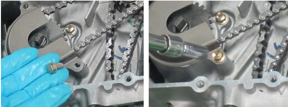
Install the oil pump cover and its two mounting bolts.
