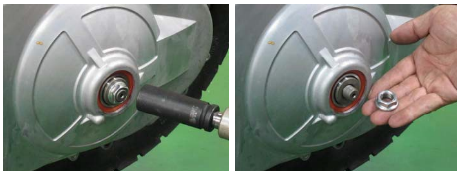
Remove the driven pulley nut with a 24mm socket.
