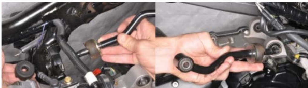
Remove the engine mounting bracket damper assembly.
