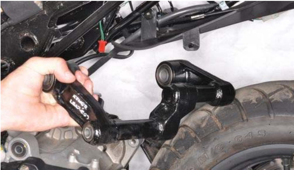
Remove the engine mounting bracket.
