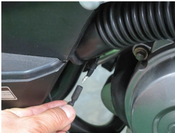
Plug in the oil pressure switch bullet connector.
