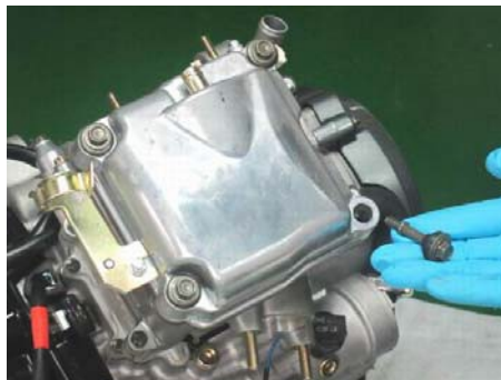
Loosen the four cylinder head cover bolts with a 10 mm socket. Remove the cylinder head cover bolts with washers and grommets. Note the gold colored and longer bolts are on the right side.
