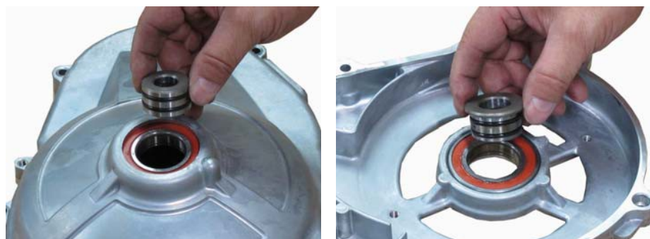
Remove two bearing collar.
