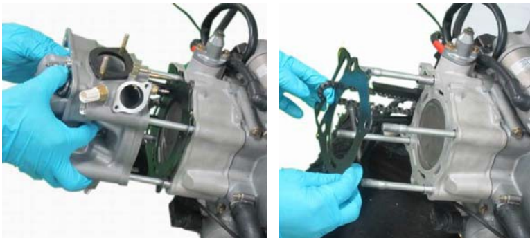
Remove the cylinder head assy and gasket.
