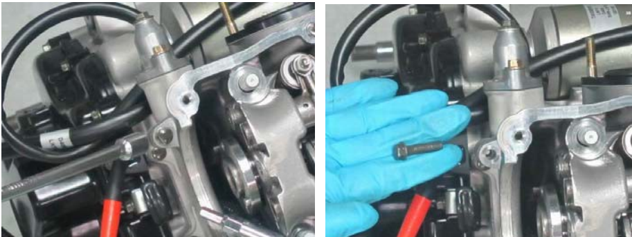
Remove the two bolts on the right side with a 8mm socket.
