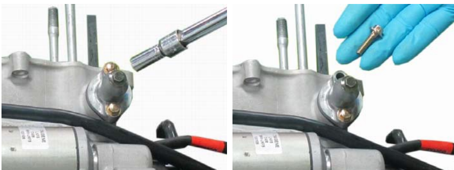
Loosen the cam chain tensioner mounting bolts evenly with an 8 mm socket.
