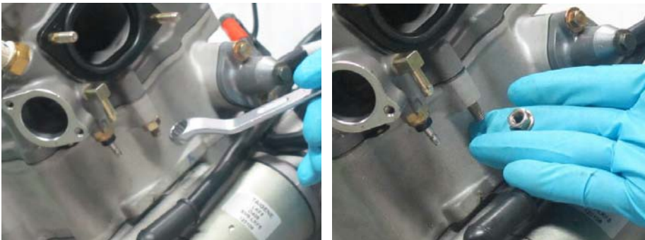
Remove the nut on the inlet pipe side with a 10mm socket.
