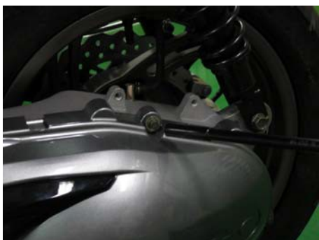
Remove 6 the belt case plastic cover bolts with an 8 mm socket.
