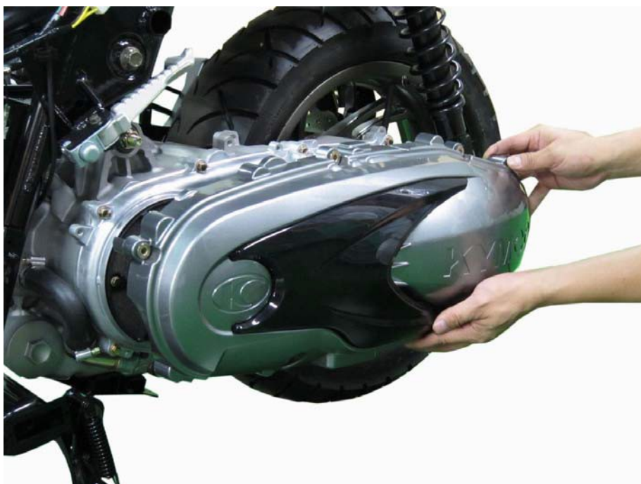
Install the belt case plastic cover.
