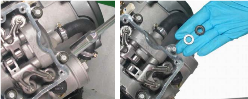
Remove the two nuts and washers on the left side with a 14mm socket.
