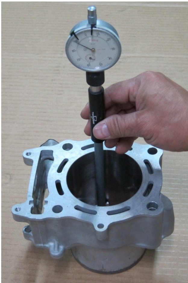
Measure the cylinder diameter as described below with a telescoping gauge.
