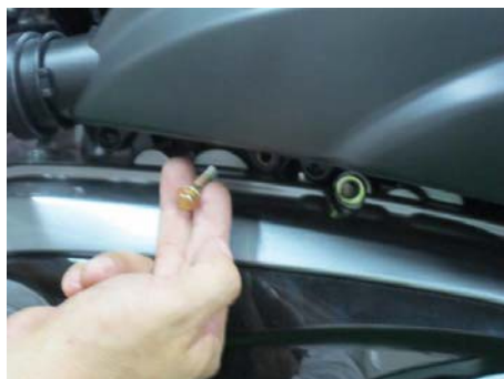
Remove 2 the air cleaner bolts with an 8 mm socket.
