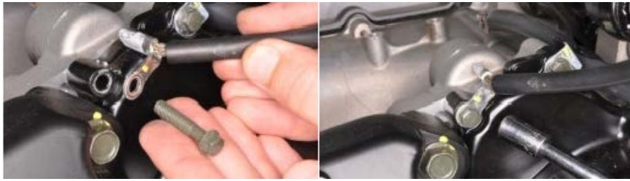
Install the main engine ground to the right side of the engine. Tighten the main engine ground bolt securely with an 8 mm socket.
