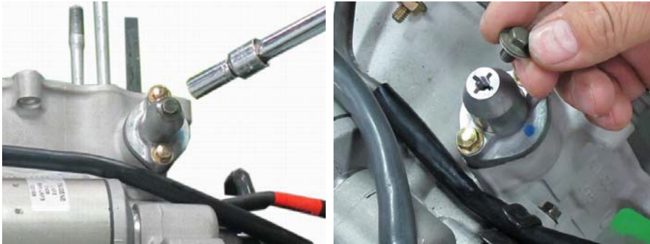
Remove the cam chain tensioner cap bolt with a 8 mm socket.
