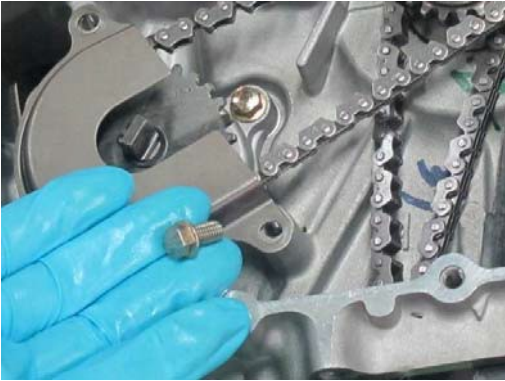
Remove the two oil pump cover bolts and the oil pump cover.
