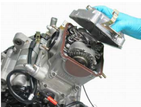
Remove the cylinder head cover and gasket. Discard the gasket and replace it with a new item on installation.
