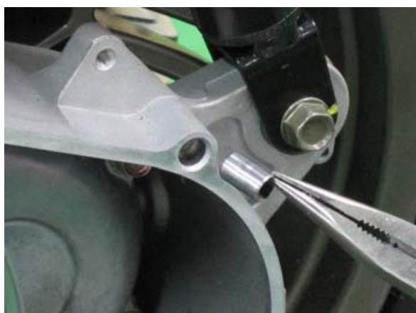
Remove the two dowel pins.
