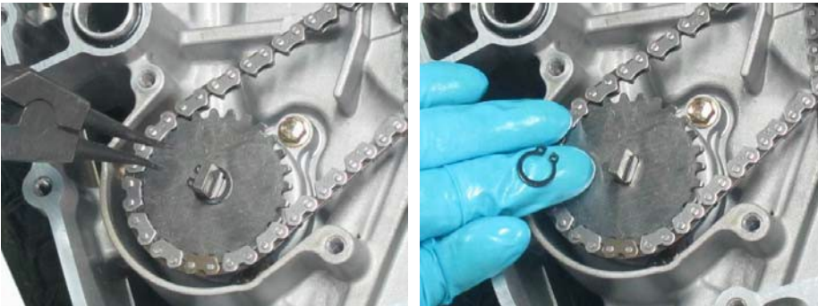
Remove the snap ring on the oil pump shaft with snap ring pliers.
