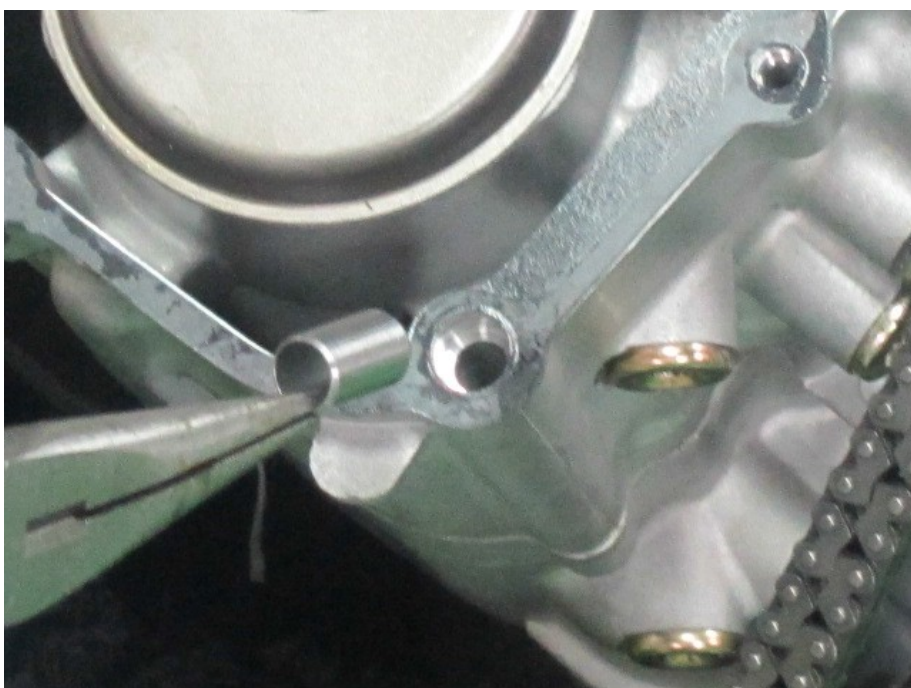
Remove the two dowel pins.
