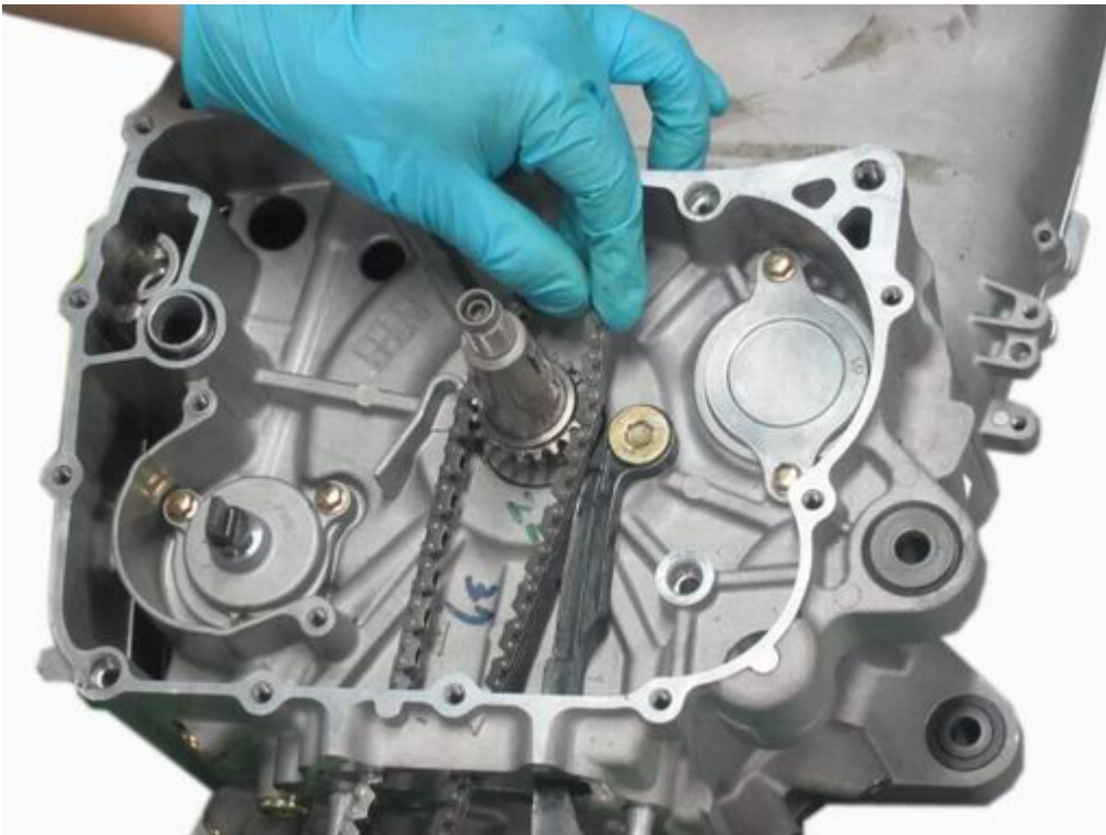
Install the cam chain around the timing sprocket teeth on the crankshaft.
