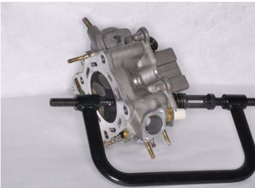
Push down the valve springs with a valve spring compressor to allow enough room to install the split keepers. The valve cotter installer tool can also be used to install the split keepers.
