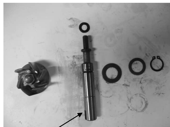
Water pump shaft
