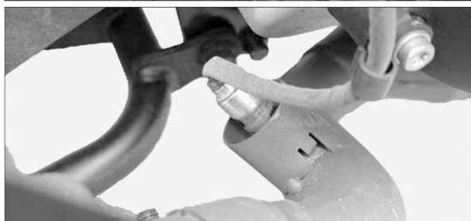
This vehicle is provided with O2 Sensor for reducing generation of pollutants in the exhaust gas.
