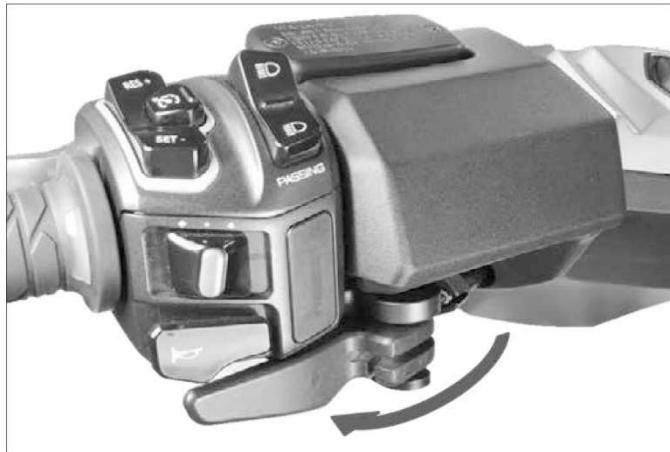
Turn Parking Lever to the left and click into lock position. To unlock, just turn Parking Lever back to its original position (on the right).
