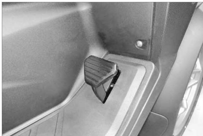
This vehicle is equipped with the foot brake function as an auxiliary to the front/rear braking system. Thus, the foot brake has a linkage to the front/rear brake when braking.
