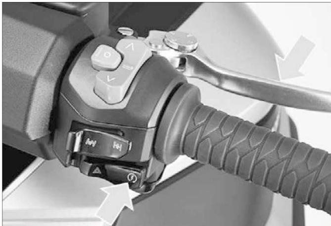
6. If starting is difficult, release the Start Button and wait for a few seconds before trying again. Each re-try shall not exceed 5 seconds, for preserving battery power.
