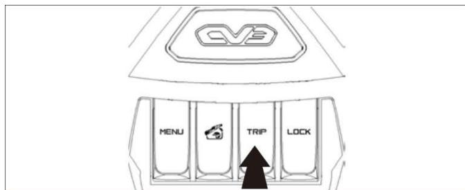
Press the "TRIP" button on the central multifunction switch to switch trip modes on the main screen.
