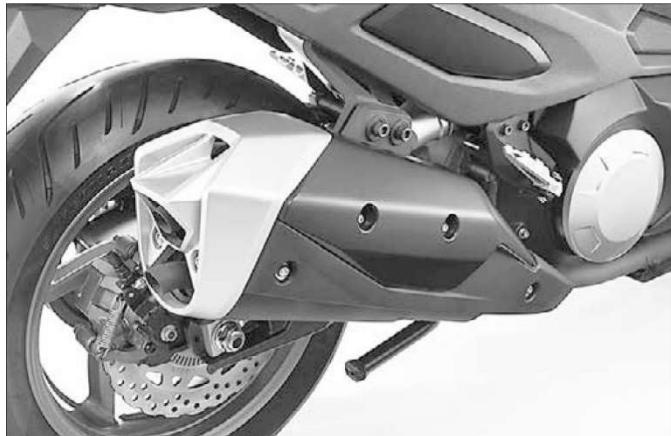
Catalytic Converter is used for reducing generation of pollutants in the exhaust gas.
