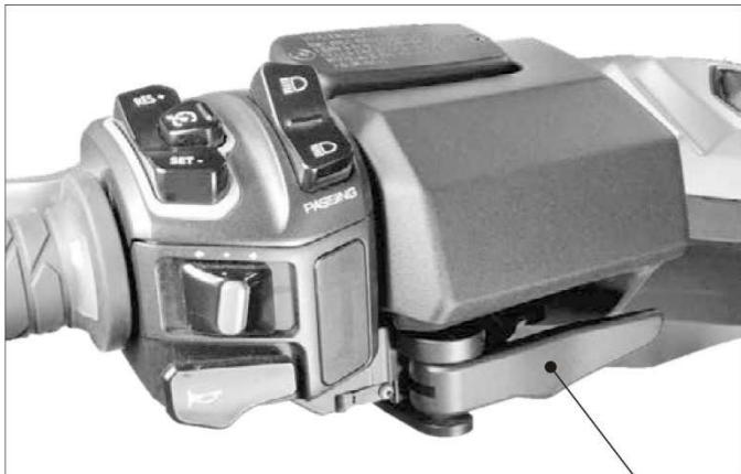
This vehicle is provided with a Parking Lever for locking up the rear tire, so as to prevent accident caused by rear tire movement when parking the vehicle on a slope.
