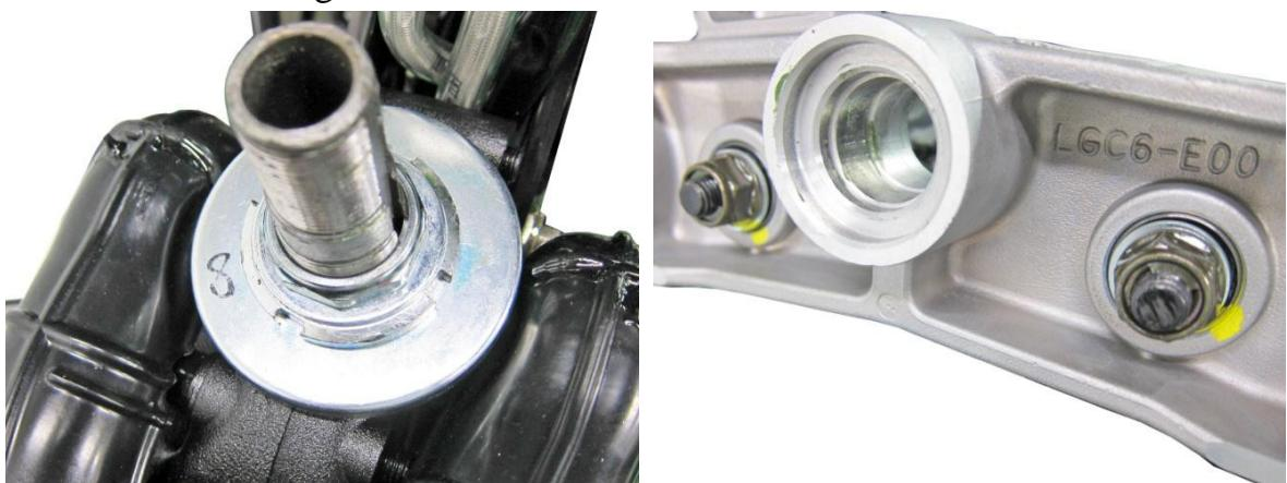
Remove the octagonal nut and the washer in order to separate the Steering Handlebar Unit. Tightening torque value during the installation: 3-4 kgf-m (30-40 N-m)
