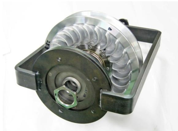
Loosen and remove the spring compressor tool.
