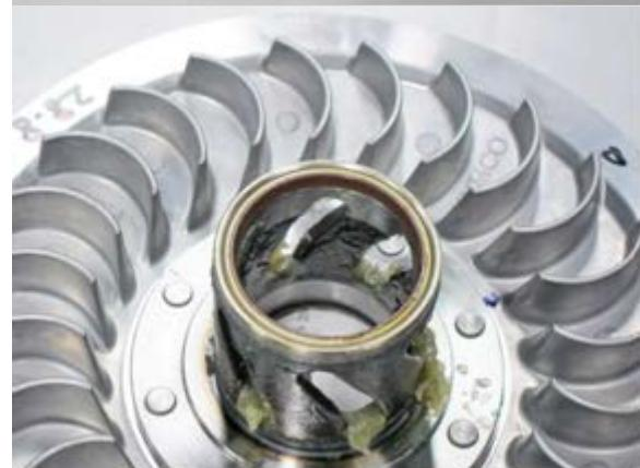
Replace the upper-side oil seal of Passive Drive Disc.
