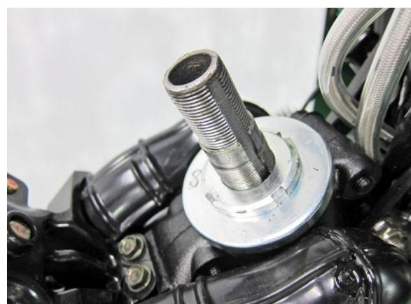
Remove the open-end nut (square nut) from the Top Seat ring with a special tool.
