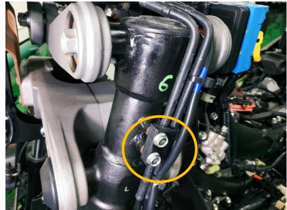
Move the oil pipe of the left and right head tubes to one side and then remove the dust-resistant rubber cover from the head tube.
