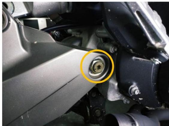
Tightening torque: 900–1100kgf.m
