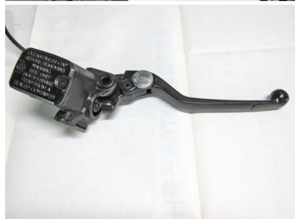
Install the brake master cylinder to the mount. Install the front and rear brake cables and adjust them to their appropriate free play. Install the dust boot.
