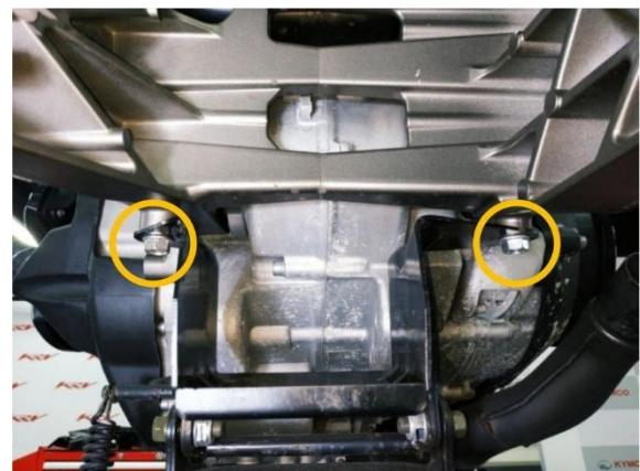
Remove the rear fork swingarm bolt.
