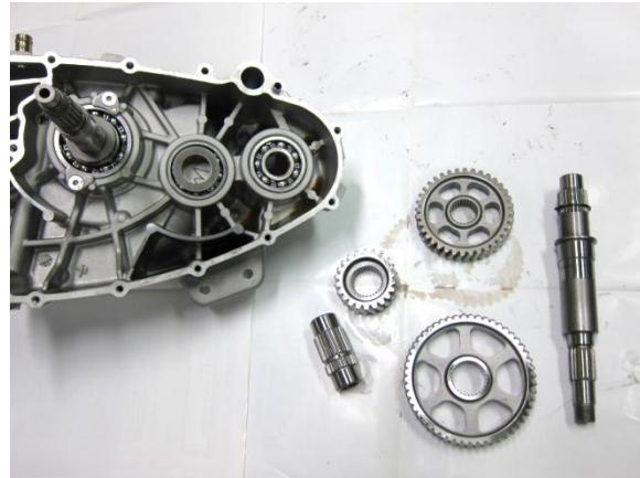
Remove the washer and remove the drive shaft.
