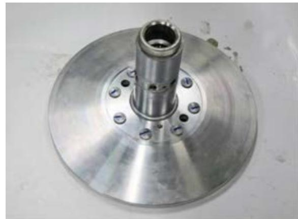
Replace the lower-side oil seal of Passive Drive Disc.
