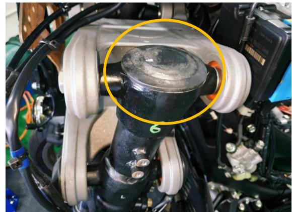
Remove the nut and then pull out the Front Fork head tube unit and then it will be separated easily.
