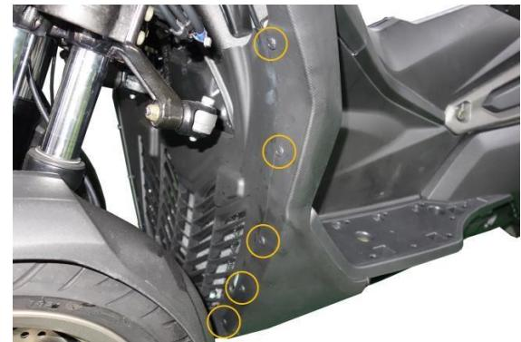
Remove B screws from the pedal and the right protection cover.
