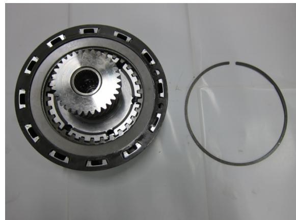
Remove the retainer and spring.
