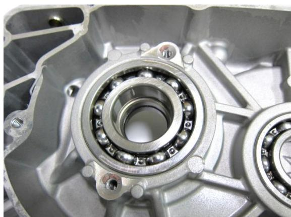
Remove the bearing by bearing puller tool.
