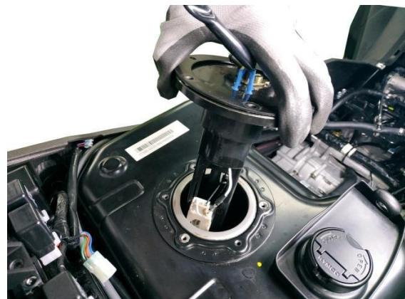
Remove the oil gas recovery pipe and then remove the oil tank.
