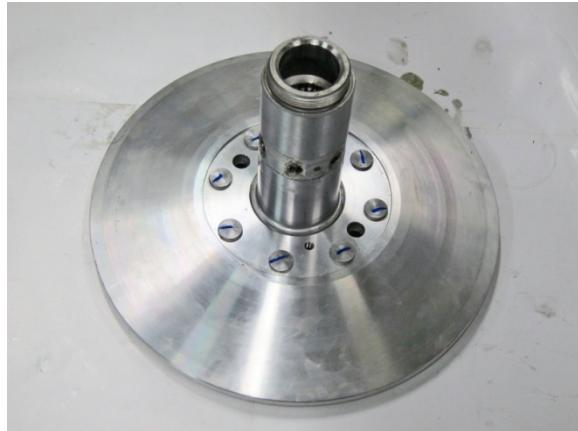
Replace the seals from the driven pulley.
