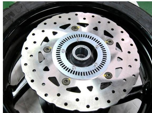
Remove the Rear Wheel socket and then remove the bolt from the Reading Panel.
