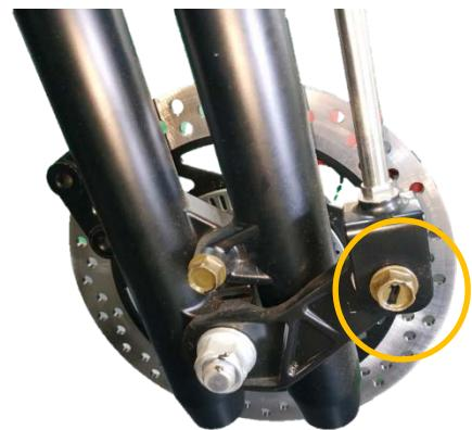
Remove 2 hexagonal socket screws from the upper side of Front Fork Locking Rod Unit.
