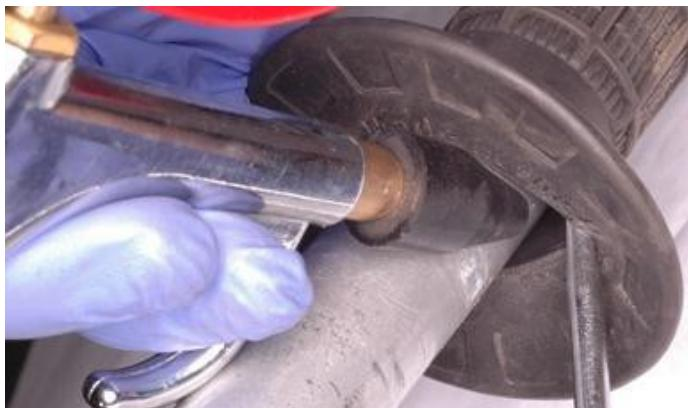
Remove the Handlebar Cover with an air gun. When installing new Handlebar Cover, clean the installation area (removing the residual glue). Apply slight amount of superglue and then install the handlebar cover. Use the vehicle after the glue is dried through.
