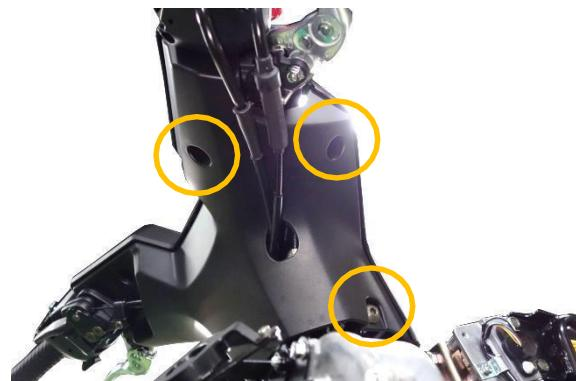
Remove 3 screws underneath the left steering handlebar cover.
