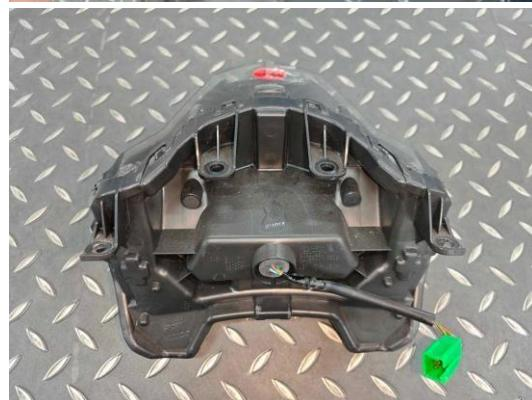
The rear light assembly includes the taillight, brake light, and left and right turn signals. If damaged, the entire rear light assembly must be replaced.
