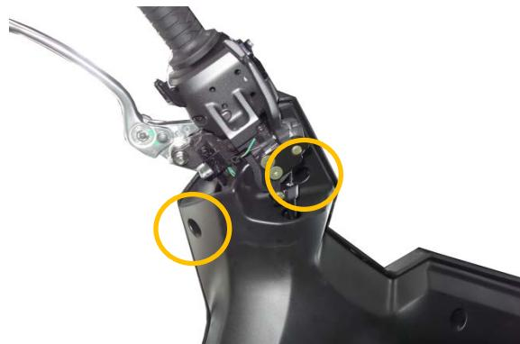
The removal shall be executed with plastic removing tool to prevent from hurting the plastic surface.
