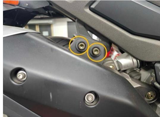
Remove 1 screw under the exhaust pipe
