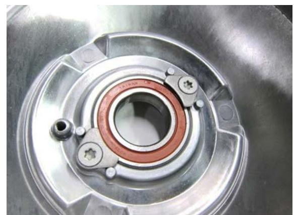
Remove the C-shape clip from the bearing with an external caliper and then remove the bearing with the bearing puller.
