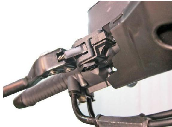
Remove the lead wire connector from the brake indicator switch. Remove the right brake handle and the brake indicator switch.
