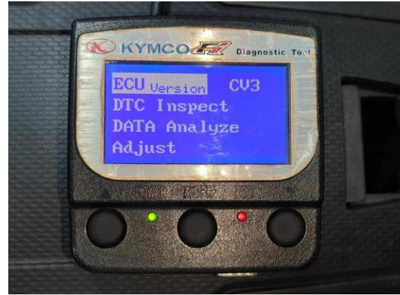
Display of Software/Hardware Version and Calibration Code
