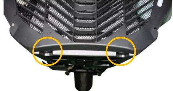
Remove 2 screws from both sides respectively and then remove Fender-A.
