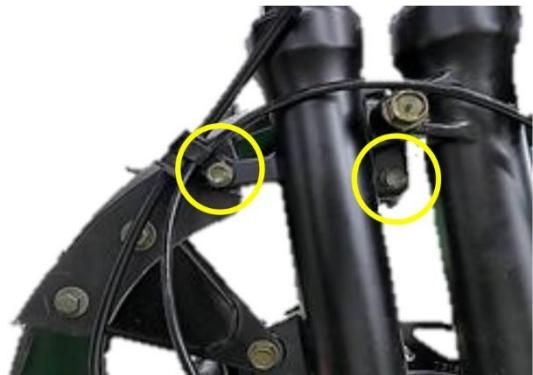
Remove the front wheel Fender cover.
