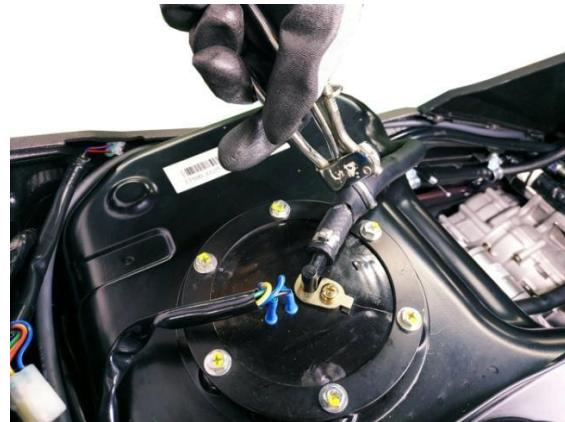
Loosen the fuel pipe clamp with high-pressure retaining clip.
