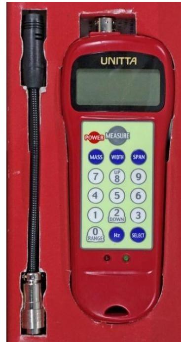
~1. Input Belt mass constant, width and belt wheelbase.
