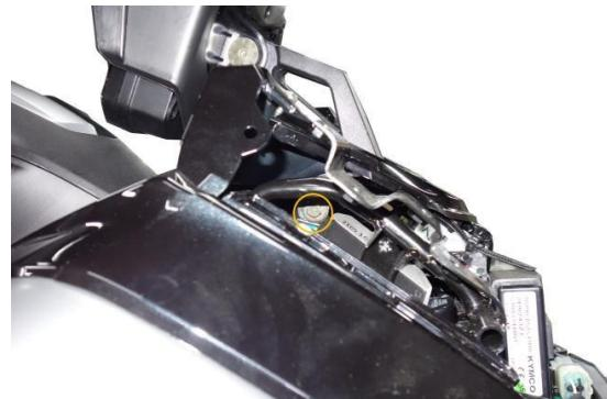
Insert the joint area with a screwdriver and you can pry open the fixing plate easily. Take out the fixing plate and the metering assembly can be removed easily.
