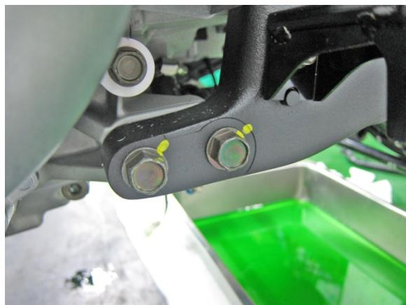
Carefully move the front frame forward and separate it from the engine.
