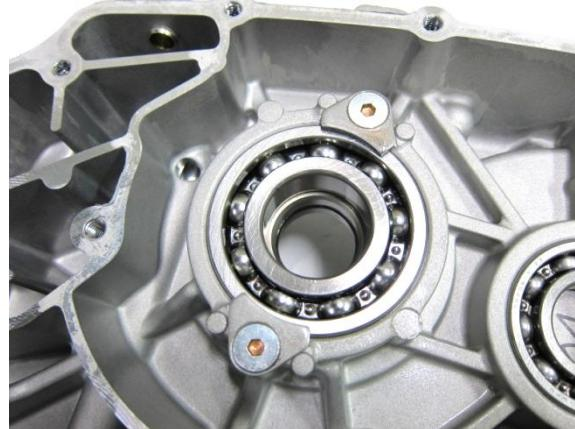
Remove the two bearing fixed plate.
