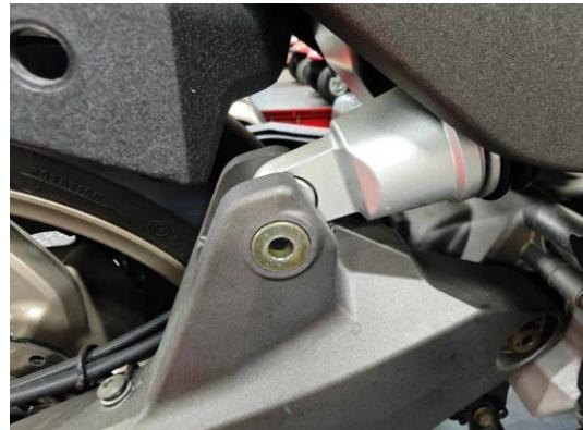
Next, remove the single upper shock absorber bolt.
