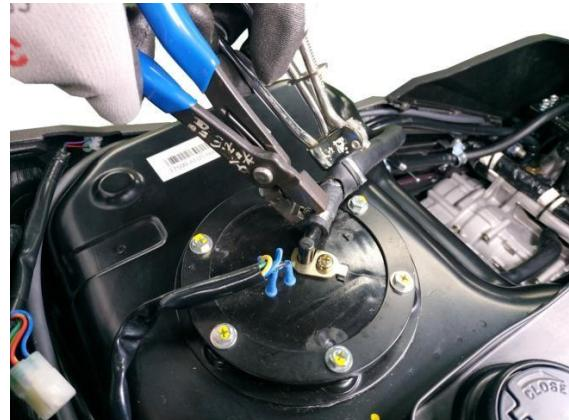
Then take out the fuel pipe with the pipe-loosening clip.
