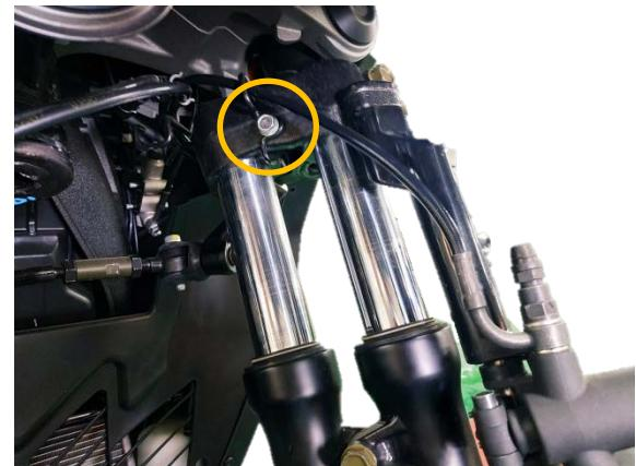
Remove the screws from lower side of Front Fork Locking Rod Unit.
