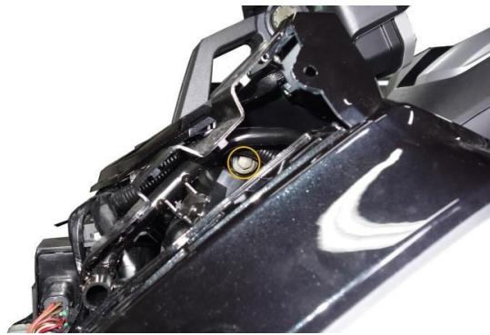
Remove the right screw from the metering assembly.
