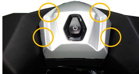
After remove the center screw, remove the upper steering handlebar cover.
