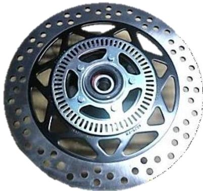
When installing the encoder disc, follow the star-shaped order.
