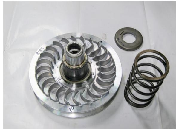
Check if the spring of Passive Drive Disc is abnormally worn. If required, replace it with a new one.
