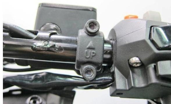
During the installation, confirm that the fixing hole of the mounting base is inserted into the fixing hole of the steering handlebar.
