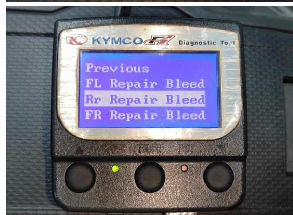
Select “Rear Wheel Exhausting,” the ABS will start the exhausting process for the rear wheel hydraulic lines.
