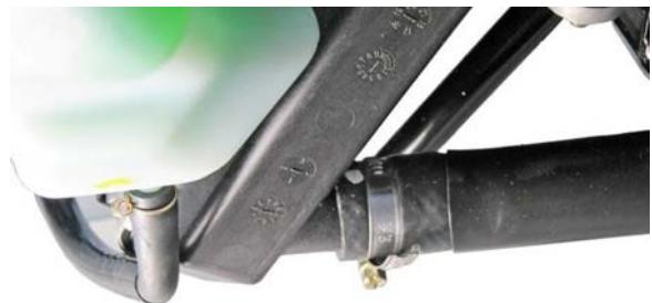
Remove the Radiator lock bolt.
