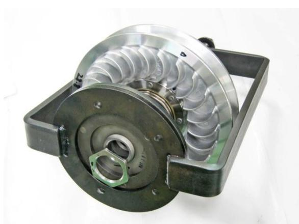
Disassemble the Passive Drive Disc Unit.
