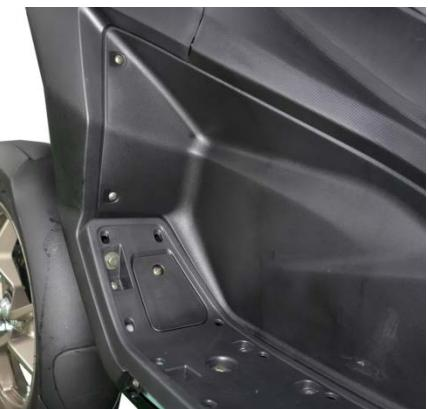
Remove the protection cover screws and then remove the protection cover and the Auxiliary Radiator cap.
