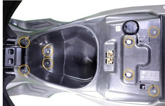
Before removing the storage box, it is required to remove the connected LED wire and the power socket connector
