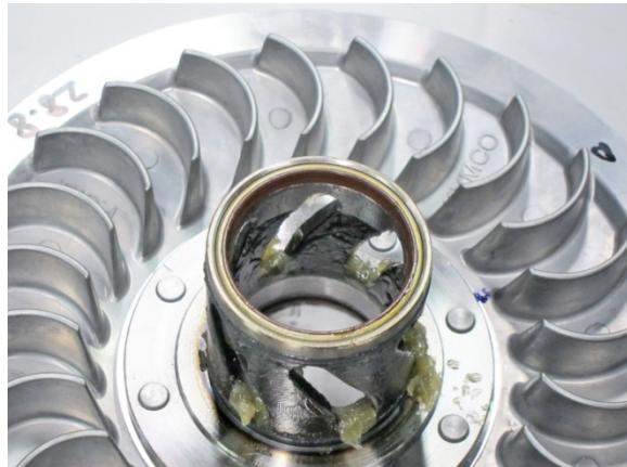
Replace the O-rings of the driven pulley.
