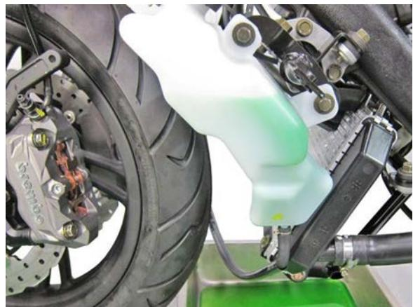
Remove 2 bolts from the Auxiliary Radiator.
