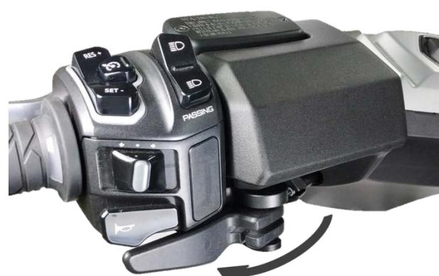
Before adjusting the Hand Brake, loosen the nut and then tighten the nut.
