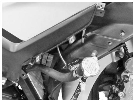
Note: If any heat sink is dented or sticking together, separate the heat sink row one by one.
