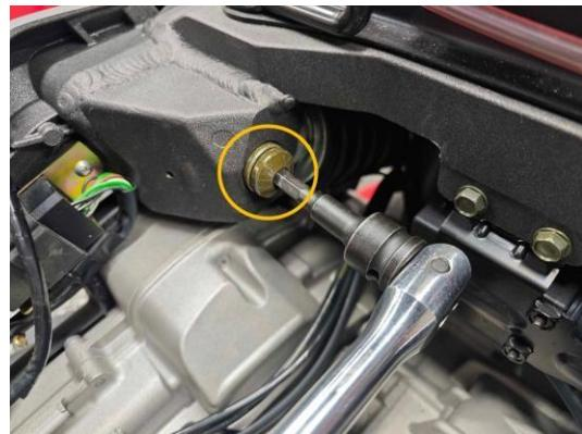
Carefully take off the shock absorber and the bolt.
