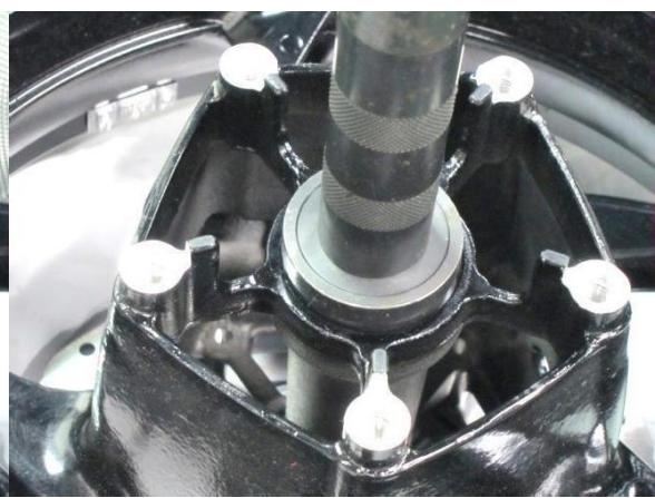
Install the new bearing with the Bearing Installation Device. After being installed, the bearing shall be flush with the rim face without any protrusion.
