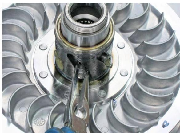
Remove the drive plate from Passive Drive Disc.
