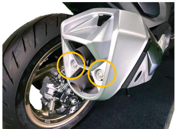
Remove the exhaust pipe rear cover.
