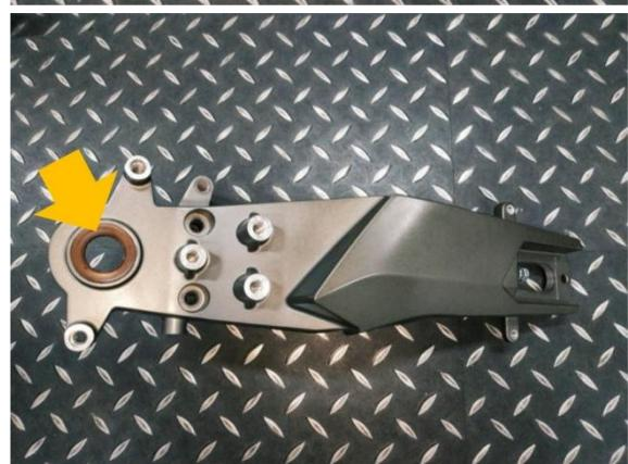
Remove the inner oil seal and bearing.
