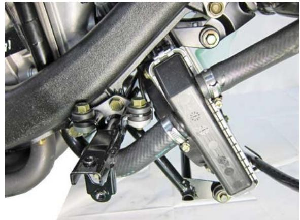
Move the Radiator pipeline and the rest of other lock bolts.
