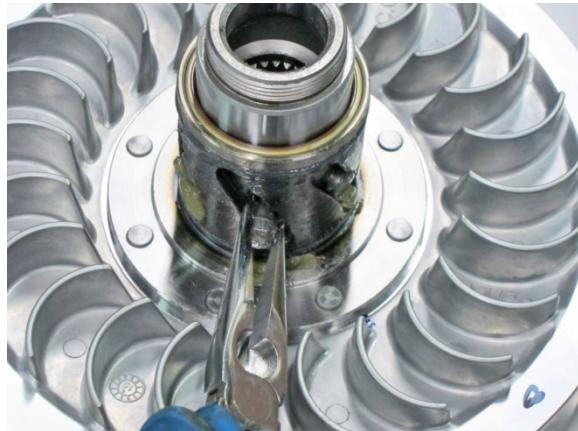
Separate the left and right faces of the driven pulley.
