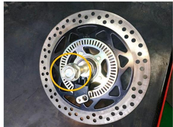
Remove the Front Wheel Hub Assembly. Remove 5 screws from the disc and then remove the wheel speed reading panel.
