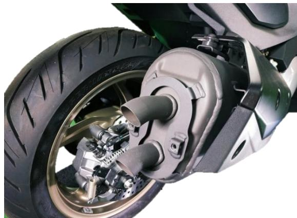
Next, remove the 2 hex socket screws of the exhaust pipe upper cover.
