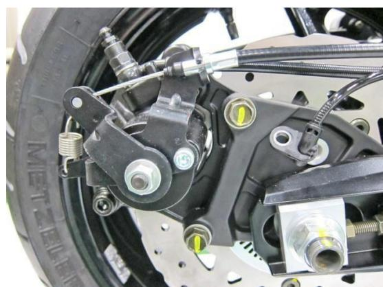
Apply blue Loctite agent on the bolts. If required, make new bolt replacement.
