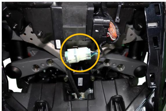
Remove the left and right indicator lamp connector wire underneath the hand lamp.
