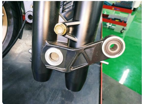
During the installation, restore the Front Fork back to the positioning point and then insert the disc screws.
