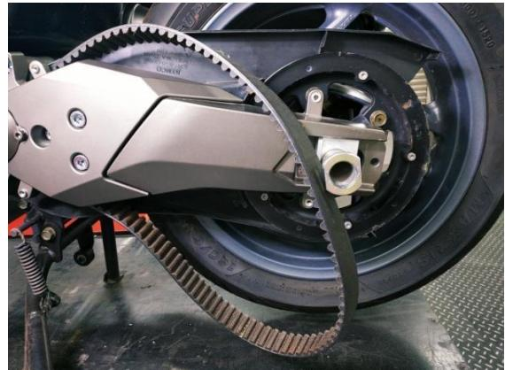
Remove the rear wheel axle screw, and remove the related adjustment components.
