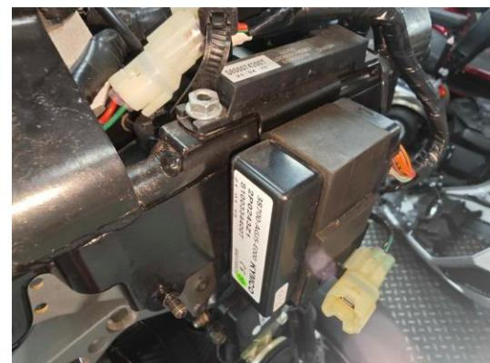
Remove the storage box. Unscrew the fixing screws of the seat opening controller and remove its wires and connectors. Remove the seat opening controller.
