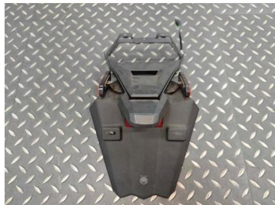
Unscrew the two hex socket screws on both sides.
