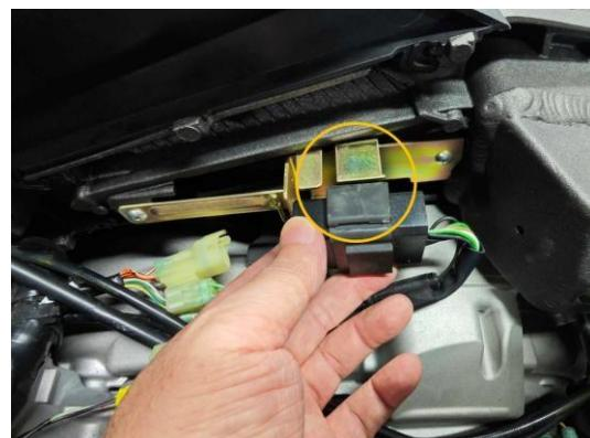
Remove the heated handlebar controller.
