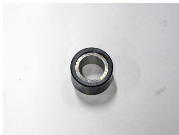
Remove the rollers and check them for excessive or uneven wear. Replace the weight rollers as needed.
