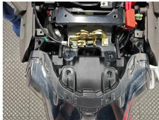
Remove the rear light assembly connector.
