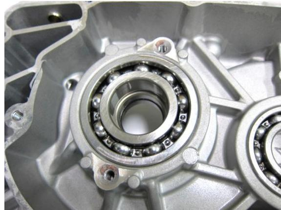
Remove the bearing by bearing puller tool.
