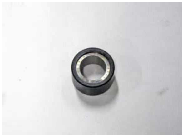
Check if the weight rollers are presenting any wearing or abrasion sign. If required, replace it with a new one.
