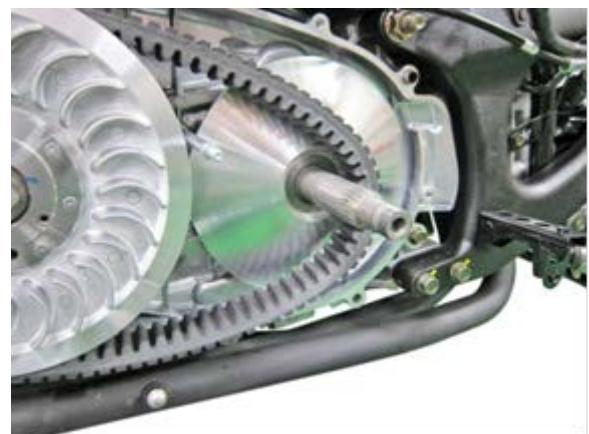
Slide Drive Disc Disassembly Diagram
