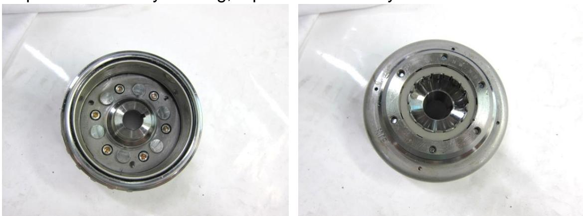
Remove the starting clutch gear.
