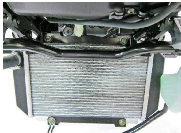
Remove the Radiator from the frame.
