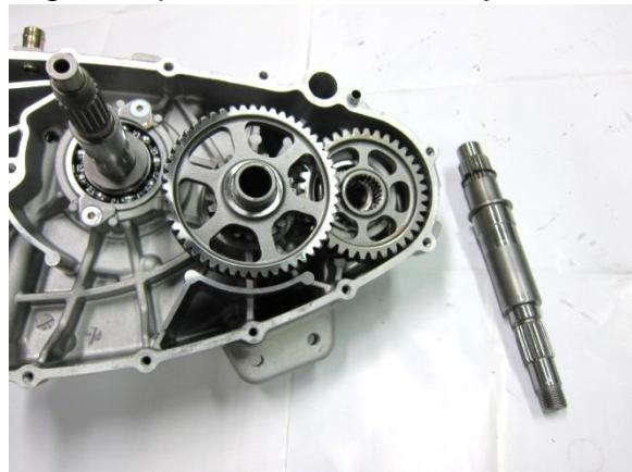
Remove the counter A gear and remove the final gear.
