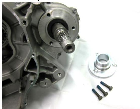
Remove the bolts and remove the left mission case.
