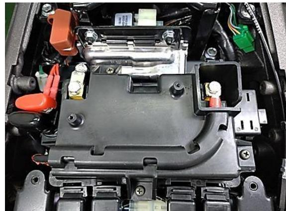
Alternatively, if you want to remove the battery, first remove the battery cover by unscrewing 3 screws.
