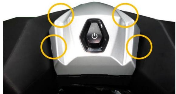
After remove the center screw, remove the upper steering handlebar cover.
