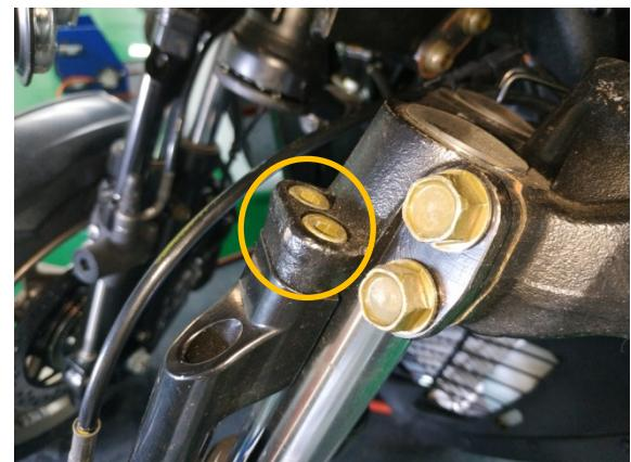
When removing the Front Fork Locking Rod Unit, put both bushings aside for use again.
