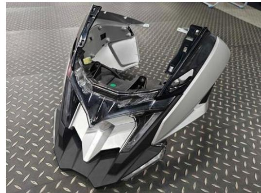
Remove the mounting screws/plastic screws of the right/left light assembly.
