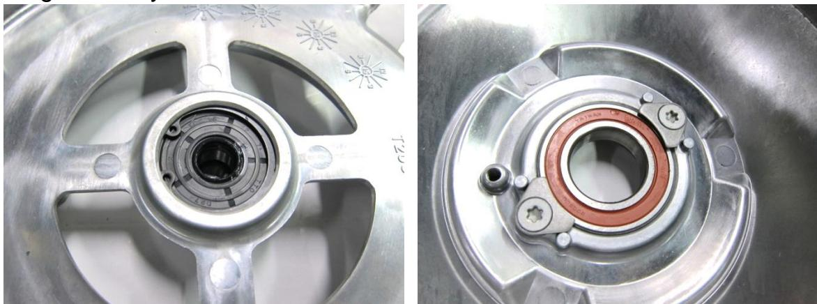
Remove the bearing snap ring with snap ring pliers.
