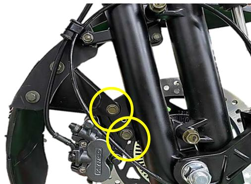
Remove 3 bolts from the fender cover and then remove the fender cover.
