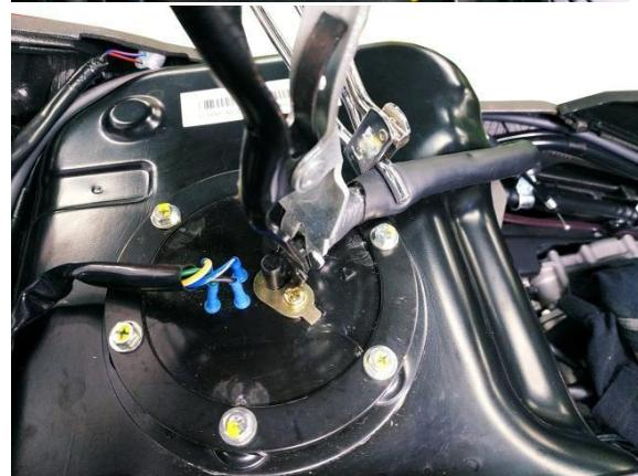
Connect the Oil Pressure Gauge and then start the Fuel Pump test. If failing to meet the specifications, replace it with a new one.
