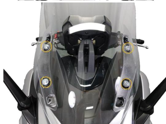
Remove the windshield fixing base.
