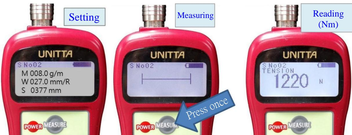
Step 2-2: Measure the belt tension with Belt Audio Tensioner.
