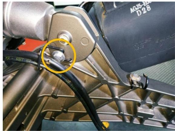
Remove the shock absorber lower screw
