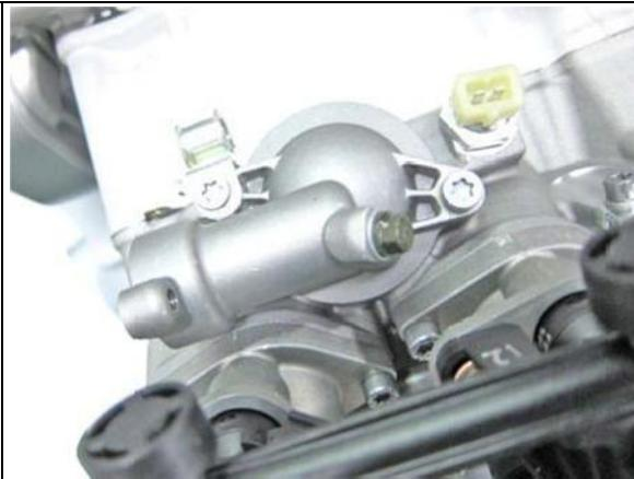
Remove the WTS with 17mm socket.
