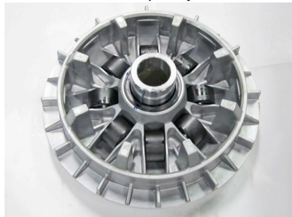
Remove the rubber damper pieces from the ramp.
