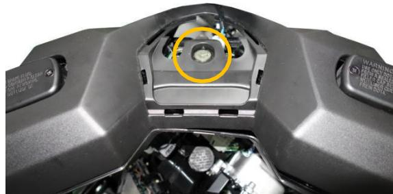
Remove the lower steering handlebar cover.
