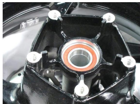
Check if the bearing is rotating smoothly and if any abnormal sound is heard. If abnormal, replace it with a new bearing.
