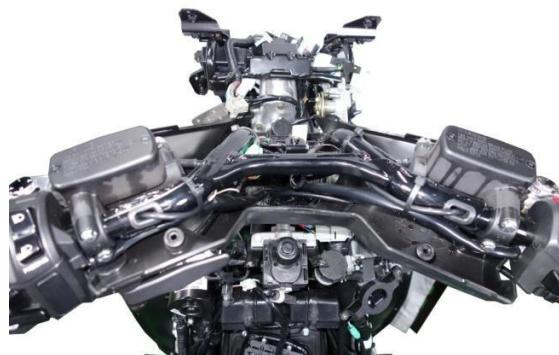
Remove 2 bolts from the brake main cylinder cover with a screwdriver and then remove the cylinder cover. Next, take out the dust cover and the rubber cover.
