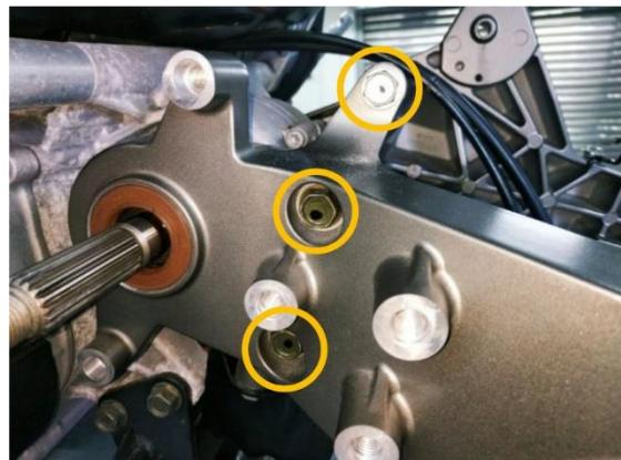
Remove the lower guard of the rear fork swingarm.
