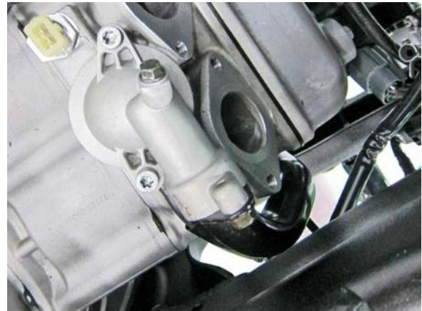
Take out the water temperature regulator water pipe from the Radiator.
