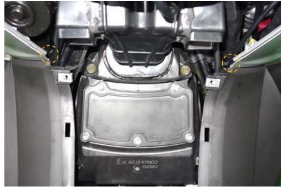
Remove 1 screw from the left and right pedals respectively.
