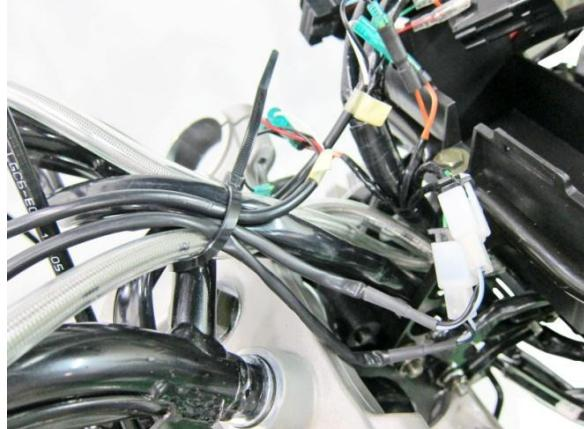
Separate the lead wire connector of each switch.
