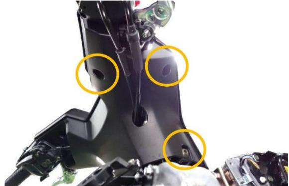
Remove 3 screws underneath the left steering handlebar cover.
