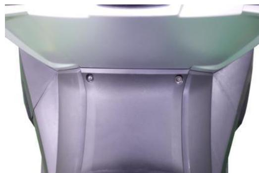
The center cover can be dismantled by removing 2 plastic screws from the upper side.
