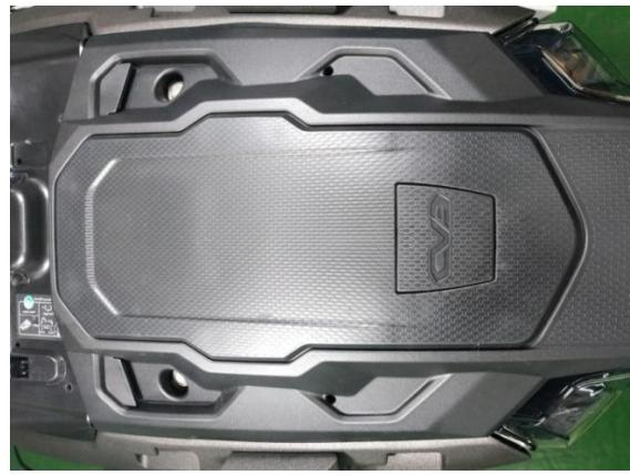
Remove 6 screws and then remove the seat cushion protective cover.
