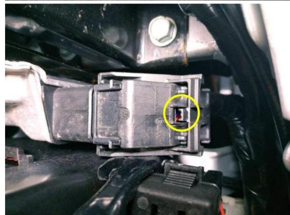
After that, push it straight to the bottom. On hearing the “click” sound, it means the ECU has been opened to the intended position.
