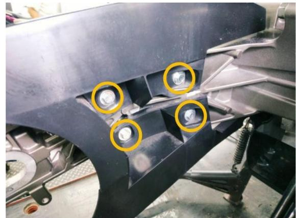
Remove the 3 screws on the front belt pulley cover
