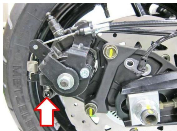
Remove the bolt from rear brake caliper.
