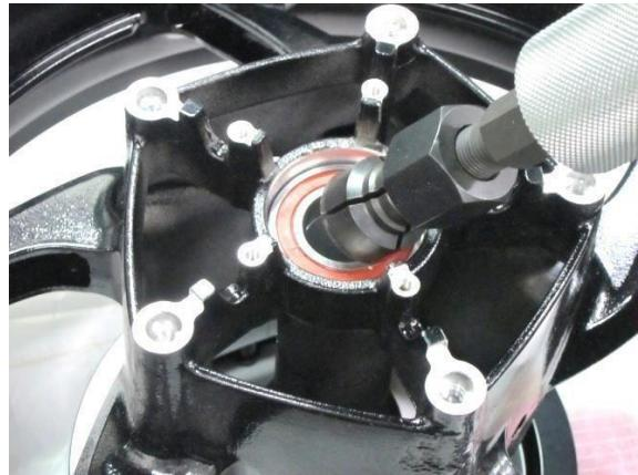
Install the new bearing with the Bearing Installation Device. After being installed, the bearing shall be flush with the rim face without any protrusion.
