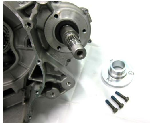
Remove the bolts and remove the left mission case.
