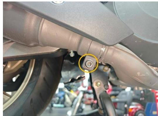
Remove the rear section of the exhaust pipe.
