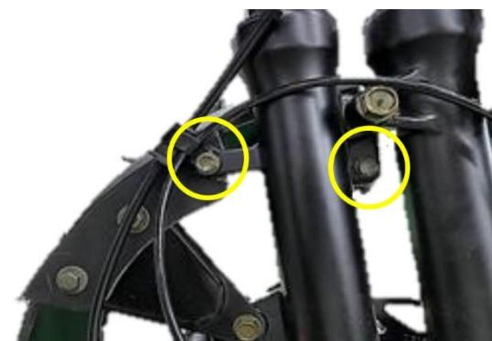
Remove the screws from the wheel speed sensor and the securing hook and then remove the wheel speed sensor.
