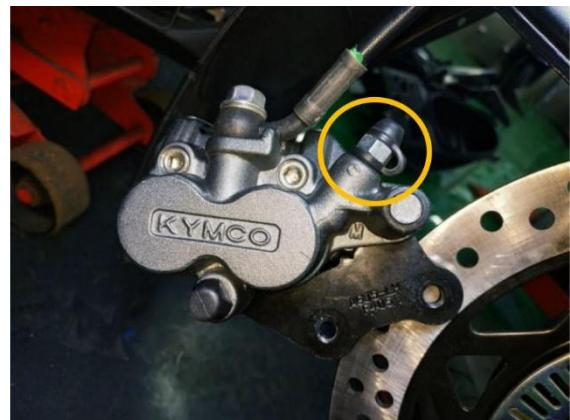
Remove the bolts from the oil pipeline. If required, replace the oil pipeline bolts and washers with new ones.
