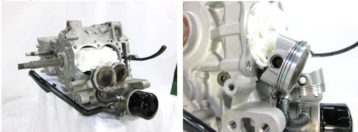
Remove the piston pin and the piston.
