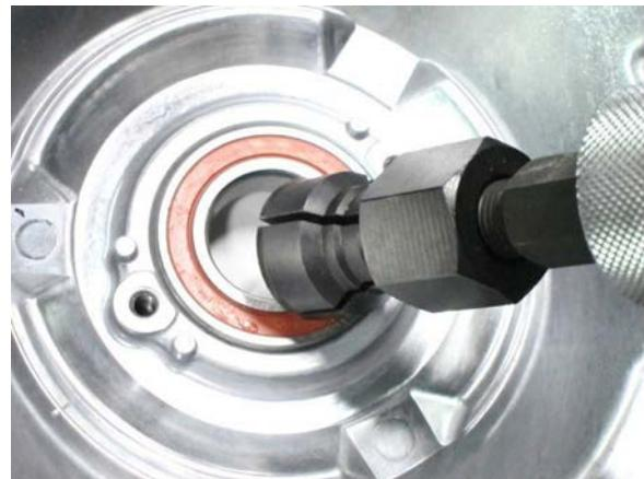
Install new bearing with the bearing installer and then install new C-shape clip with the external caliper.
