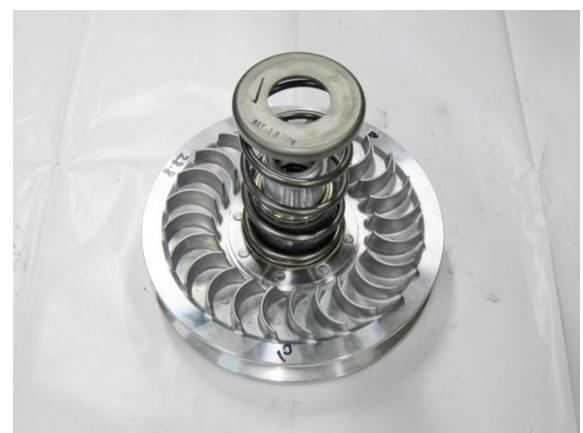
Take out the spring and the securing plate.
