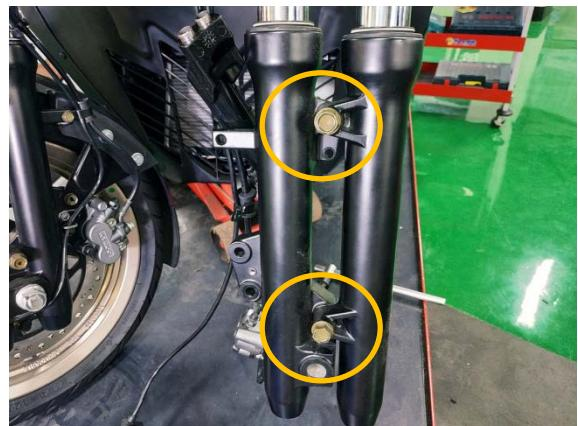
Remove 4 screws from the front and rear sides of Front Fork.
