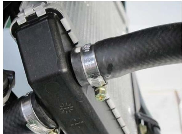
Remove the Radiator lower water pipe securing clip.
