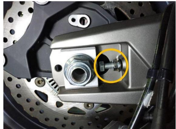
Remove the rear axle mounting nut.
