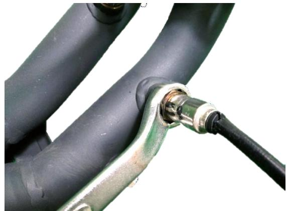
When removing the third oxygen sensor, use a suitable No. 17 socket, like the one used for spark plug removal.
