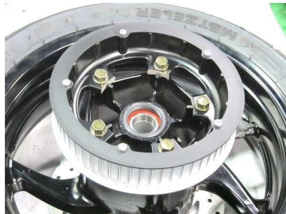
Remove the bolts from the rear drive pulley of outer drive belt. Tightening torque value required for the installation: 3–4 kgf.m (30–40 N·m)
