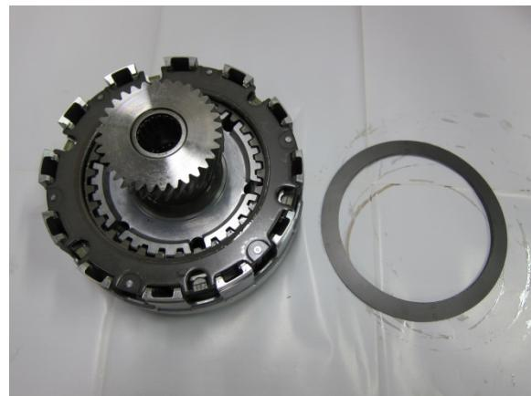
Remove the retainer and friction plates set.
