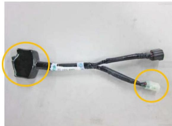
Connect the 4-pin CAN connector to the CAN jack of the connector.
