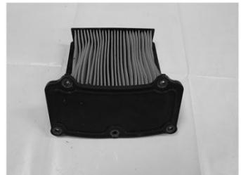
Filter core of the Air Filter
