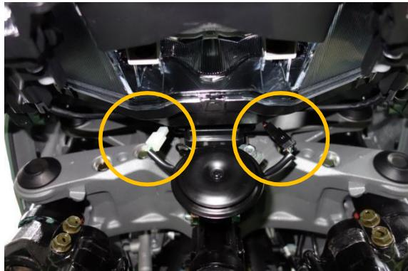
Dismantle the section connecting with the upper lever plate and then lift open the front-left and front-right protection covers. After that, remove the entire unit, lamp and front cover assembly.
