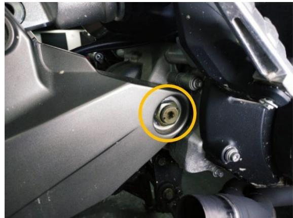
Tightening torque: 900–1100kgf.m
