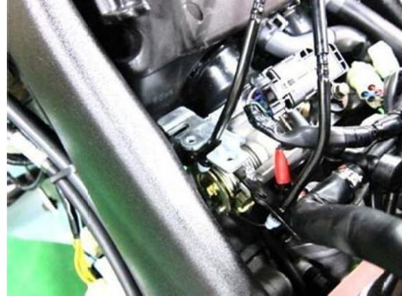
Loosen the Throttle Valve lead wire from the throttle wire securing position of the Throttle Valve.
