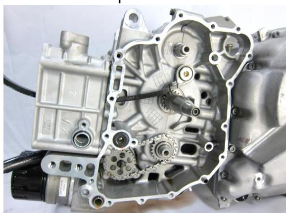
Remove the three bolts and remove the oil pump.
