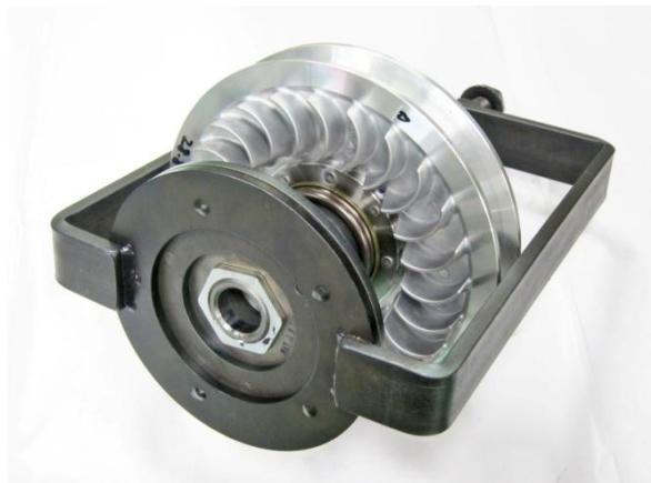
Remove the nuts from the spring compressor of Passive Drive Disc with pliers. Release the spring compressor and then disassemble the Passive Drive Disc.
