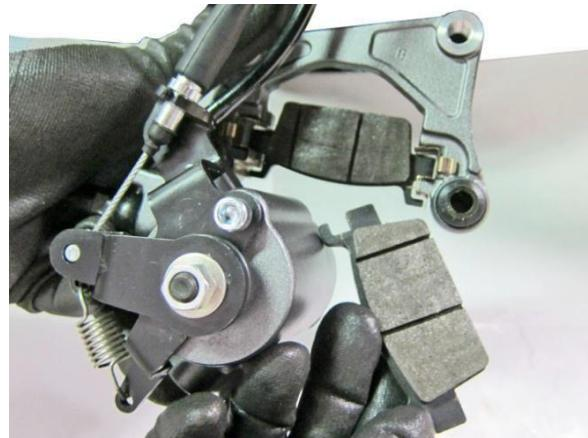
Make new parts replacement if excessively worn or jammed or partially worn.
