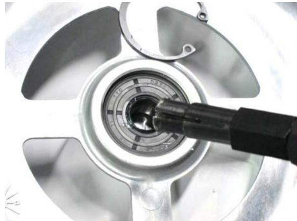
Remove the bolts from the bearing fixing plate and then remove the bearing with the bearing puller.
