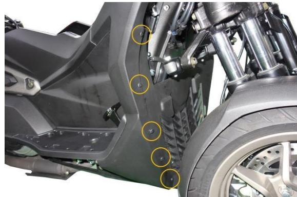
Remove 2 plastic fixing screws hidden underneath the front protection cover.
