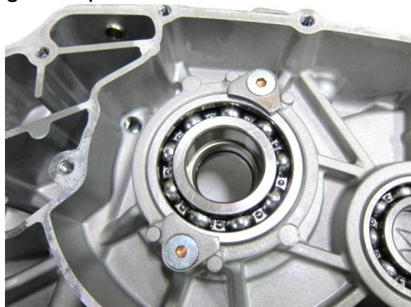
Remove the two bearing fixed plate.
