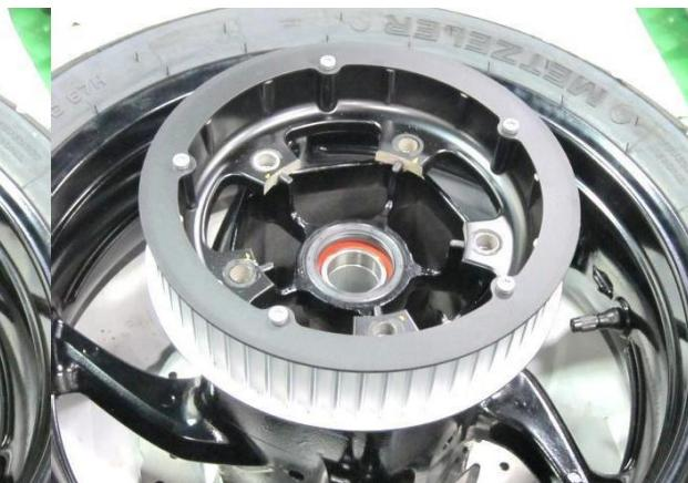
Remove the rear drive pulley of the outer drive belt.
