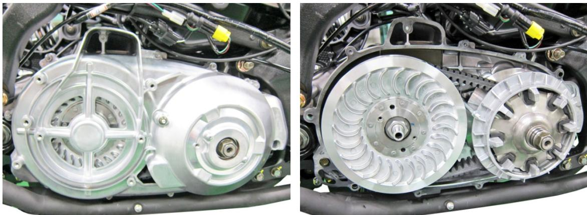
Remove the gasket and two dowel pins.
