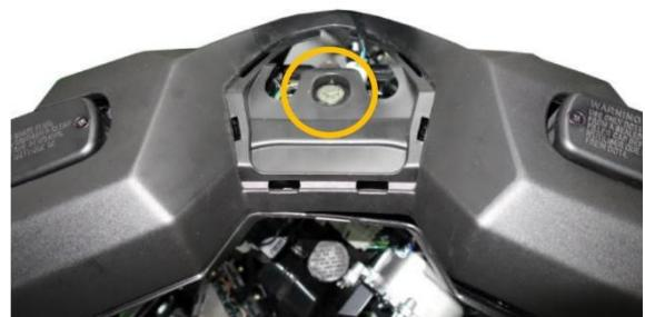
Remove the lower steering handlebar cover.
