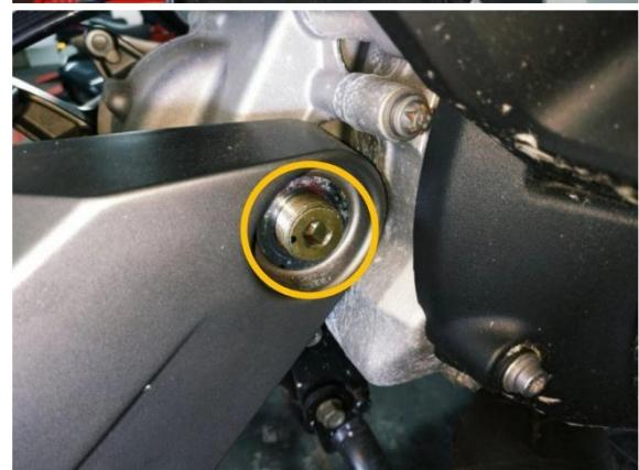
Separate the left and right rear fork assemblies.
