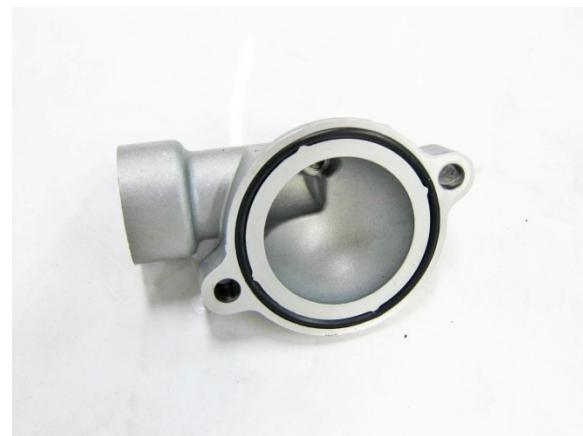
Note: Replace a new seal when installing.
