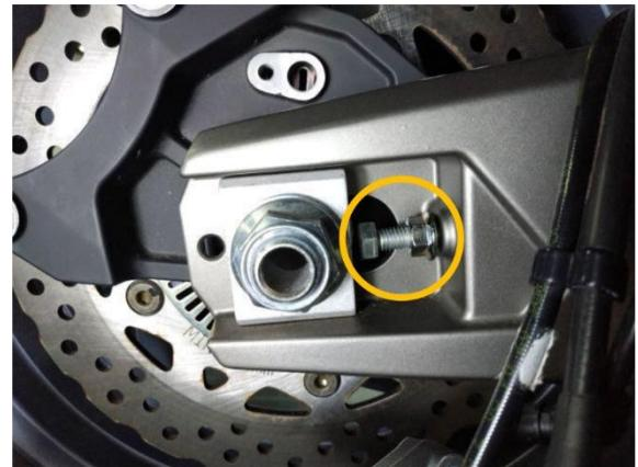
Remove the rear axle mounting nut.
