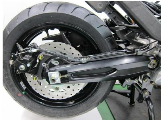
Remove the bolt from the lining pad of rear brake caliper.
