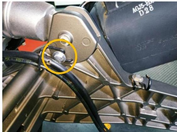
Remove the shock absorber lower screw
