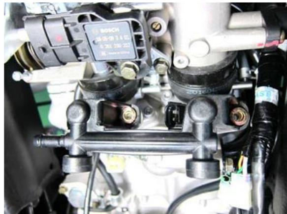
Remove 2 washers from the bolt and then lift the Fuel Injector upward from the intake manifold.
