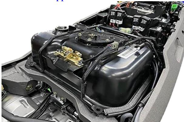
Remove 4 screws from the oil tank support and then remove the oil tank support.
