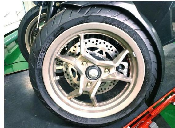
Remove 2 screws from the caliper and then remove the caliper.
