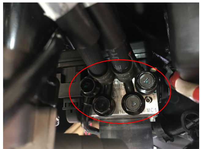
ABS ECU & ABS Hydraulic unit
