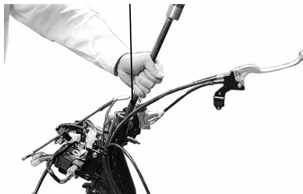
Bottom Cone Race Ball Race Remover
