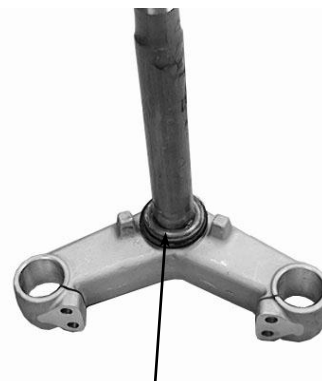
Bottom Cone Race Ball Race Remover
