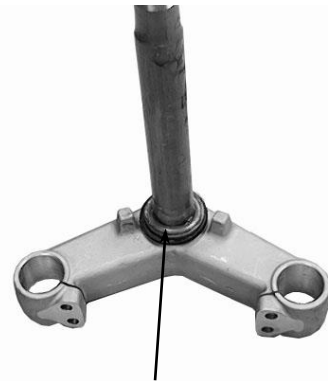
Bottom Cone Race Ball Race Remover
