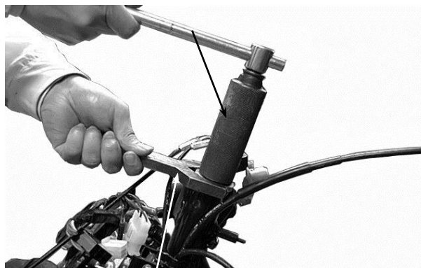
Steering Stem Lock Nut Wrench
