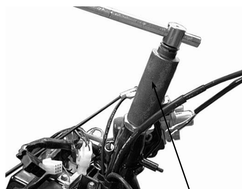
Steering Stem Lock Nut Wrench
